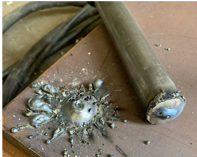
Figure 4.19 - Unsuccessful Stud Weld
