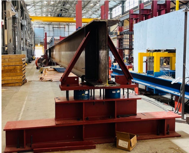
(a) End Brace During Specimen Construction
