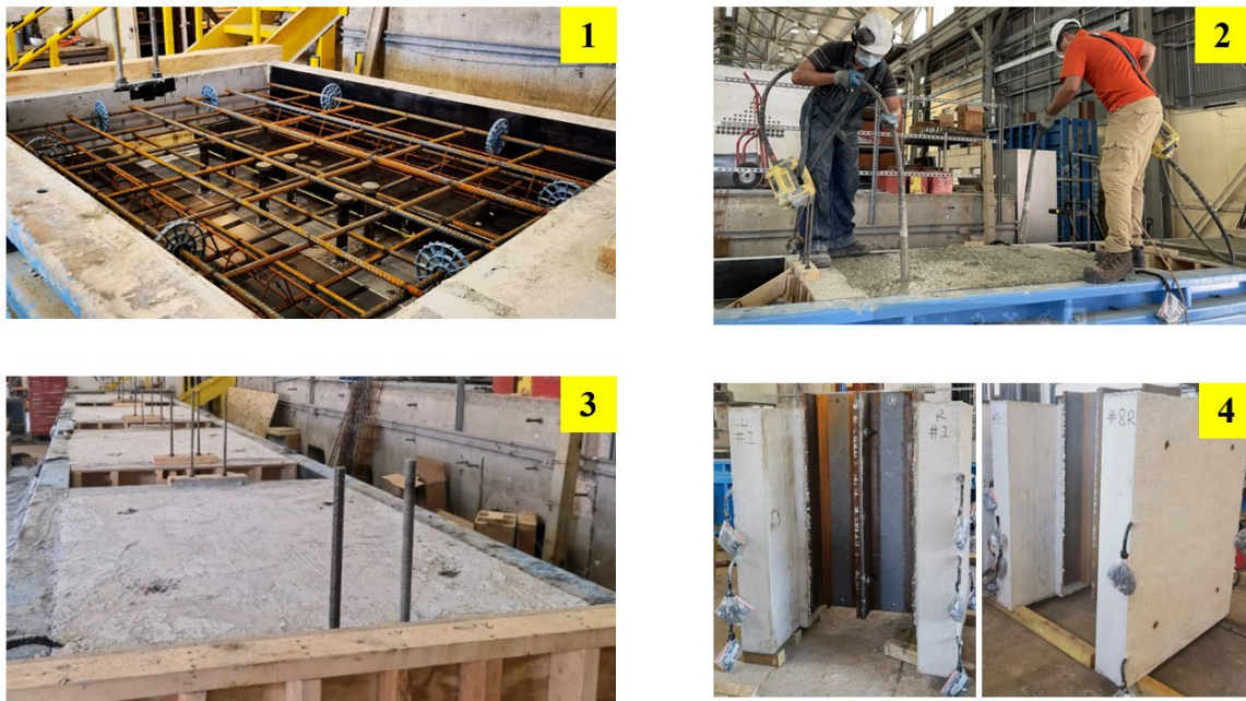
Figure 5.26 - Fabrication Process for Specimen (1) Steel Beam and Reinforcement Placed in the Formwork (2) Concrete Being Cast and Vibrated (3) Concrete Being Cured Inside the Formwork (4) Specimens Removed from the Formwork
