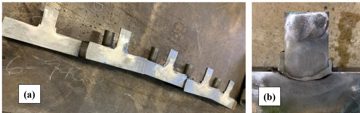
Figure 4.22 - Macro Etch Weld Test. (a) Welds Are Cut in the Middle and Polished, (b) Cross-Section of a Weld Treated with Nitric Acid
