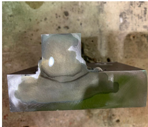
Figure 4.30 - Macro Etch Weld Test for 1" Diameter Shear Stud Welded on 1" Thick Plate
