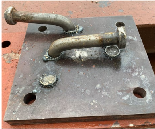
Figure 4.38 - Failed Bend Test for 1-1/8" Studs Using Counterclockwise Cable Loop, Straight Polarity, and No Surface Preparation
