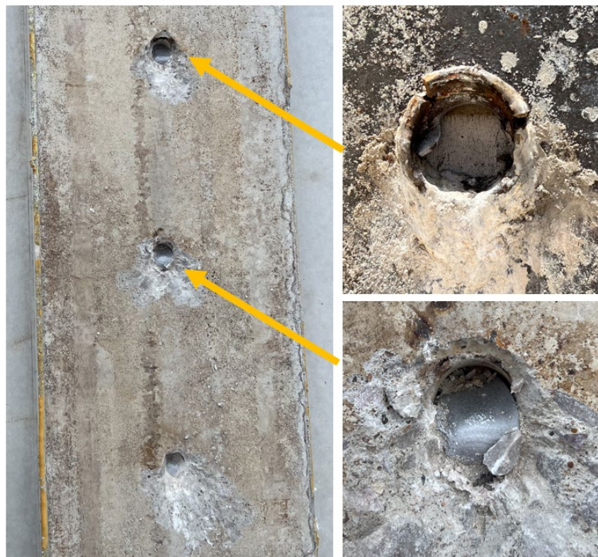
Figure 6.5 - Specimen No.2F: Concrete Deck After Failure with Enlarged Photos of Studs
