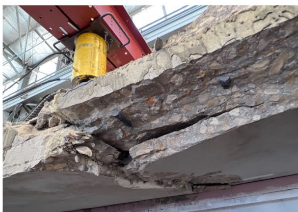
Figure 8.99 – Beam Specimen No. 2 – East Side of Crushed Section of Deck
