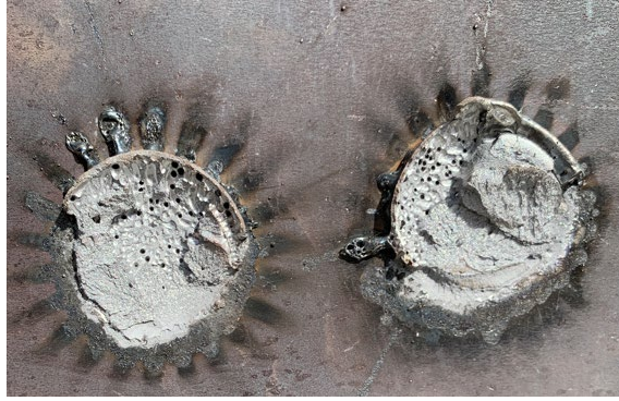
Figure 4.49 - 1-1/4" Studs Welded Using 2275A, 1.45s, S Polarity, Surface Preparation, One Clockwise Cable Looping on 1" Plate. Fracture Section of Failed Bend Tests.
