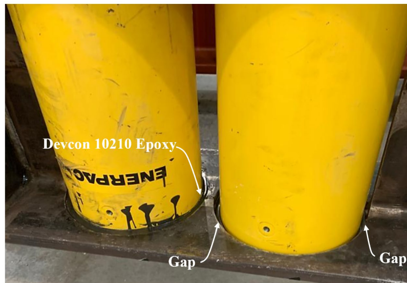
Figure 5.22 - Epoxy is Used to Fill the Gap Between Actuators and Lateral Support
