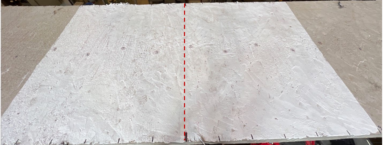
Figure 8.65 – Beam Specimen No. 1 - Portion of Deck over Interior Support Prepared for Tracking Cracks
