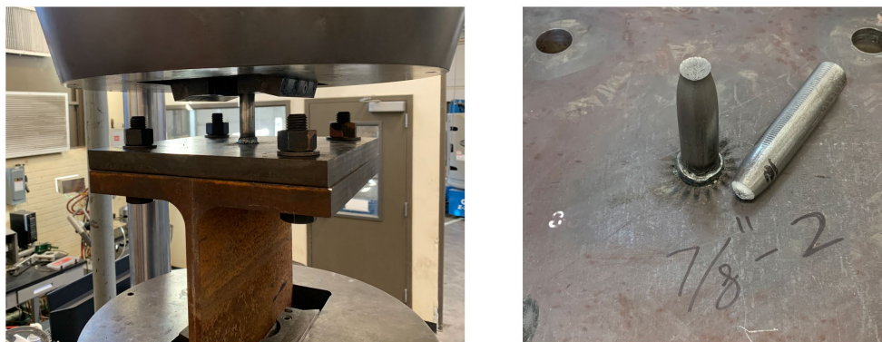
Figure 4.21- Weld Tension Test Setup and a Successful Test
