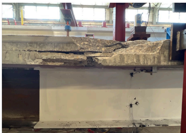
Figure 8.100 – Beam Specimen No. 2 -West Side of Crushed Section of Deck
