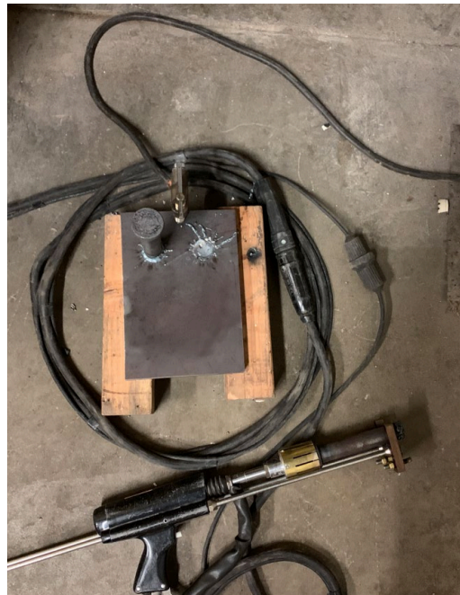
Figure 4.7 - Cable Looping Around the Welding Point
