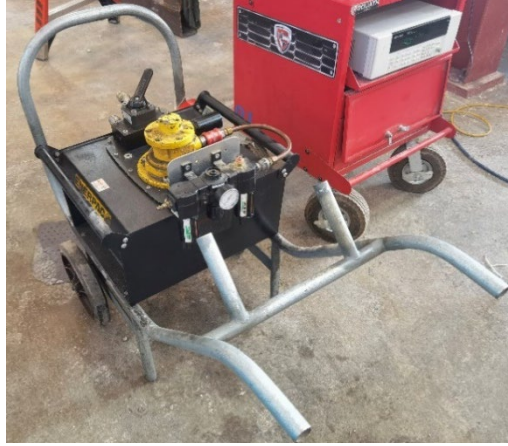
Figure 5.23 - Air Powered Hydraulic Pump
