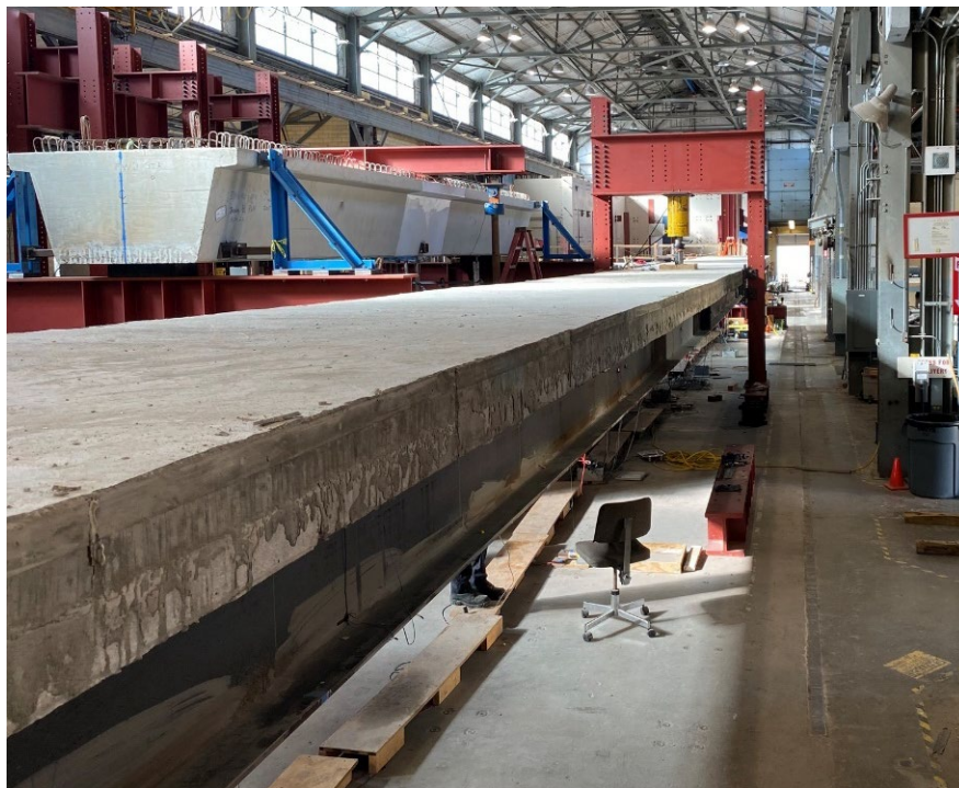
Figure 8.95 – Beam Specimen No. 2 Prior to Single-Span Test
