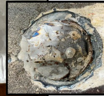
Figure 8.79 - Macro-Etch Test Results for Bright Spot Failure Mode
