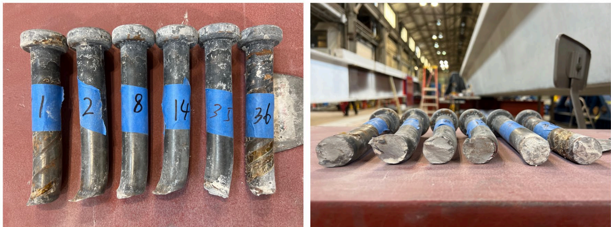
Figure 8.83 – Deformed Shape of Fractured Shear Studs
