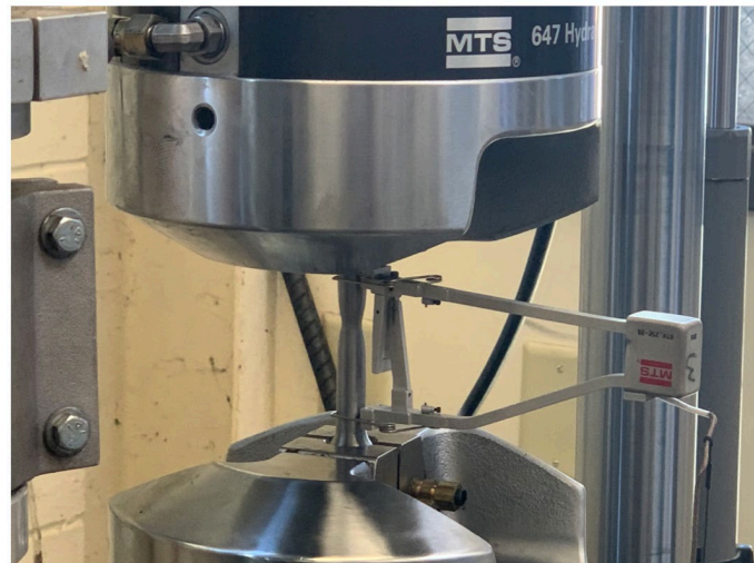
Figure 4.10 - Tension Coupon Test Setup
