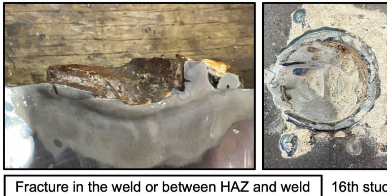
Figure 8.82 – Macro-Etch Test Results for Wide Crater Failure Mode
