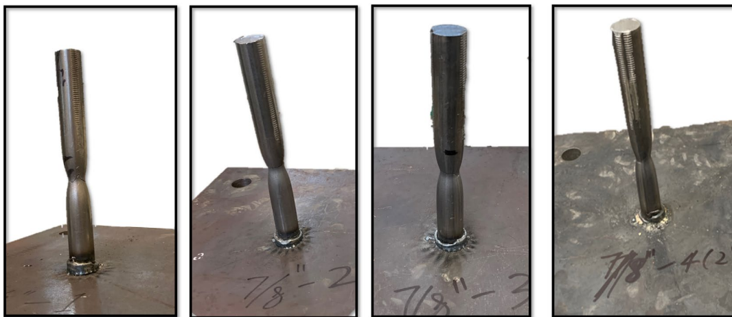
Figure 4.25 - Weld Tension Tests for 7/8" Studs
