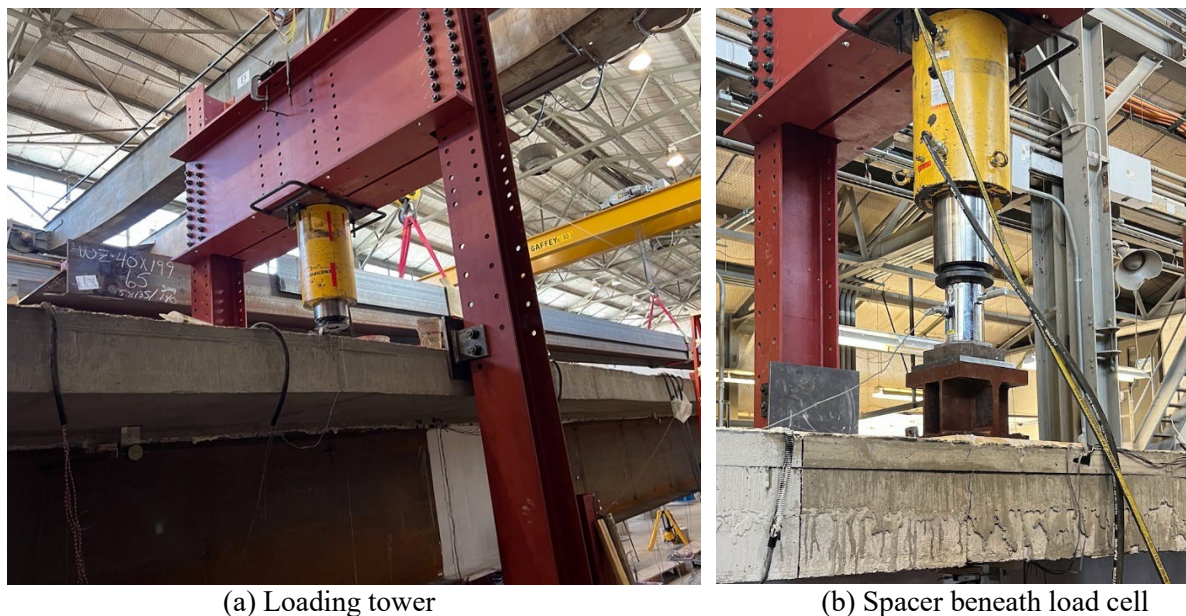
Figure 8.21 – Photos of Loading Tower
