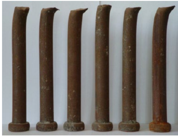
Figure 2.6 - Example of Shear Stud Fracture in a Push-out Test (Xue, et al. 2012)
