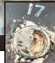
Figure 8.81 – Macro-Etch Test Results for Deep Fracture Failure Mode
