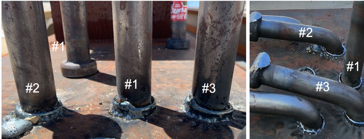
Figure 4.52 - 1-1/4" Studs on Girders with 3.5" Thick Flange Welded Using 2500 amps, 2 s, R Polarity, No Cable Looping, No Surface Preparation
