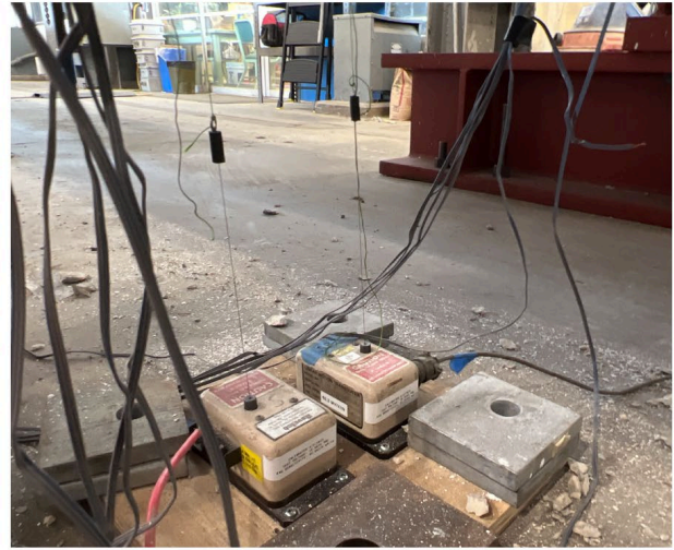
Two SPs at middle span
