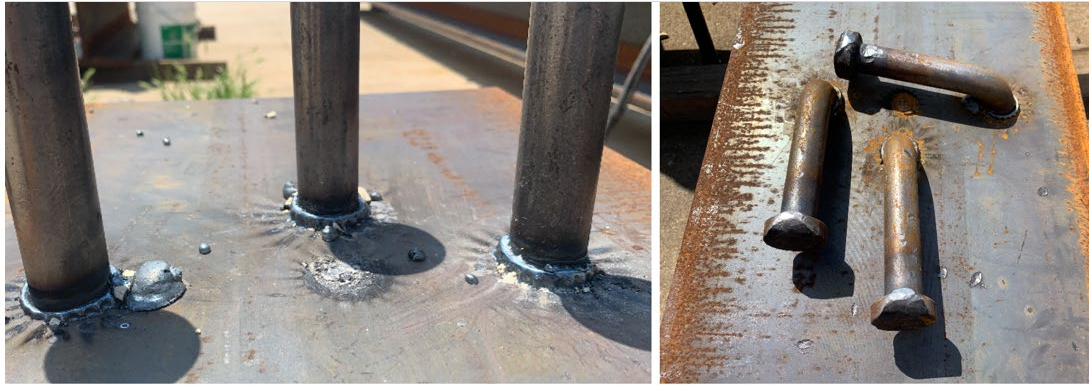
Figure 4.45 - 1-1/8" Studs Welded Using 2250A, 1.55s, R Polarity, No surface Preparation, No Cable Looping on a W14×99 Girder. 90° Bend Test Results
