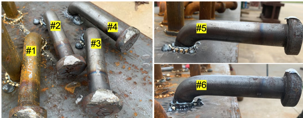
Figure 4.44 - 1-1/8" Studs Welded Using 2250A, 1.55s, R Polarity, No Surface Preparation, No Cable Looping on a W14×132 girder. 90° Bend Test Results
