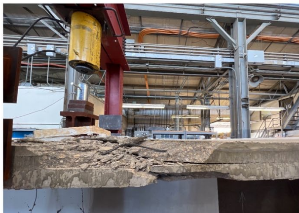
Figure 8.99 – Beam Specimen No. 2 – East Side of Crushed Section of Deck
