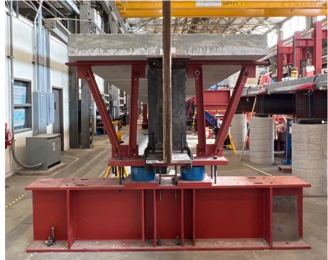
(b) End Brace for Specimen after Construction
