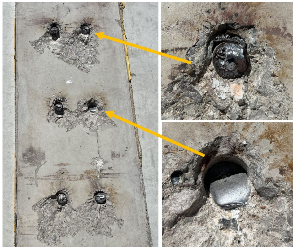
Figure 6.8 - Specimen No.4F: Concrete Deck After Failure with Enlarged Photos of Studs
