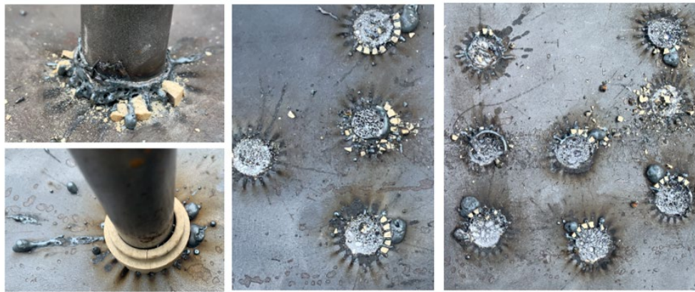
Figure 4.40 - 1-1/8" Studs Welded Using 2050A, 1.3s, S Polarity, One Clockwise Loop, and Surface Preparation on a W14×132 Girder. Weld Collar (left photos) and Fracture Surfaces After Bend Test (center and right photos)
