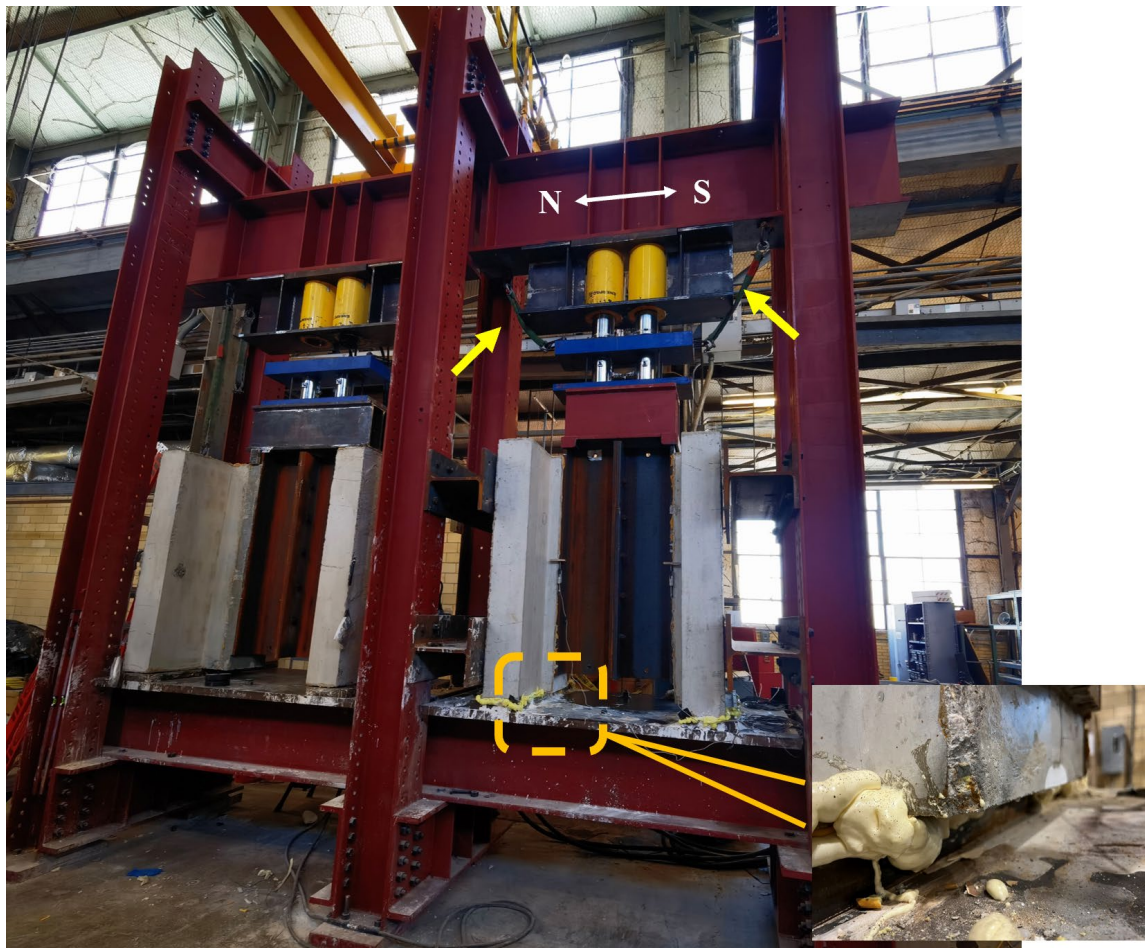
Figure 5.21 - Photo of Specimens in the Test Setup with Enlarged View of the Haunch Bottom - Safety Measures for Load Assembly Can Be Seen (With Arrows) Between 4" Thick Load Spreader Plate and W30×211 Load Beam
