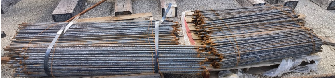
Figure 5.36 - Reinforcing Bars Used in Push-Out Specimens
