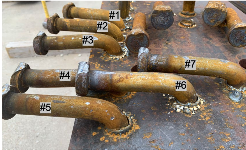
Figure 4.43 - 1-1/8" Studs Welded Using 2250A, 1.55s, R Polarity, No Surface Preparation, No Cable Looping on a W14×500 Girder with 3-1/2" Thick Flange. 90° Bend Test Results
