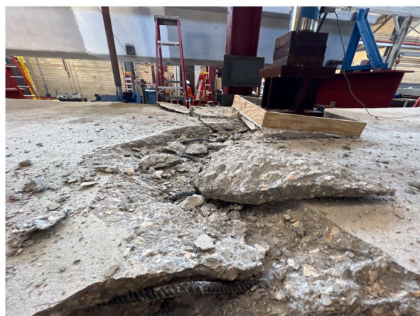
Figure 8.100 – Beam Specimen No. 2 -West Side of Crushed Section of Deck
