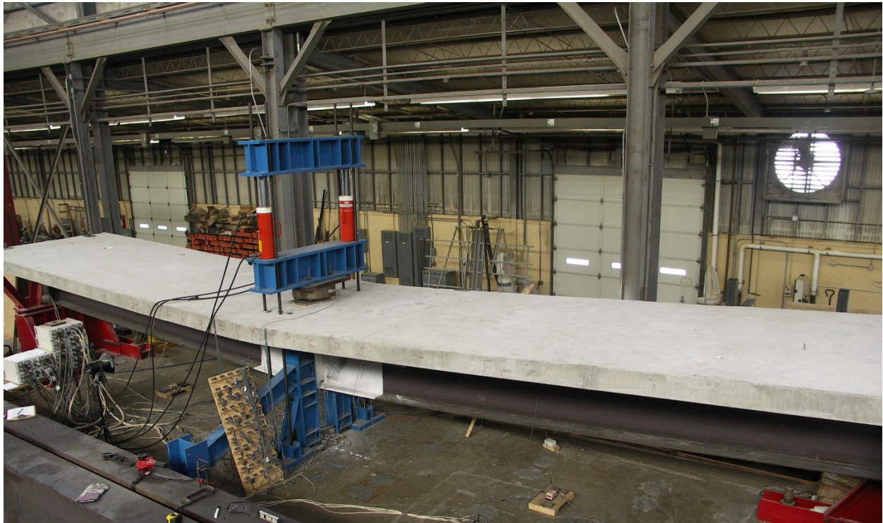
Figure 2.4 - Example of Laboratory Test of a Composite Beam (Kwon, et al. 2007)
