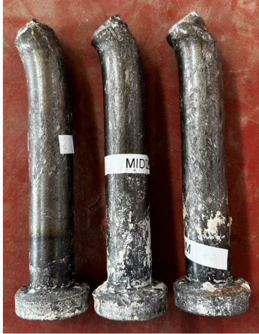
Figure 5.60 – Deformation of Studs After Testing
