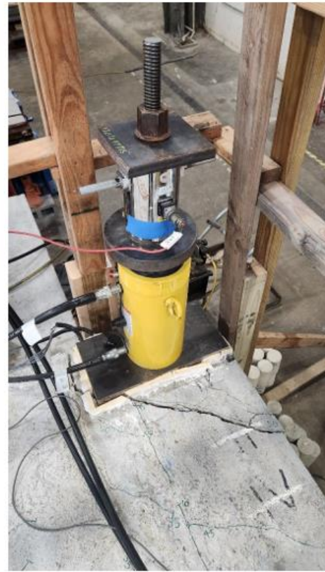
(c) Shear crack from top view
