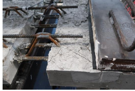
(b) After flexural and shear cracks develop in concrete during load testing
