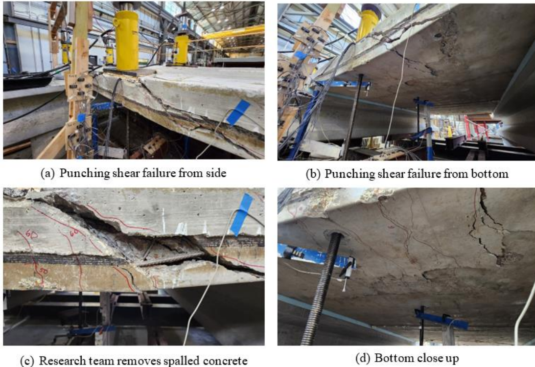
Figure 4-40: Test 8 – Electro-Welded Panel Pair Positive Moment Long Span – Punching Shear at Ultimate Load
