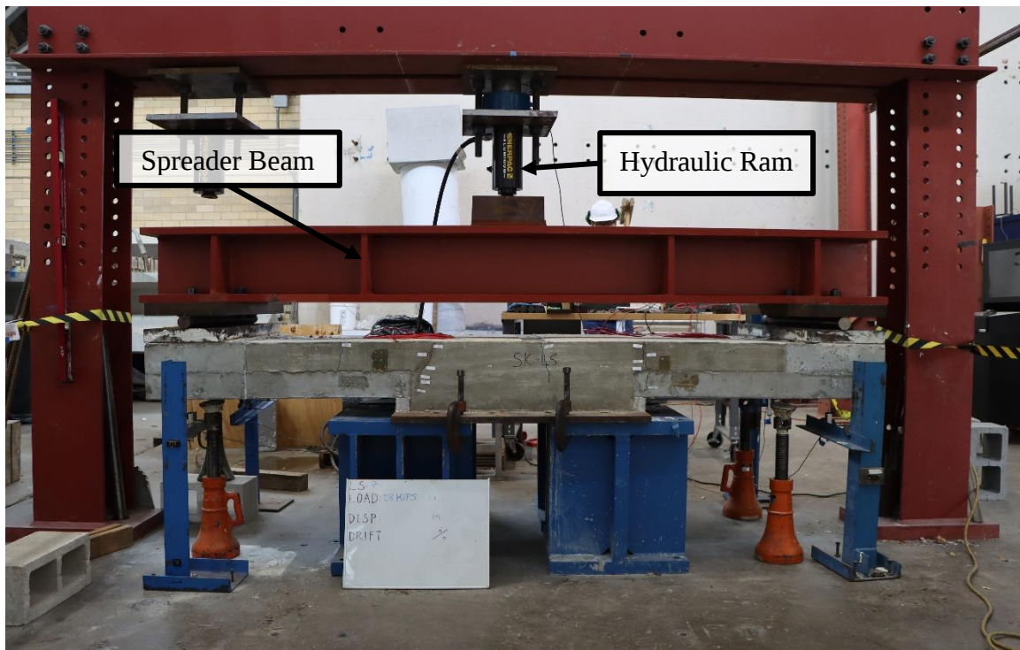
Figure 5-20: Test Setup for Monotonic Loading
