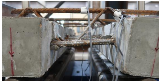
(b) Wire trusses slip out of the panels during loading
