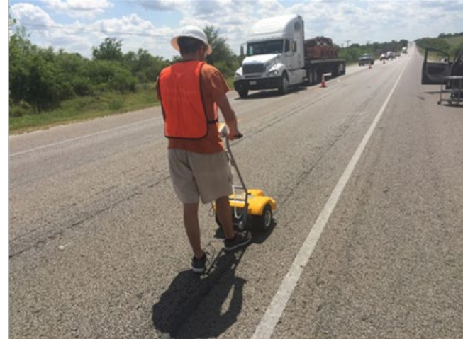
Figure 1.16 Micro-GripTester device (left) and field operation (right)
