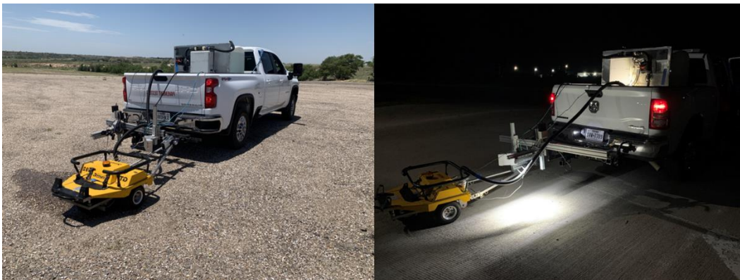
Figure 7: Data collection prototype system during daytime (left) and nighttime (right) conditions.
