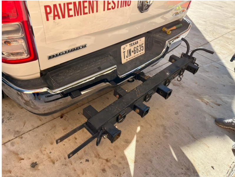
Figure 1: Mounting piece used to adjust the position of the friction trailer.
