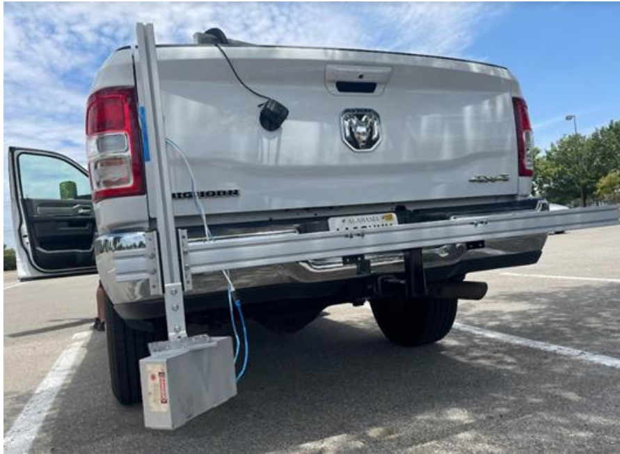
Figure 32: Laser system mounted onto vehicle
