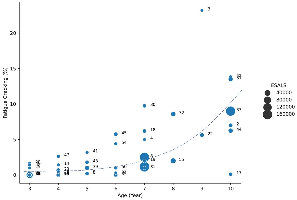
**Figure 4.2. Maximum alligator cracking, age and ESALS of 341D mixtures.**
