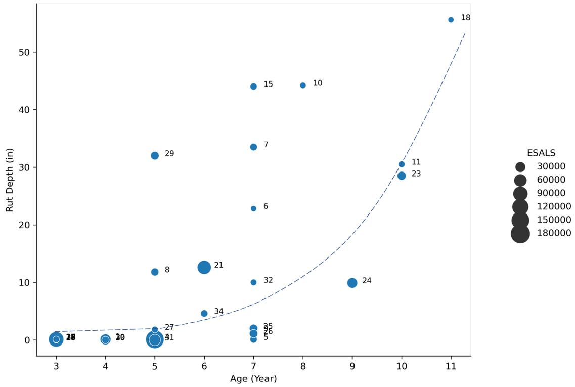
**Figure 4.3. Maximum average rutting, age and ESALS of 341C mixtures (note: The PA standard is to record rutting in inches, however, it is evident that several readings are not in inches).**
