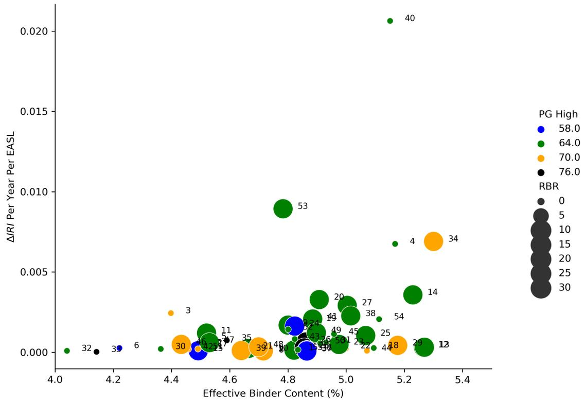
**Figure 4.10. Relation between normalized *IRI* changes and effective binder content of 341D mixtures**
