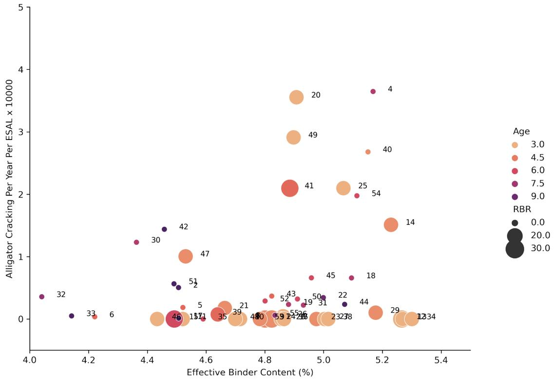
**Figure 4.9. Relation between normalized alligator cracking and effective binder content of 341D mixtures.**
