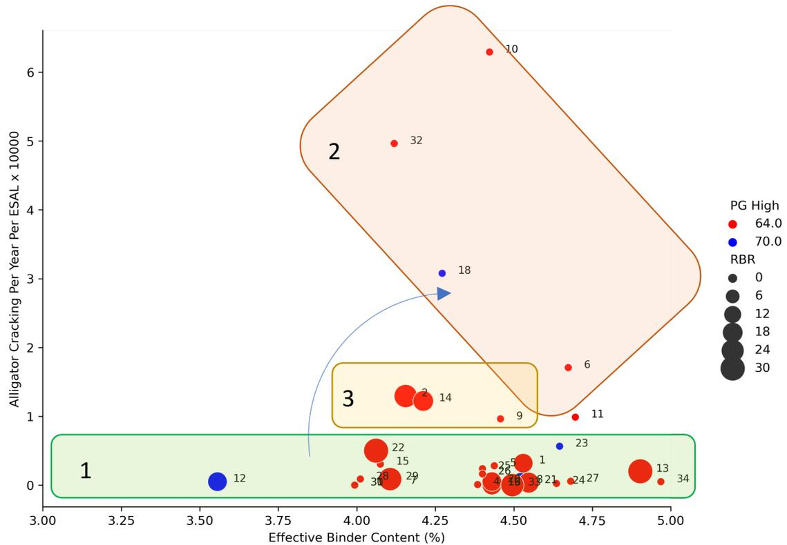
**Figure 4.5. Relation between normalized alligator cracking and effective binder content of 341C mixtures.**
