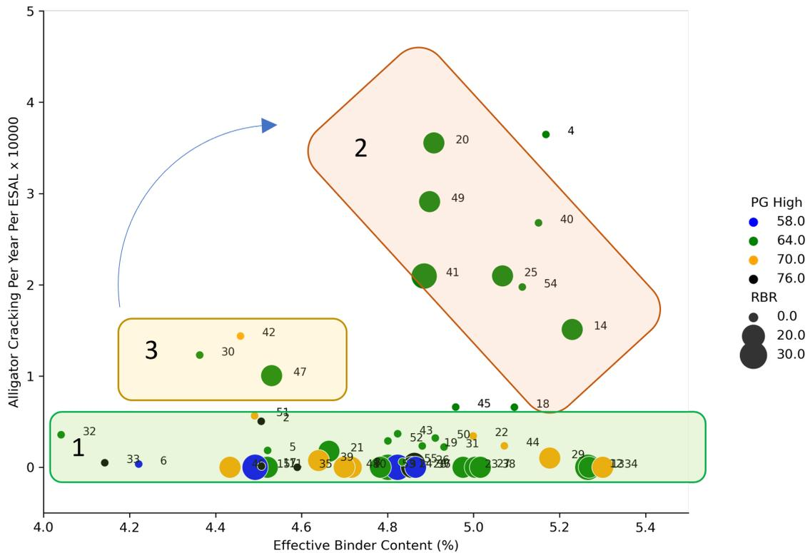
**Figure 4.8. Relation between normalized alligator cracking and effective binder content of 341D mixtures.**
