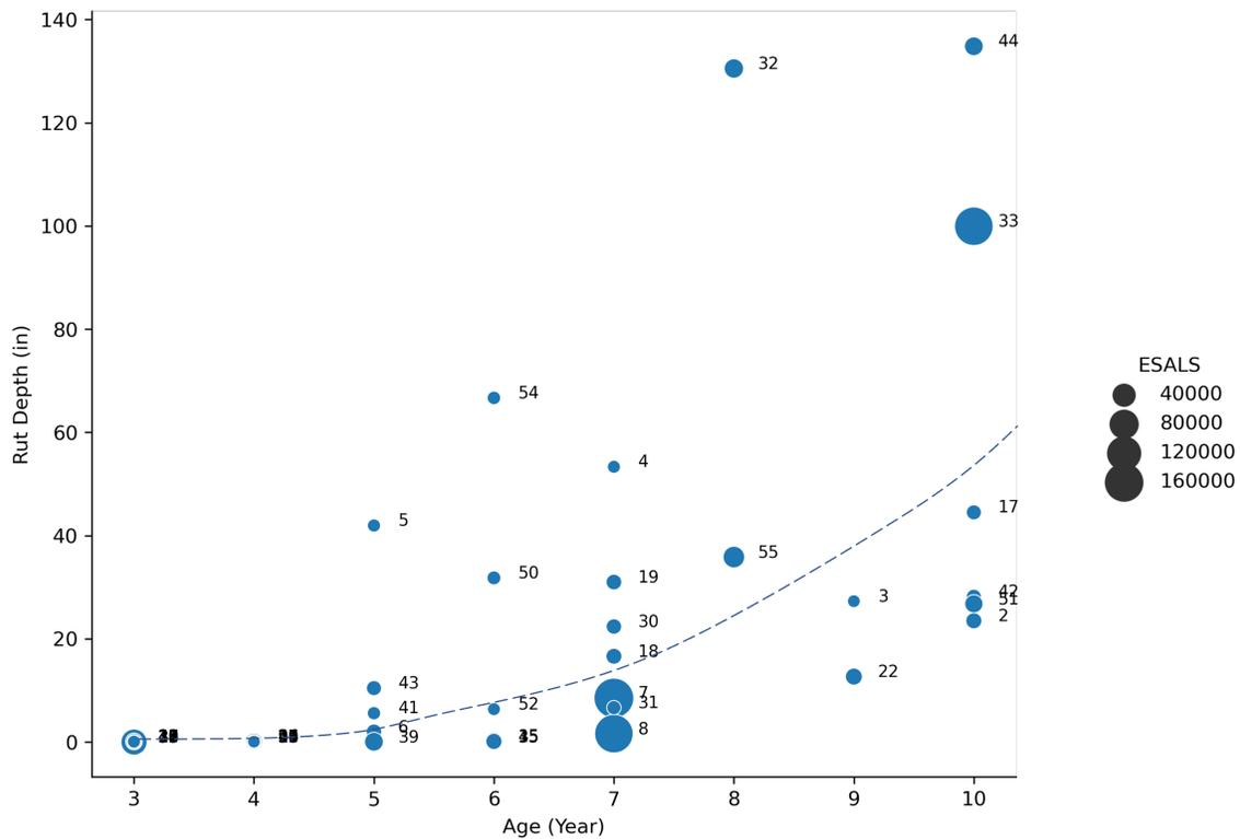
**Figure 4.4. Maximum average rutting, age and ESALS of 341D mixtures (note: The PA standard is to record rutting in inches, however, it is evident that several readings are not in inches).**
