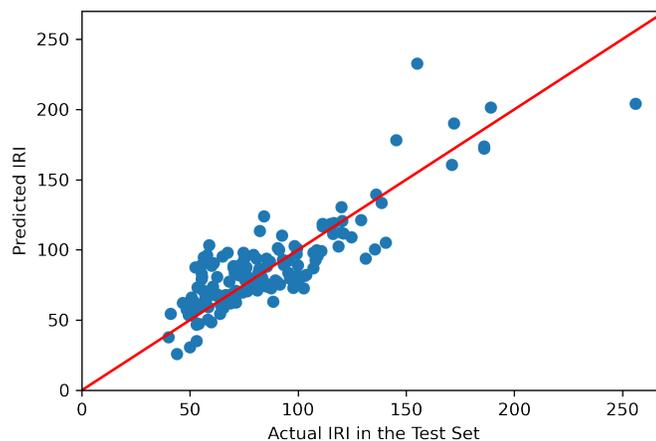
**Figure 3.9. Test Results of the Neural Network Model with IRI as the Dependent Variable**
