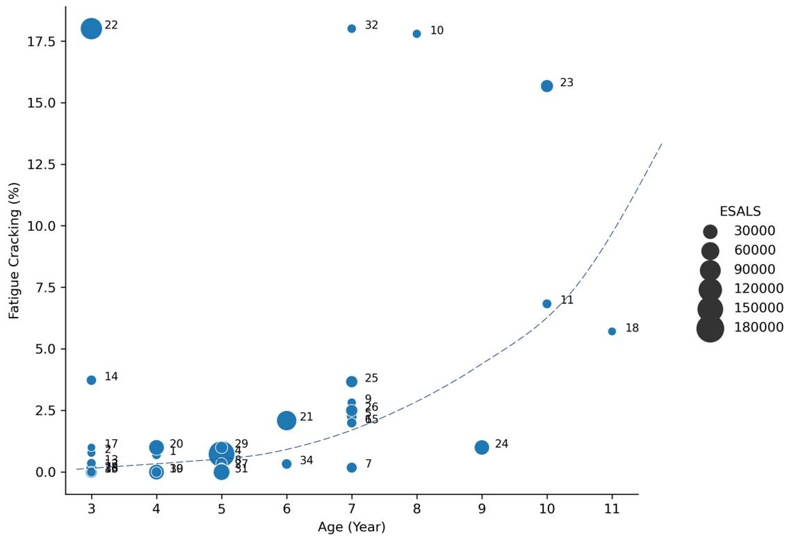
**Figure 4.1. Maximum alligator cracking, age and ESALS of 341C mixtures.**
