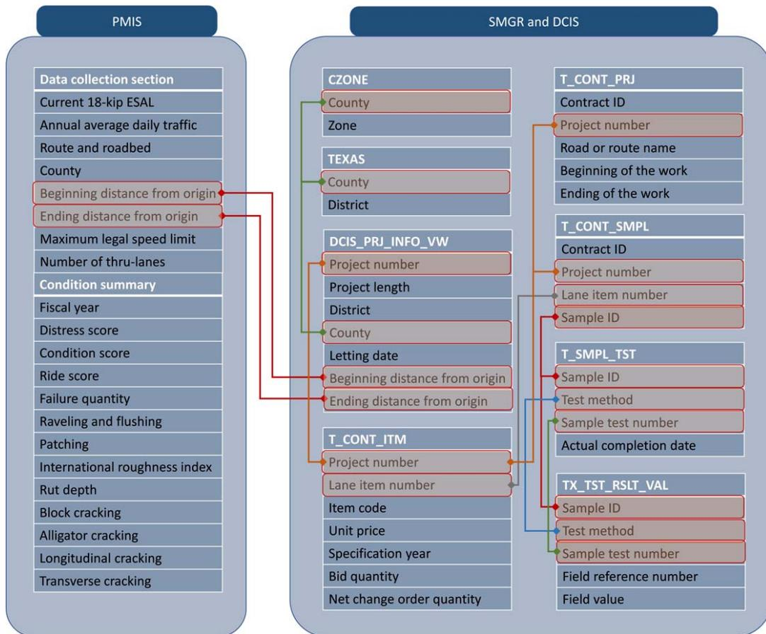
**Figure 2.1. The in-house data repository with tables and data fields relevant to this work. The common primary keys that can be used to integrate different tables from different sources are highlighted.**
