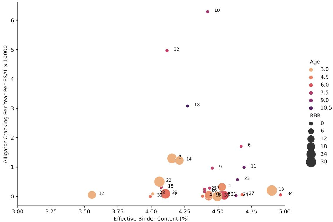
**Figure 4.6. Relation between normalized alligator cracking and effective binder content of 341C mixtures.**
