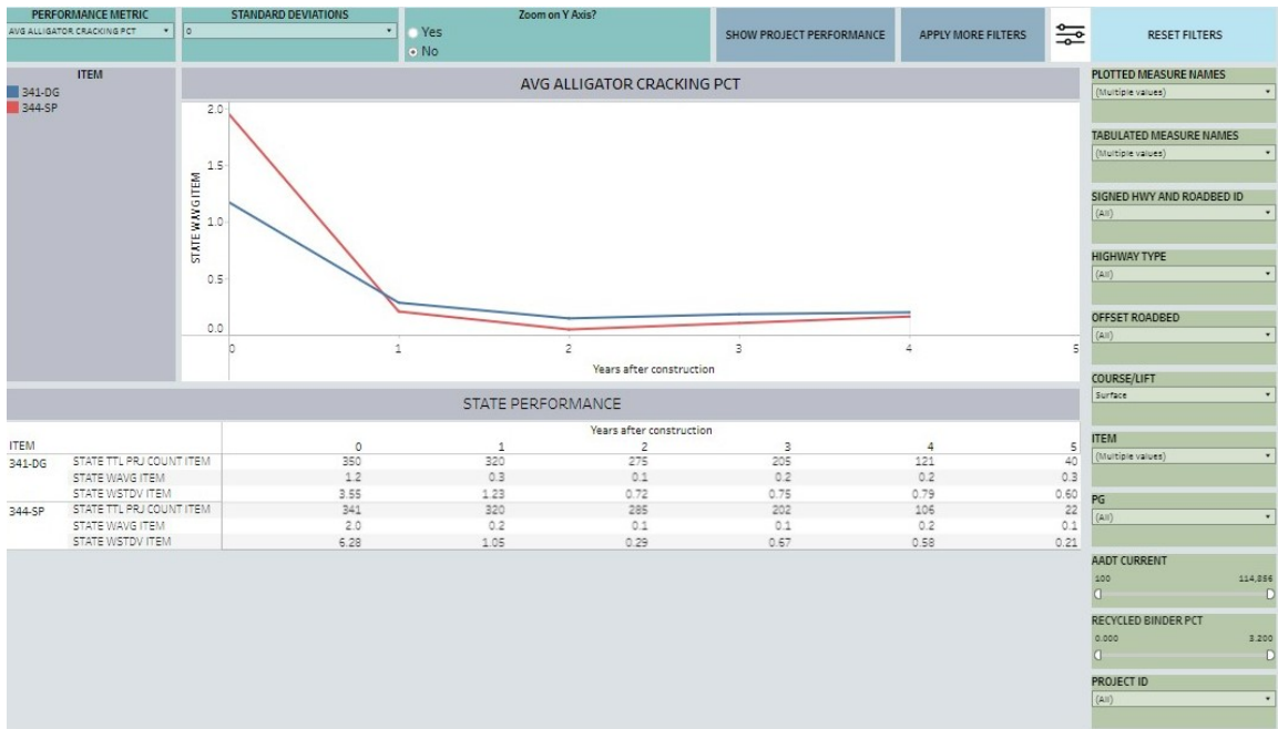
Figure 3.4. Tableau dashboard showing the average alligator cracking for different items over time.
