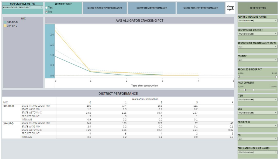
Figure 3.8. Tableau dashboard showing the weighted average percentage of alligator cracking for different mixes.
