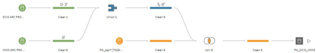
Figure 2.8. Tableau Prep Builder flow integrating the pavement condition information from the “PA-perf” data-source (Figure 2.5) with the DCIS (Figure 2.6) and MMS (Figure 2.7) project and location information.
