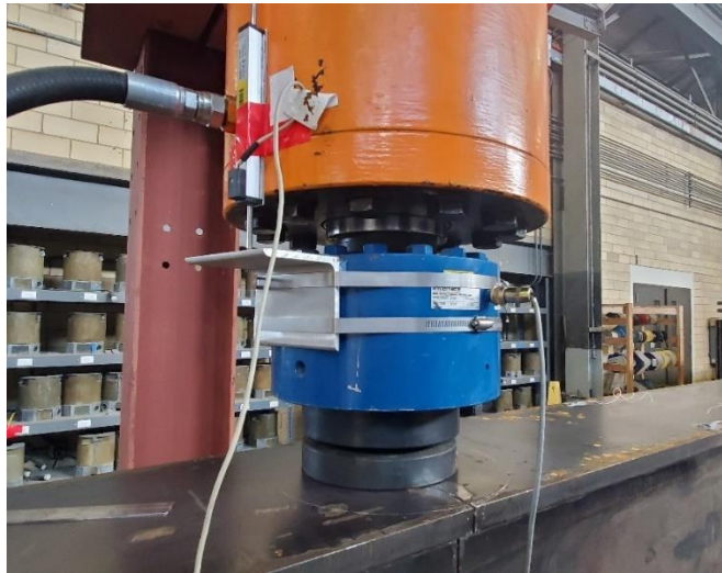
Figure B.9: Hydraulic ram with 200-kip Interface load cell for force feedback and linear potentiometer for displacement feedback
