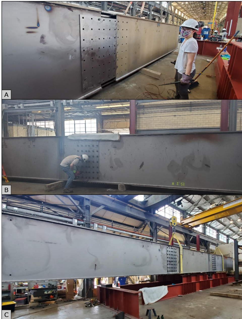
Figure 4.12: Test specimen assembly sequence: (A) fitting of the North end segment to the test segment; (B) tightening of bolted splices; and (C) lifting of the assembled test specimen.
