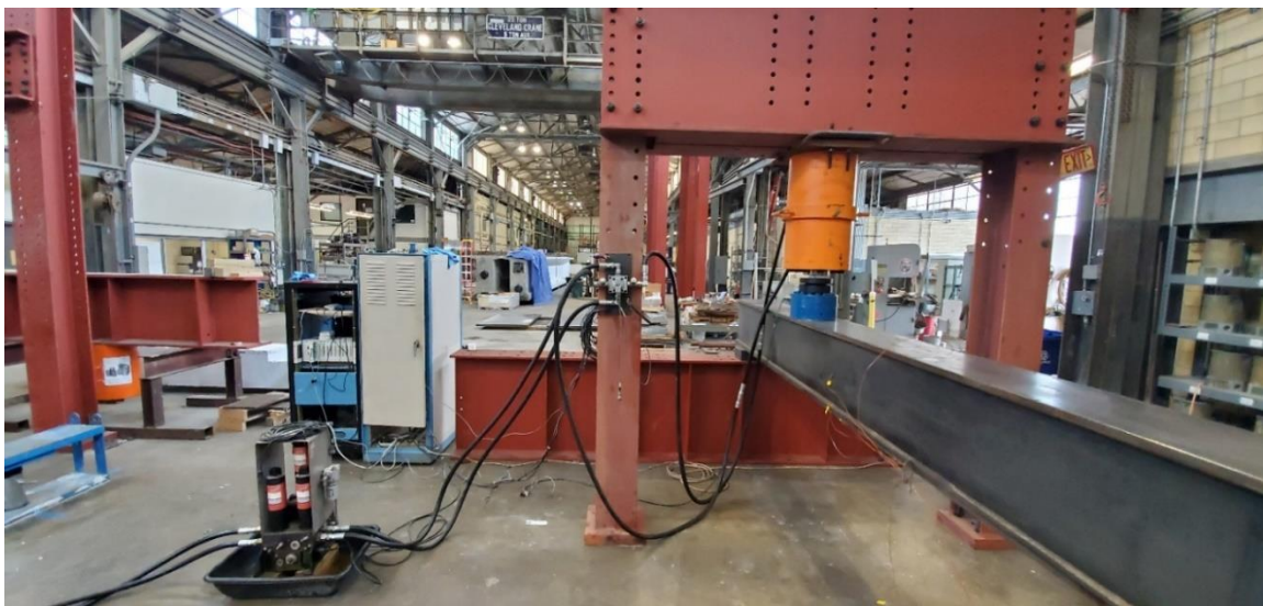
Figure B.10: Closed-loop system setup for pilot specimen cyclic loading
