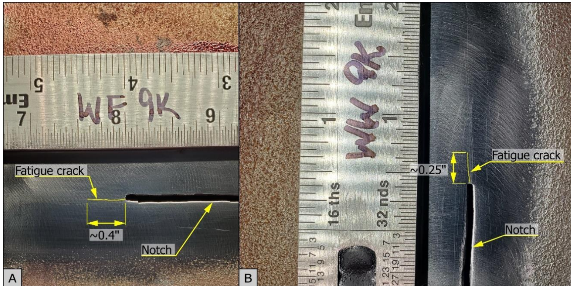
Figure 5.4: Baseline Specimen: fatigue cracks emanating from notches: (A) West flange and (B) West web
