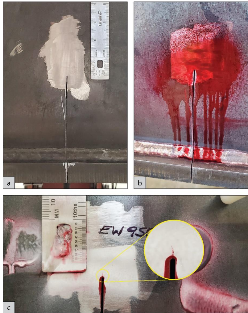
Figure B.13: Crack inspection using dye penetrant method. (a) Notch tip area polished and cleaned; (b) application of penetrant dye on the notch tip area; (c) developer application that allows the observation of the fatigue crack.
