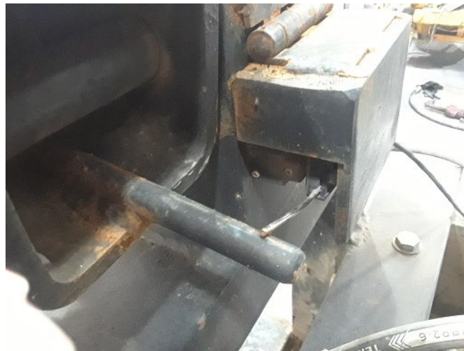
Figure 3.11: Successful plow rig extension and rotating limit switch on 4498-H
