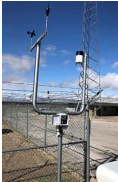
Figure 6.2: RX3000 weather station installed at a TxDOT facility in the Abilene area
