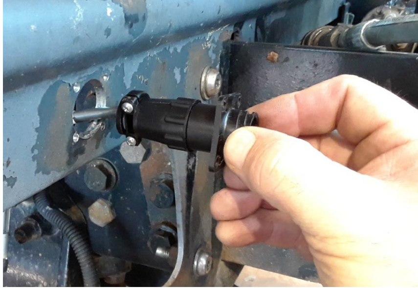
Figure 3.8: A hole is drilled on the bumper to install the cable plug assembly.
