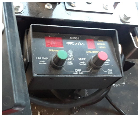
Figure 3.6: Spreader control box
