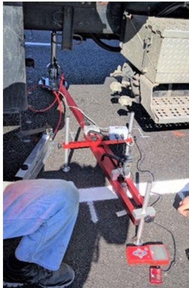
Figure 6.13. UT's static plate load test apparatus with loaded truck as reaction.
