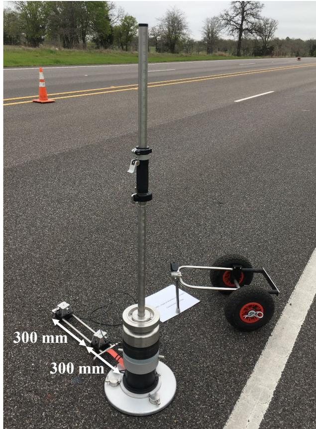
Figure 6.16. UT's light weight deflectometer during testing.
