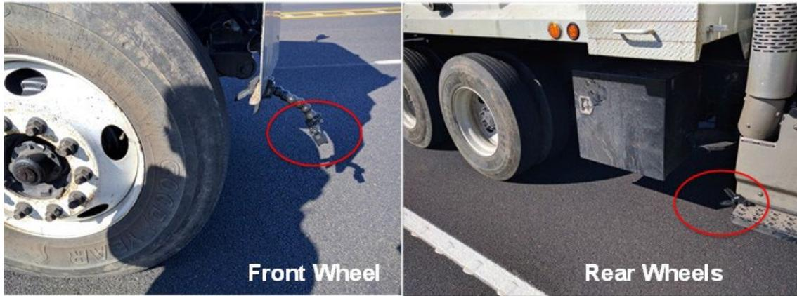
*Figure 8.4. GoPro cameras mounted to capture front and rear wheel paths.*
