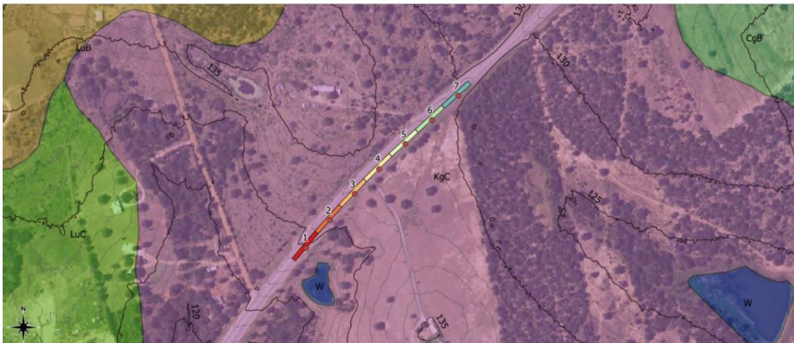
Figure 4.1. USDA soil map and USGS elevation data from site of instrumented test sections at SH-21.
