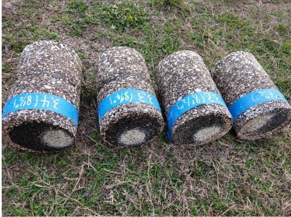
**Figure 4.28. Pavement cores collected from field test sections.**
