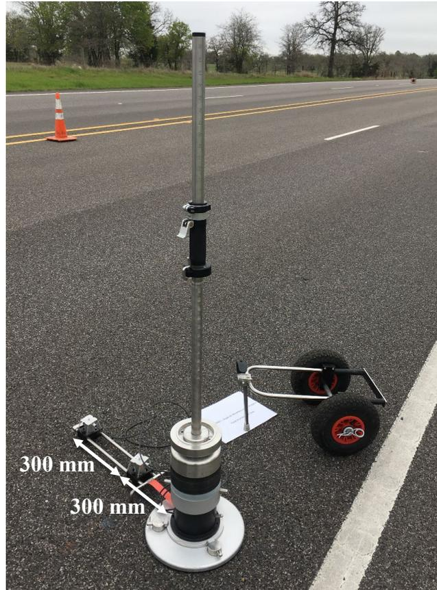
Figure 7.15. UT's light weight deflectometer during testing.
