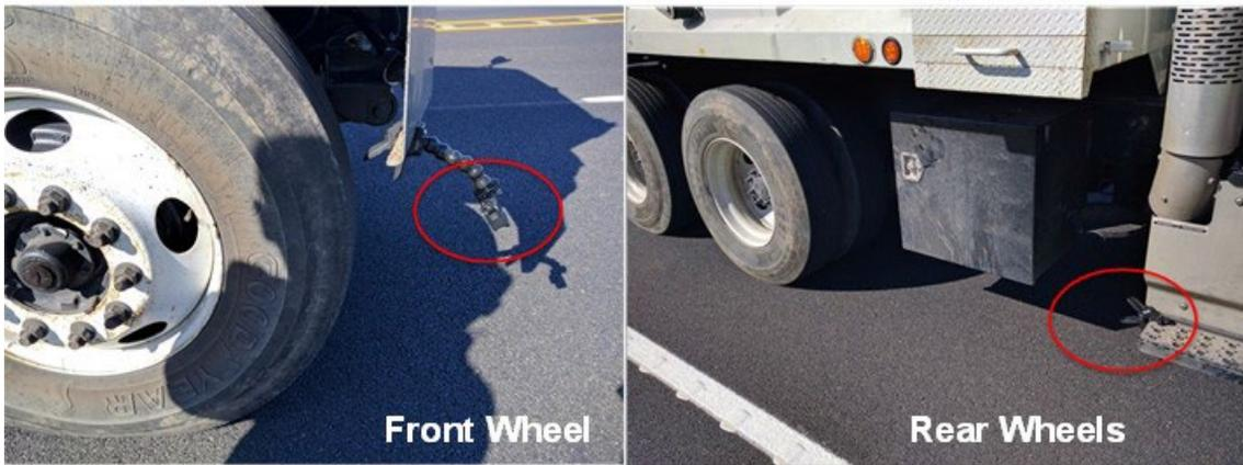
Figure 6.6. GoPro cameras mounted to capture front and rear wheel paths.
