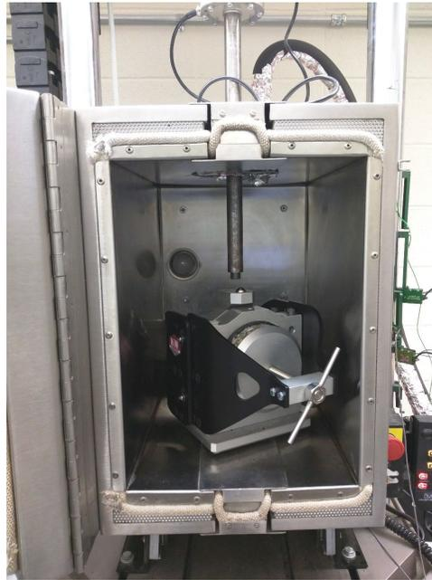
***Figure 4.30. Asphalt-reinforcement interface shear test.***
