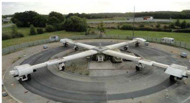
Figure 2.26. Photograph showing IFSTTAR fatigue test carrousel (IFSTTAR, 2012).
