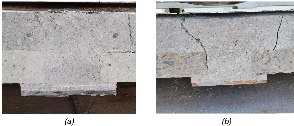
Figure 7.1 1 inch panel to girder gap check: (a) 1.5 inch hooked end fiber SFRC and (b) 1 inch twisted fiber SFRC
