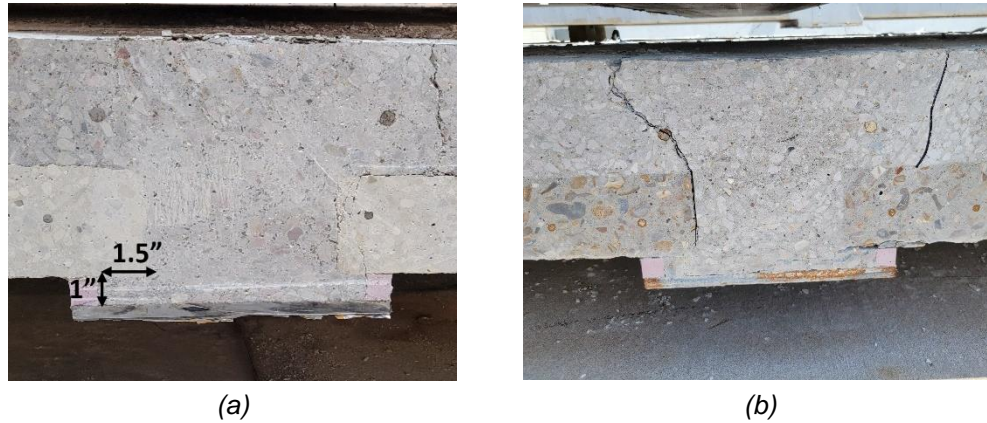
Figure 4.11 Cut cross-section of (a) 1.5 inch hooked end fiber SFRC and (b) 1 inch twisted fiber SFRC specimens
