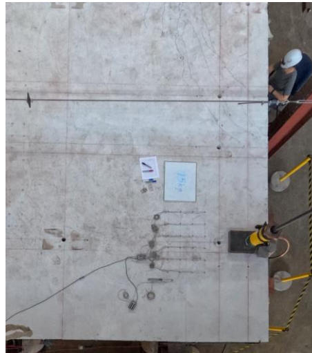
Figure 6.19 Overhang edge loading configuration
