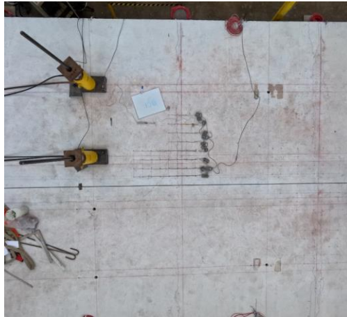
Figure 6.16 Tandem axle near panel joints configuration
