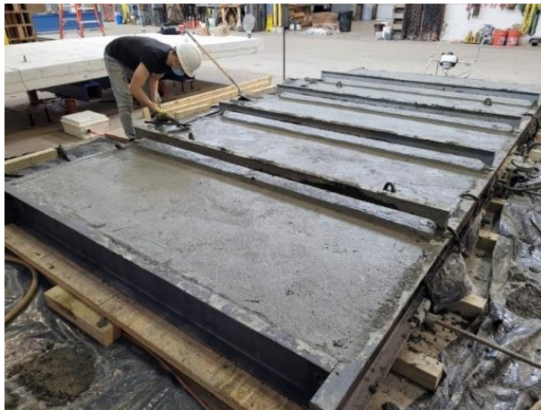
Figure 4.8 Leveling and smoothing of specimen
