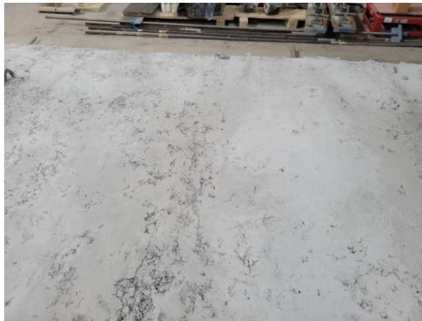
Figure 4.10 Uneven surface of S1-3 specimen due to low slump
