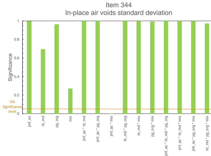
Figure 3.8. ANOVA for standard deviation of Item 344 in-place air voids. Here, jmf_ac denotes the design asphalt content specified in the job mix formula (JMF), rb_md denotes the recycled binder percentage from the mix design, pg_org is the original binder grade, mix is the mix type or aggregate gradation, and wma is warm mix asphalt.
