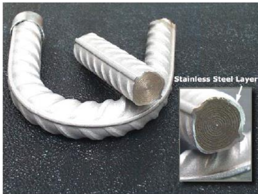
Figure 2.1: Stainless steel-clad reinforcement (Clemena, Kukreja and Napier 2003)
