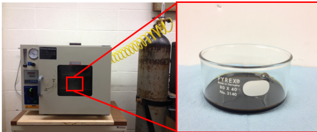
Figure 4.27. Micro-extraction procedure. Drying the solvent using a vacuum oven to obtain the extracted binder
