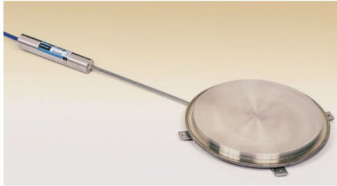
Figure 8.12: Model 4815 earth pressure cell (geokon.com)
