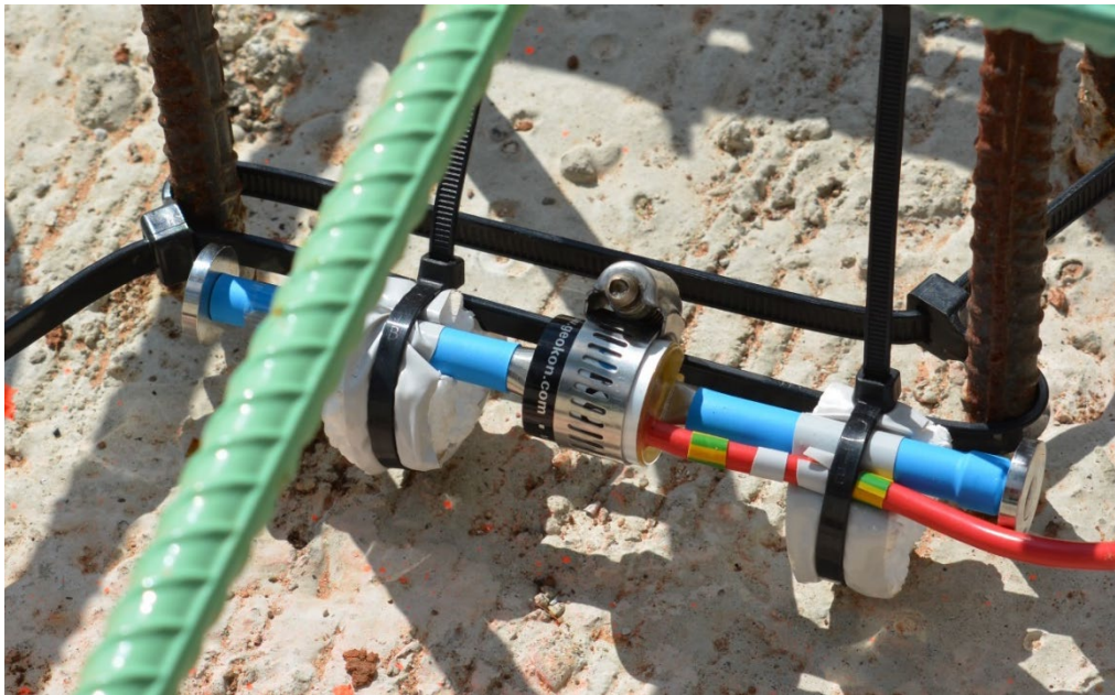
Figure 8.48: Different colored tape represents binary values to help identify sensor
