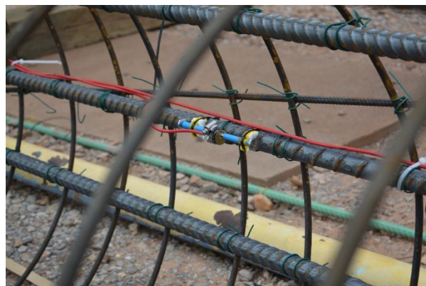
Figure 8.59: Strain gauges attached to long rebars of drilled shafts
