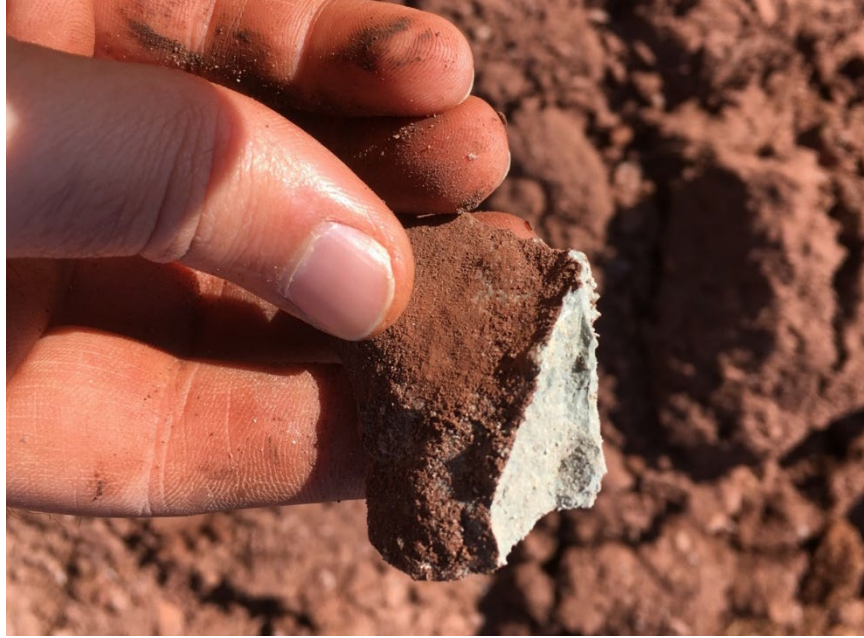
Figure 8.39: Gray shale covered with powdery red dirt recovered from a depth of 30 ft
