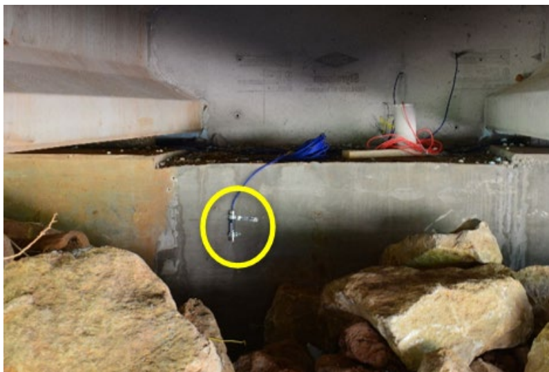
Figure 8.86: Creekside piezometer installed on abutment cap
