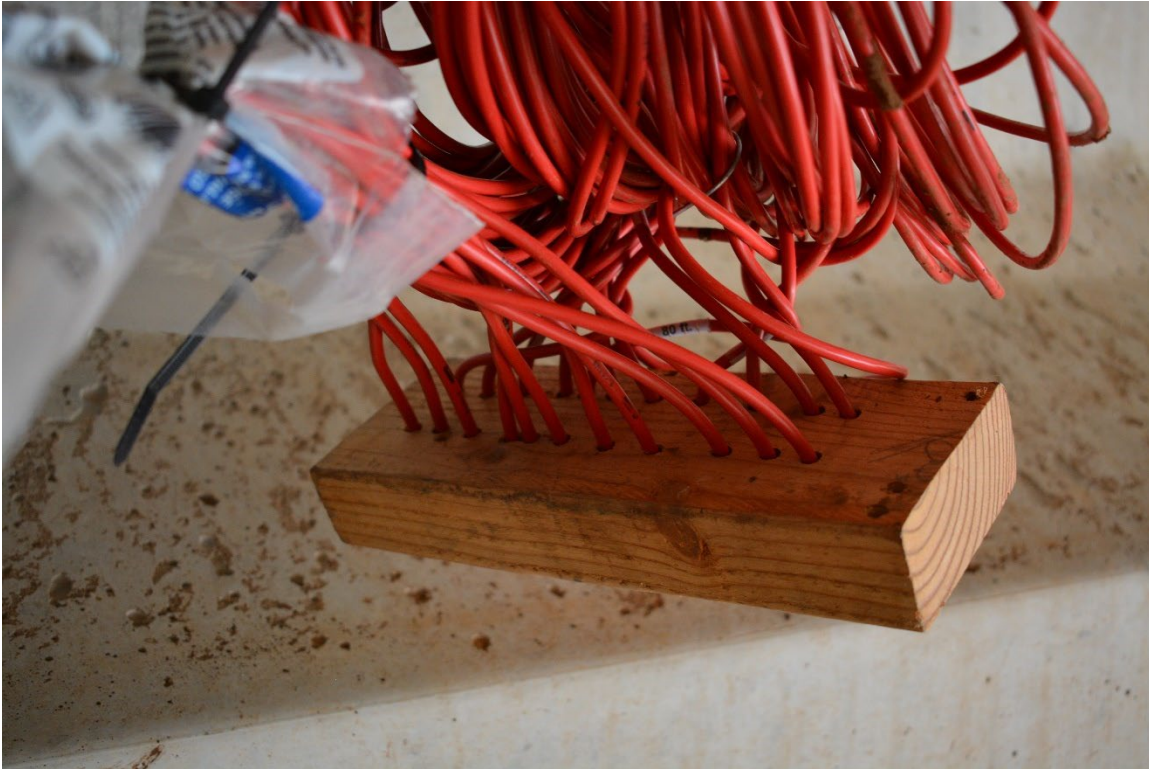
Figure 8.50: Predrilled block of wood used to help keep track of cables coming from embedded strain gauges
