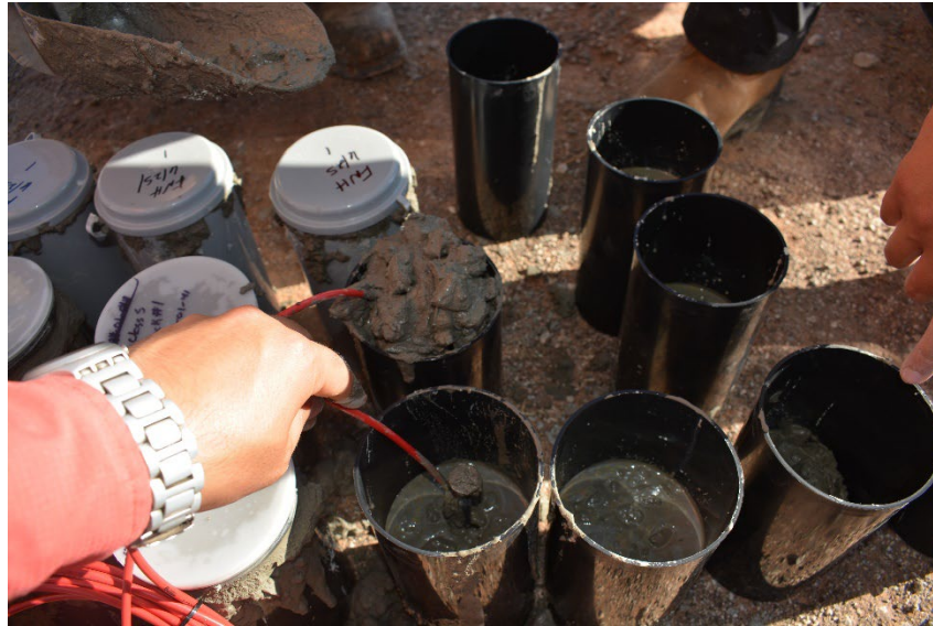
Figure 8.77: Instrumented concrete sample cylinders
