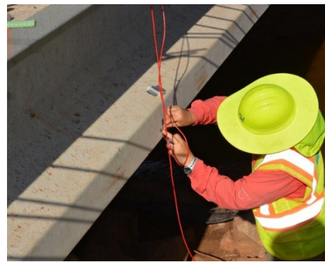
Figure 8.71: Installation of miniature strain gauges on bridge girder: (a) epoxied strain gauge; and (b) strain gauge installation (cables are routed along top flange)
