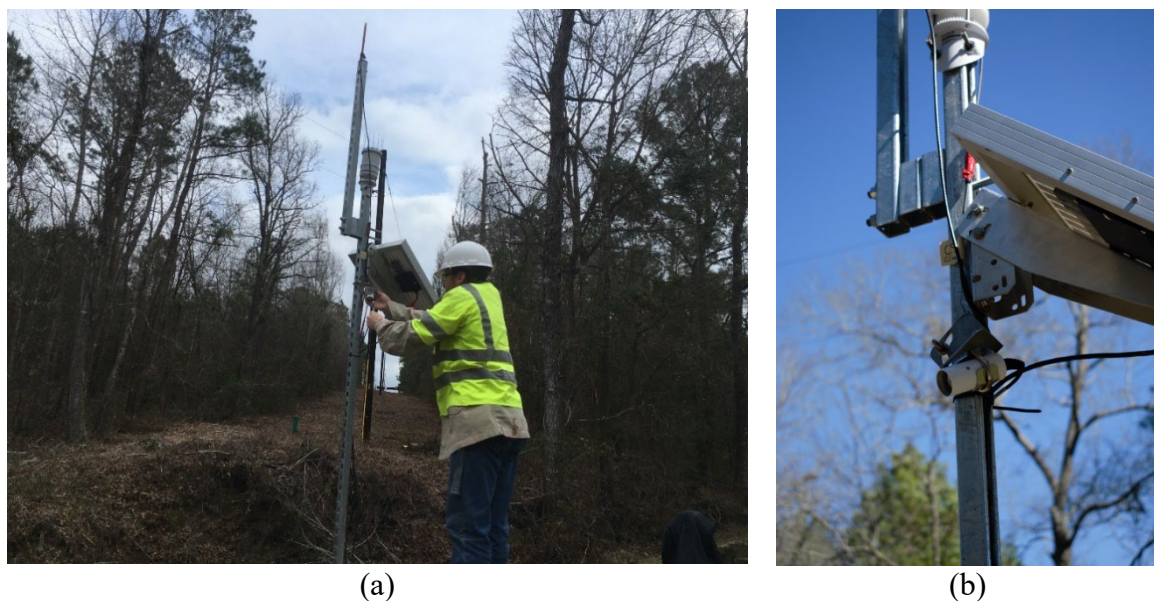
Figure 7.21: Closeup of pole-mounted equipment on south abutment, which includes solar panel, ClimaVue50, SI-111SS and lightning protection device: (a) installation of SI-111SS for measuring deck surface temperatures; and (b) closeup of SI-111SS
