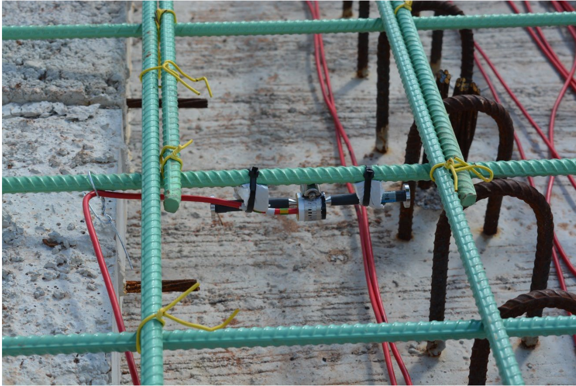
Figure 8.46: GK-4200L as installed on the deck, perpendicular to the direction of the bridge, March 2020
