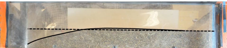
Figure 6.15: Photos from top viewing window of soil box during passive movements test: (a) at beginning of test; and after (b) cycle 1.5; (c) cycle 1.10; (d) cycle 2.5; (e) cycle 2.10; (f) cycle 3.5; and (g) cycle 3.10
