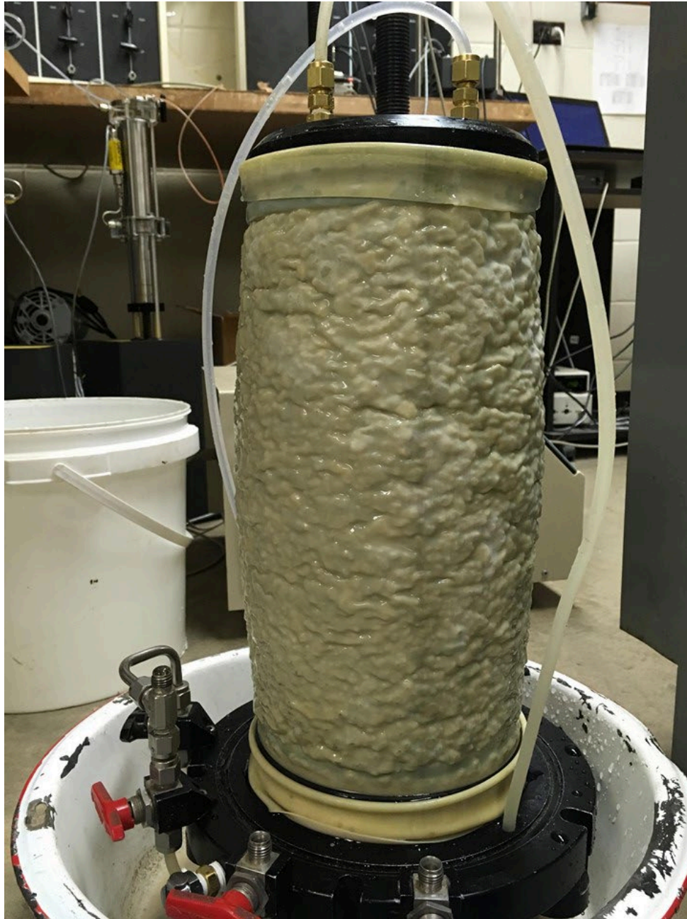
Figure 4.26: Triaxial specimen at failure (9 psi effective confinement)
