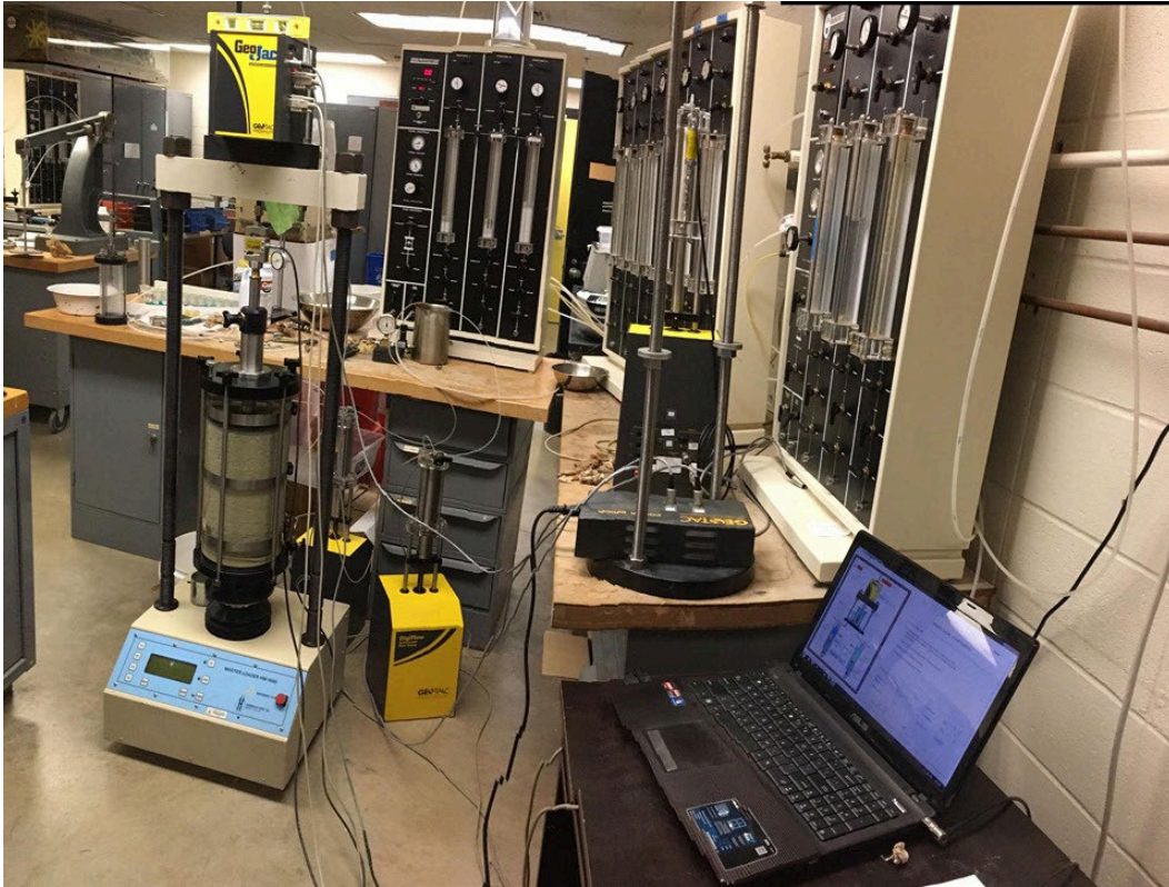
Figure 4.23: Triaxial setup used to measure shear strength of Mack Creek soil
