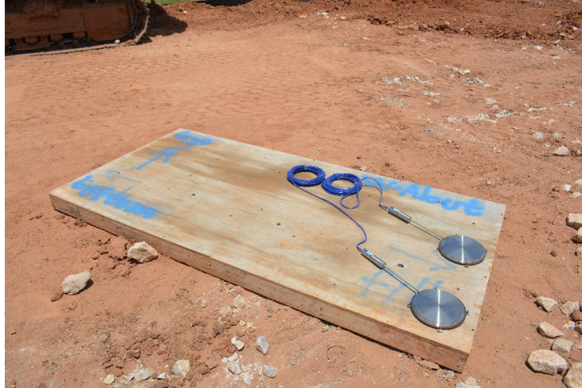
Figure 8.74: Pair of earth pressure cells mounted on back of form intended for west abutment backwall
