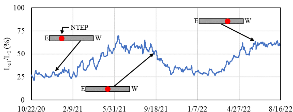
Figure 9.8: Time-history of NTEP distance from east abutment wall, normalized to total length of bridge
