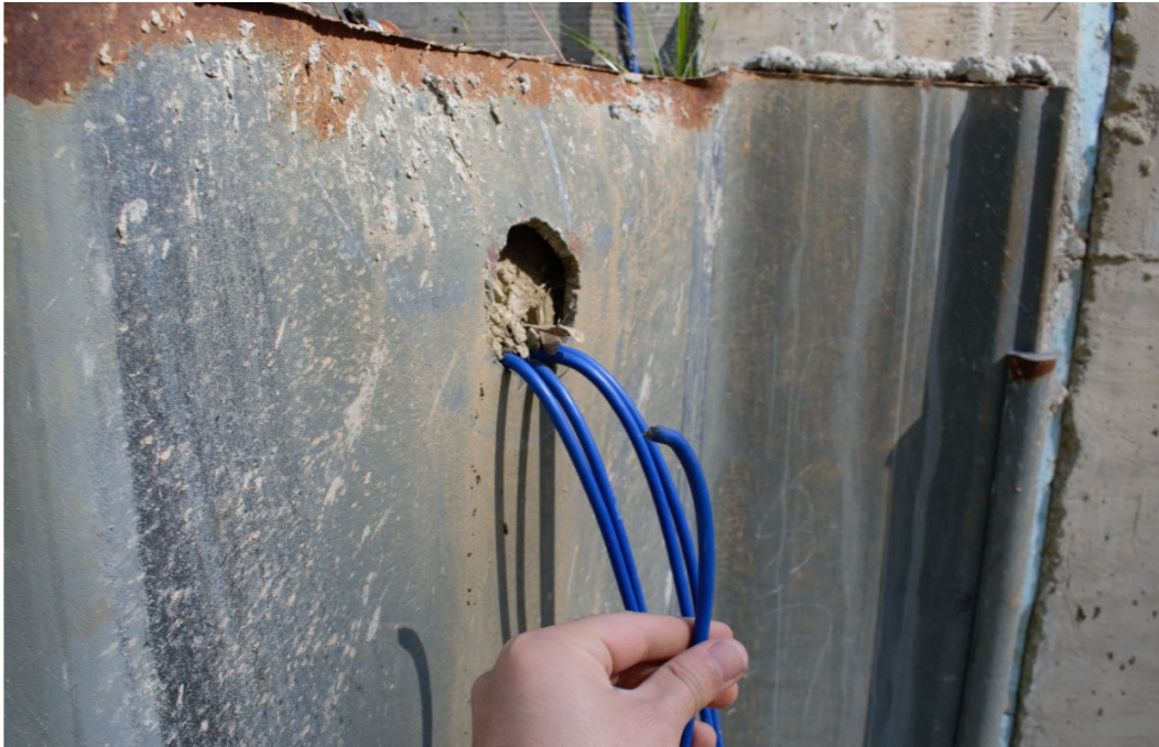
Figure 4.22: Damage to earth pressure cell cables due to unanticipated settlement of concrete
