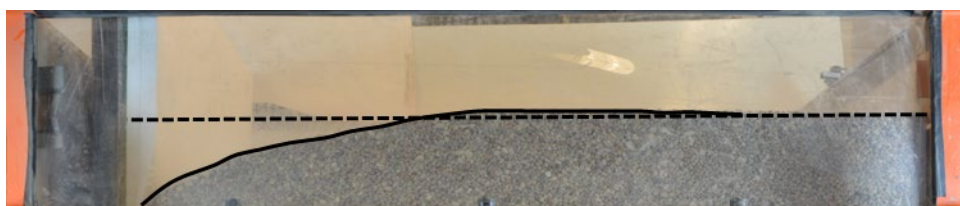
Figure 6.27: Photos from top viewing window of soil box during geofoam inclusion test: (a) at beginning of test; and after (b) cycle 1.5; (c) cycle 1.10; (d) cycle 2.5; (e) cycle 2.10; (f) cycle 3.5; and (g) cycle 3.10
