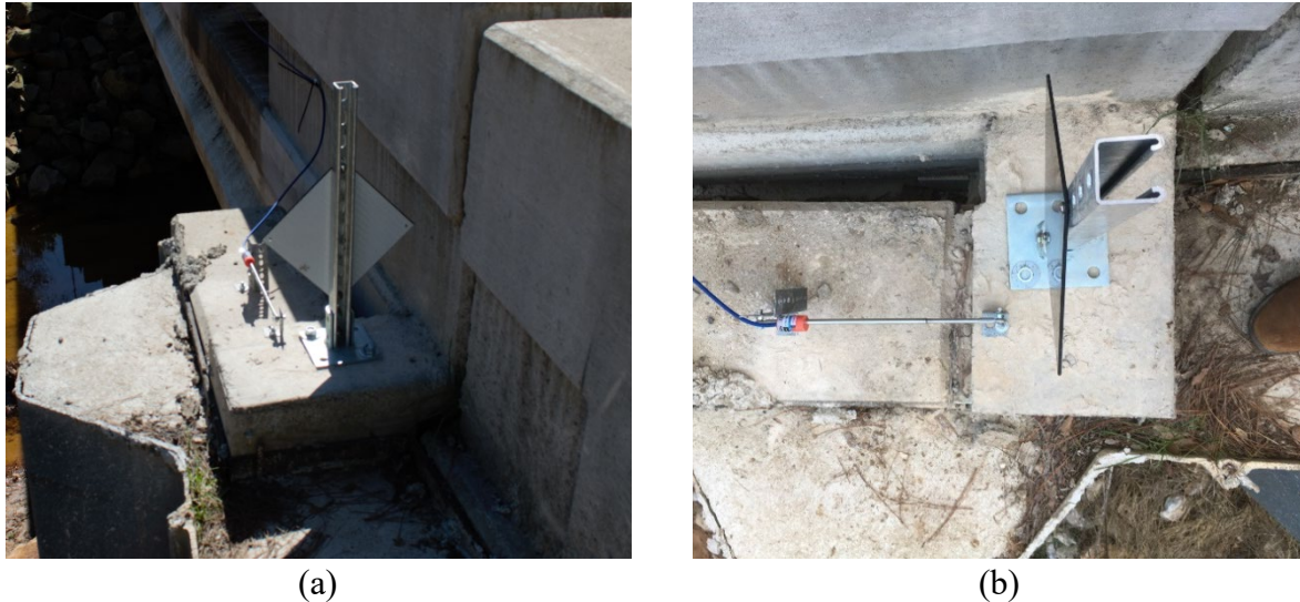
Figure 7.20: Closeup of equipment installed on north abutment, laser target and crackmeter installed between backwall and pile cap: (a) view from behind; and (b) top view
