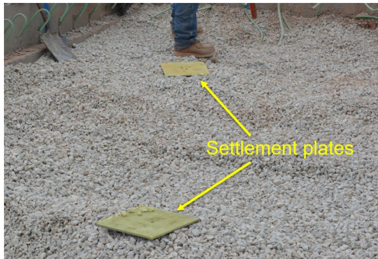
Figure 8.81: Stainless steel plates attached to top flange of settlement sensors
