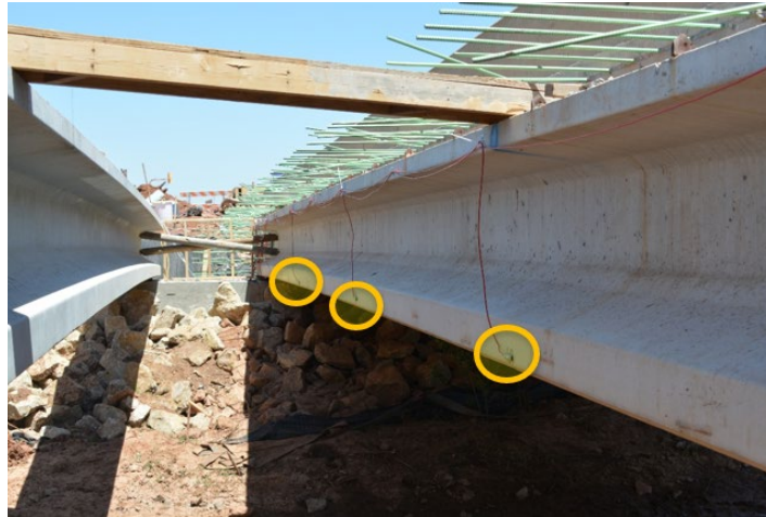
Figure 8.72: Mounted miniature strain gauges on bottom flange of middle girder
