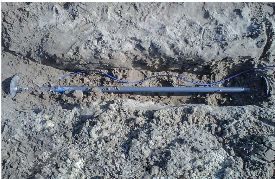
Figure 8.16: Model 4430 deformation meter (geokon.com)
