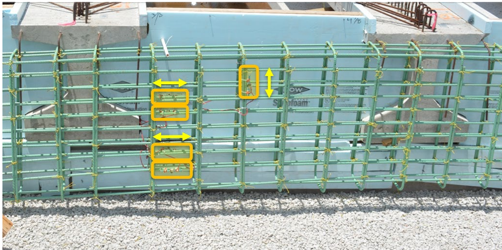
Figure 8.73: Location of three pairs of concrete-embedded strain gauges on east abutment backwall
