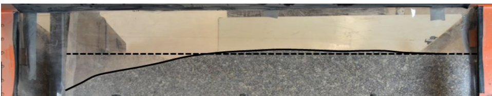
Figure 6.7: Photos from top viewing window of soil box during baseline test: (a) at beginning of test; and after (b) cycle 1.5; (c) cycle 1.10; (d) cycle 2.5; (e) cycle 2.10; (f) cycle 3.5; and (g) cycle 3.10
