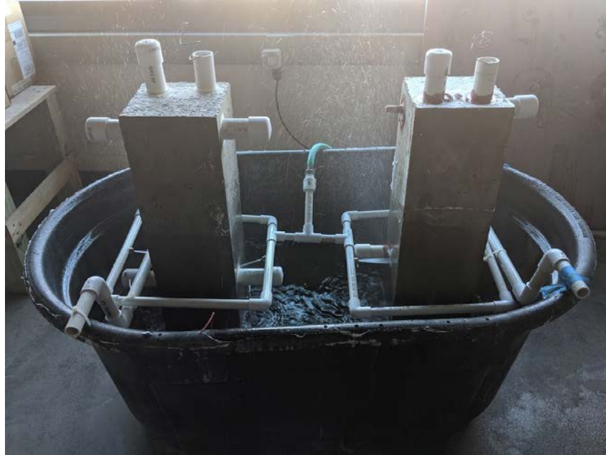
(a) Marine Exposure Tank
