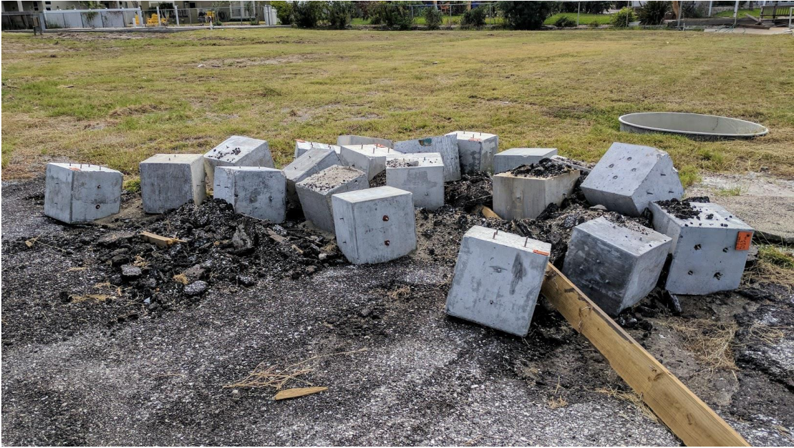
Figure 2.12 Exposure blocks bulldozed as part of Hurricane Harvey cleanup process in Port Aransas
