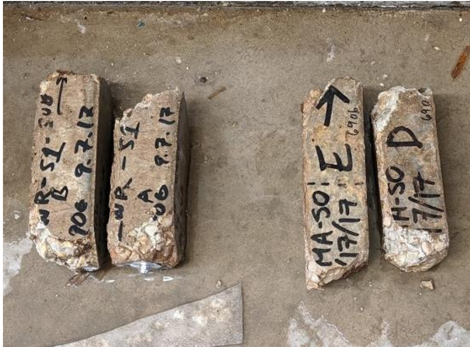
Figure 4.27 Failed samples submerged in sodium sulfate trough
