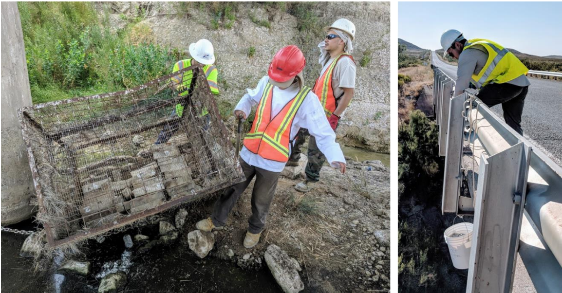
Figure 4.6 Site 2 samples are stored inside a lobster cage below bridge (left) and samples are lifted to road level via bucket (right)
