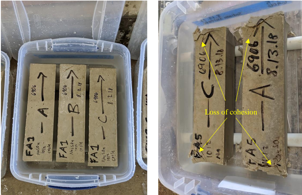
Figure 4.24 Sodium sulfate solution samples exhibiting minimal (left) and significant (right) loss of cohesion
