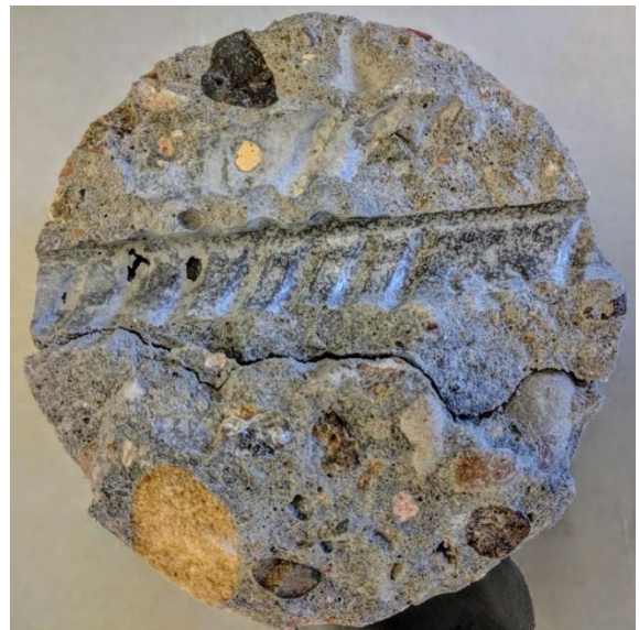
Figure 7.14 Rebar placed at a depth of 3.5 in. from the top of slab (left), and rebar imprint at the bottom of core (right)
