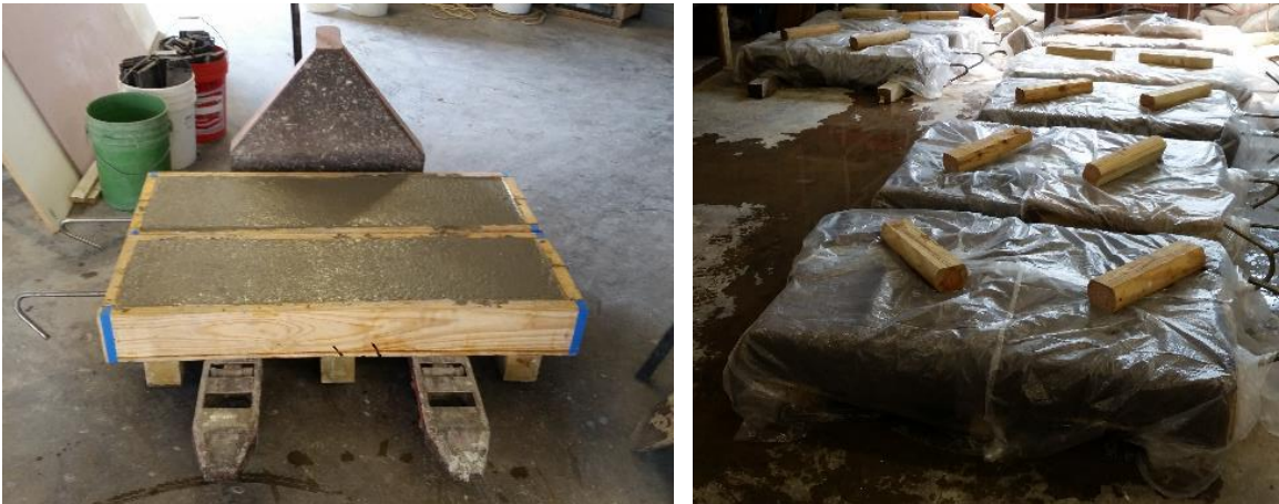
Figure 3.7 Marine exposure block casting (left) and curing (right)
