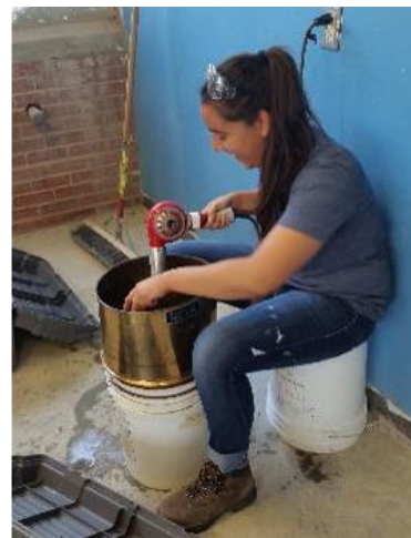
Figure 2.2 LWFA ponding (left) and drying LWFA with cool air (right)
