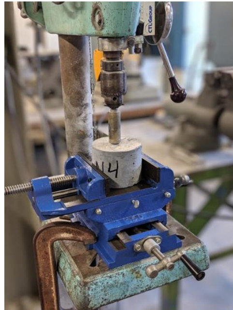
Figure 3.11 Sample schematic per ASTM C1556 (left), and test specimen being profiled (right)
