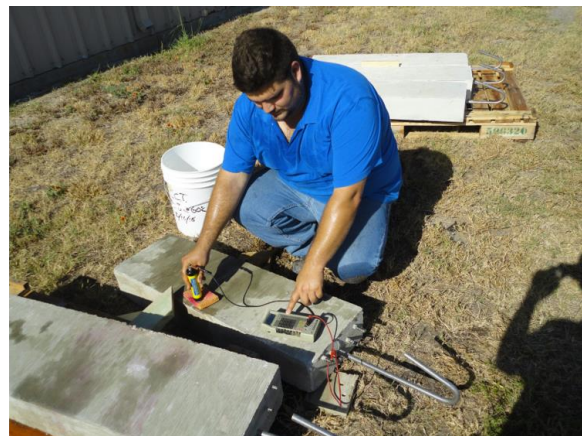
Figure 3.13 Half-cell potential measurement diagram ASTM C876 (left), Measurement on field specimen (right)
