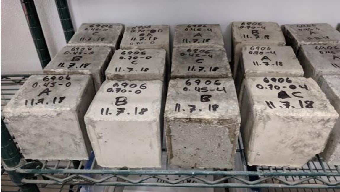
Figure 4.20 Concrete cube samples for NCHRP 244 Series II testing in drying condition
