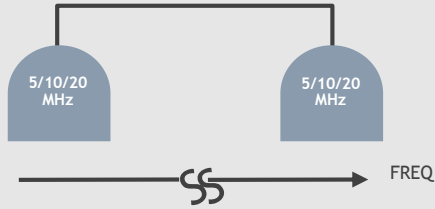
CARRIER AGGREGATION FOR COMBINING MULTIPLE LTE CARRIERS
