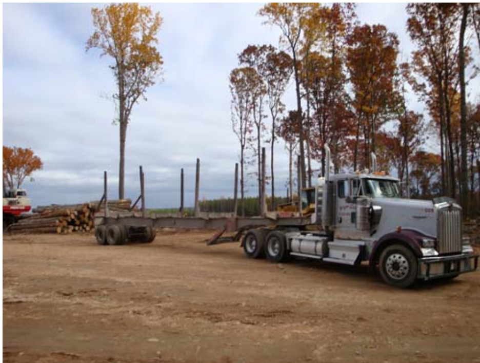
Figure 5.85: Class 8 (GVWR) or Class 9 (FHWA Vehicle Classification) Five-axle Truck with a Four-bolster Trailer
