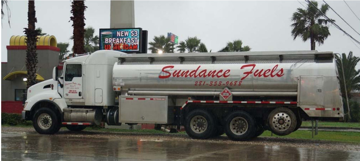
Figure 5.100: 4,500-gallon Single-unit Tanker Truck
