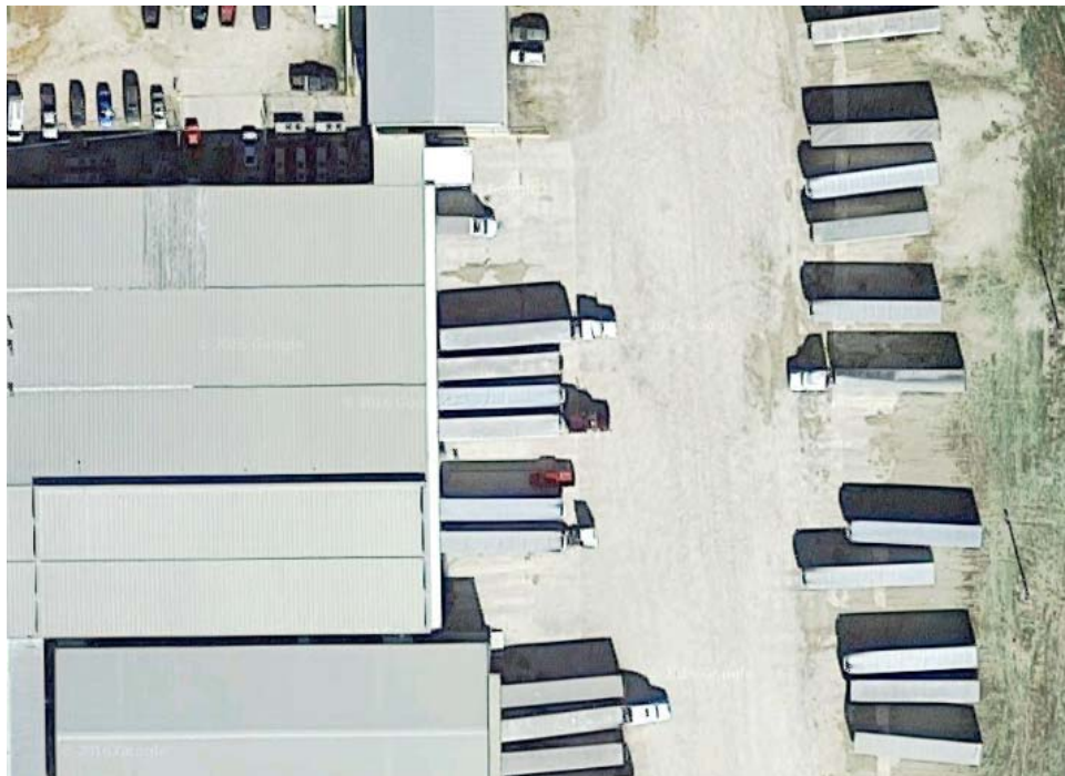
Figure 5.72: Satellite View of a Part of the Wharton County Foods LLC Processing Facility; All Freight Vehicles Visible Are Class 9 Single Trailer Five-axle Trucks
