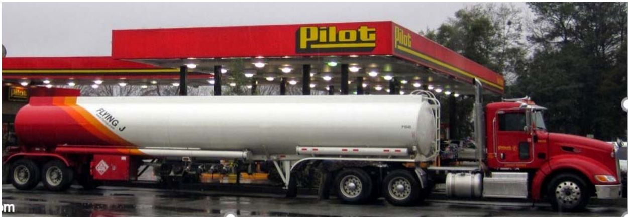
Figure 5.99: 9,000-gallon Tractor-trailer Tanker Truck
