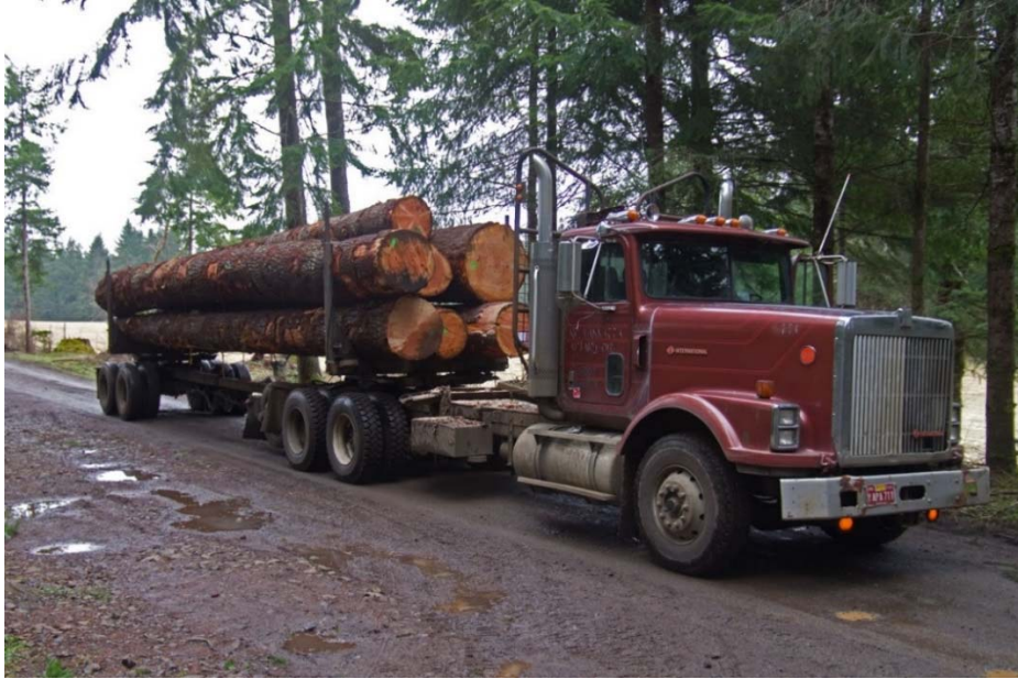
Figure 5.84: Class 8 (GVWR) or Class 9 (FHWA Vehicle Classification) Five-axle Truck with a Pole Trailer
