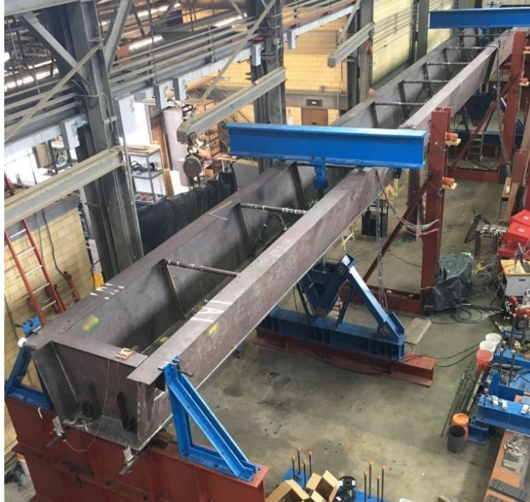
Figure 3-3 –Steel Tub Girder - Test Setup
