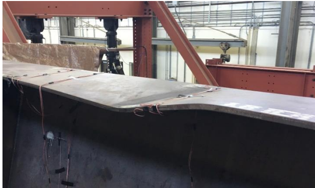
Figure 3-56 - Local Buckling of West Top Flange of Tub #2 at Midspan – View 2
