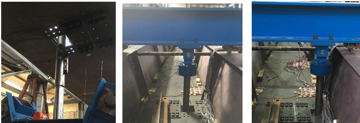
Figure 3-8 - GLS ram location: Left) Concentric, Center) Eccentric, e=8'' , Right) Eccentric, e=16''
