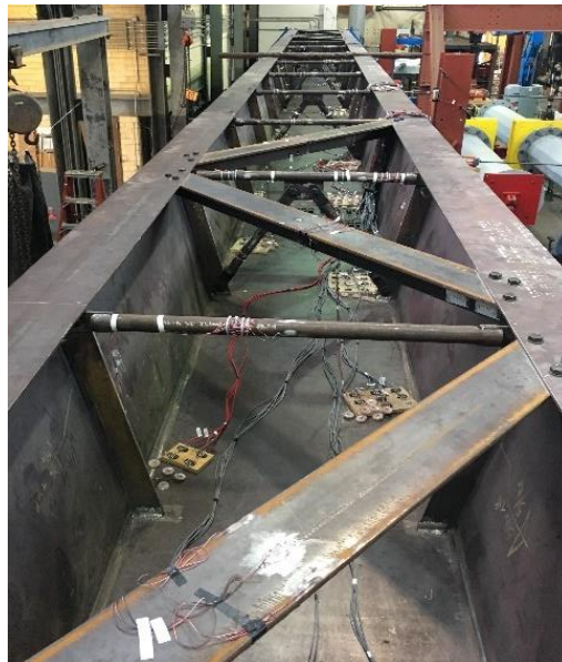
Figure 3-18 - Top Lateral Bracing System
