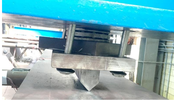
Figure 3-11 - Knife Edge and Thrust Bearing Assembly
