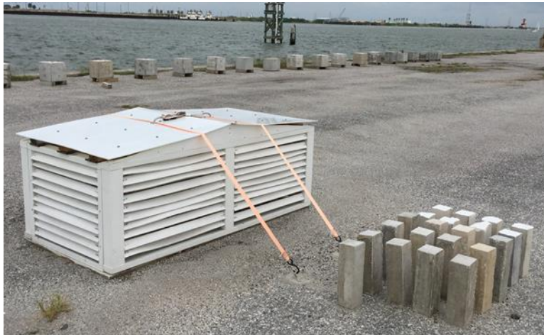
Figure 8.5: Carbonation Exposure Site on the Gulf Coast
