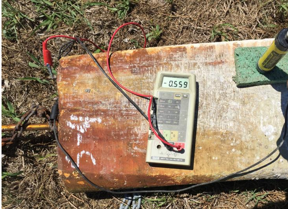
Figure 7.5: Half-Cell Potential Measurement Procedure
