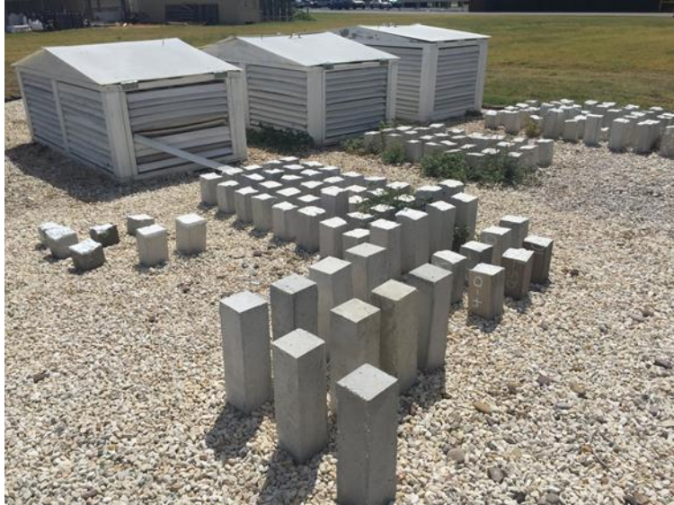
Figure 8.4: Carbonation Exposure Site in Austin, TX
