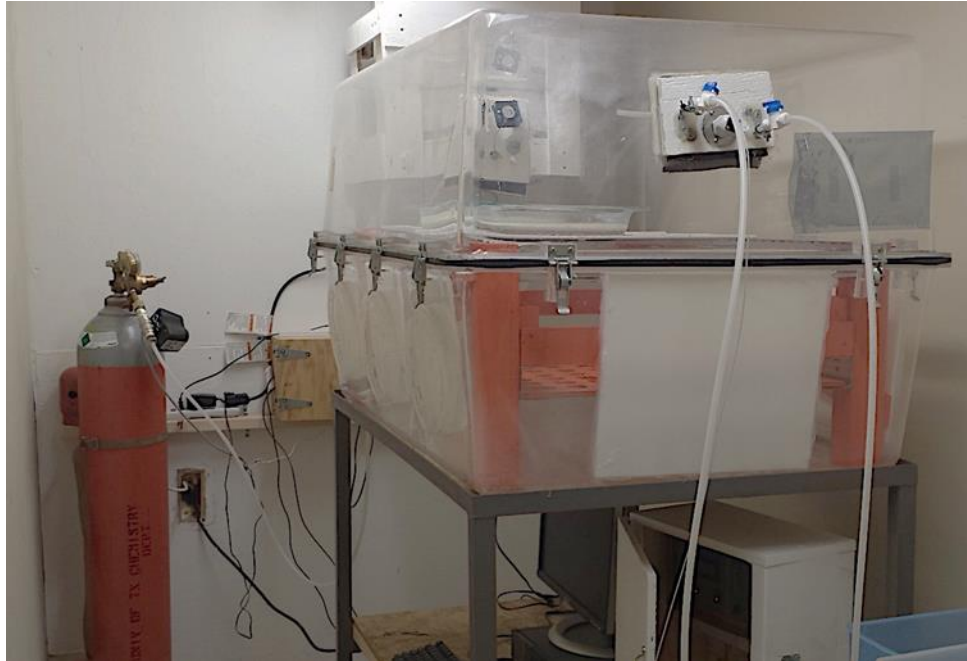
Figure 8.32: Picture of Accelerated Carbonation Chamber
