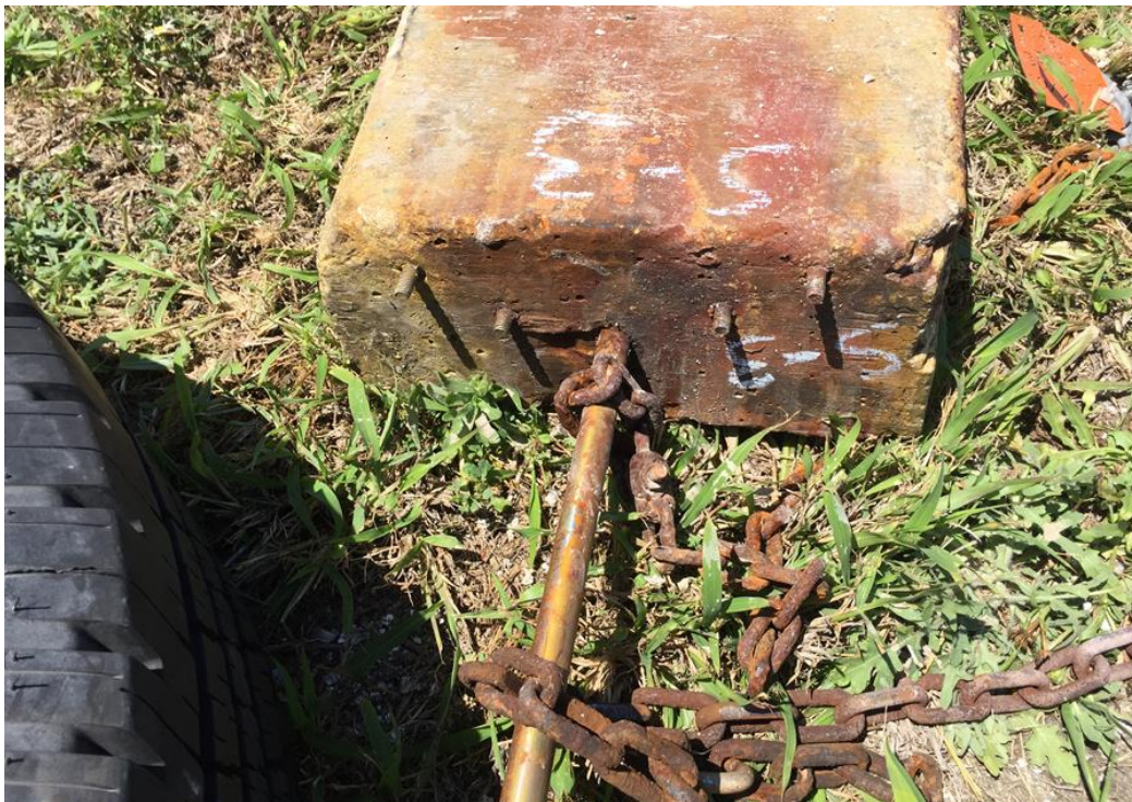
Figure 7.4: Cross-Sectional View of Actual Specimen after Being Pulled Out of Seawater
