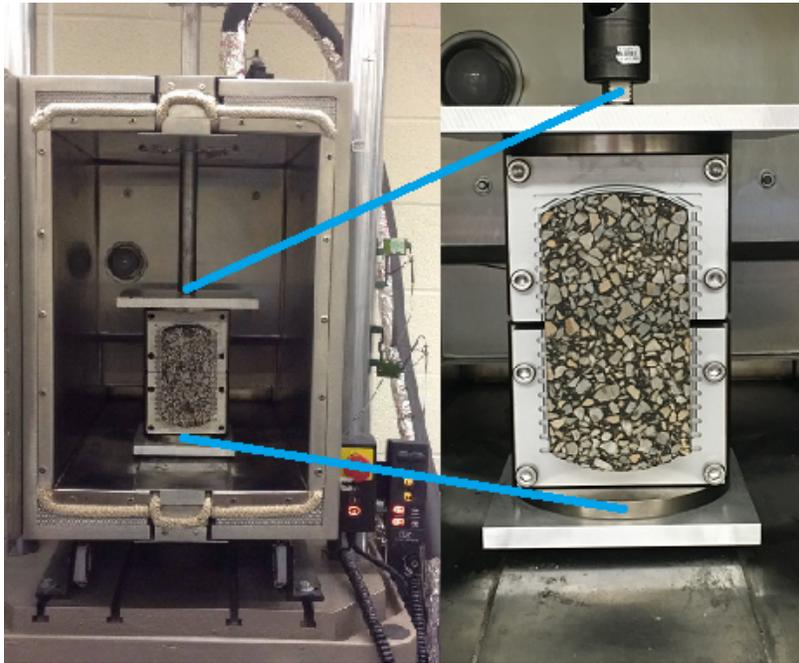
**Figure 4.9. Overlay Specimen Configuration in the Servo-Hydraulic Machine**
