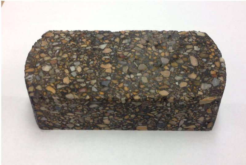
**Figure 4.7. Specimen Used For Overlay Test**
