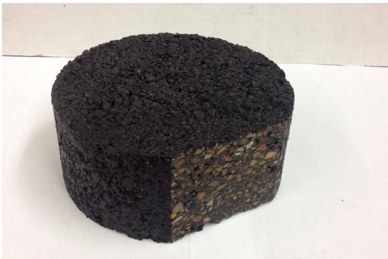
**Figure 4.6. Specimen Used For Hamburg Wheel Tracking Test**
