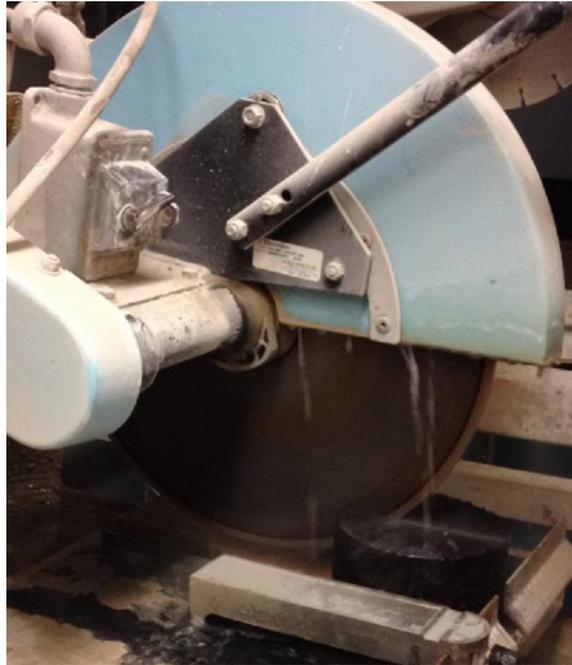
**Figure 4.5. Saw Used For Hamburg Wheel Tracking and Overlay Specimens**
