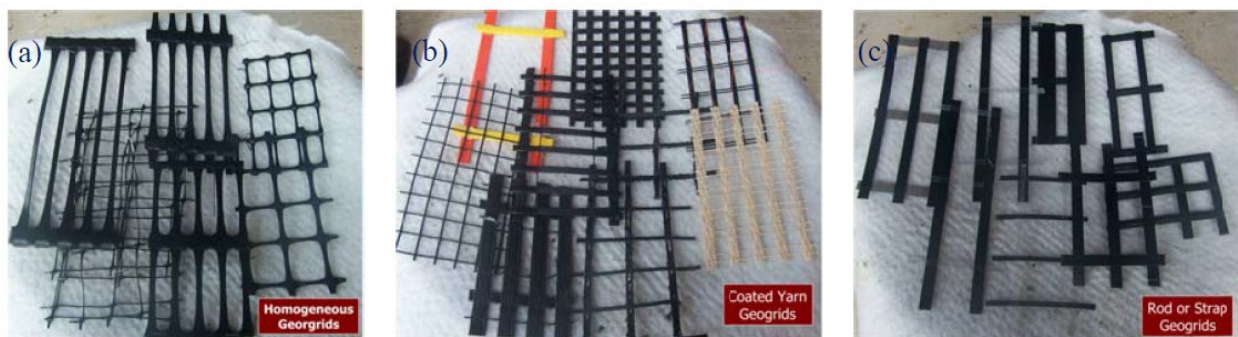
Figure 2.1 Various types of Geogrids: (a) Homogenous; (b) Coated Yarn; (c) Welded
