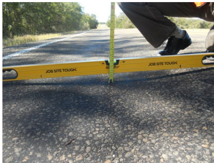
Figure 4.10 Measurement of a significant rutting during condition survey of the FM2 pavement test sections
