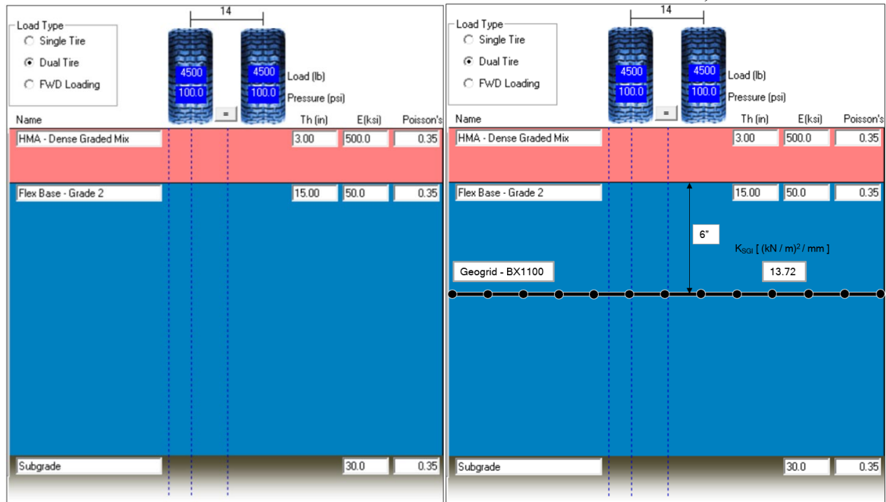
Figure 8.5. Stiffness of Subgrade Variant, E_s = 30.0 psi
