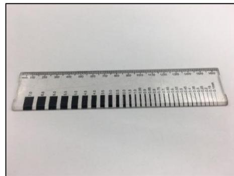
(b) Crack-comparator gauge
