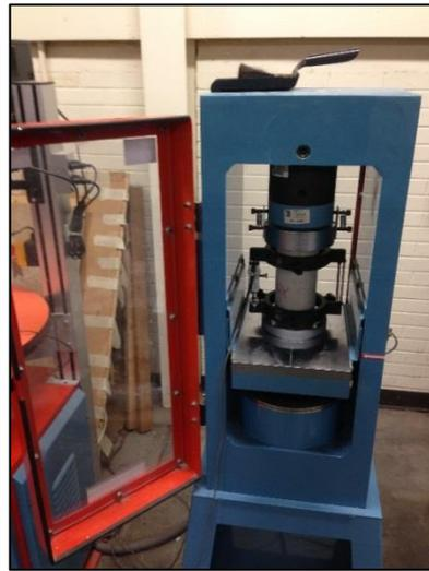
(b) Match-cured cylinder being tested
