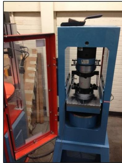
(b) Match-cured cylinder being tested
