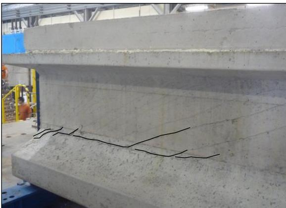
(a) Horizontal shear failure (Hovell et al., 2011)
