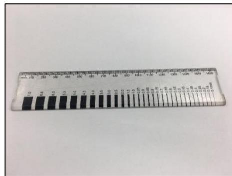
(b) Crack-comparator gauge
