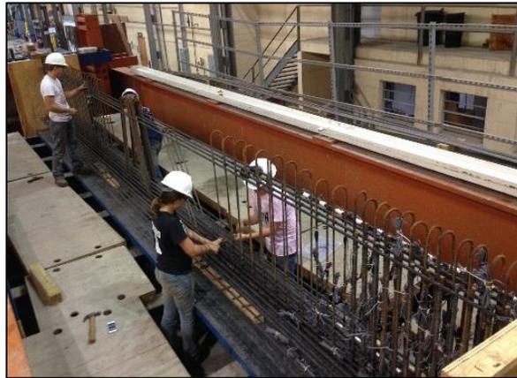
(c) Tying the mild-steel reinforcement
