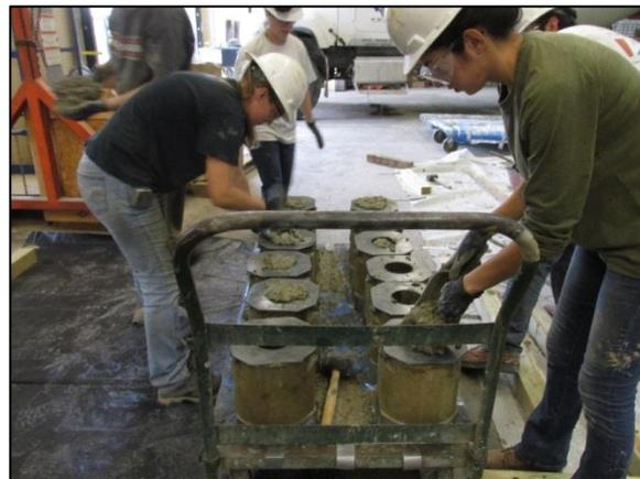
(b) Casting match-curing cylinders
