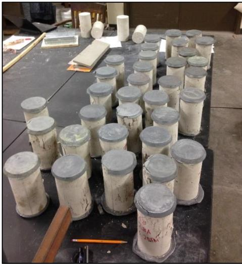
(a) Tested match-cured specimens
