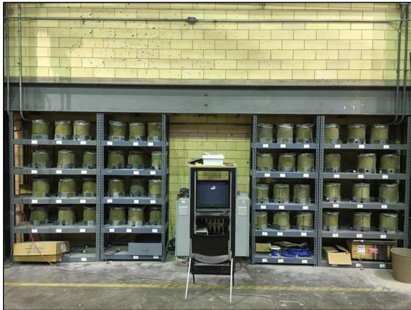
**Figure 5-12- Match-curing system**
