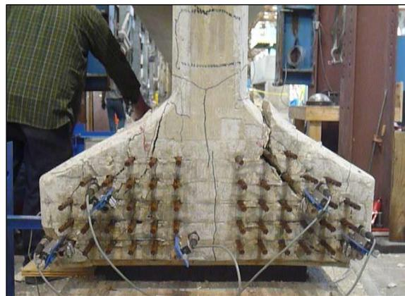
(b) Anchorage-induced shear failure (Garber et al., 2016)
