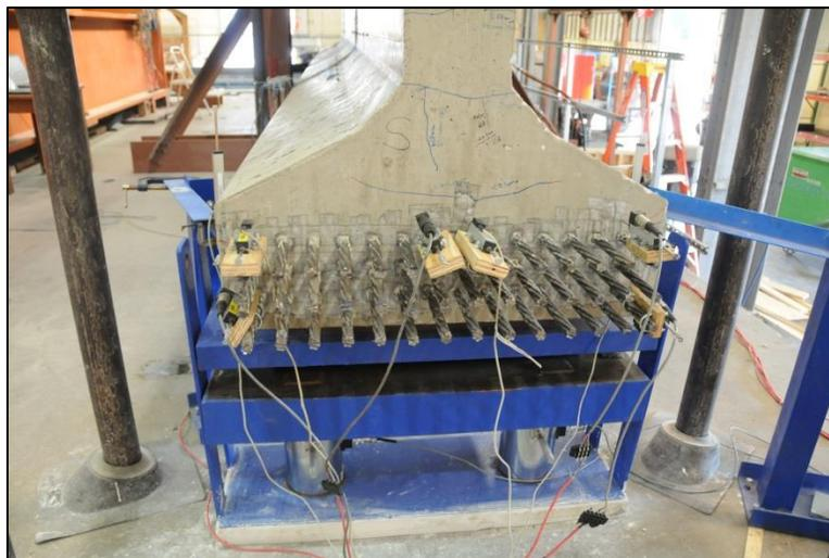
**Figure 5-19- Displacement transducers used for measuring strand slip**
