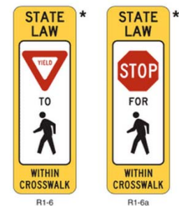
Figure 65: R1-6 and R1-6a Warning Signs (TxDOT, 2012b)
