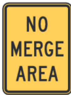
Figure 13: No Merge Area W4-5P Sign (MUTCD, 2012)
