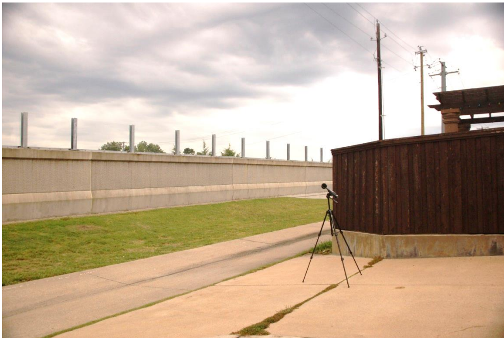
Figure 2.47 Noise measurement at Site #5: 4714 Petersburg Drive behind noise wall and noise wall addition
