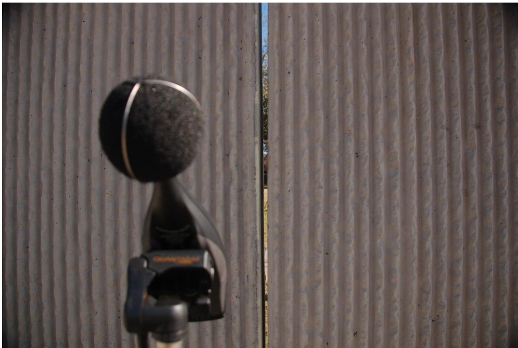
Figure 7.36 Noise test conducted in front of noise wall with an open expansion joint without sealant material in the background
