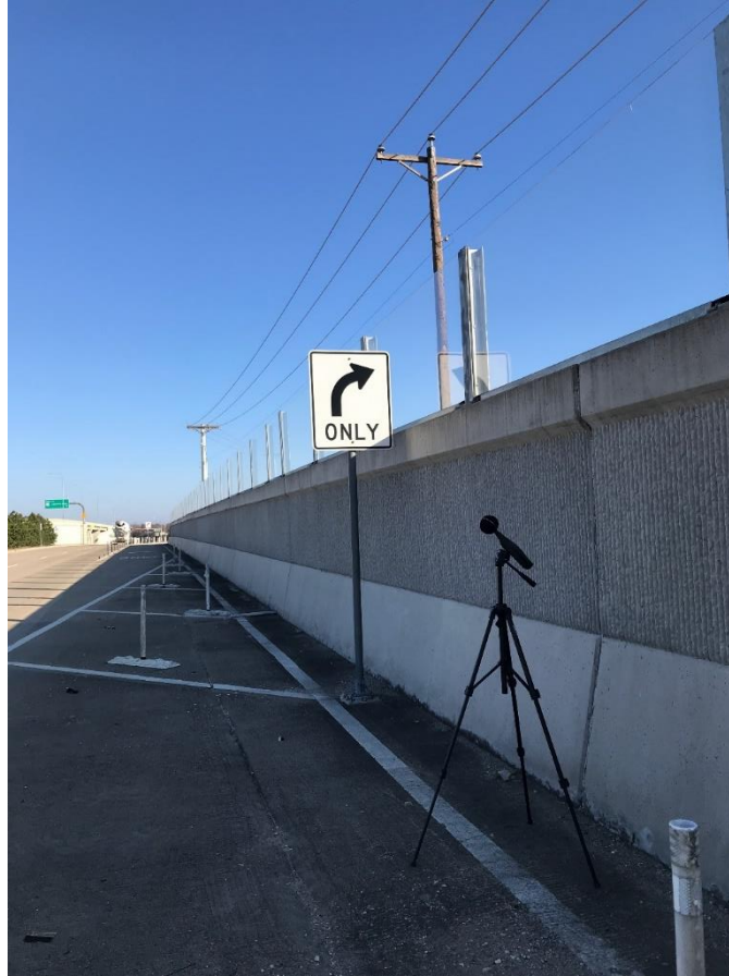
Figure 6.21 Sound meter in front of east noise wall (Photo by Ray Umscheid)
