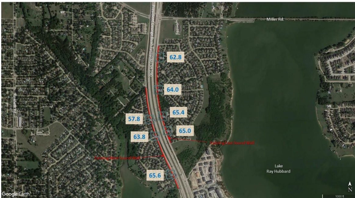
Figure 6.2 Average noise level results by receiver (post-barrier)
