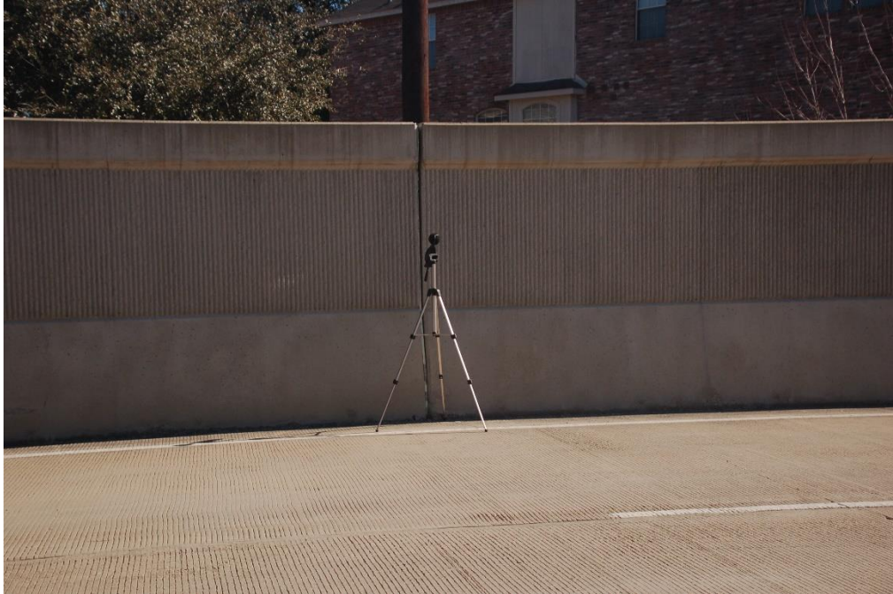
Figure 6.17 Sound meter in front of noise wall
