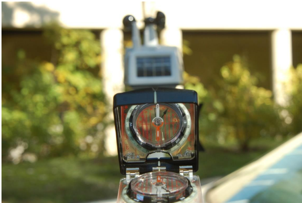
Figure 5.7 Use of the mirror compass for orientation of the weather station: the solar panel of the weather station, in the background, is positioned so that it faces south
