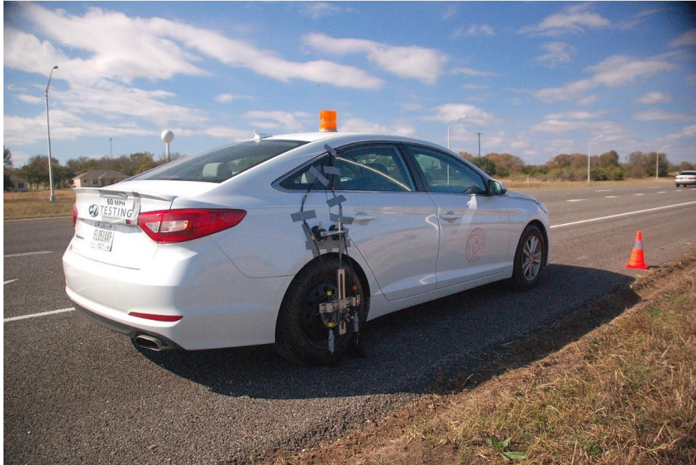
Figure 3.28 Test vehicle and OBSI fixture
