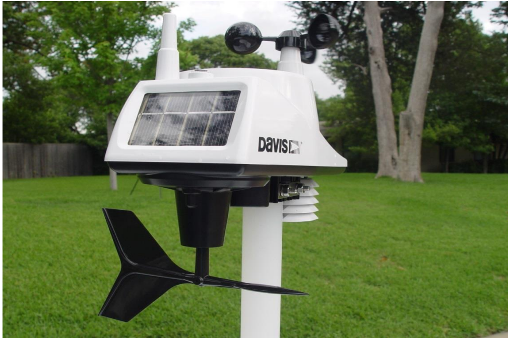
Figure 5.3 Davis Instruments portable weather station, showing the ISS
