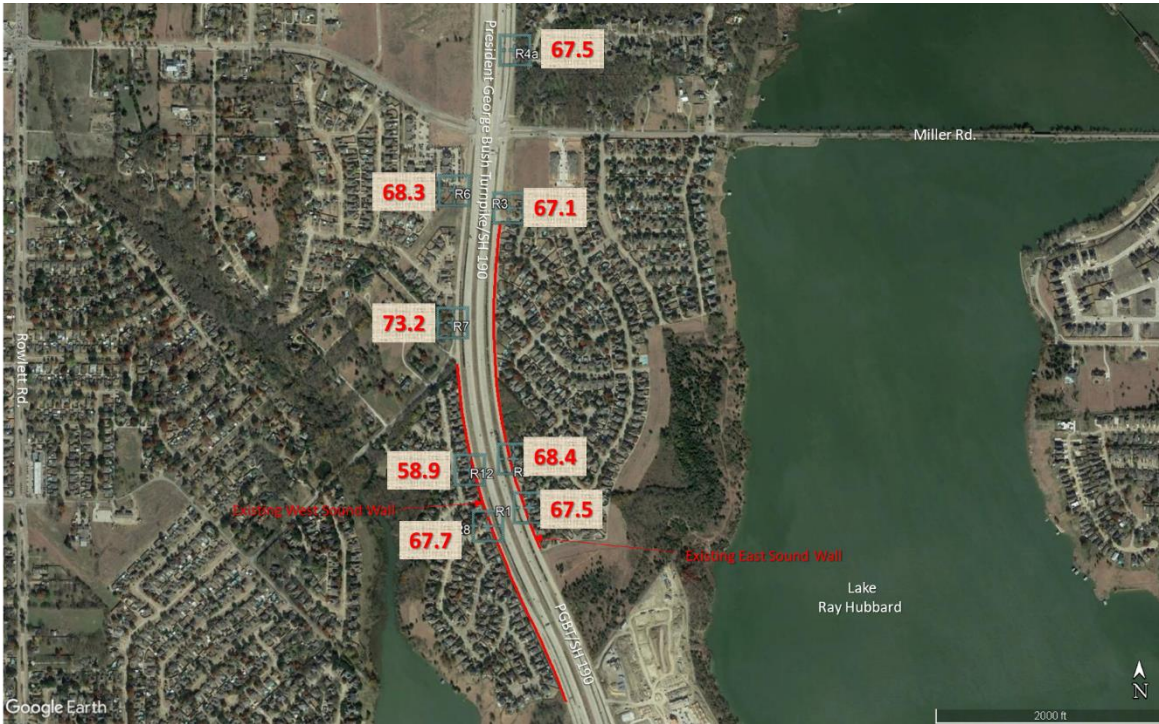
Figure 6.1 Average noise level results by receiver (pre-barrier)
