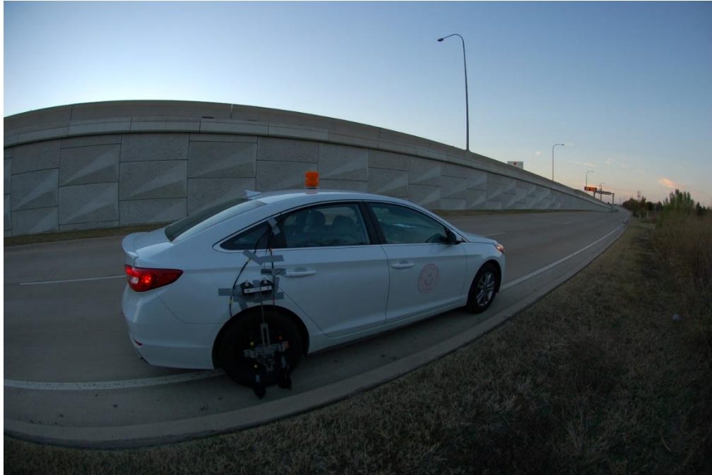
Figure 3.29 OBSI Test vehicle on SH 190 frontage road
