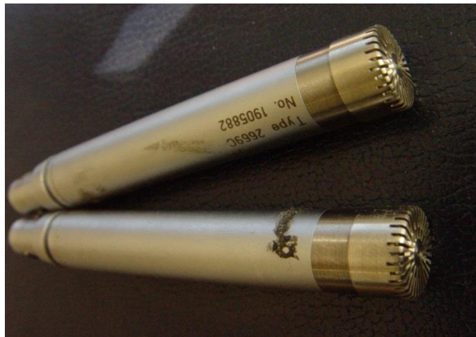
Figure 3.27 Half-inch Sound Intensity Microphone Pair
