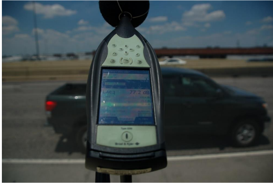
Figure 9.64 Test conducted behind noise wall panels of Segment 2: 77.2 dBA (May 29, 2018)
