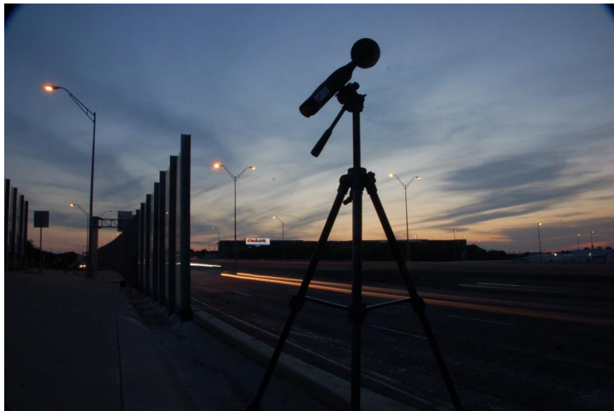
Figure 9.67 IL test with simultaneous meters; meter next to traffic (June 13, 2019)
