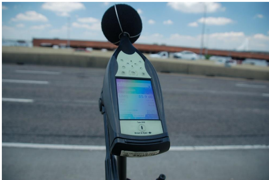
Figure 9.61 Test conducted next to the I-30 main lanes traffic: 85.9 dBA next to main-lane traffic (May 29, 2018)
