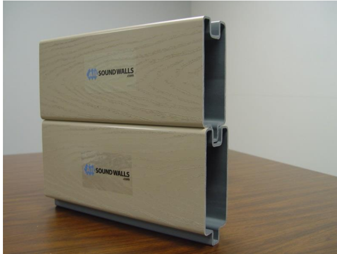
Figure 2.6 ALL Sound Walls product samples delivered to CTR: Tuf-Barrier product (reflective) made of PVC
