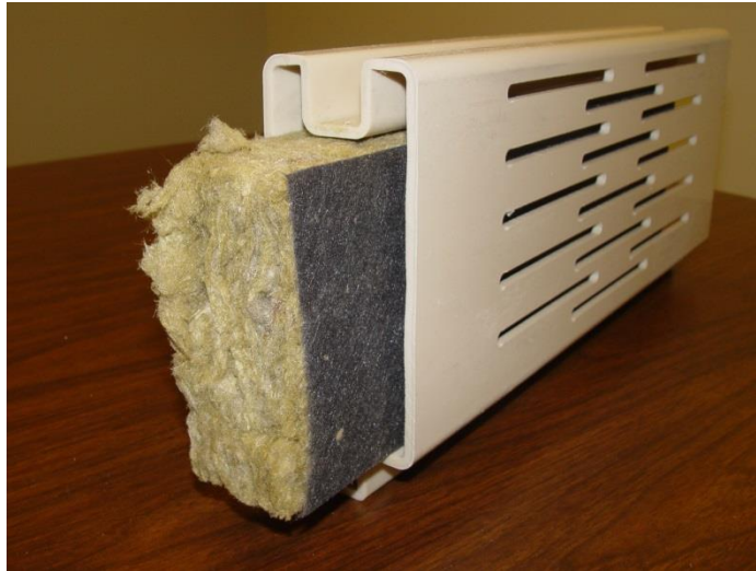
Figure 2.4 AIL Sound Walls product sample delivered to CTR showing the absorptive material (acoustical mineral wool) encased in the PVC stackable panel
