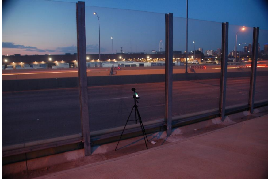
Figure 9.68 IL test with simultaneous meters; meter behind noise wall (June 13, 2019)
