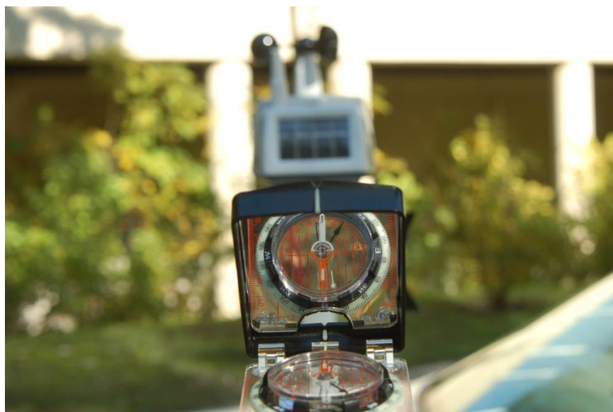
Figure 6.7 Use of the mirror compass for orientation of the weather station: the solar panel of the weather station, in the background, is positioned so that it faces south
