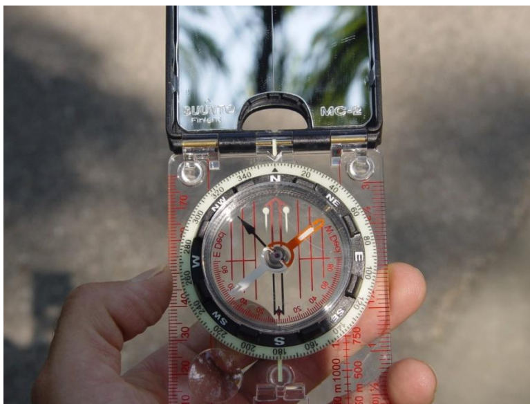
Figure 6.6 Mirror compass used for orientation of the weather station
