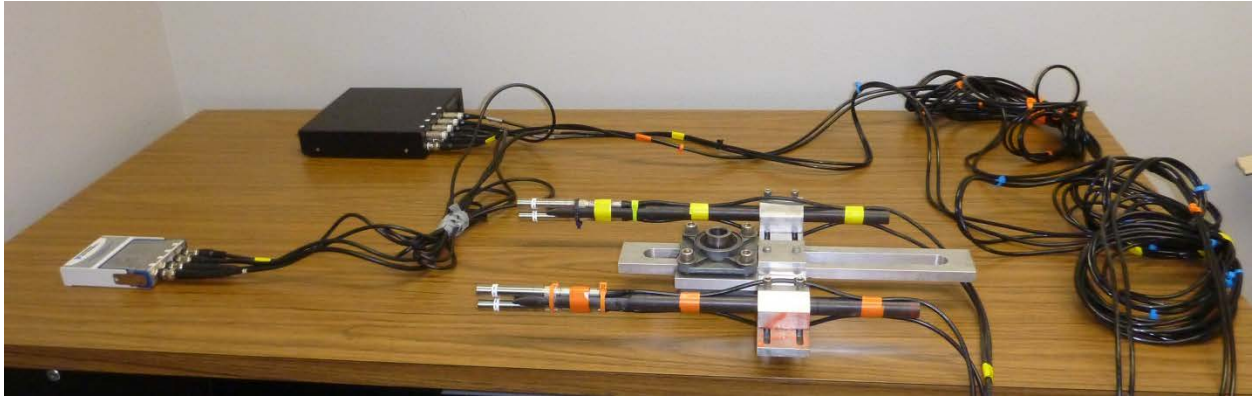
Figure 3.25: OBSI fixture and data acquisition equipment
