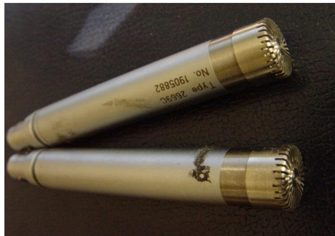
Figure 3.27: Half-inch sound intensity microphone pair
