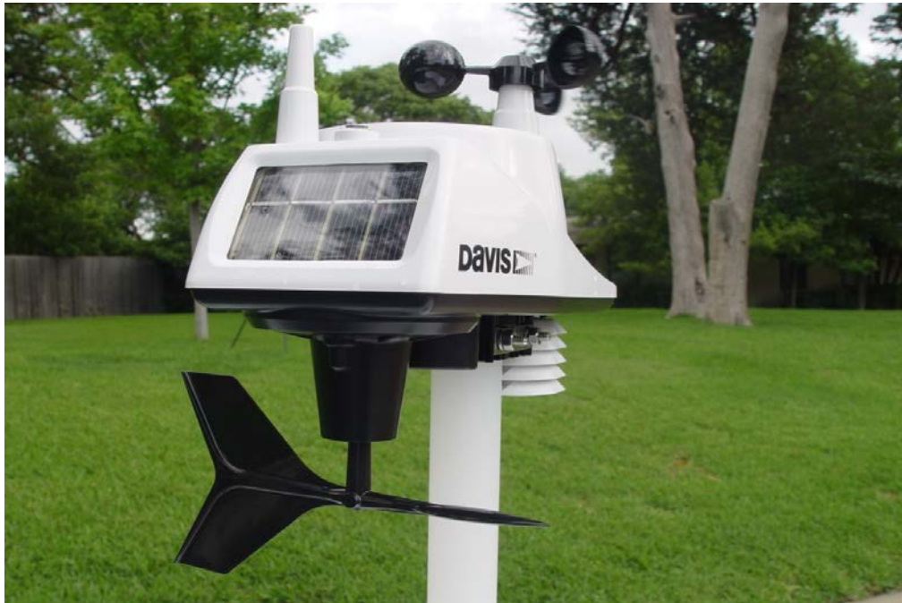
Figure 4.3: Davis Instruments portable weather station, showing the ISS
