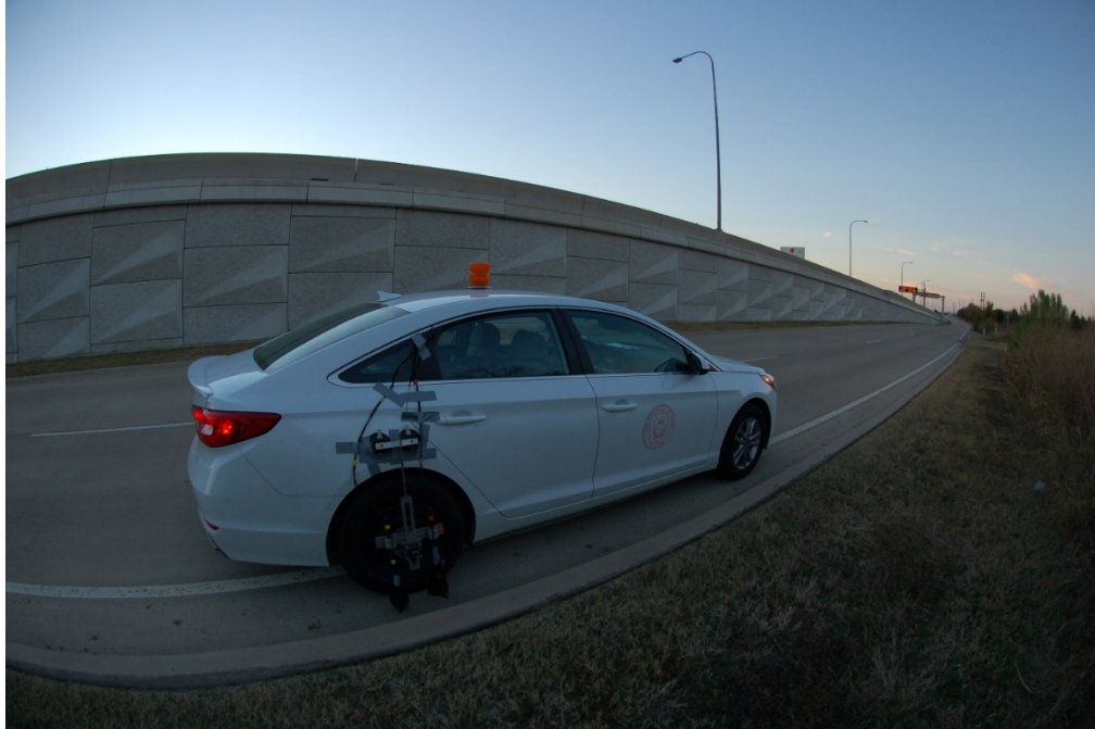
Figure 3.29: OBSI Test vehicle on SH 190 frontage road
