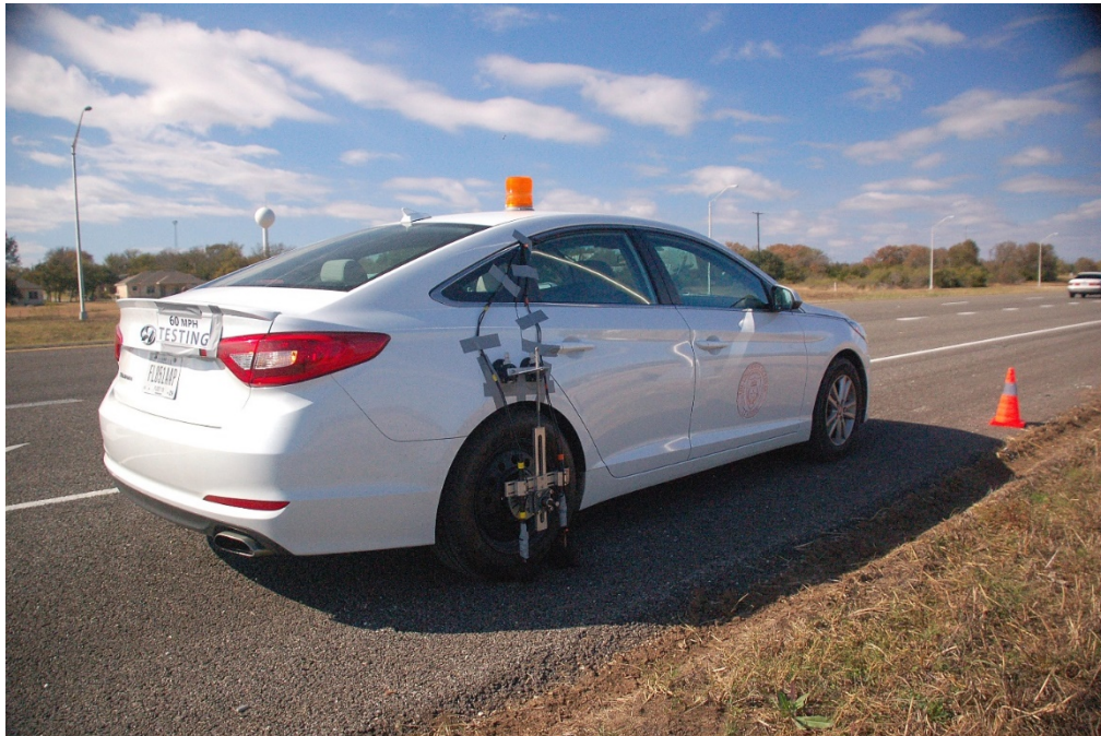
Figure 3.28: Test vehicle and OBSI fixture
