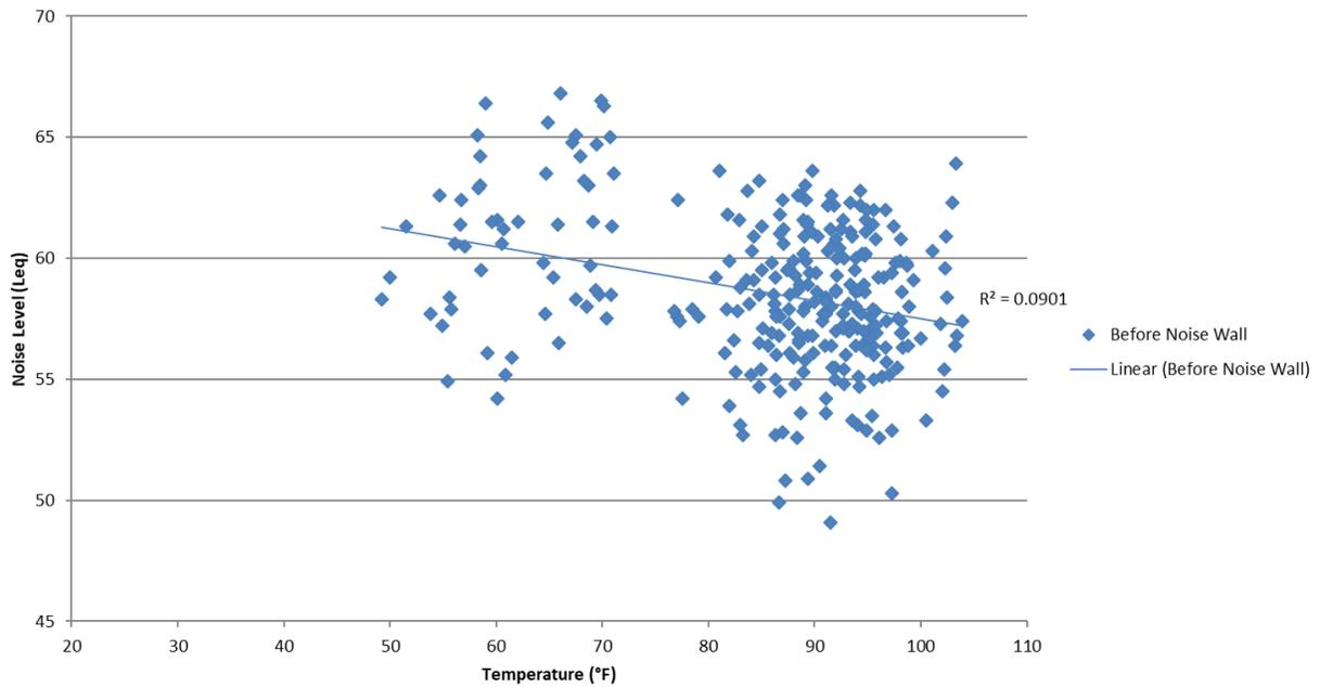
Figure 7.11: Noise level and temperature for Site 2
