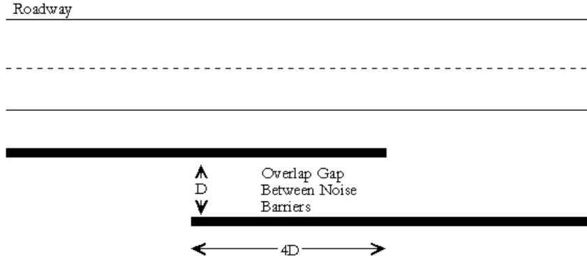
Figure 5.21: Plan view representation of overlapping barriers (FHWA-EP-00-005)
