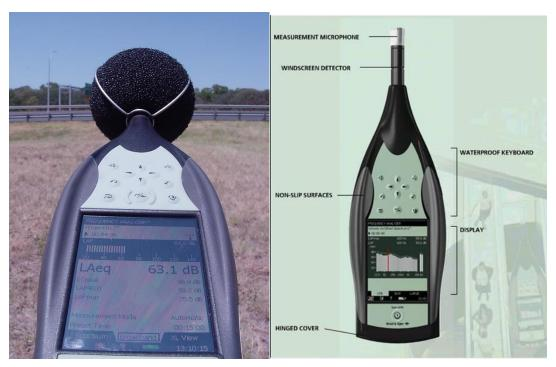
Figure 6.1: Sound pressure level meter
