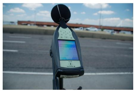
Figure 9.50: Test conducted next to the IH 30 main lanes traffic: 85.9 dBA next to main-lane traffic (May 29, 2018)
