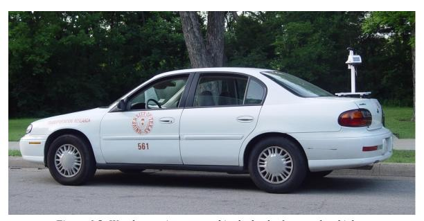
Figure 6.5: Weather station mounted in the back of research vehicle
