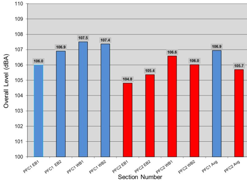
Figure 3.27: Recent OBSI results confirming degradation of acoustic benefits of both PFCs
