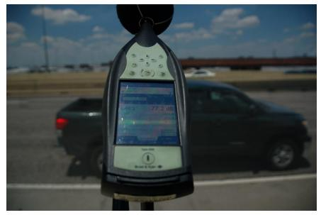
Figure 9.53: Test conducted behind noise wall panels of Segment 2: 77.2 dBA (May 29, 2018)
