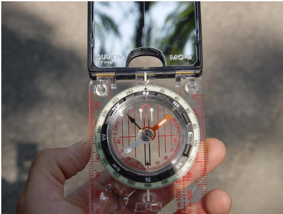
*Figure 6.6: Mirror compass utilized for orientation of the weather station*
