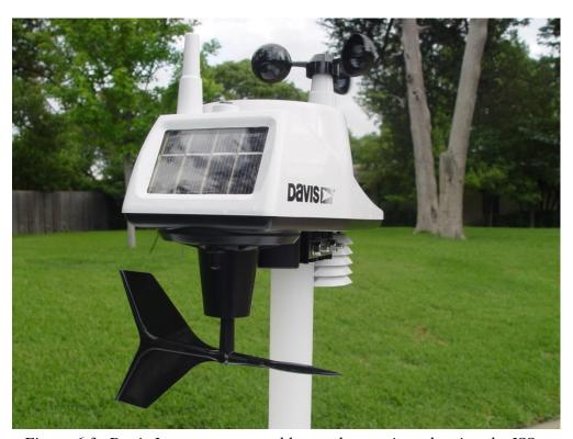
Figure 6.3: Davis Instruments portable weather station, showing the ISS
