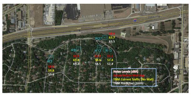
Figure 7.4: Site 2 average noise measurements, before noise wall installation, compared with TNM predictions
