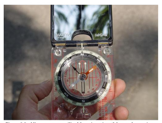
Figure 6.6: Mirror compass utilized for orientation of the weather station
