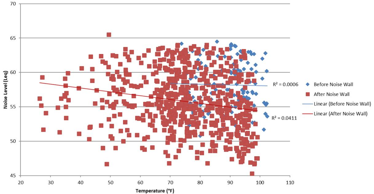
Figure 7.10: Noise level and temperature for Site 1
