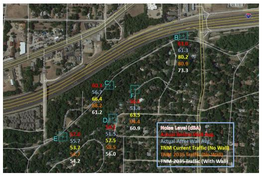
Figure 7.2: Site 1 average noise measurements, before and after noise wall installation, compared with TNM predictions
