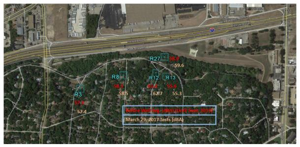
Figure 9.8: Site 2 noise measurements prior to Site 1 wall installation compared to March 2017 tests
