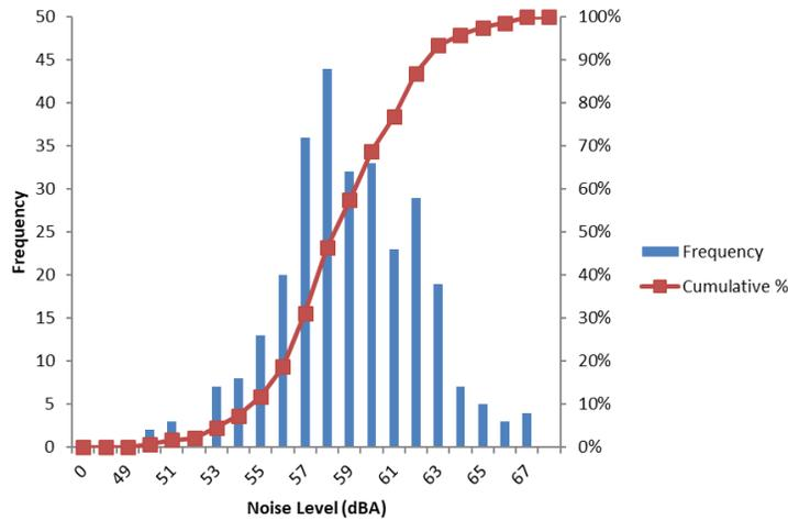
Figure 7.20: Site 2 frequency distribution for pre-barrier tests
