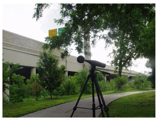
Figure 6.19: Noise measurement at Coombs Creek Trail Park (Location B) prior to noise barrier installation
