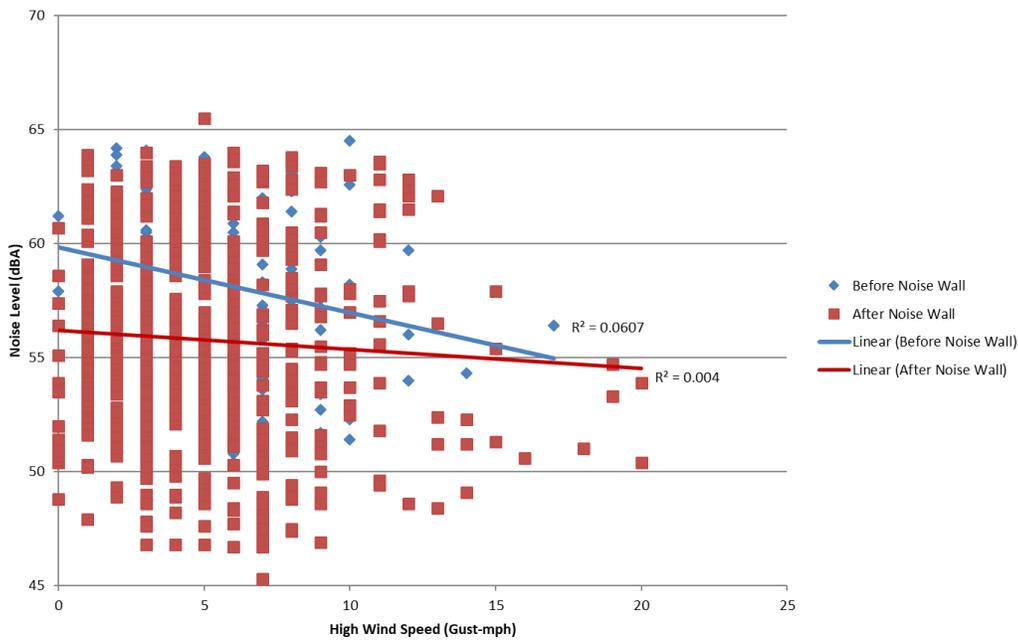
Figure 7.14: Noise level and high wind speed
