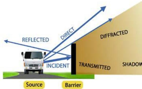
Figure 2.1: Acoustic energy and noise barrier (Bowlby 2012)
