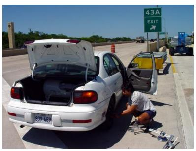
Figure 3.22: Preparing to conduct OBSI tests on IH 30 CRCP (May 2006)
