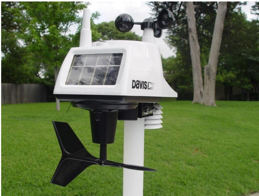
*Figure 6.3: Davis Instruments portable weather station, showing the ISS*
