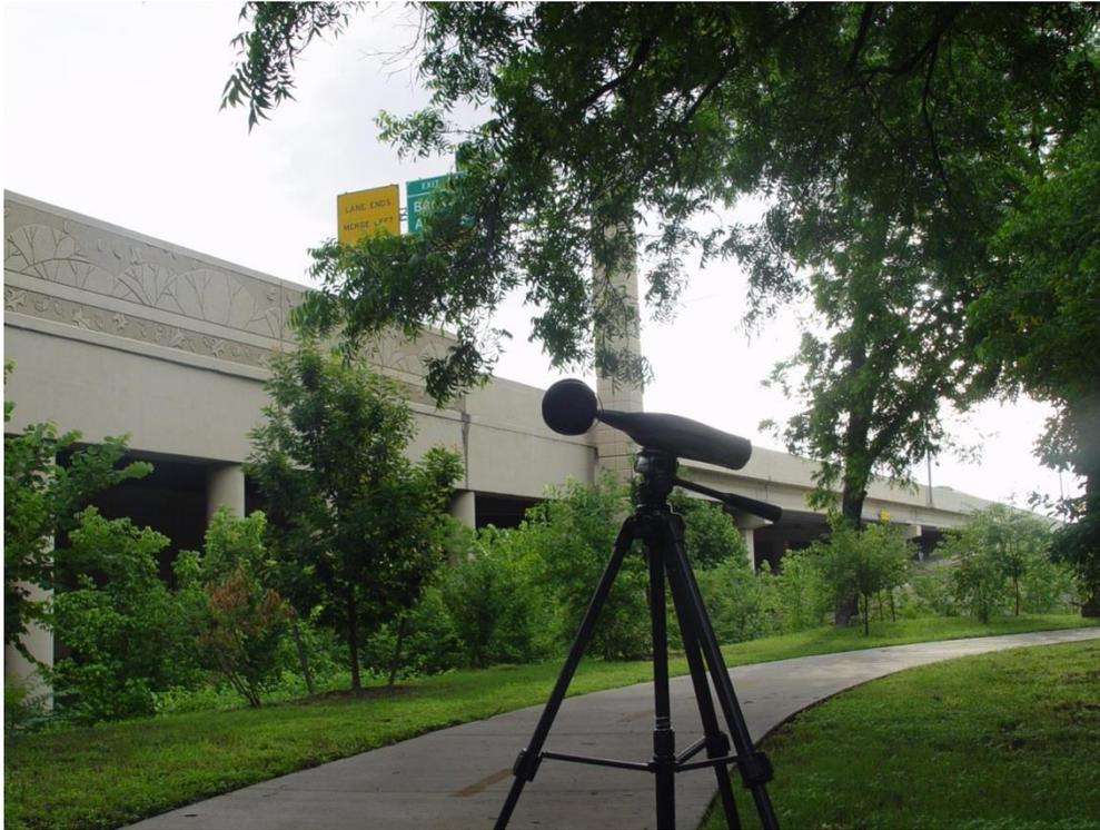
*Figure 6.19: Noise measurement at Coombs Creek Trail Park (Location B) prior to noise barrier installation*
