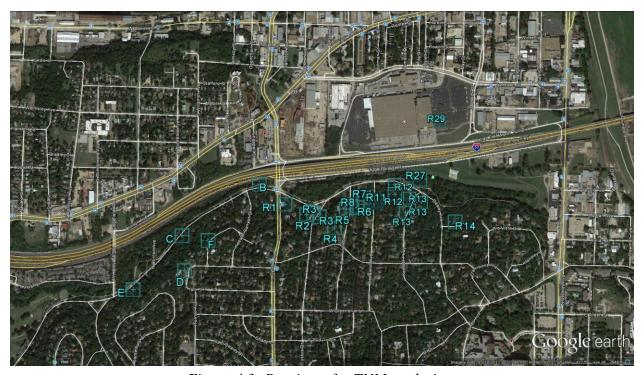
Figure 4.3: Receivers for TNM analysis
