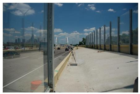
Figure 9.49: Test conducted next to the IH 30 main lanes traffic; Segment 2 on the left, Segment 3 on the right (May 29, 2018)
