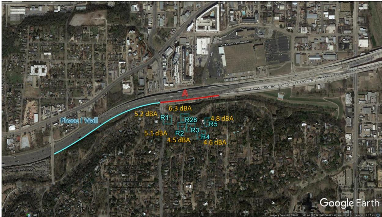
*Figure 5.12: Highest noise level results for Segment A wall with total height of 18 ft.*
