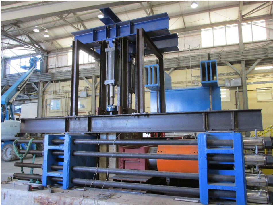
Figure 4.19: Combined axial and shear test setup at FSEL
