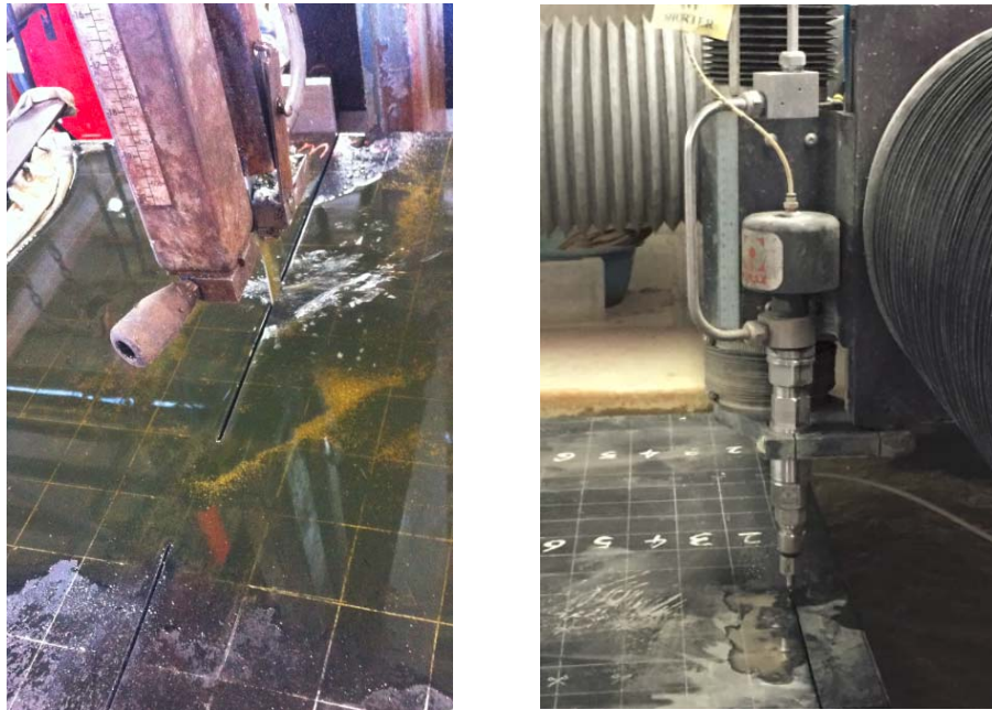
Figure 4.4: Bearing cutting process
