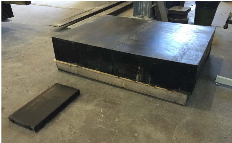
Figure 1.1: A typical elastomeric bearing and one used for higher demand application
