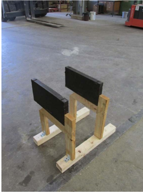
Figure 4.22: Bearings on supports before being placed in the shear test setup
