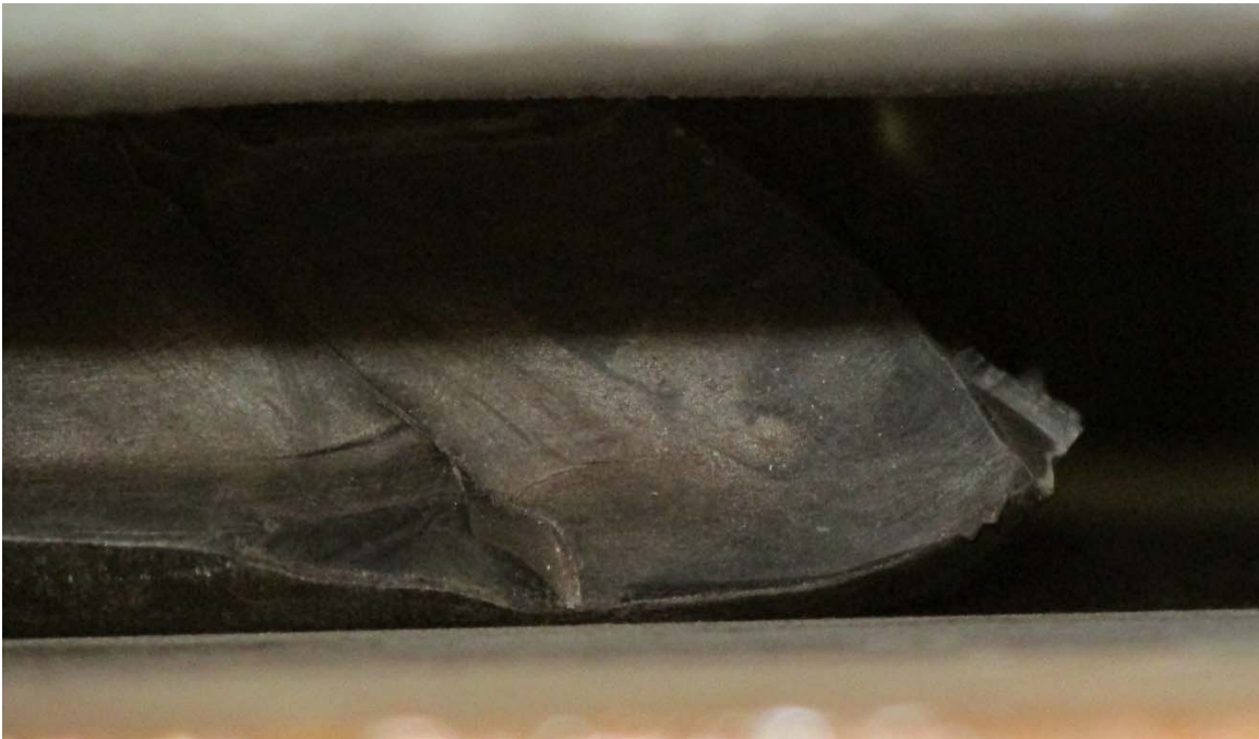
Figure 5.23: Rollover effect on bearing S
