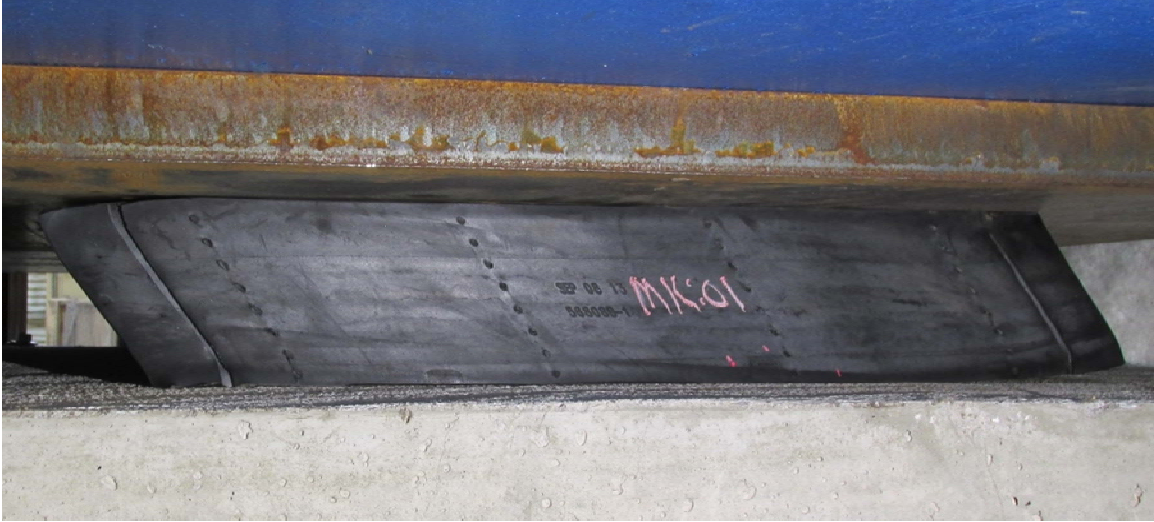
Figure 5.24: Bearing L under 2.0 ksi axial load and 100% shear strain
