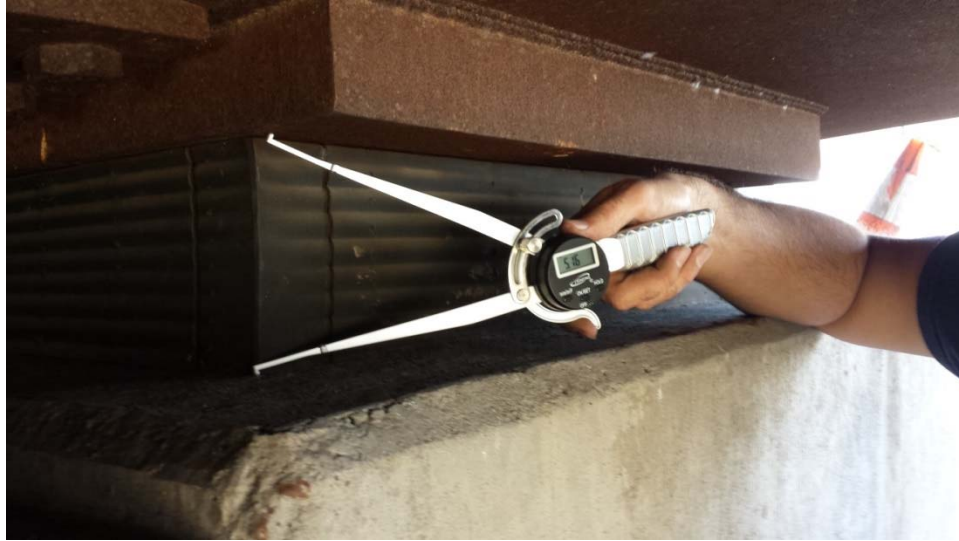
Figure 8.8: Measuring with inside caliper
