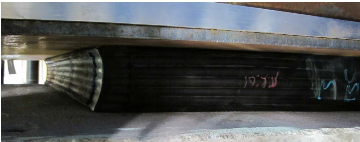
Figure 5.28: Bearing L under combined compression and rotation ( \theta=1.5^\circ )
