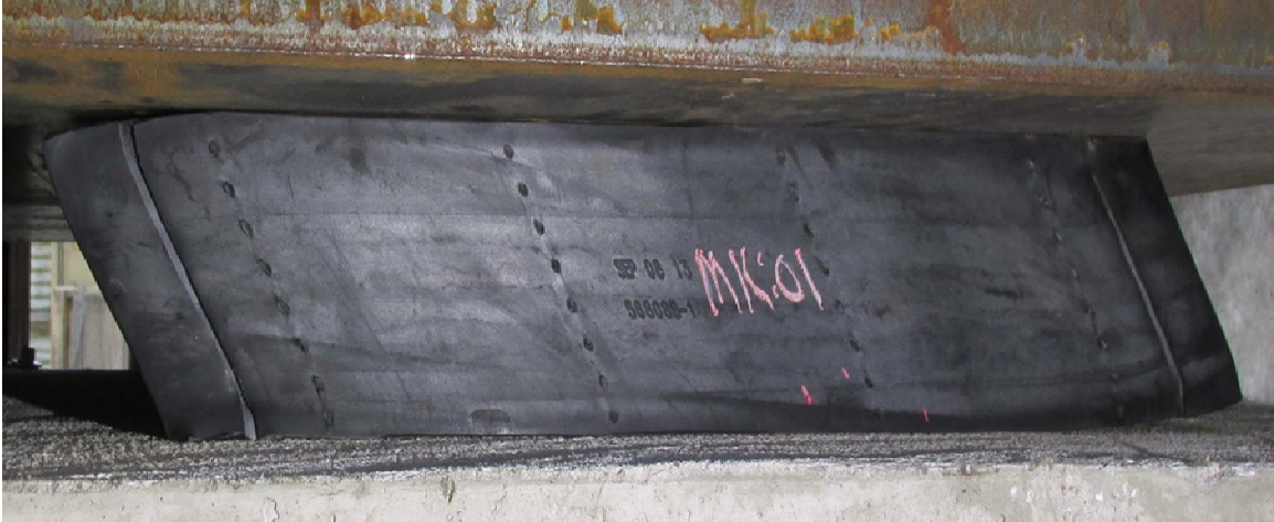
Figure 4.20: Bearing tested in shear
