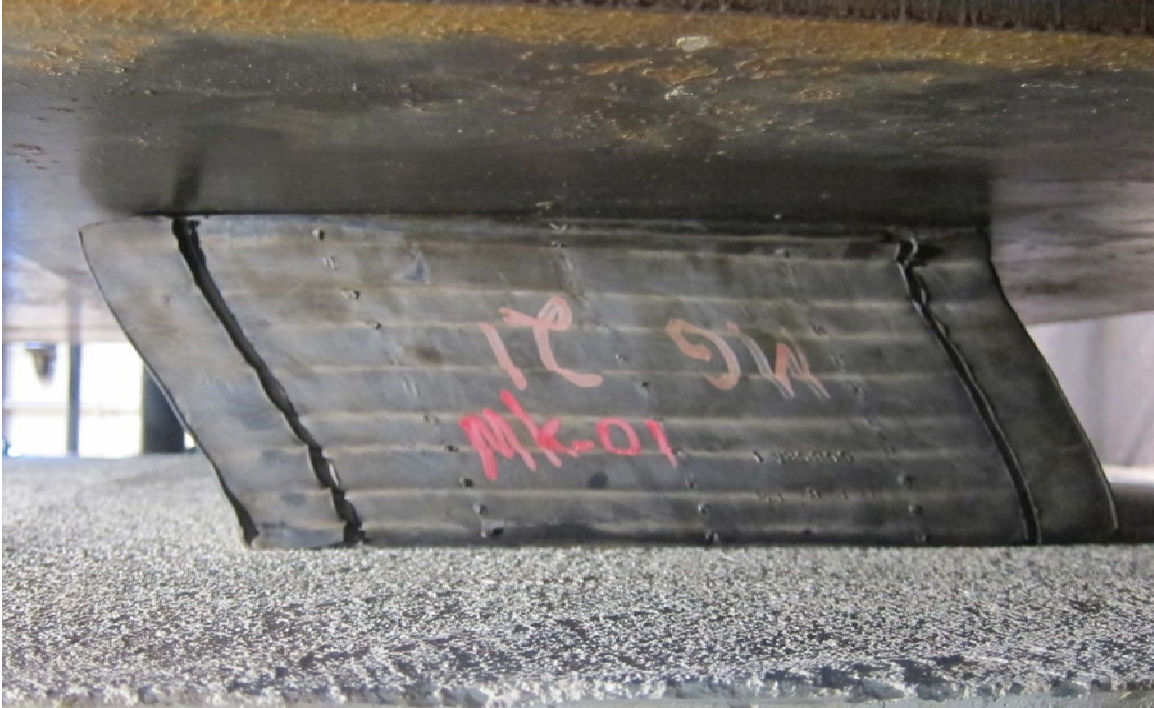
Figure 5.22: Bearing M under 1.5 ksi axial load and 75% shear strain
