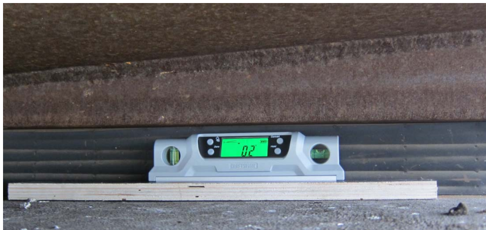
Figure 8.7: Digital level on the concrete surface
