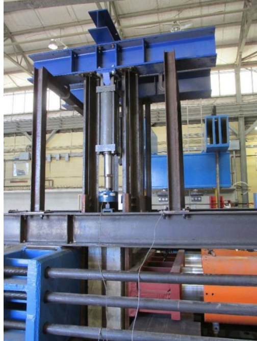
Figure 4.24: Test setup with engaged bearings
