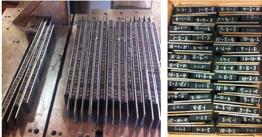
Figure 4.7: Preparing DST specimens from bearing strips
