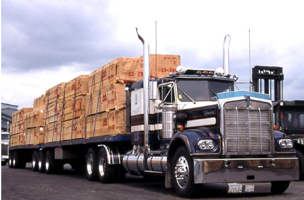
Figure 4.51: Canadian B-Train Double Longer Combination Vehicle
