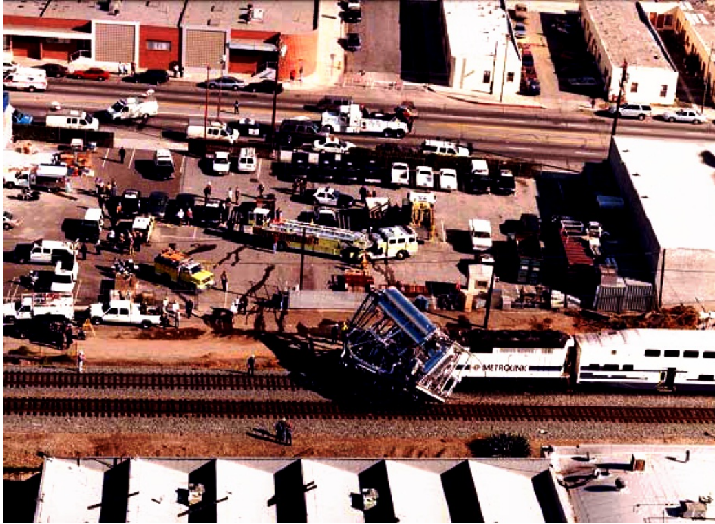
Figure 4.44: Super-Heavy Load with Condenser Struck by Train at Railway Crossing in Glendale, California [NTSB 2000]
