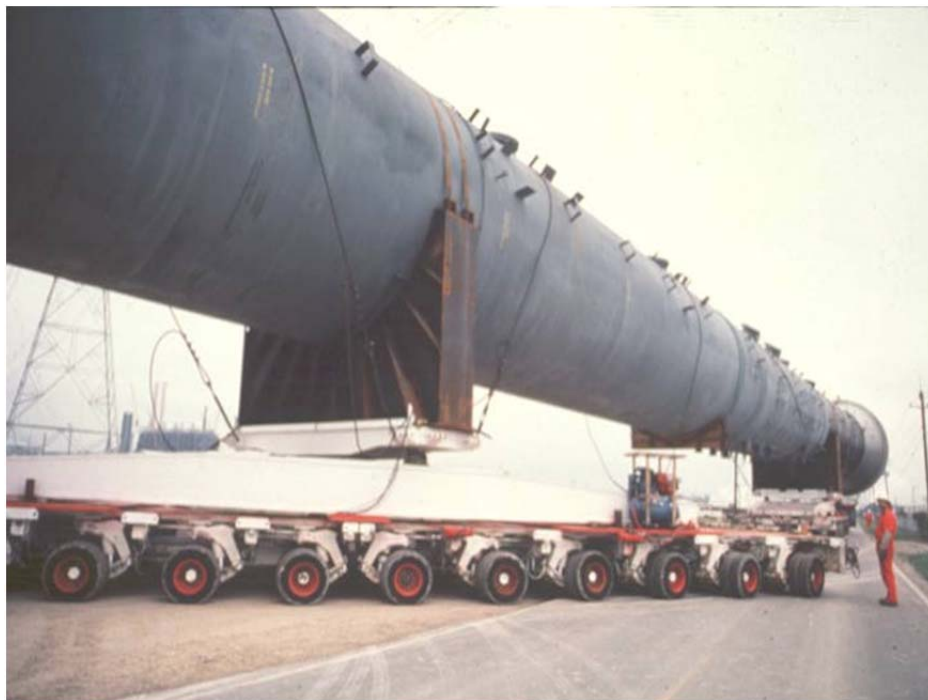
Figure 4.36: Super-Heavy Load during Transport to a Refinery along the Texas Gulf Coast
