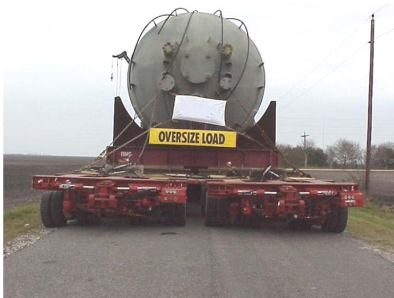
Figure 4.8: 2,000,000 lb. GVW Hydrotreater Reactor on Narrow FM Road
