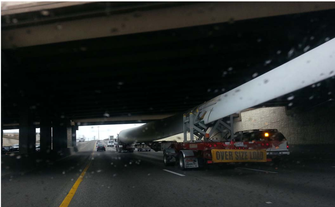
Figure 4.40: Wind Turbine Blade Transporter on IH 35 NB—Austin District
