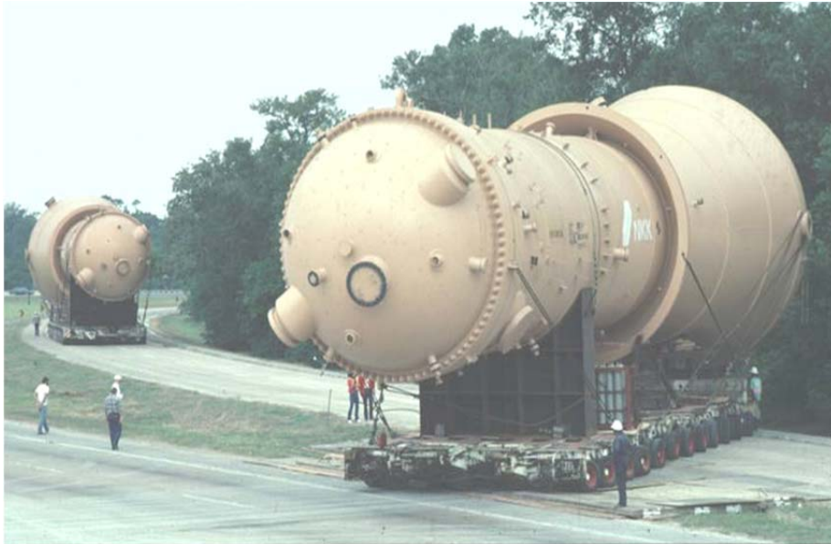
Figure 4.35: Two 1.8 Million Lb. Pressure Vessels Being Transported on a Frontage Road—Houston
