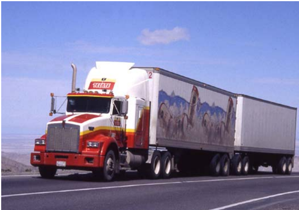
Figure 4.52: Mexican T3-S2-R4 Longer Combination Vehicle
