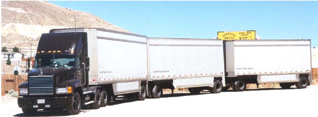
Figure 4.49: Triple Trailer Unit Longer Combination Vehicle
