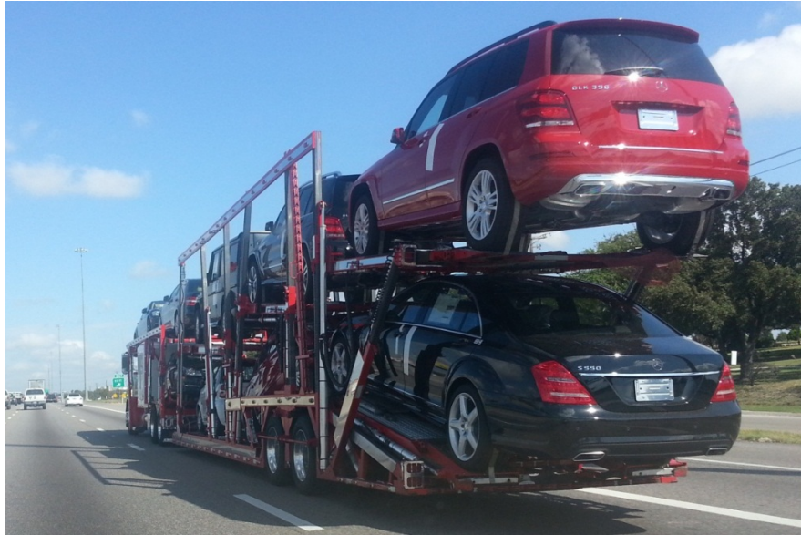
Figure 4.37: Stinger Steered Automobile Transporter on IH 35 NB
