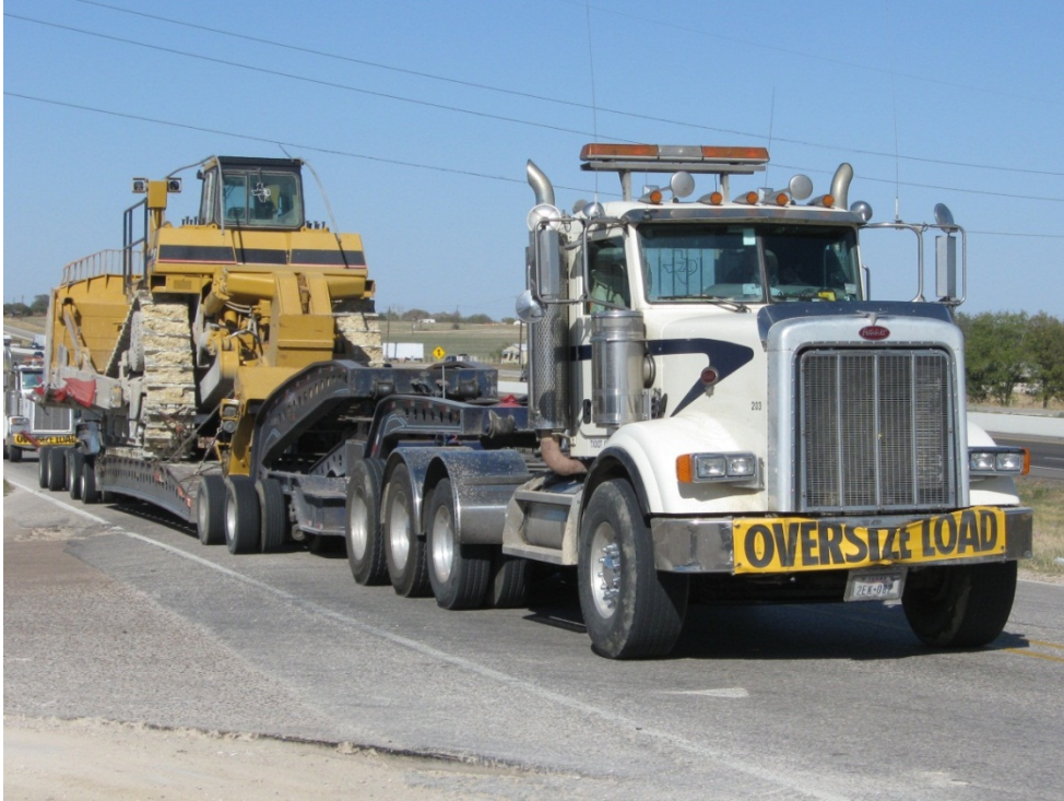
Figure 4.2: General OS/OW Single-Trip Mid-Heavy Range Load Example
