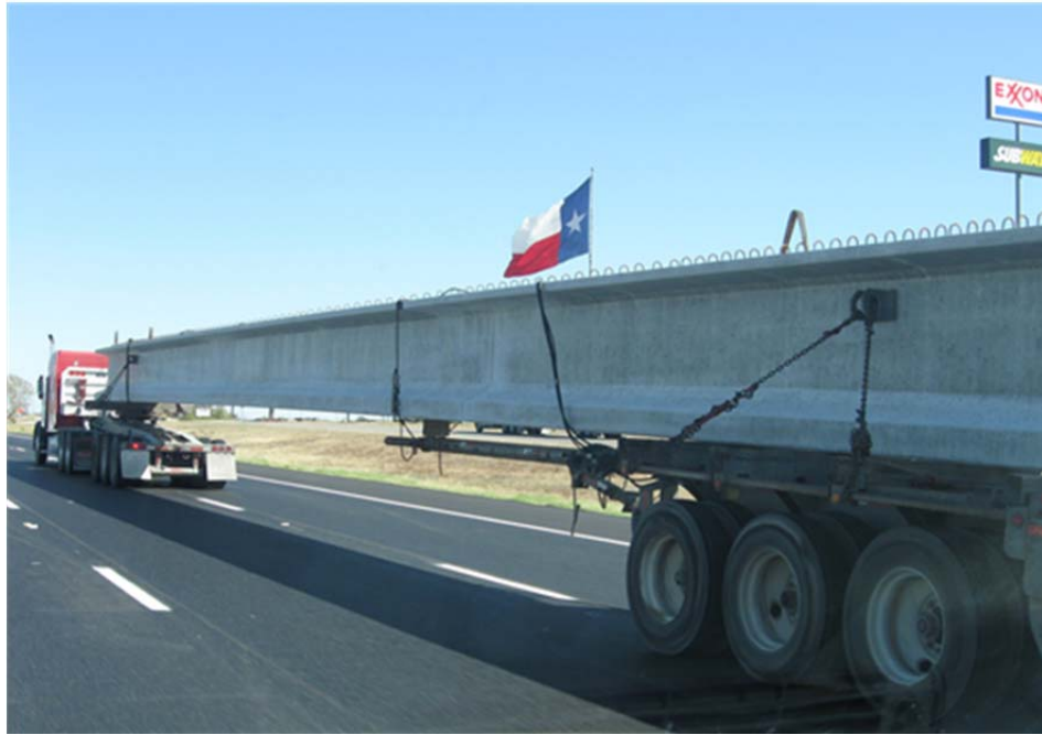
Figure 4.39: Concrete Beam Hauler on IH 35 NB—Austin District
