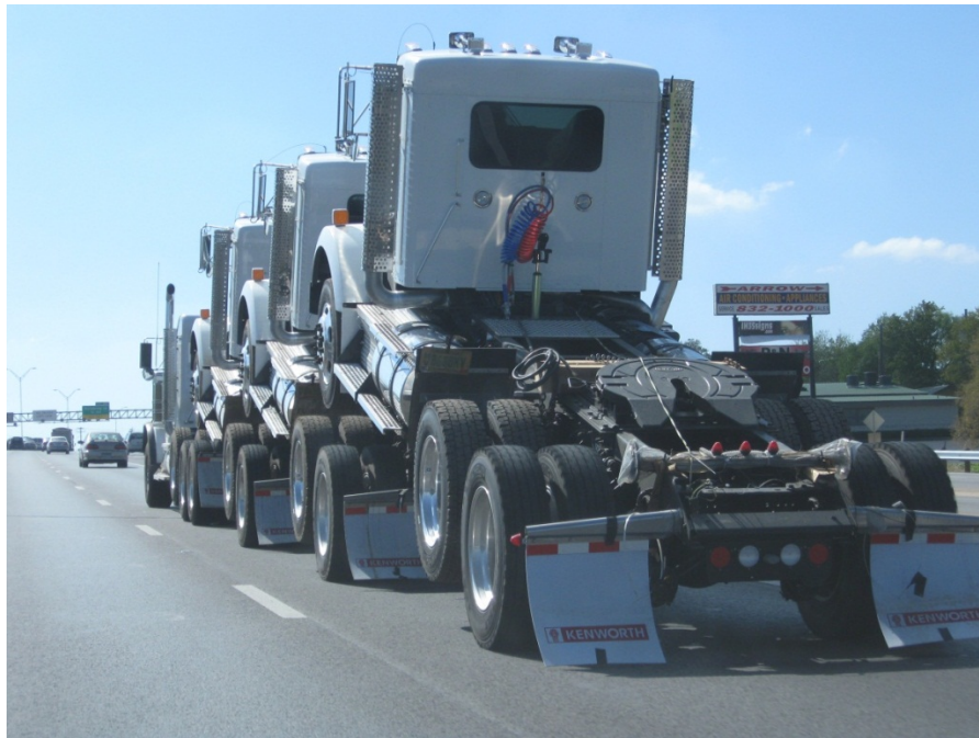
Figure 4.38: Saddle-Mount Truck Tractor Unit Operating along IH 35 SB—Austin District
