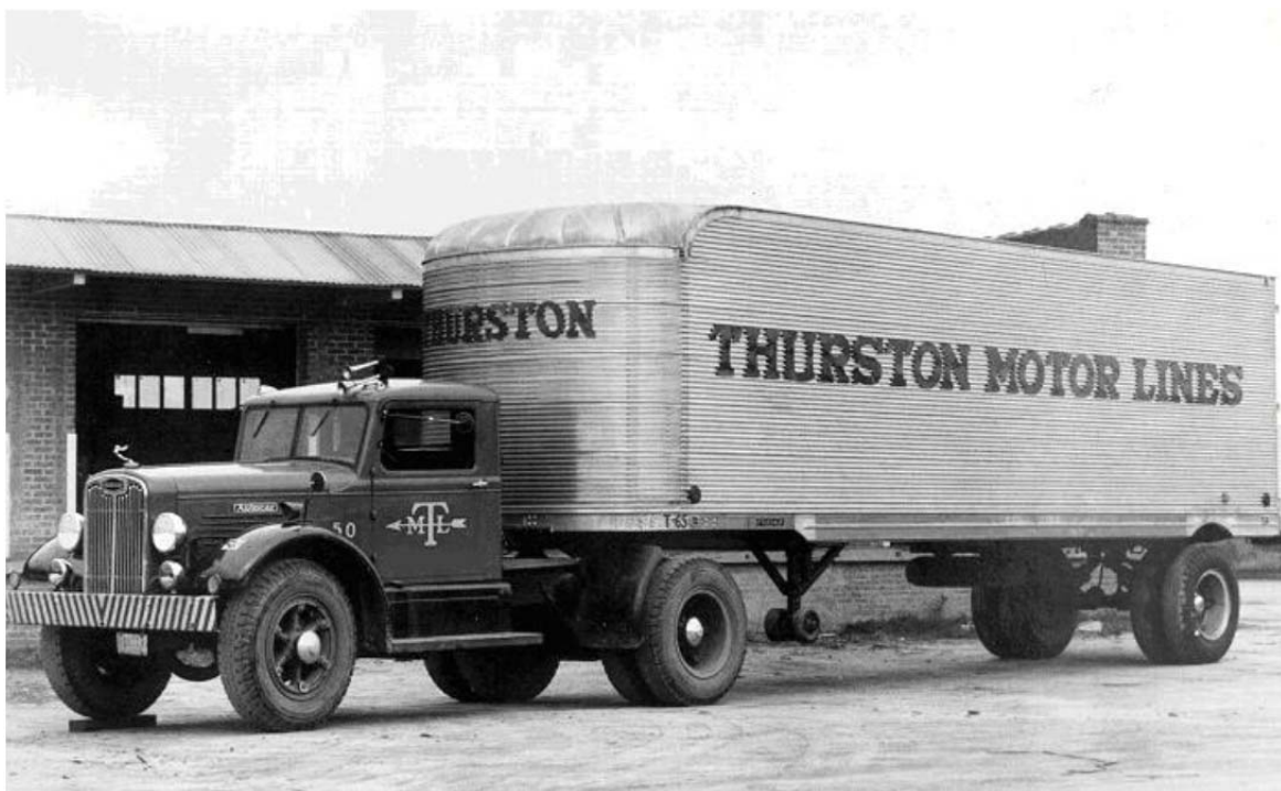
Figure 4.6: Three-Axle Tractor-Semi-Trailer Unit of the 1940s–1950s
