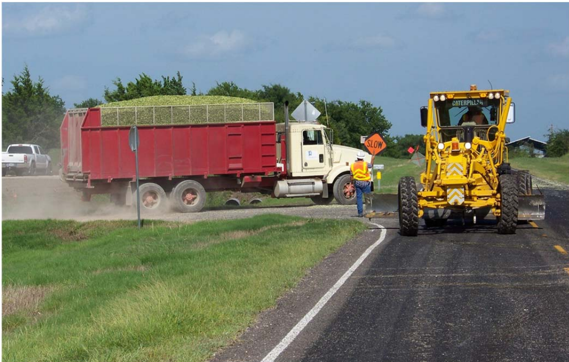
Figure 4.18: Heavily Loaded Three-Axle Straight Truck Transporting Farm Products on an FM Road
