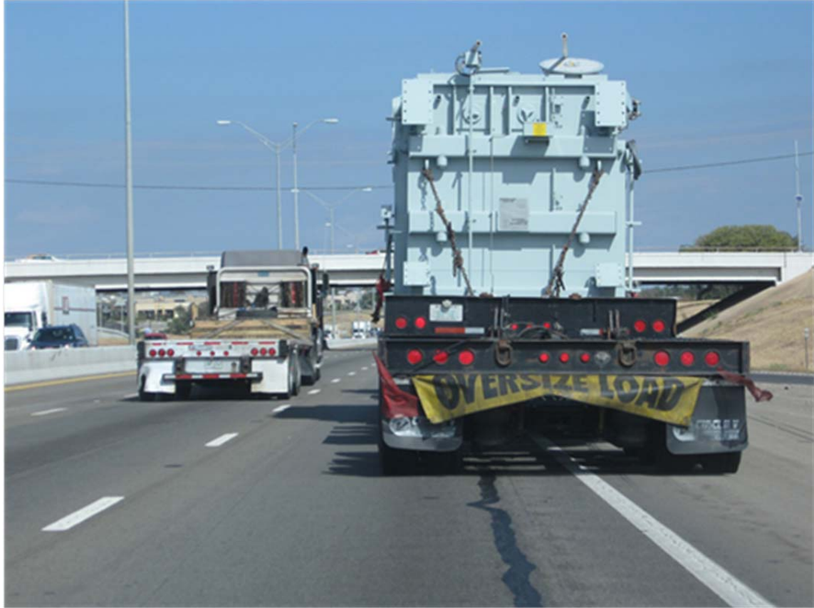
Figure 4.28: Super-Heavy Load Transporter with Transformer on IH 35 NB Main Lanes—Austin
