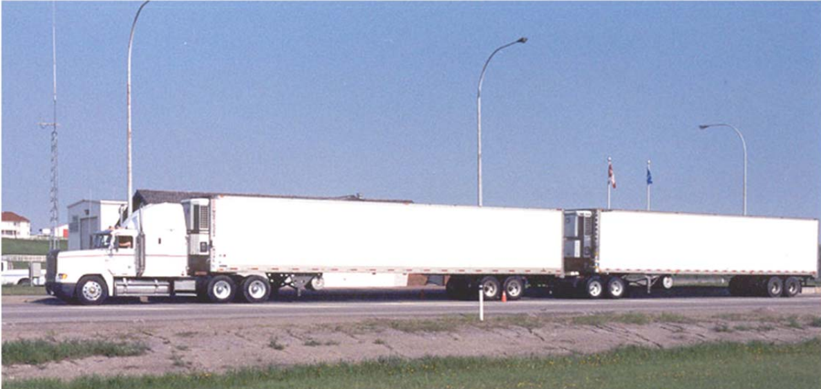
Figure 4.47: Turnpike Double (TPD) Longer Combination Vehicle (LCV)
