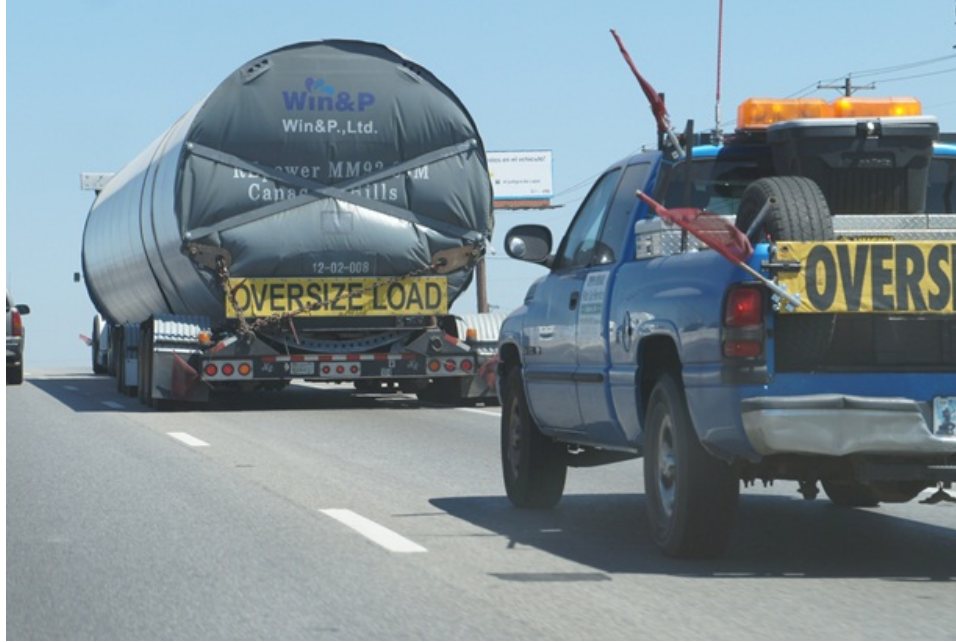
Figure 4.23: Overwidth and Overheight Load IH 35 NB—Austin District
