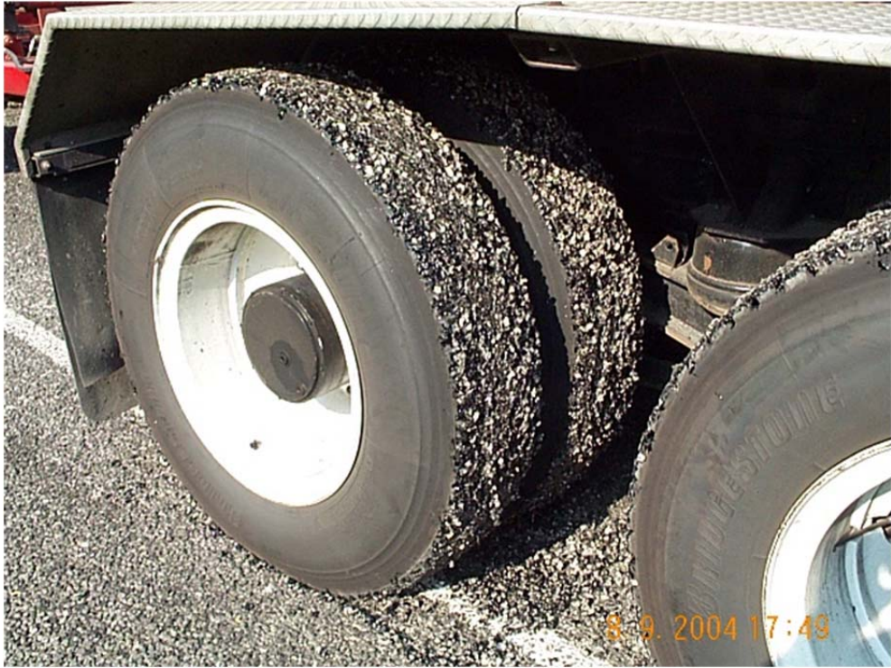
Figure 4.16: Seal Coat Picked Up by Drive Axles of Prime Mover Due to High Surface Shear Forces
