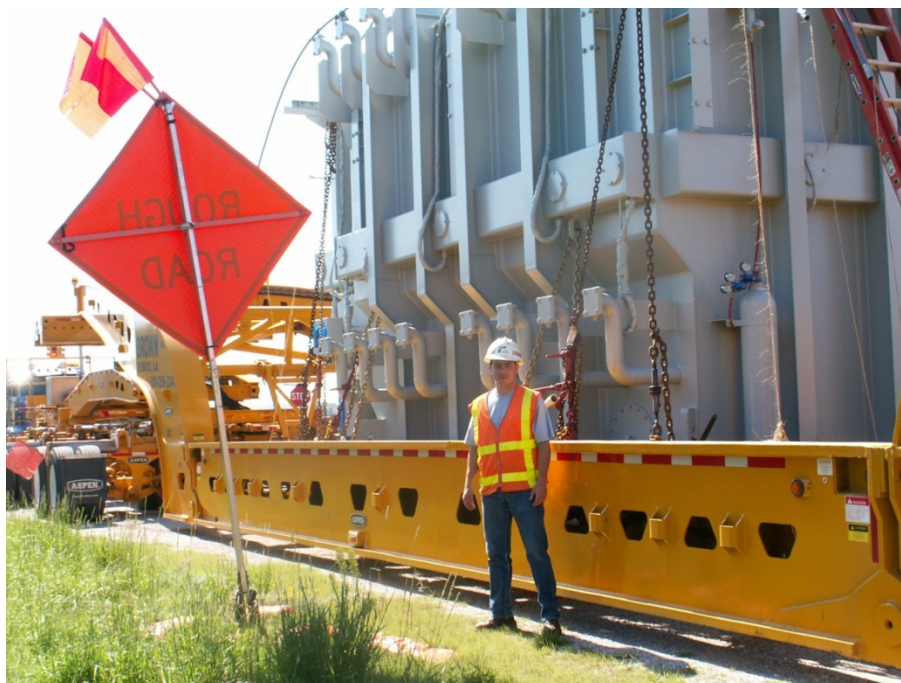
Figure 4.43: Limited vertical clearance under a transporter trailer restricts route choices.
