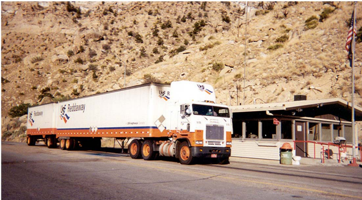
Figure 4.48: Rocky Mountain Double Longer Combination Vehicle
