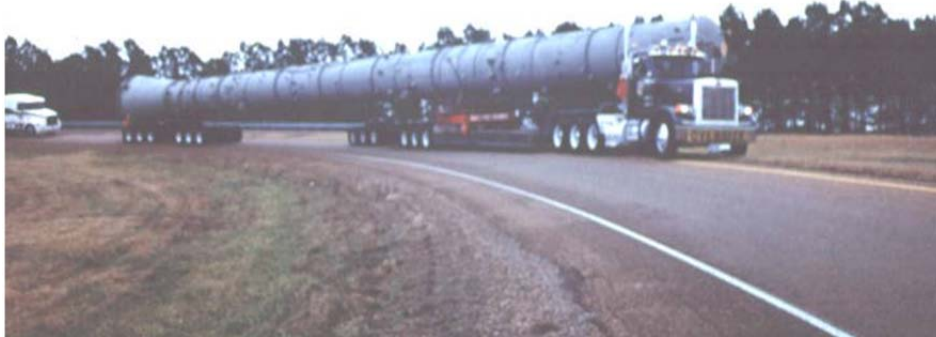
Figure 4.11: Long Load Negotiating a One-Lane Ramp that Required Driving off the Paved Surface
