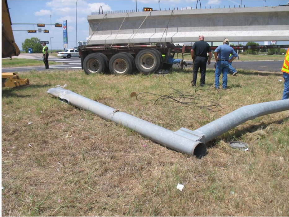
Figure 4.45: Concrete Beam Hauler with Downed Traffic Signal Mast/Arm Assembly—Austin
