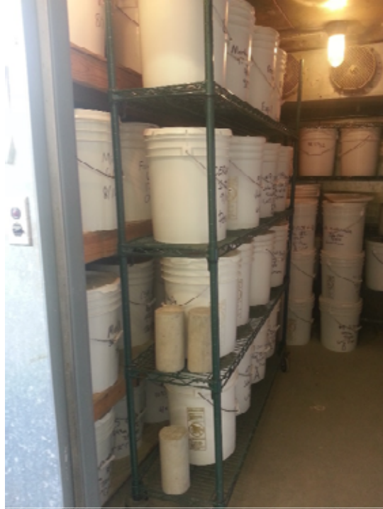
Figure 10.2: Temperature and humidity controlled room for ASTM C 1293 testing
