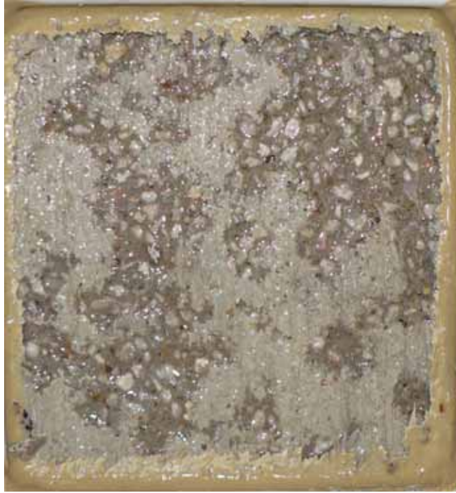
Figure 9.19: CSA-1 samples after 25 cycles (50 unavailable) according to ASTM C 672
