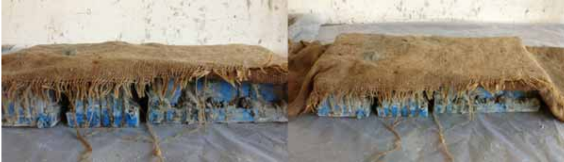
Figure 4.10: Curing set up for Phase I using damp burlap
