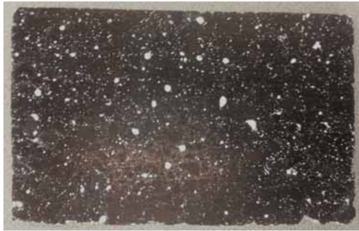
Figure 9.5: Example of final concrete specimen ready for use in RapidAir system
