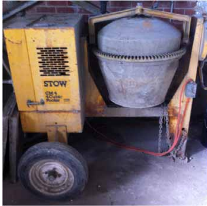
Figure 5.1: 4 ft 3 (.11 m 3 ) steel drum concrete mixer
