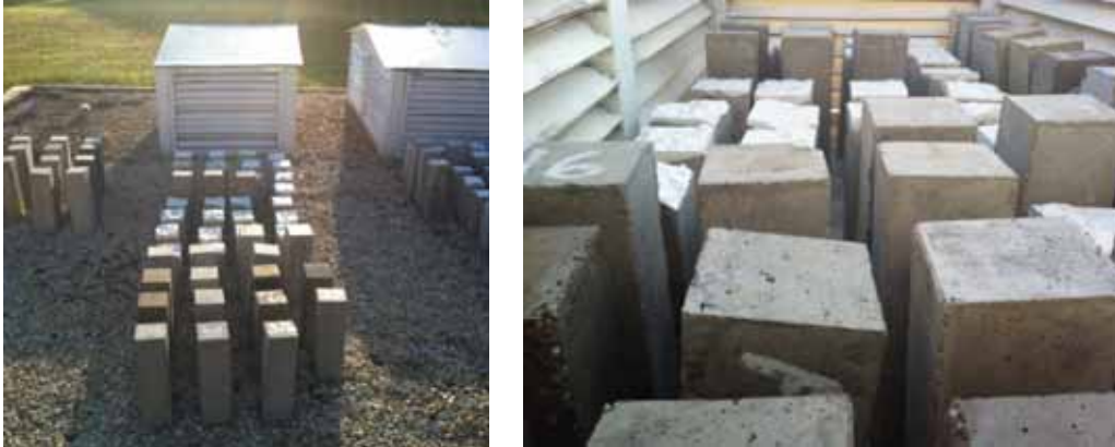
Figure 12.4: Test location of carbonation prisms
