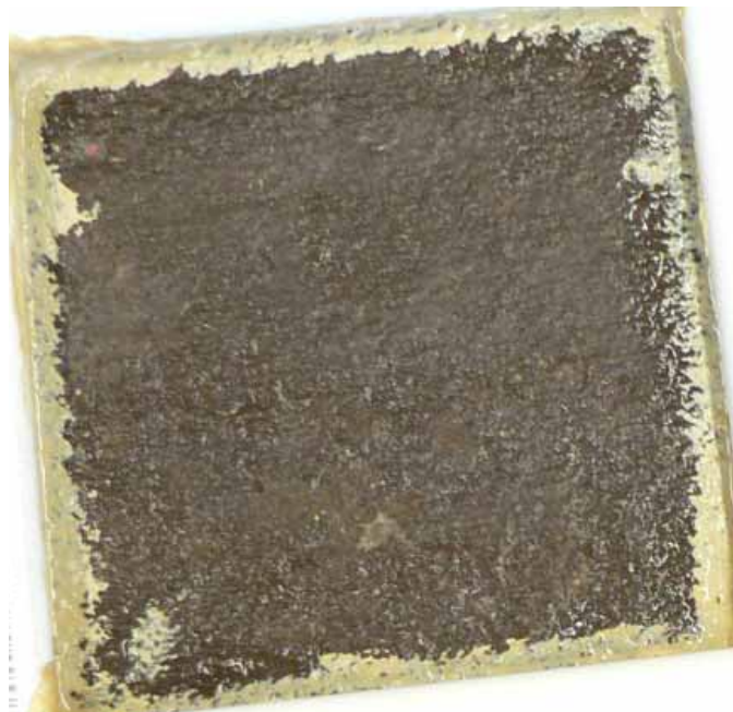
Figure 9.18: CAC-2 samples after 50 cycles according to ASTM C 672
