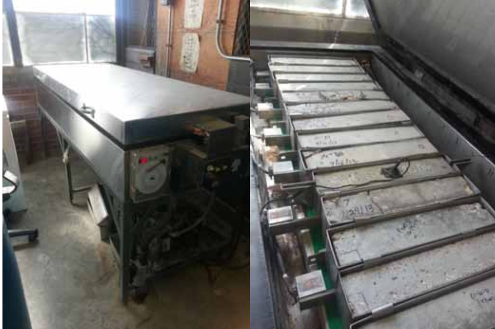
Figure 9.22: Specimens for ASTM C 666 in the freezing-and-thawing chamber
