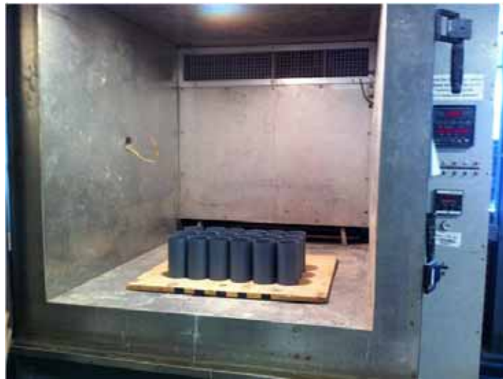
Figure 5.4: Environmental chamber for temperature robustness study
