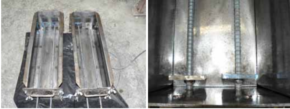
Figure 12.16: Molds for fatigue corrosion specimens displaying reinforcing steel and welded plates for development
