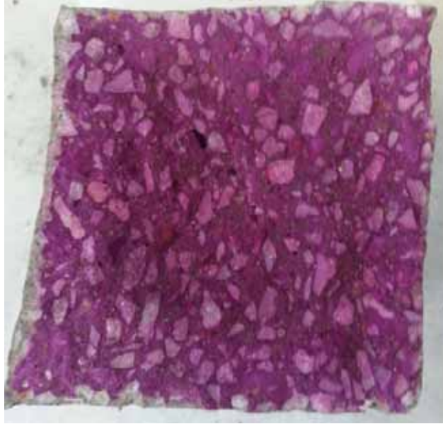
Figure 12.10: PC Type III sample displaying carbonation depth at 11 months using Phenolphthalein PH indicator
