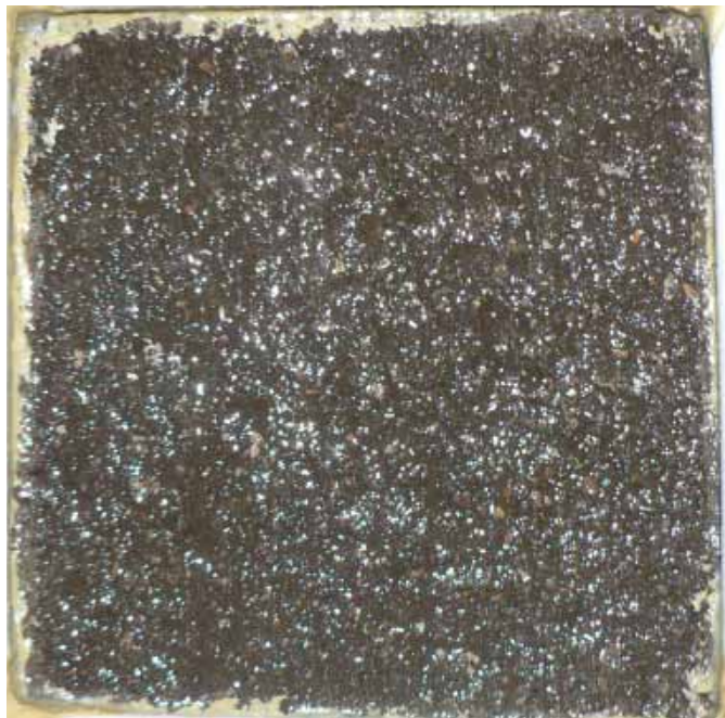
Figure 9.14: CAC-Latex samples after 50 cycles according to ASTM C 672
