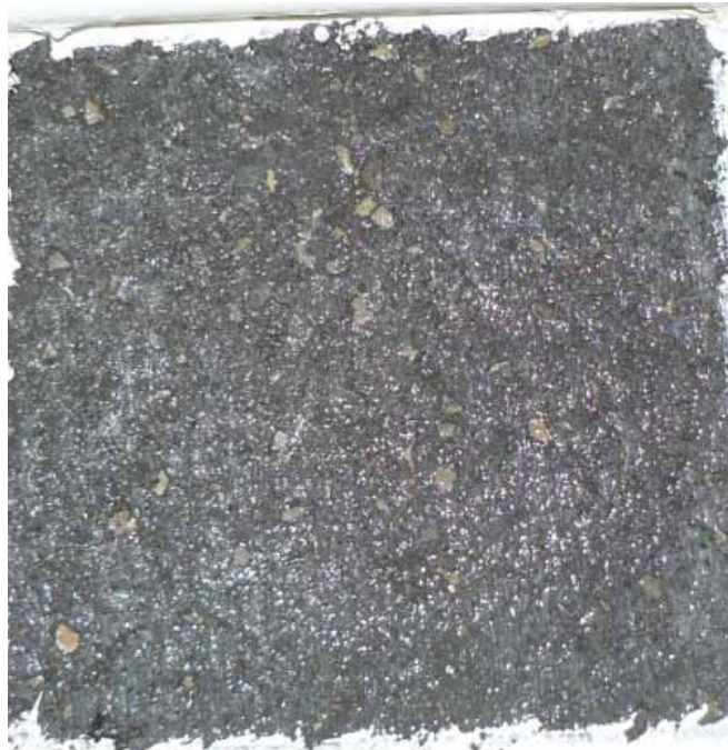
Figure 9.10: P-3 samples after 50 cycles according to ASTM C 672
