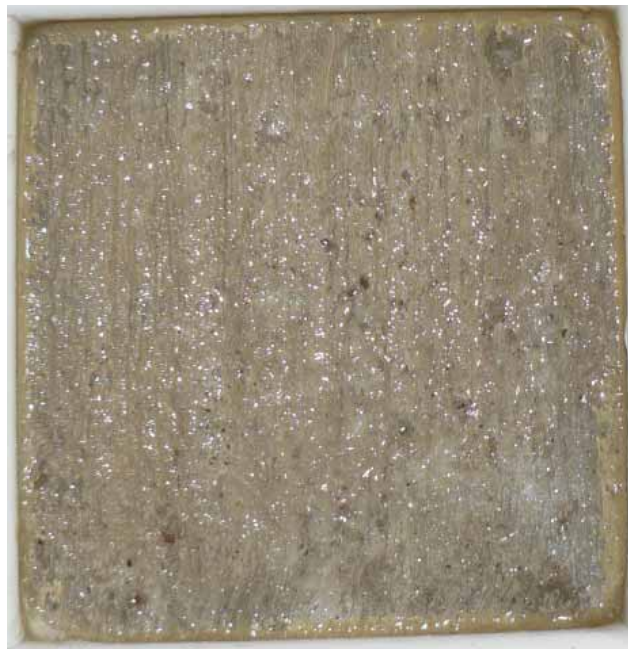
Figure 9.16: CSA-3 samples after 50 cycles according to ASTM C 672
