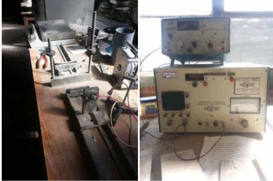
Figure 9.21: Equipment for testing the fundamental transverse frequency of concrete samples according to ASTM C 666
