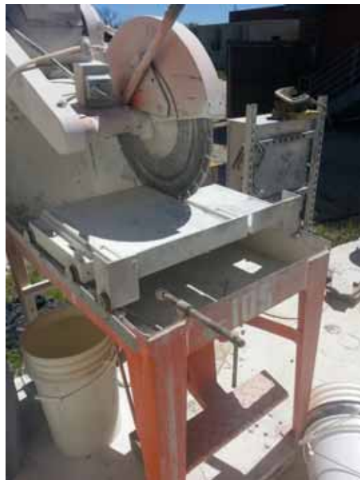
Figure 9.2: Wet saw used for cutting hardened air specimens
