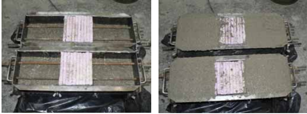
Figure 12.18: Casting top layer of fatigue-corrosion beams and displaying foam inserts for eventual repair material casting
