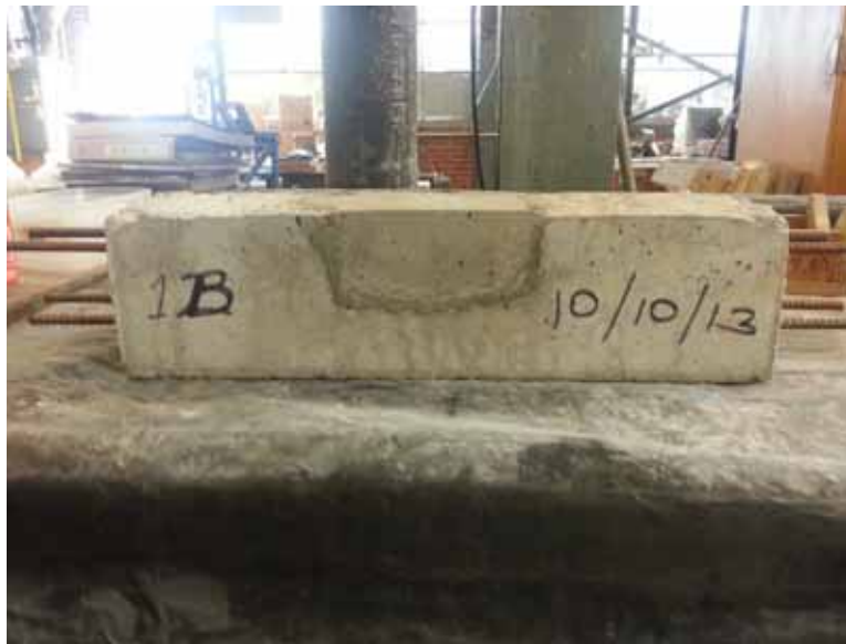
Figure 12.19: Example of final fatigue-corrosion beam and inset repair material
