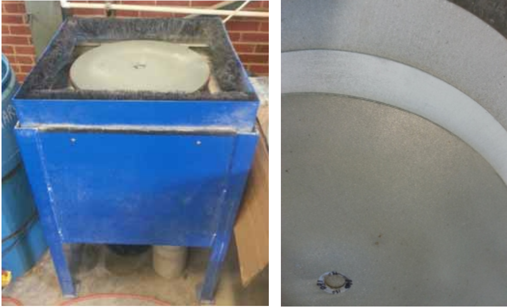
Figure 9.3: Polishing table and various grit plates for polishing hardened air specimens
