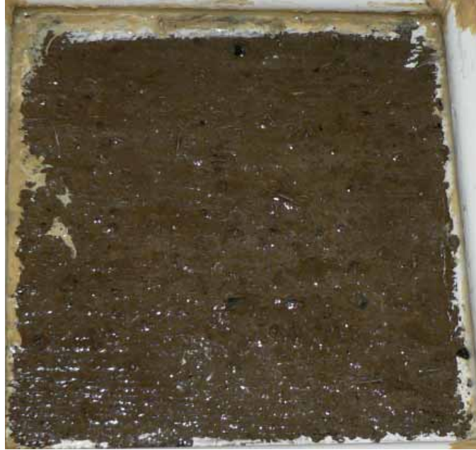
Figure 9.11: P-AAFA samples after 50 cycles according to ASTM C 672
