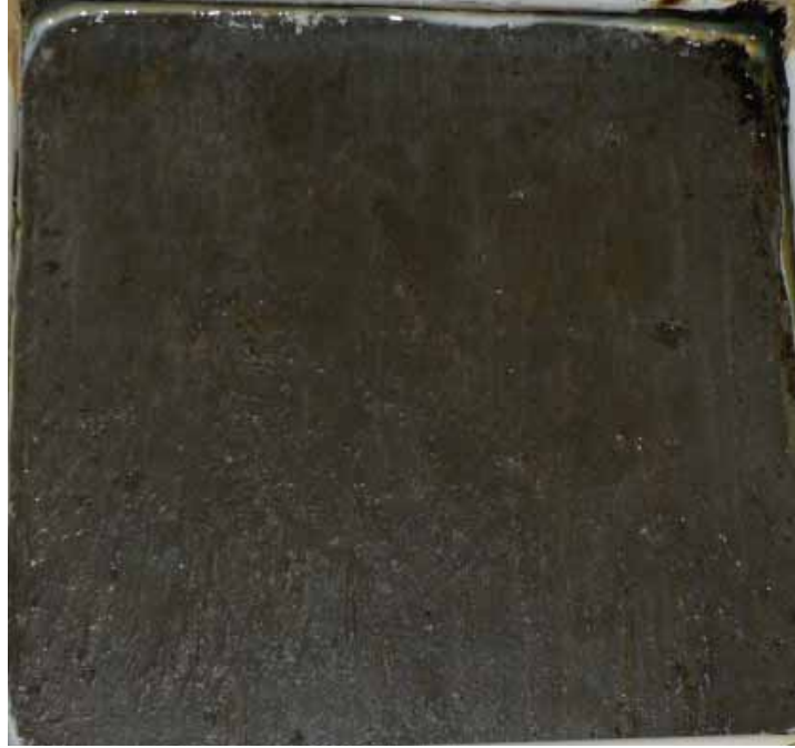
Figure 9.9: P-2 samples after 50 cycles according to ASTM C 672
