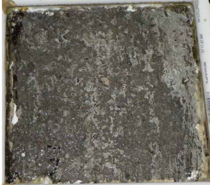
Figure 9.15: PC Type III samples after 50 cycles according to ASTM C 672
