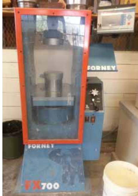
Figure 10.4: Forney FX700 compressive testing machine
