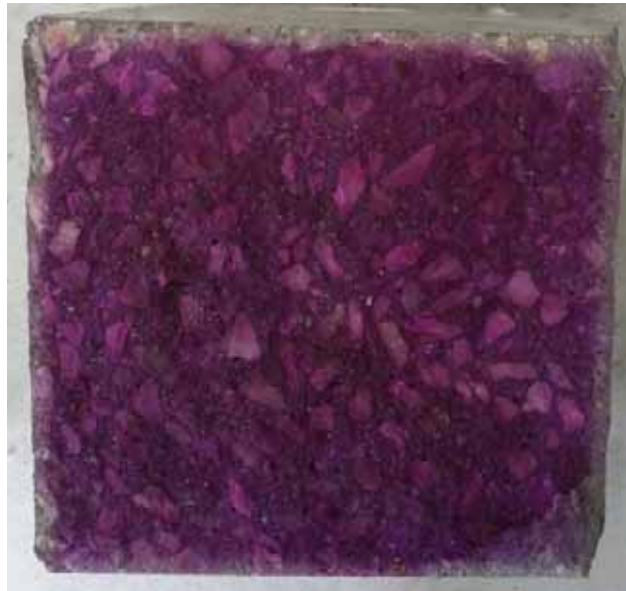
Figure 12.9: P-2 sample displaying carbonation depth at 11 months using Phenolphthalein PH indicator
