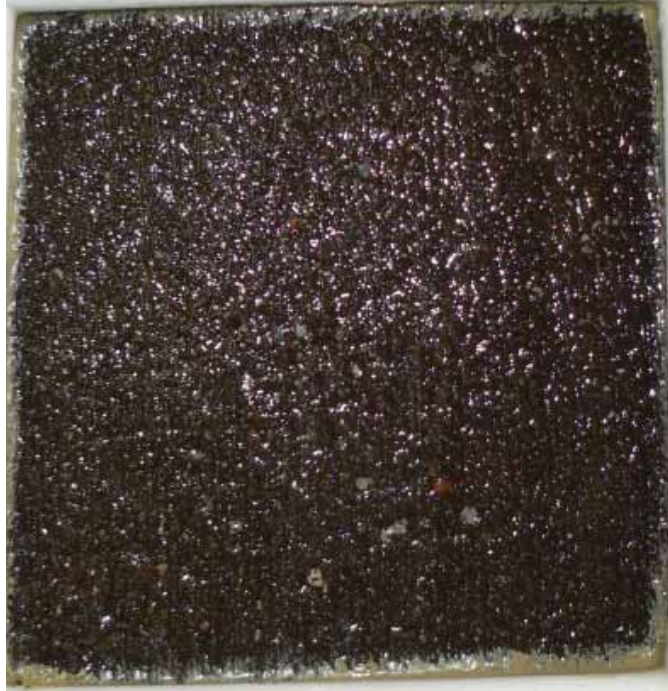
Figure 9.13: CAC-1 samples after 50 cycles according to ASTM C 672
