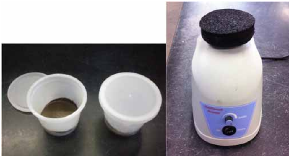
Figure 7.2: A) Grace AdiaCal TC Calorimetry Sample Holder (Bentivegna, 2012) B) Ultrasonic Mixer used for Paste Samples
