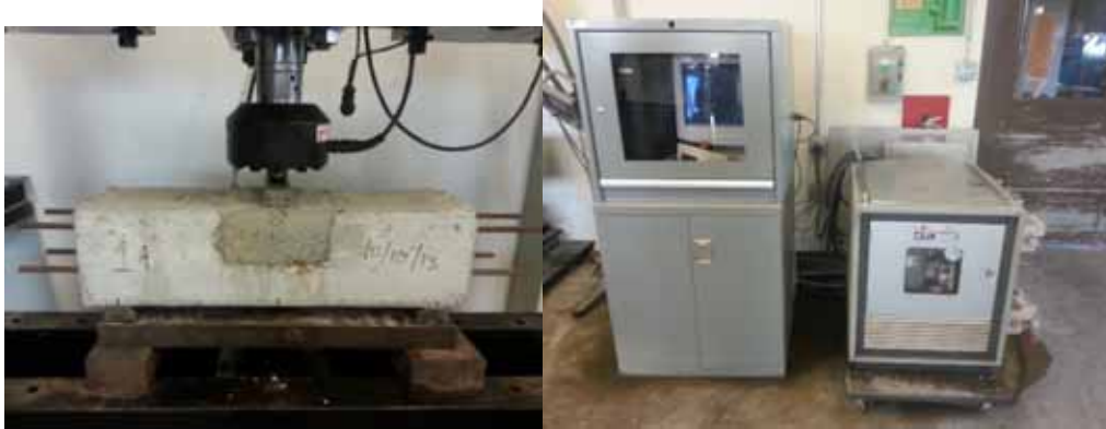
Figure 12.20: Loading fatigue-corrosion beams under repetitive loads using an MTS loading machine
