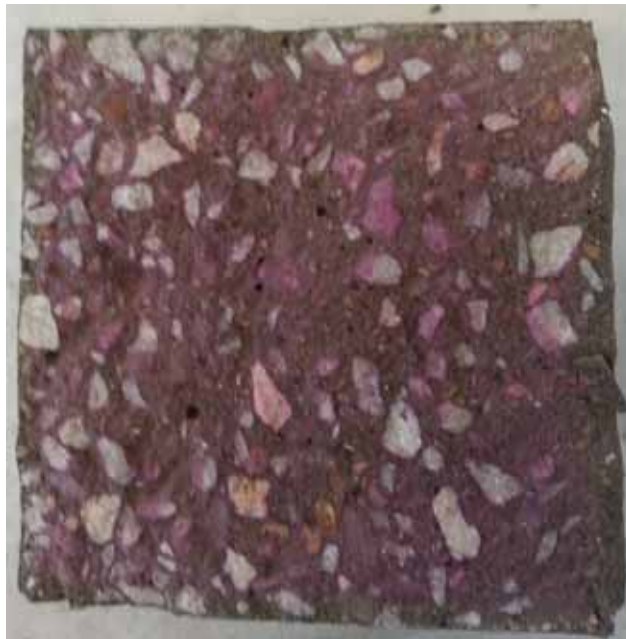
Figure 12.11: CAC-1 sample displaying carbonation depth at 11 months using Phenolphthalein PH indicator
