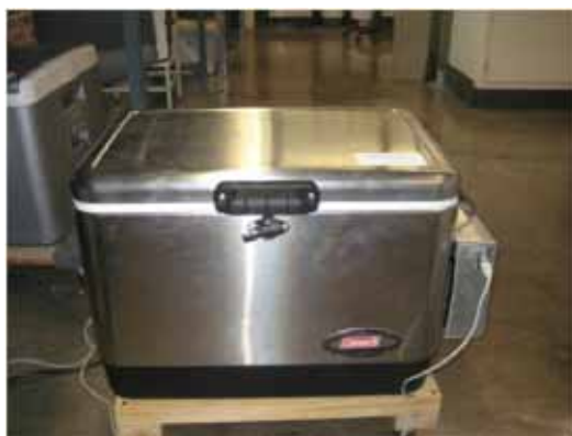
Figure 7.1: Stainless steel calorimeter chamber
