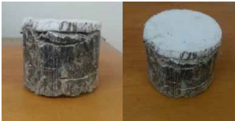
Figure 10.5: P-AAFA samples after attempting pore solution extraction via pore press
