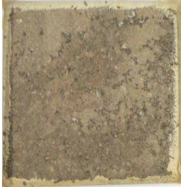
Figure 9.17: CAC-3 samples after 50 cycles according to ASTM C 672
