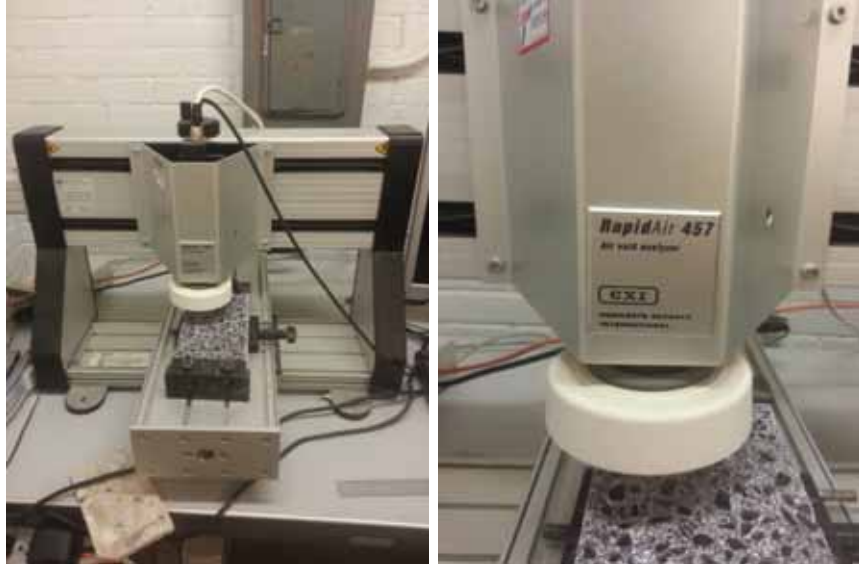
Figure 9.6: RapidAir system used for performing hardened air void analysis
