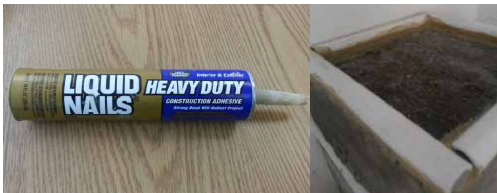
Figure 9.7: Liquid Nails adhesive and typical specimen used in ASTM C 672 testing
