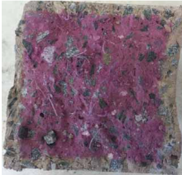
Figure 12.6: P-AAFA sample displaying carbonation depth at 11 months using Phenolphthalein PH indicator
