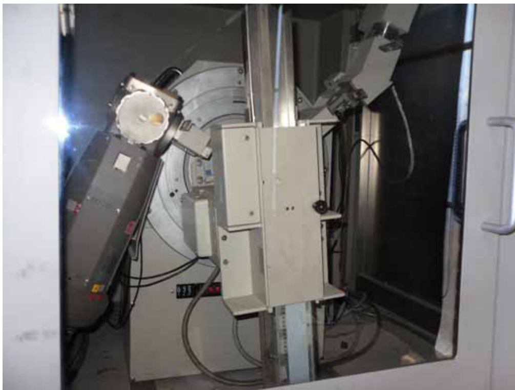
Figure 3.1: Siemens D500 diffractometer used for XRD
