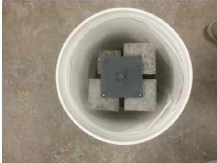
Figure 10.1: Container for moisture and orientation control of prisms for ASTM C 1293 testing
