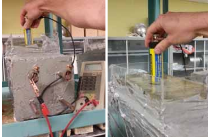
Figure 12.21: Measuring macrocell voltage of reinforcing steel using voltmeter and reference electrode
