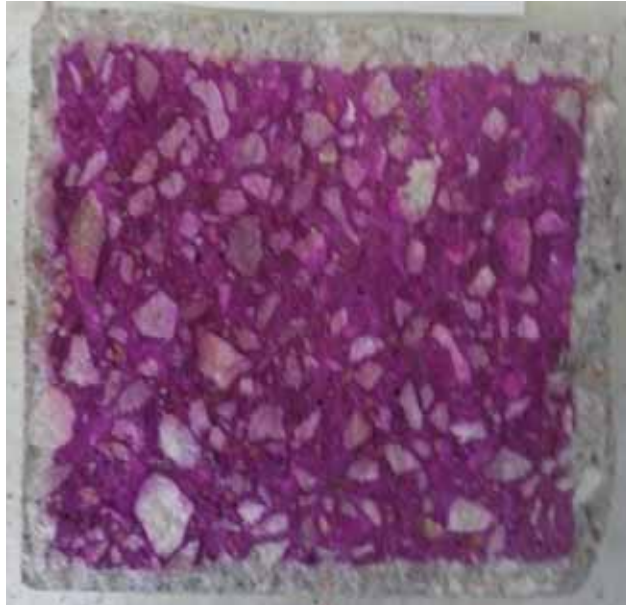
Figure 12.8: CAC-3 sample displaying carbonation depth at 11 months using Phenolphthalein PH indicator
