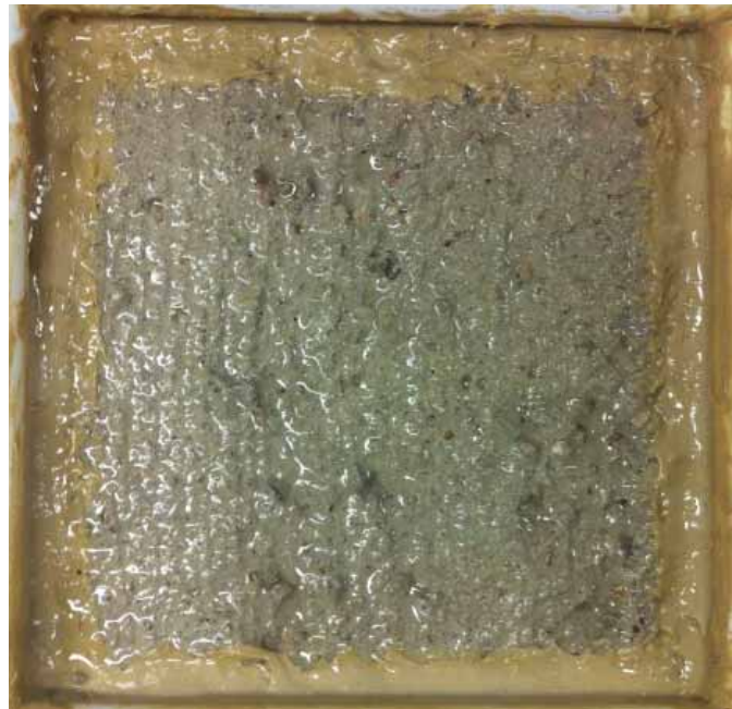
Figure 9.12: CSA-2 samples after 50 cycles according to ASTM C 672
