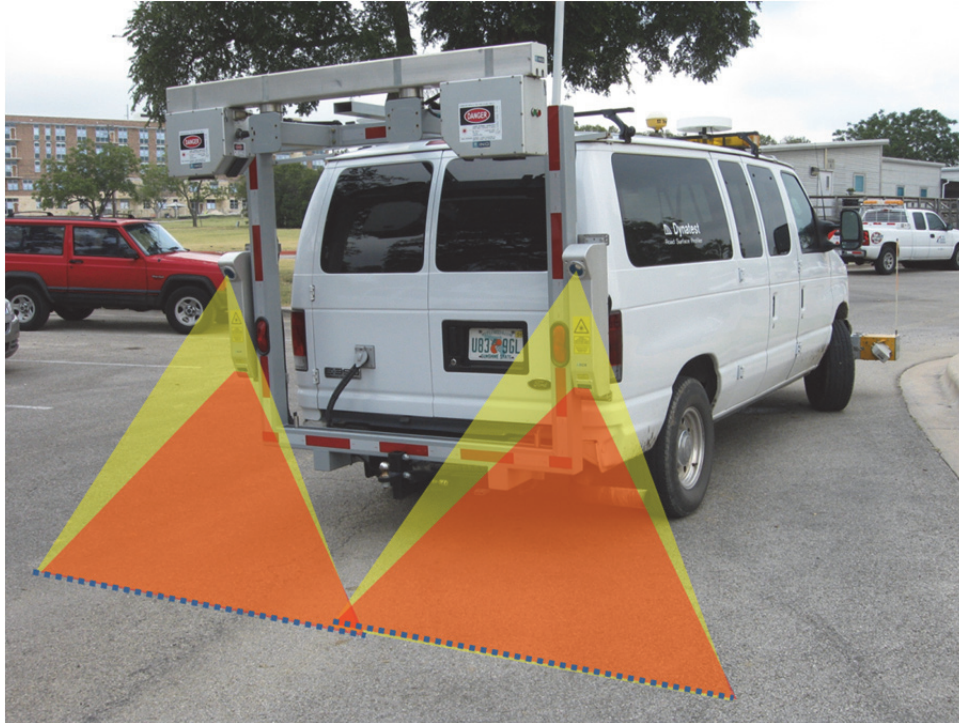
Figure 1.5: The Dynatest INO LRMS automated rut measurement system
