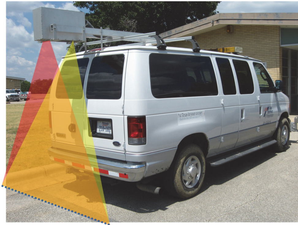
Figure 1.3: TxDOT 3D system for automated measurement of rutting
