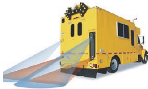
b) INO LRMS mounted on vehicle
