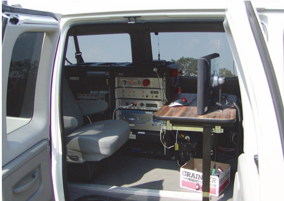
Figure 1.8: TxDOT System's Control Unit
