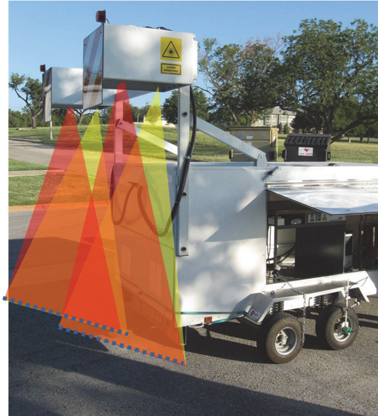
Figure 1.7: The Applus RTD INO LCMS automated rut measurement system
