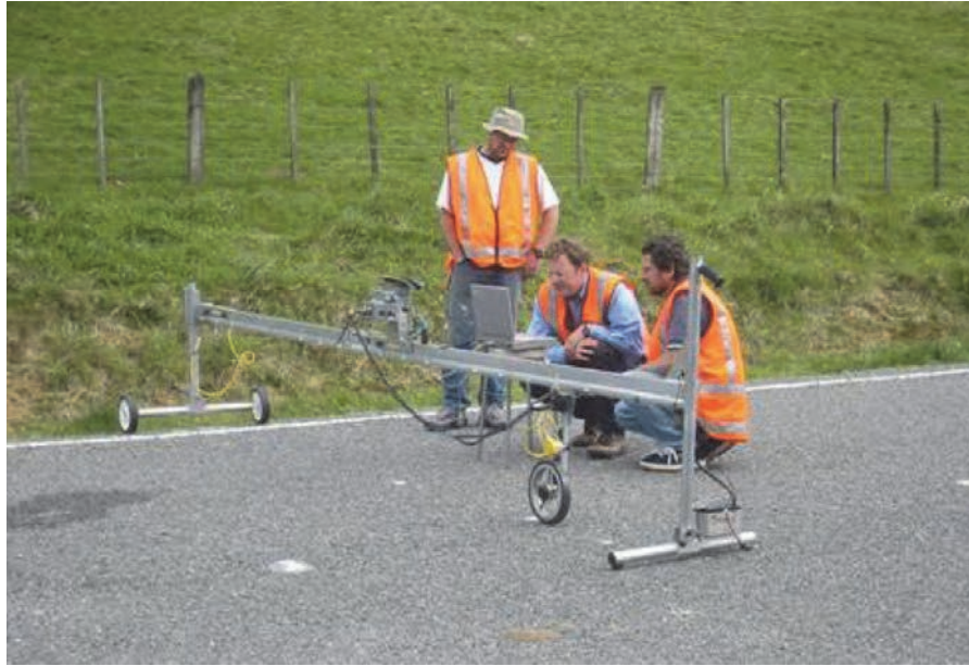
Figure 2.3: ROMDAS “TPB reference profiler” [Henning 2006]
