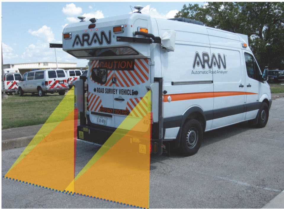
Figure 1.6: The Roadware INO LRMS automated rut measurement system
