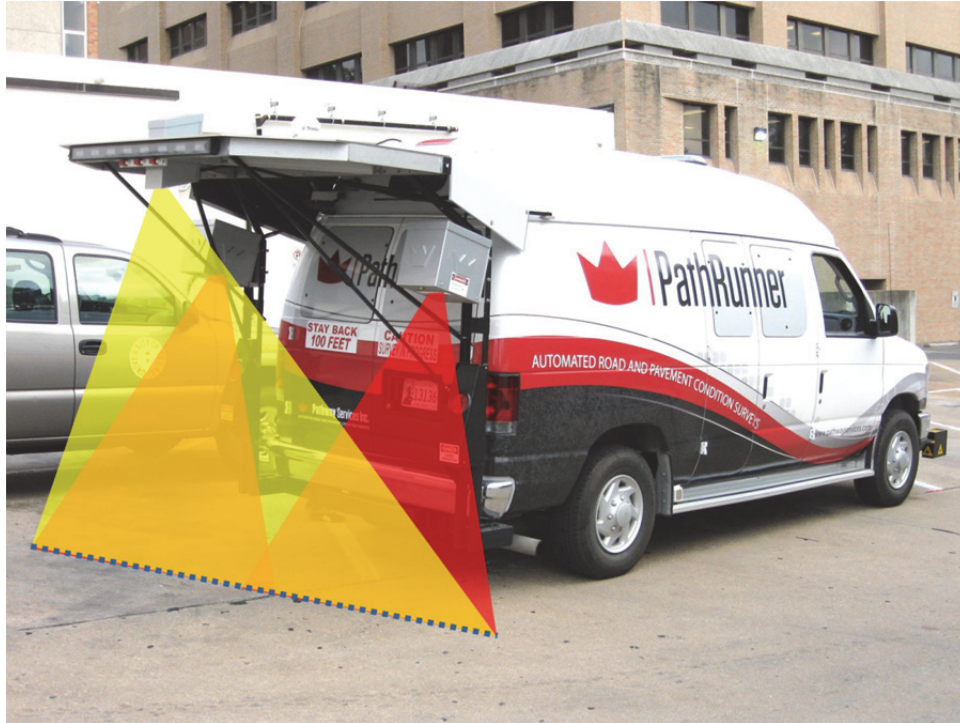
Figure 1.4: The Pathway Services automated rut measurement system
