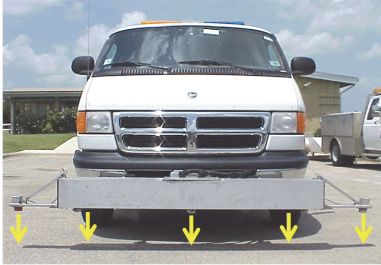
Figure 1.1: TxDOT five-point ultrasonic sensor rut bar showing sensor locations along the bar
