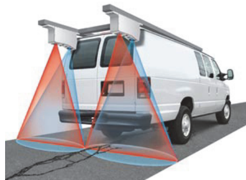
b) INO LCMS mounted on vehicle
