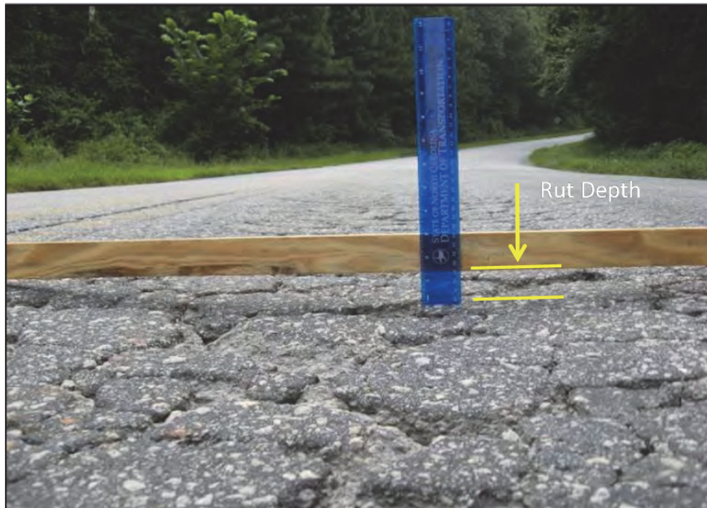
Figure 2.4: Straightedge and rut gage method field measurement
