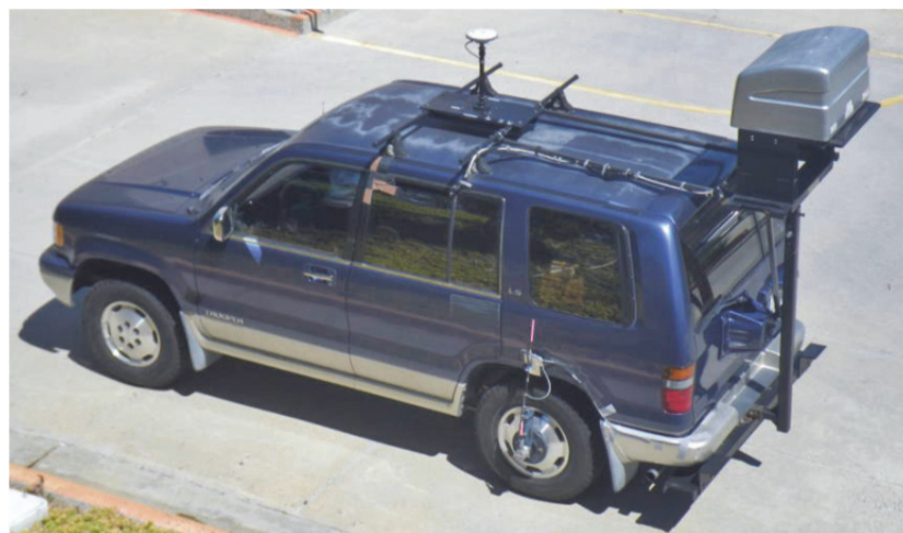
Figure 2.22: PSI PPS scanner mounted on survey vehicle (Herr, 2009)
