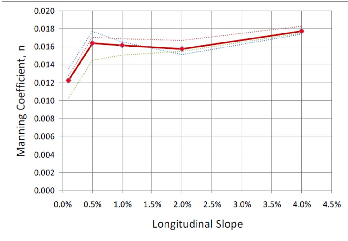
**Figure 4-2 Manning’s Roughness Coefficient as a Function of Longitudinal Slope, Averaged Cross Slope  $S_x = 2\%$  (Blue Dotted Line),  $4\%$  (Red Dotted Line),  $6\%$  (Green Dotted Line), and Average Cross Slope (Solid Red Line) with Discharge Settings  $Q = 1.0, 1.25, 1.5, 1.75,$  and  $2.0$  Revolutions at the Head Box Control Valve for Each Slope Combination**
