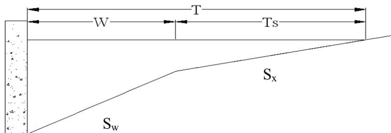
Figure 2-2 Composite Gutter Section (Johnson and Chang 1984)
