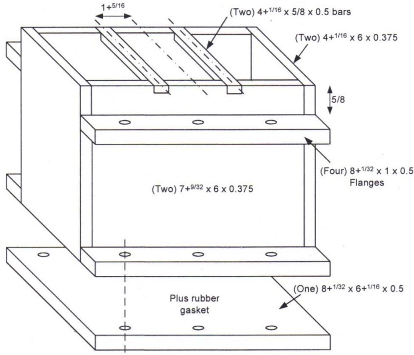
**Figure 3-5 Scaled Drawing of Model Plexiglas Deck Drain**
