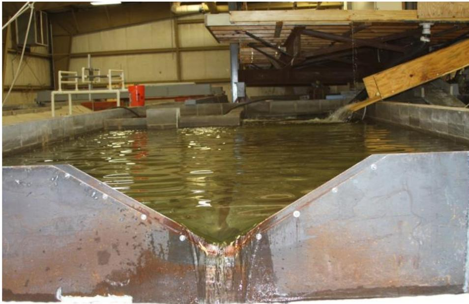
**Figure B-2 Bypass Reservoir and Weir (120 Degree)**
