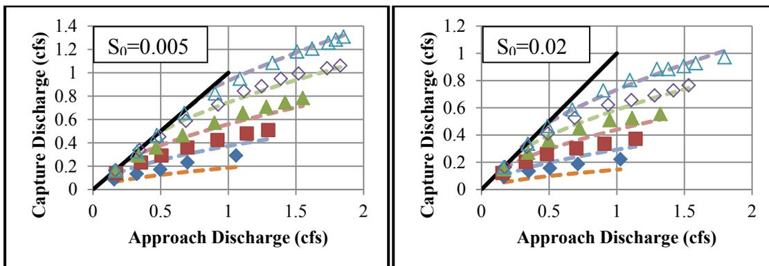
**Figure 4-9 Comparison of Developed Equation Captured Discharge vs. Measured Capture Discharge for 4% Cross Slope and Two Longitudinal Slopes for 6in. × 8in. Drain**
