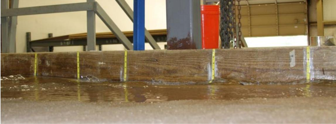
**Figure B-7 Flow Depth against Curb with 5-open 4in. × 8in. Drains at 4% Cross Slope and 0.5% Longitudinal Slope with  $Q = 1.25$  Revolutions at Head Box Valve**
