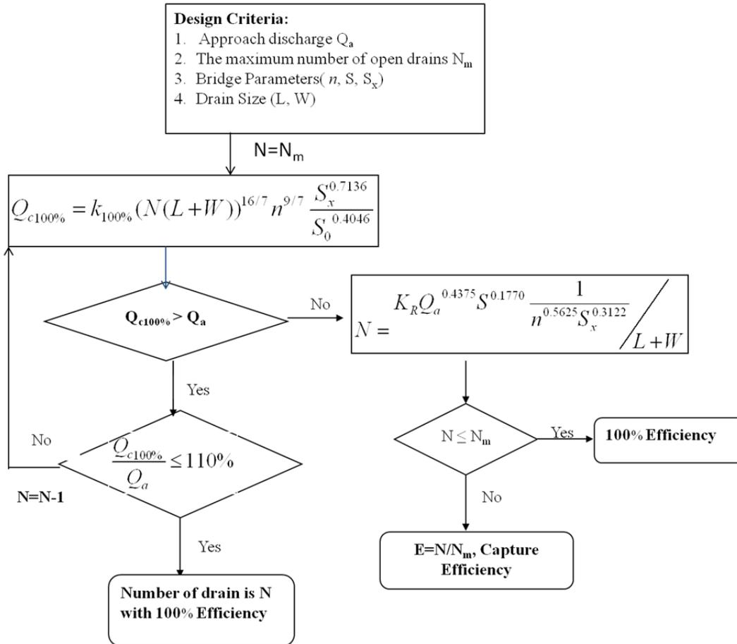
**Figure 5-1 Design Flow Chart for Rectangular Drain**
