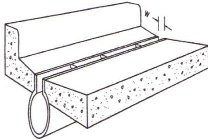
**Figure 2-7 Slotted Inlet Drain (Brown et al. 2009)**
