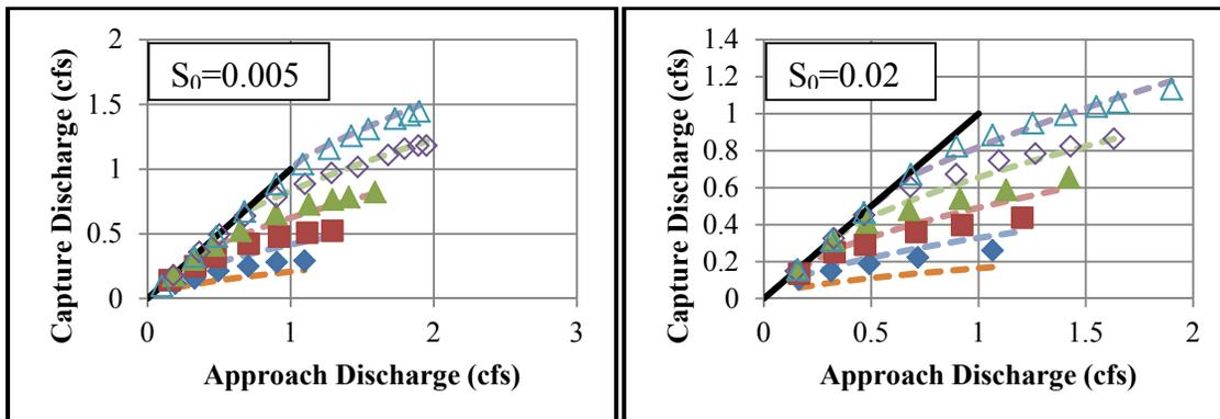
**Figure 4-10 Comparison of Developed Equation Captured Discharge vs. Measured Capture Discharge for 6% Cross Slope and Two Longitudinal Slopes for 6in. × 8in. Drain**
