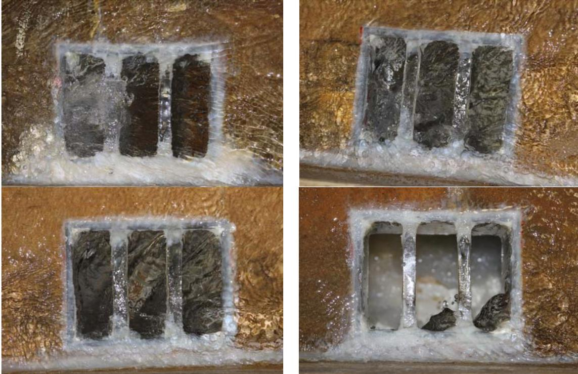
**Figure B-20 Flow from the Right (upstream) into Drains 1 (top-left), 2 (top-right), 3 (bottom-left) and 4 (bottom-right) with 4-open 6in. × 8in. Drains at 6% Cross Slope and 0.5% Longitudinal Slope with  $Q = 1.25$  Revolutions at Head Box Valve**
