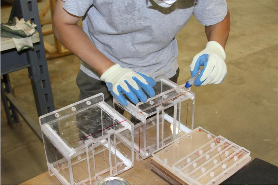
**Figure B-13 6in. × 8in. Drain Flange Construction**
