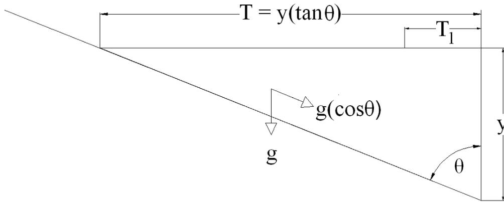
Figure 2-5 Cross Section of Gutter Flow (Li 1954)
