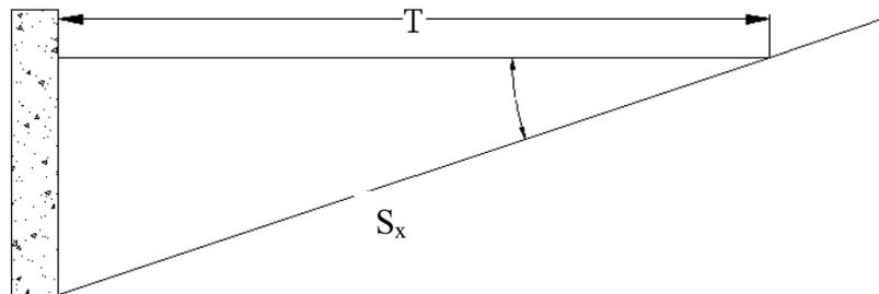
Figure 2-1 Uniform Cross Slope Section (Johnson and Chang 1984)
