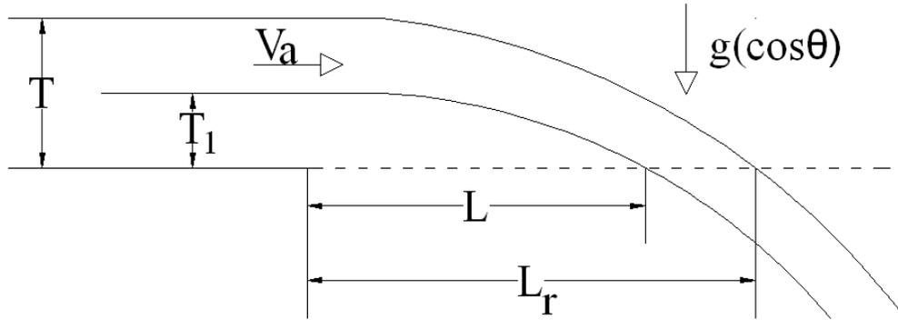
Figure 2-4 Plan View of Lateral Flow (Li 1954)
