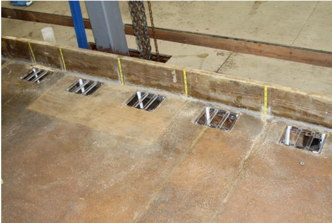
**Figure 3-4 Plexiglas Drain Installments along Model Roadway**
