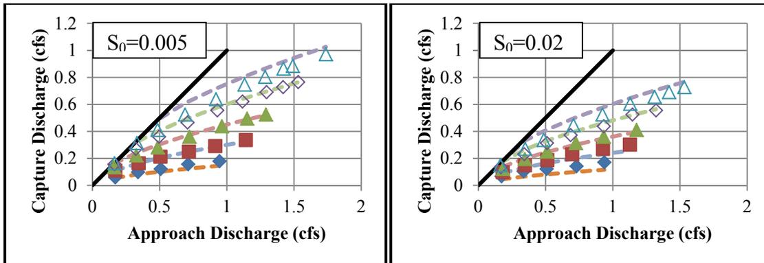
**Figure 4-8 Comparison of Developed Equation Captured Discharge vs. Measured Capture Discharge for 2% Cross Slope and Two Longitudinal Slopes for 6in. × 8in. Drain**
