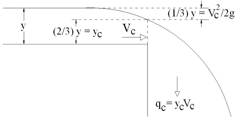
**Figure 2-6 Lateral Flow into a Drain Inlet**
