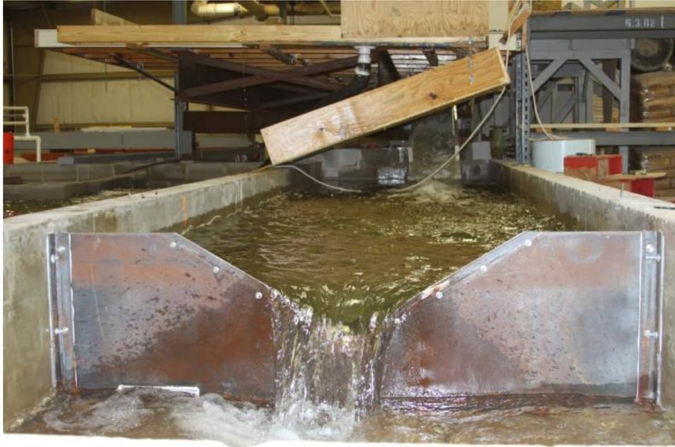
**Figure B-1 Capture Reservoir and Weir (120 Degree)**
