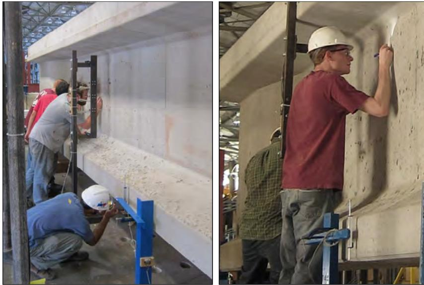
Figure 3.34: Cracks Marked with Felt Tip Marker
