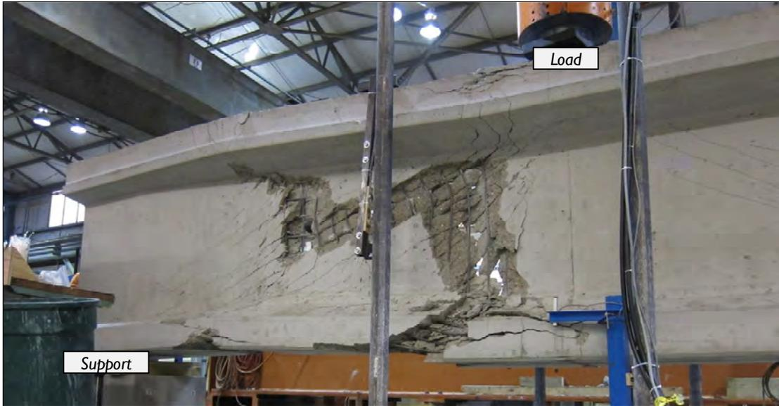
Figure 4.17: Failure of Control Specimen, Tx62-3(S)
