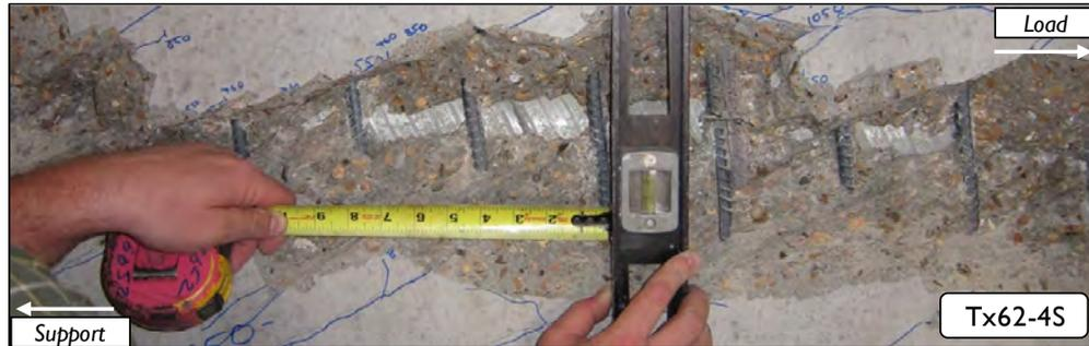
Figure 4.19: Horizontal Displacement between the Top and Bottom of the Duct
