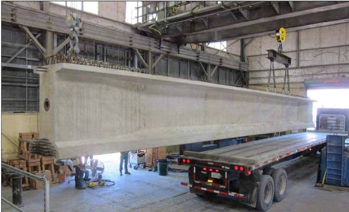
*Figure 3.20: Two Crane Lift System at FSEL*
