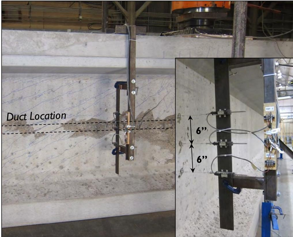
Figure 3.32: Web Expansion Measurement System
