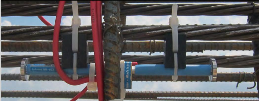
*Figure 3.26: Vibrating Wire Gauge Attached to Top Strands*
