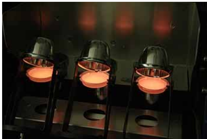
Figure 10.1: XRF Sample Preparation
