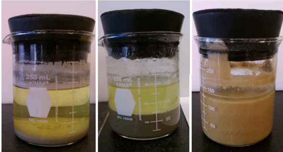
Figure 5.24: Differences in Gel Heights of Low Calcium Ash (left), Moderate Calcium Ash (middle), and High Calcium Ash (right)
