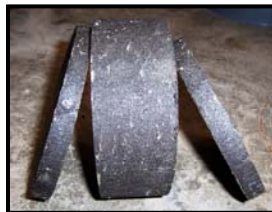
Ends of the compacted sample are removed using a saw
