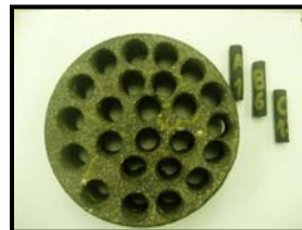
About 15 to 20 test specimens are cored from a single SGC compacted sample
