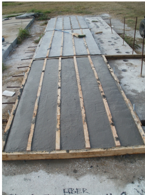
Figure 4.10: Customized Restrained Shrinkage Slabs
