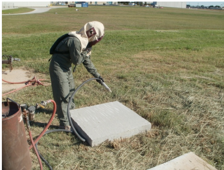
Figure 4.11: Sandblasting in progress
