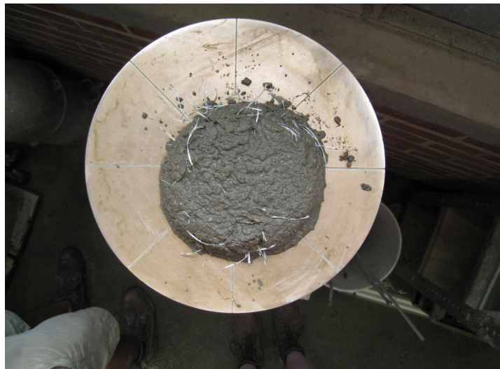
Figure 4.6: Mortar with fiber before adding WRDA 82
