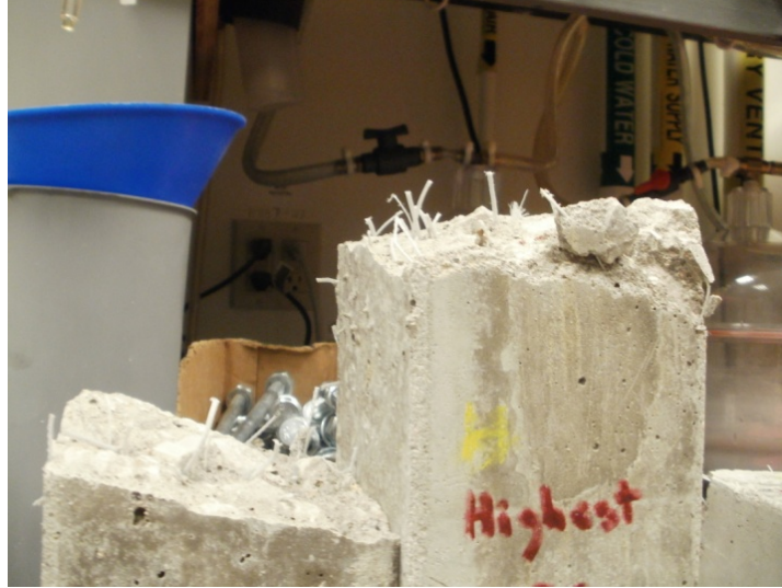
Figure 4.27: Failed interface of the specimen with highest ARS
