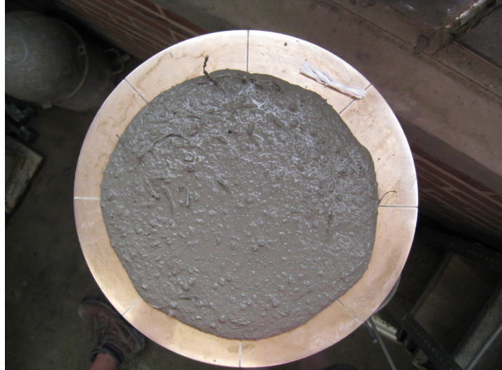
Figure 4.7: Mortar with fiber after adding WRDA 82
