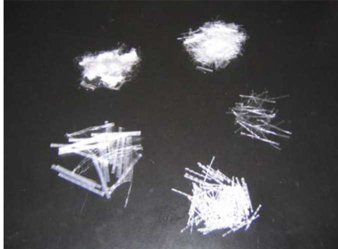
Figure 2.3: Different forms of polypropylene fibers
