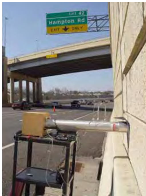
Figure 2.9: Impedance tube in situ testing of IH-30 retaining wall
