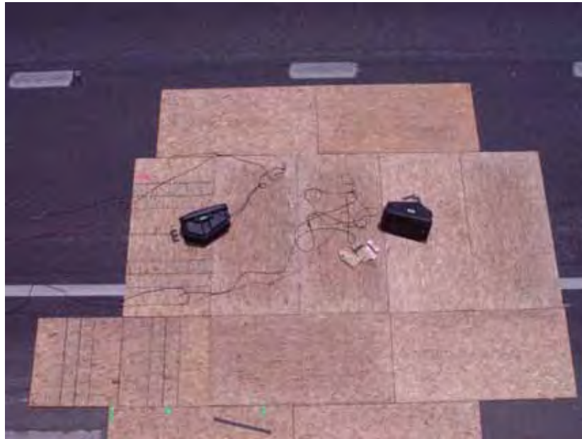
Figure 2.8: MLS test with speakers placed on plywood to reduce propagation absorption from PFC
