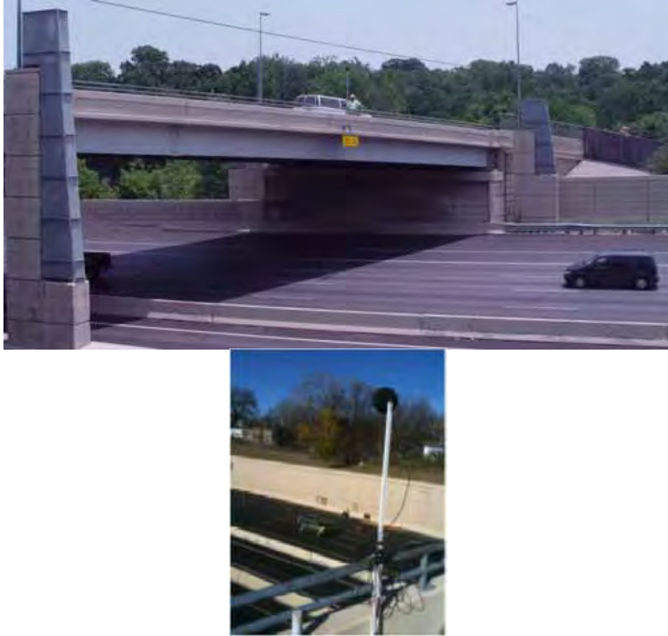
Figure 2.5: Measuring reflected noise from the Edgefield Avenue Bridge
