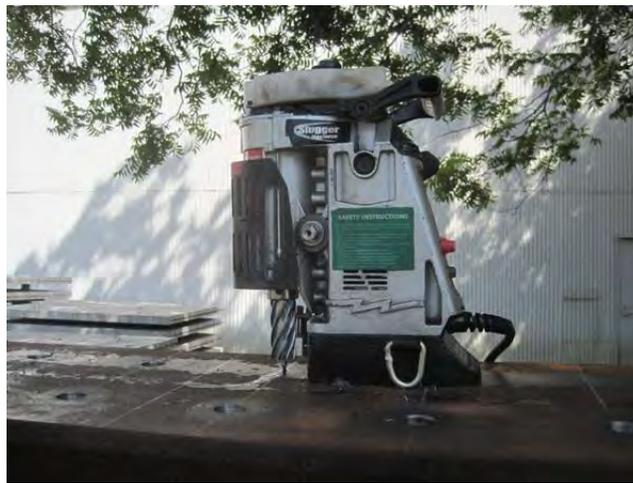
*Figure 7.10: Drilling Holes for Wall Beams*
