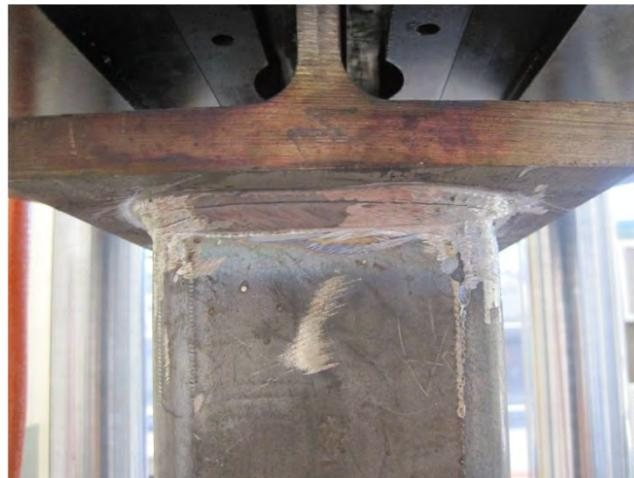
Figure 4.42: Example of Fatigue Crack Forming at Fillet Weld Root in Square HSS Connection
