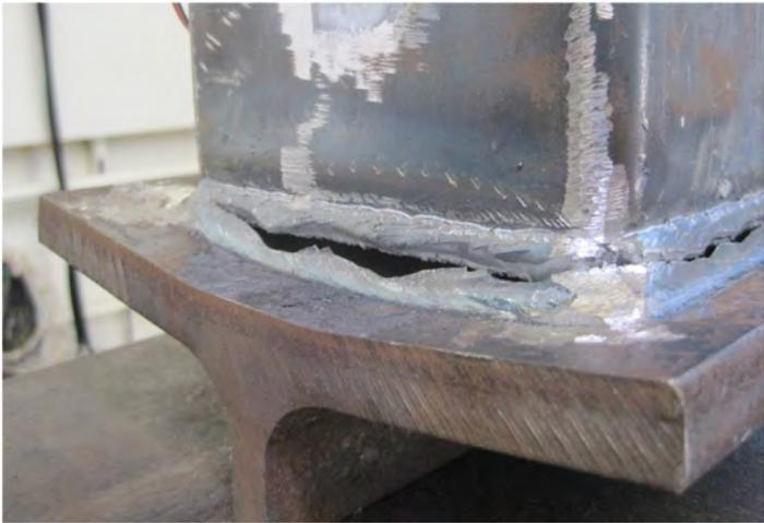
Figure 4.38: Fractured Connection
