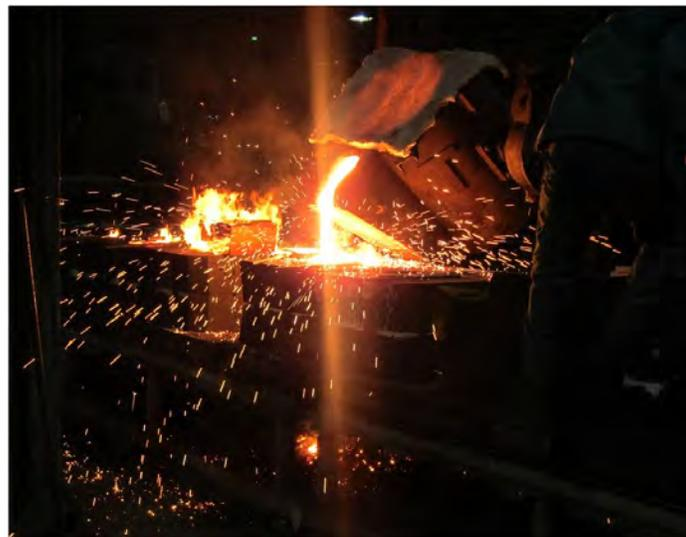
*Figure 3.19: Pouring the Steel into the Sand Molds*
