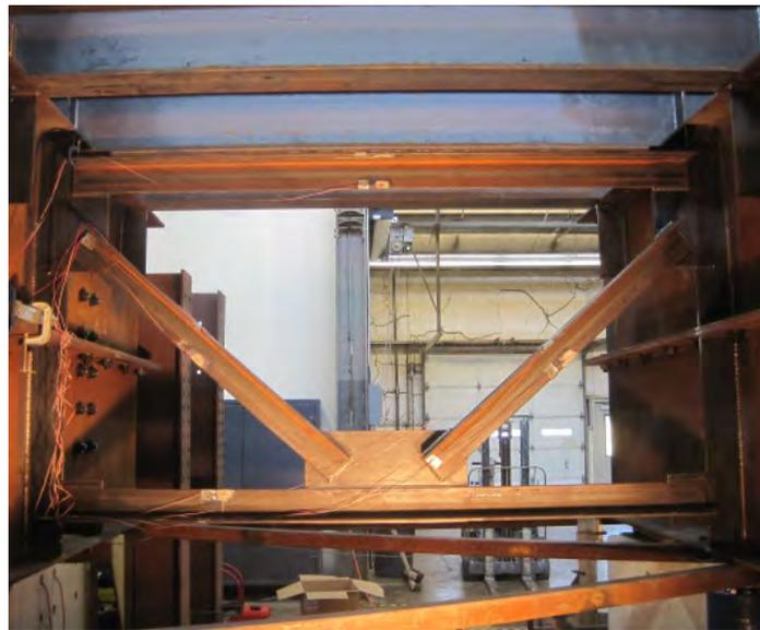
Figure 7.39: Typical K Frame Specimen in Test Setup
