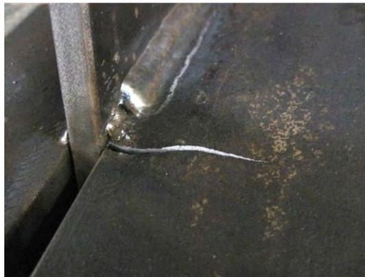
Figure 7.68: Typical Z Frame Double Angle Fatigue Crack (ZF\_DA\_1)
