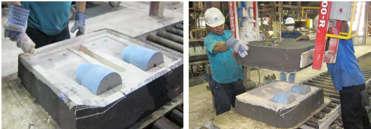
Figure 3.12: (a) Setting the Cores and (b) Closing the Sand Mold
