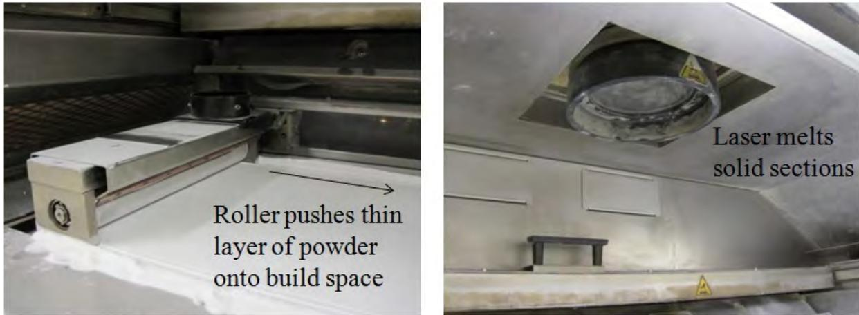
*Figure 3.3: (a) Roller and (b) Laser*
