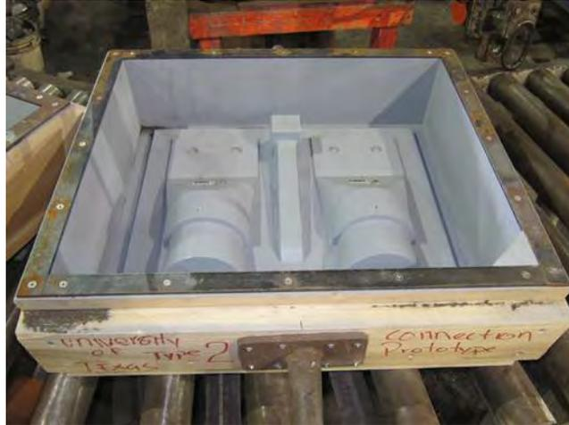
*Figure 3.6: Wooden Pattern for Use in Sand Casting*
