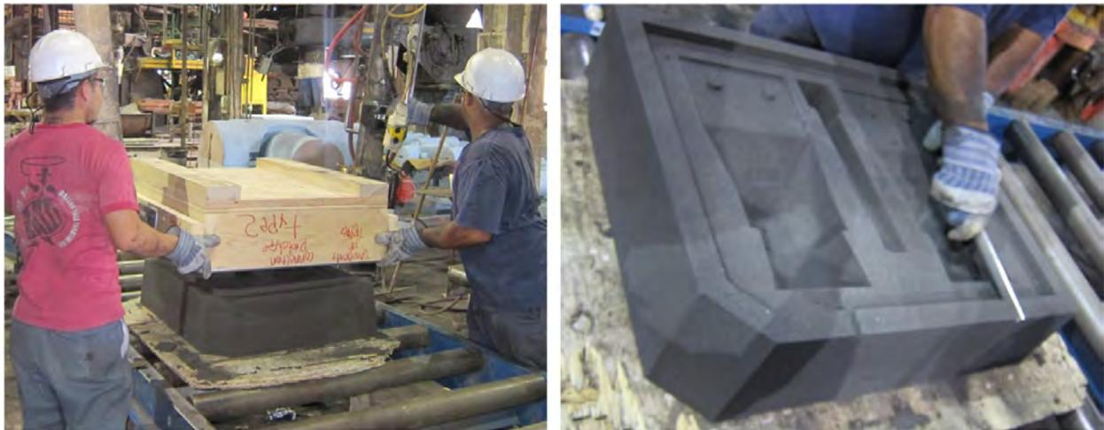
*Figure 3.9: (a) Removing Pattern from Sand Mold and (b) Adding Vents along Parting Line*
