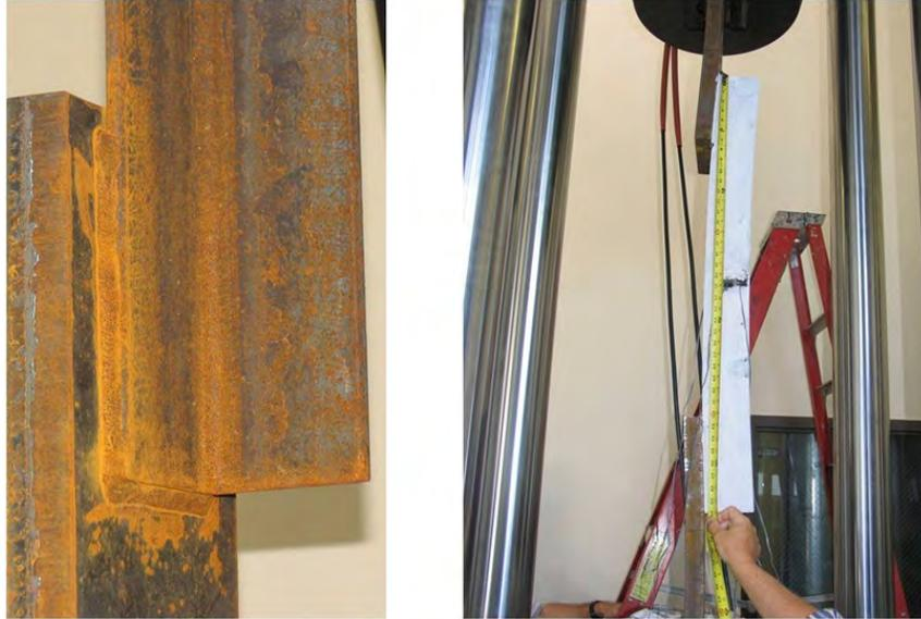
Figure 2.20: (a) Eccentric Connection of Angle and (b) Bending of Angle due to Eccentricity
