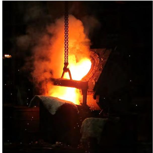
*Figure 3.16: (a) Ladle and (b) Pouring Steel into Ladle*
