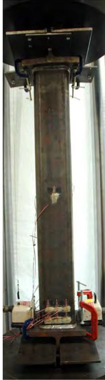
*Figure 4.35: Ultimate Strength Test of Square HSS 5 x 5 x 3/8 and WT 9 x 35.5*
