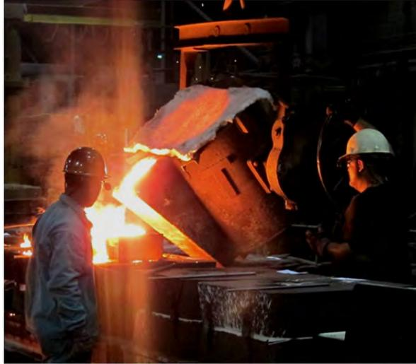
*Figure 3.20: Casting Steel Material Test Blocks*
