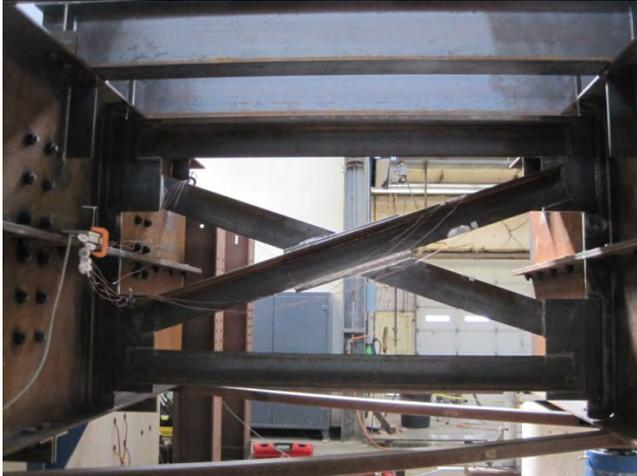
Figure 7.34: Typical Unequal Leg X Frame in Test Setup
