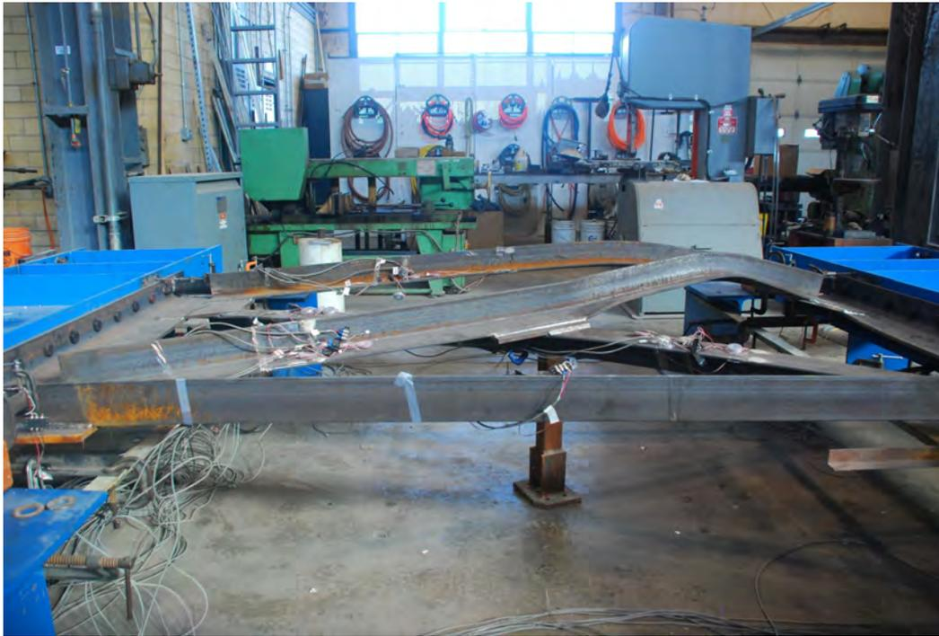
*Figure 5.19: Step 2: Buckling of the top strut*
