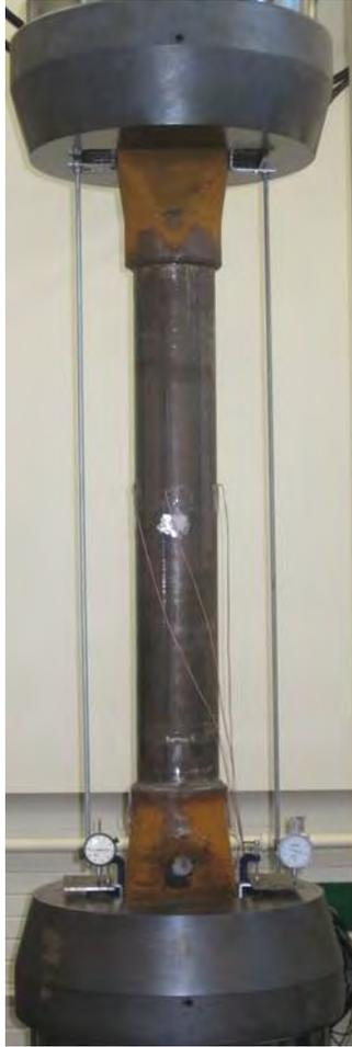
*Figure 4.18: Cast Steel Connection Stiffness Tests with Dial Gages*
