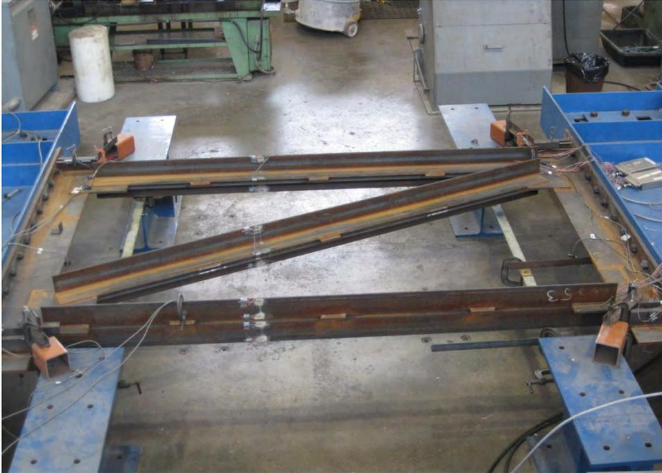
Figure 5.46: Double Angle Z-frame 2 Specimen
