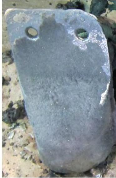
*Figure 3.15: Example of Steel Casting with Incomplete Run-Out*
