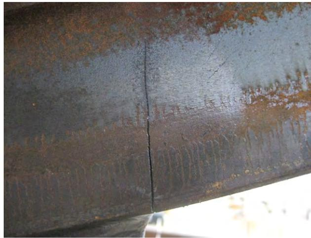
*Figure 7.26: Fatigue Crack at Forward Edge of Fillet Weld into Angle Member (XF\_2)*
