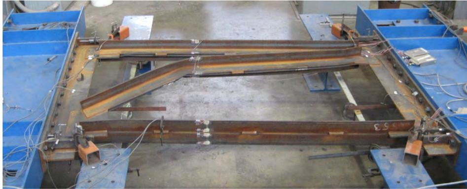
Figure 5.48: Failure of Double Angle Z-frame
