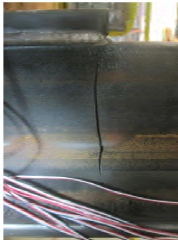
Figure 7.50: Crack in Tension Strut (KF\_1)
