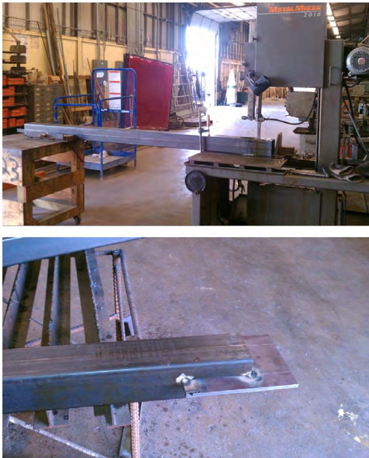
*Figure 5.32: Slotted Tube Connection Fabrication*
