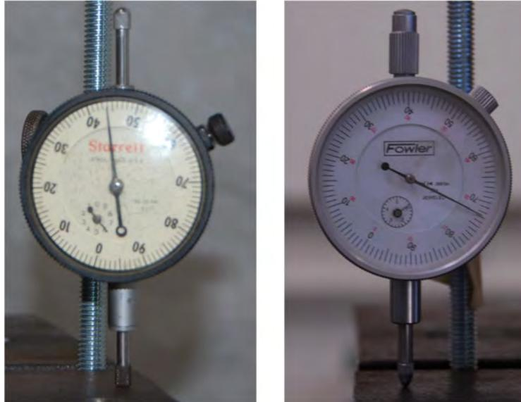
*Figure 4.3: Displacement Dial Gage with (a) 0.001" Accuracy and (b) 0.0001" Accuracy*
