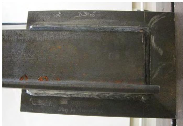
*Figure 4.59: Single Angle Connection*
