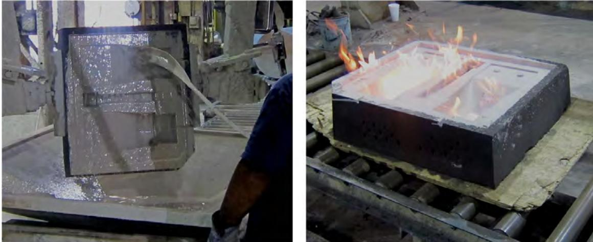
*Figure 3.10: (a) Flow Coating the Sand Mold and (b) Burning the Sand Mold*
