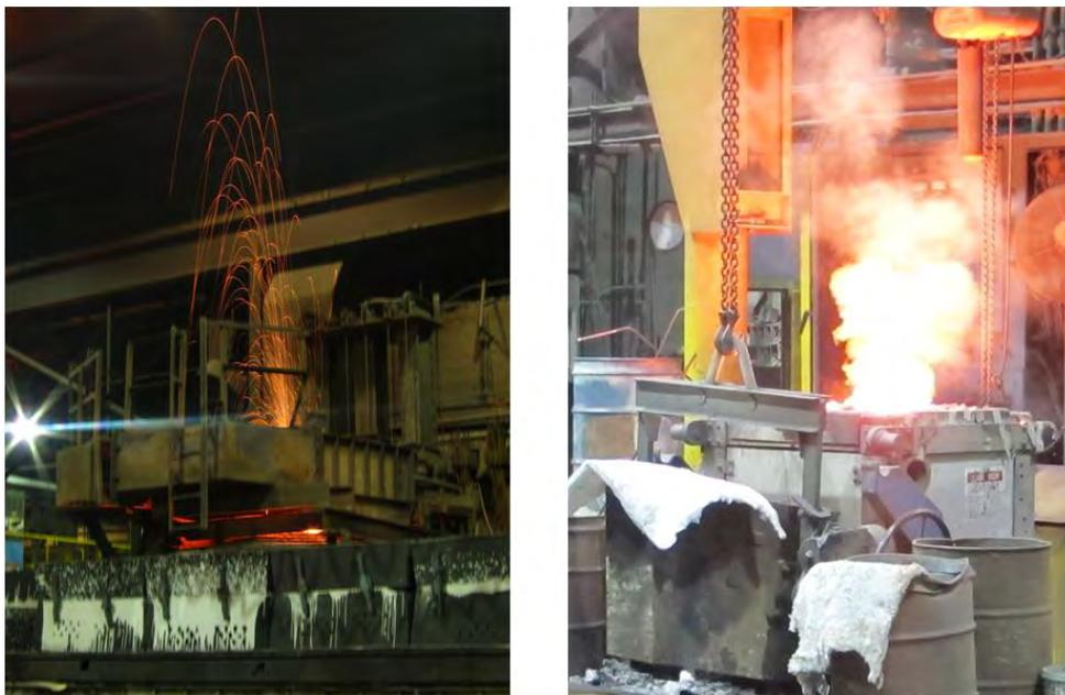
Figure 3.13: (a) Electric Arc Furnace and (b) Small Induction Furnace
