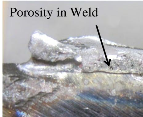
Figure 2.15: Porosity in Cross Section of Fillet Weld (Example)
