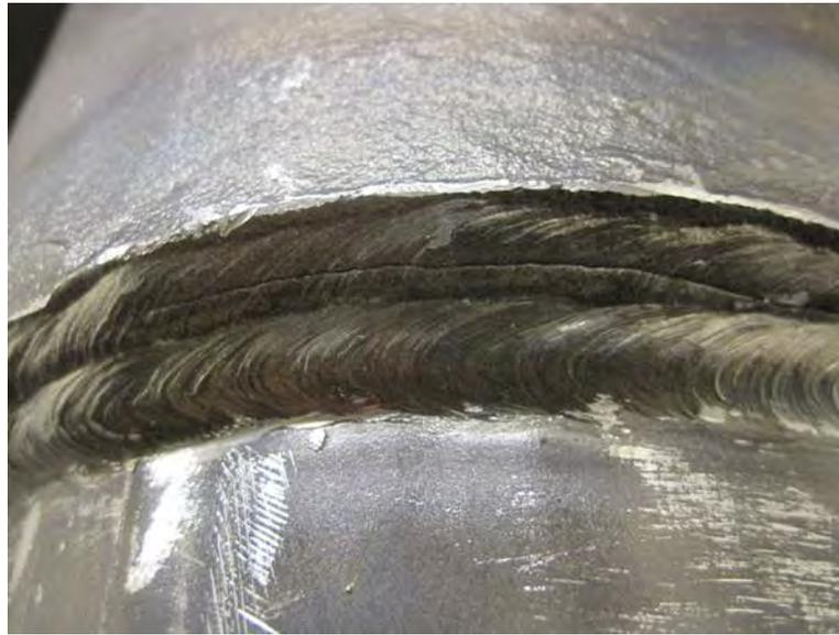
*Figure 4.24: Cast Steel Connection Fatigue Crack*
