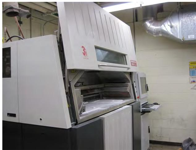
*Figure 3.2: Rapid Prototyping Machine*
