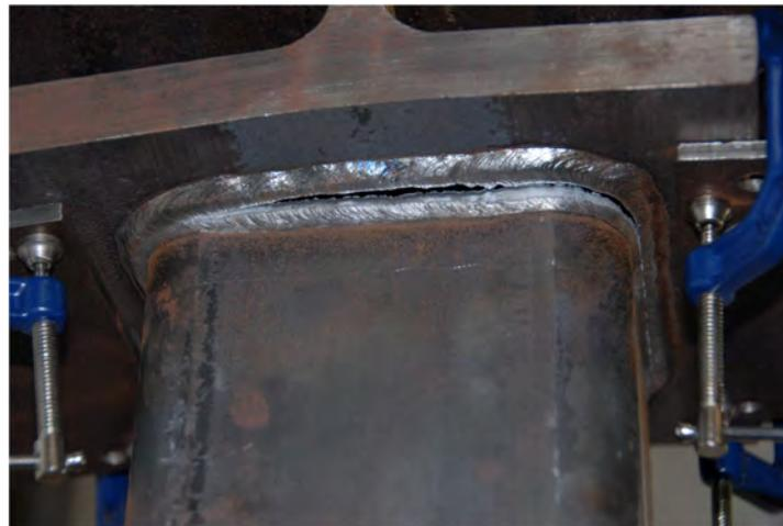
*Figure 4.36: Fracture in Fillet Weld Connection*
