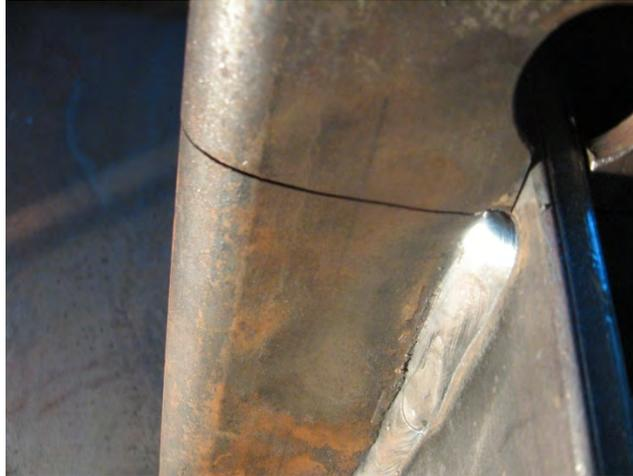
Figure 7.63: Example of Fatigue Crack (ZF\_HSS\_4)
