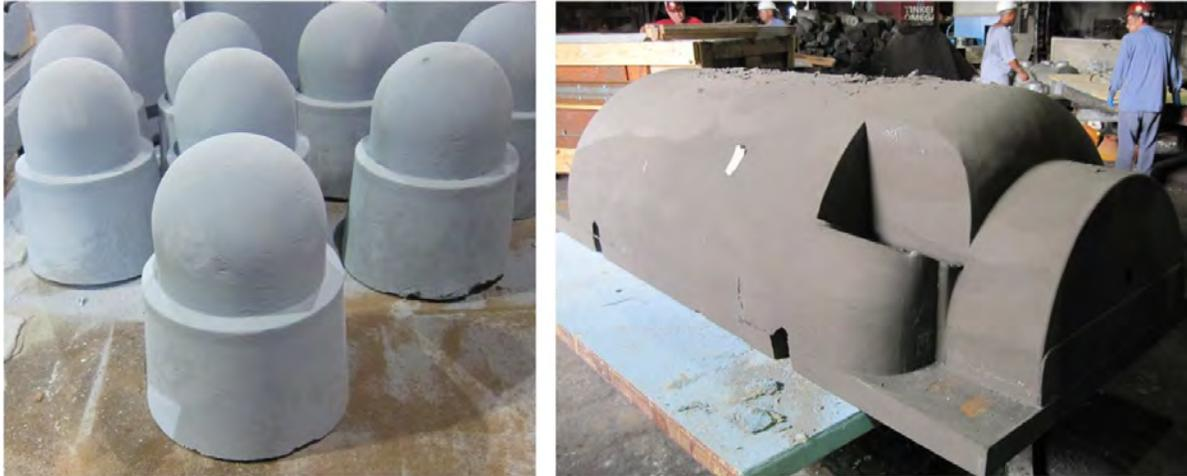
Figure 3.11: (a) Cores used for Cross Frame Connection and (b) Large Sand Core
