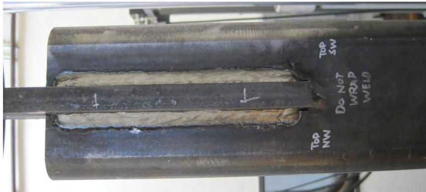
*Figure 4.46: Knife-Plate Connection*
