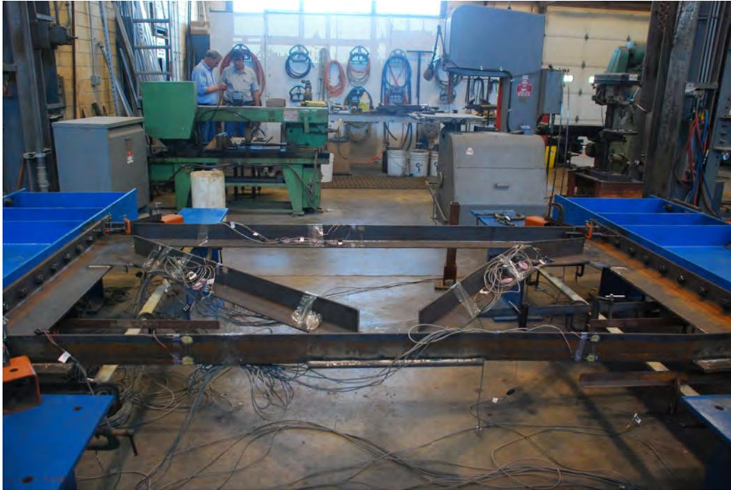
Figure 5.28: Buckling of the Single Angle K-frame
