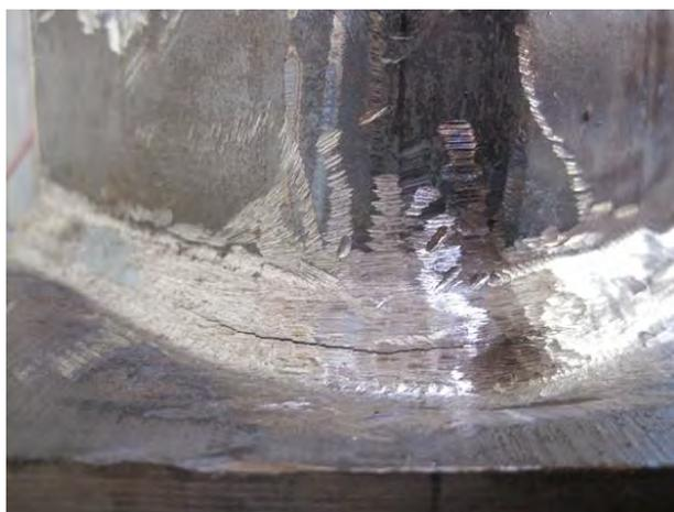
*Figure 4.45: Example of Fatigue Crack Forming at Fillet Weld Root in Diamond HSS Connection*
