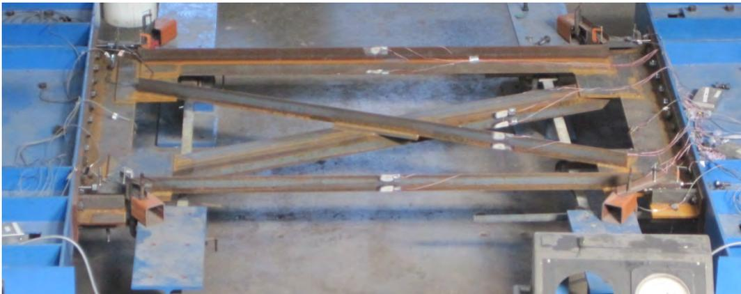
*Figure 5.58: Single Angle Unequal Leg X-frame Specimen*
