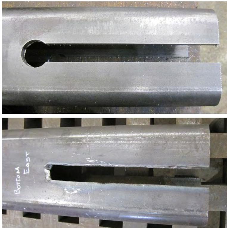
Figure 4.48: Fabrication of Knife-Plate Connection Using (a) Band Saw and (b) Plasma Torch
