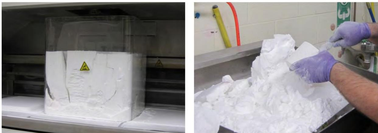
*Figure 3.4: (a) Removal of Powder Block and (b) Cleaning of Prototype*
