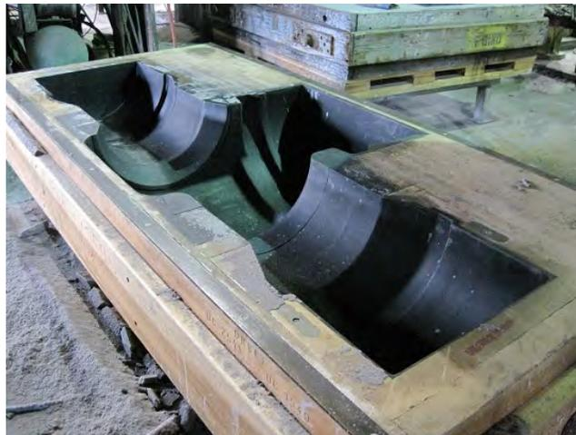
*Figure 3.7: Polyurethane Core Box*
