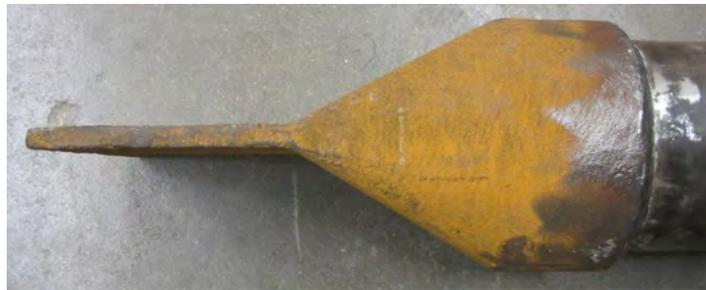
*Figure 4.12: Cast Steel Cross Frame Connection (Side View)*
