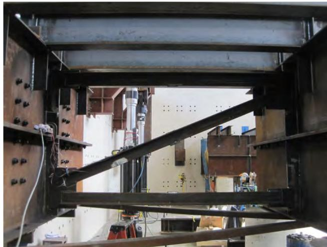
*Figure 7.65: Z Frame Double Angle Specimen in Fatigue Test Setup*
