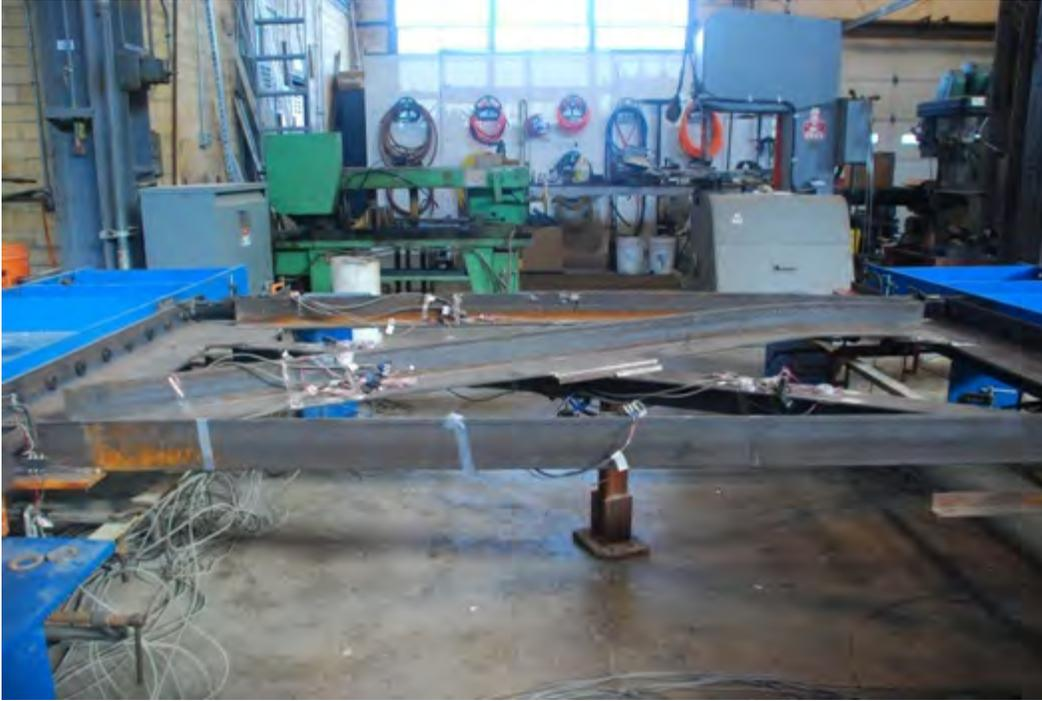
*Figure 5.18: Step 1: Buckling of the compression diagonal*
