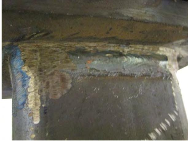
*Figure 4.43: Example of Fatigue Crack Forming at CJP Weld Toe in Square HSS Connection*
