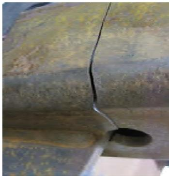
*Figure 7.58: Typical Z Frame HSS Fatigue Crack (ZF\_HSS\_2)*
