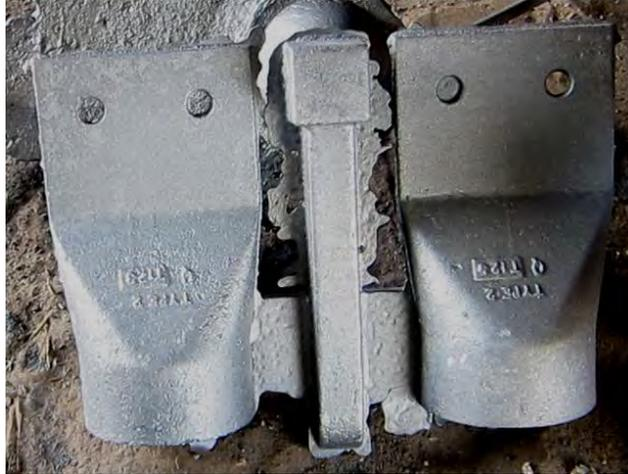
*Figure 3.21: Cross Frame Connections Following Shot-Blast*
