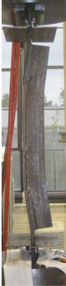
*Figure 4.63: Deformed Single Angle Connection*
