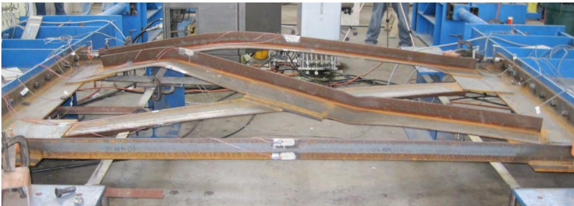
Figure 5.60: Failure of Single Angle Unequal Leg X-frame
