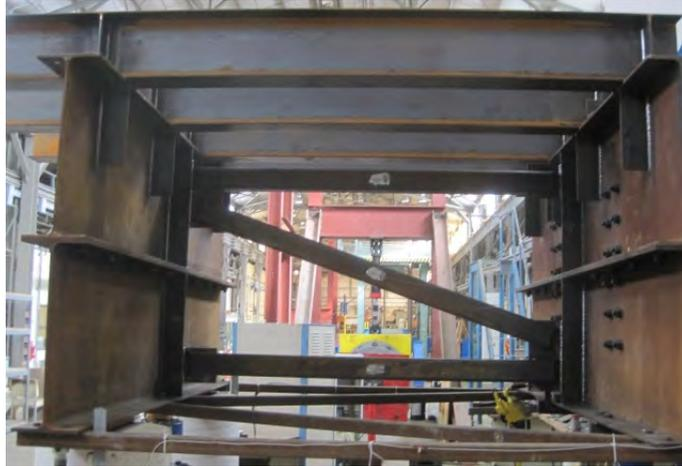
Figure 7.56: Z Frame HSS Specimen in Fatigue Test Setup
