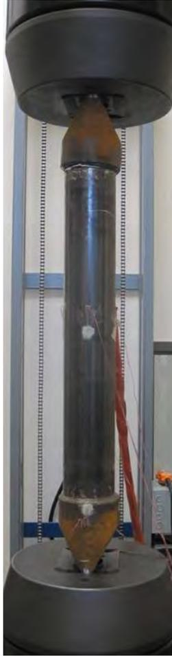
*Figure 4.20: Cast Steel Connection Test in 550 kip MTS Testing Machine*
