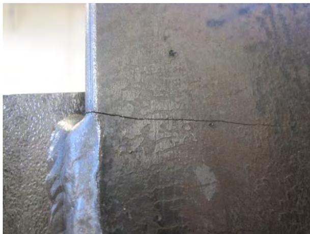
Figure 4.57: Double Angle Connection Fatigue Crack (Angle Member)
