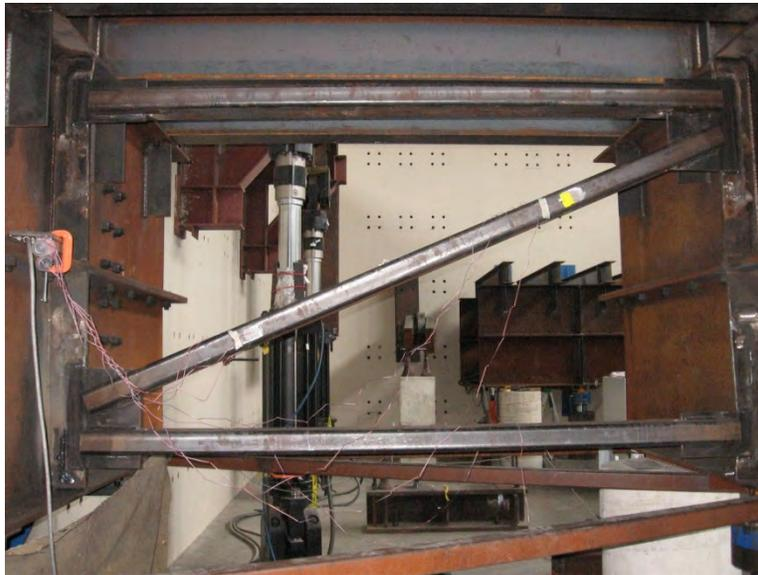
*Figure 7.62: Rectangular HSS Z Frame in Test Setup*
