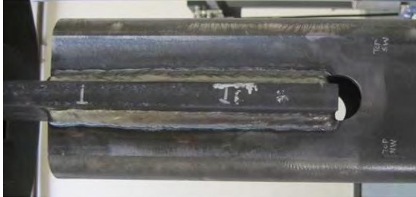
Figure 4.47: Knife-Plate Connection with Drilled Stress Relief Hole
