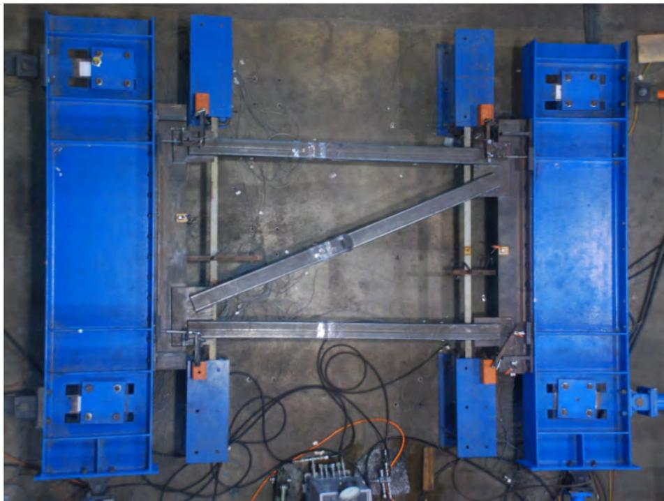
Figure 5.34: Square Tube Z-frame Specimen
