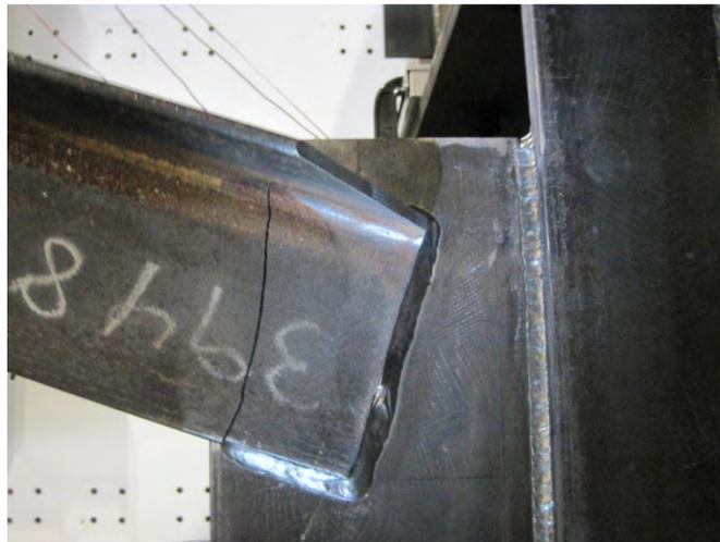
*Figure 7.36: Typical Unequal Leg X Frame Fatigue Crack (XF\_UL\_3)*
