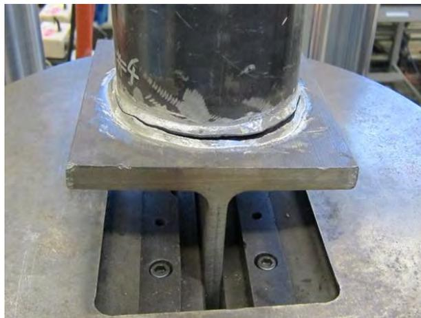
*Figure 4.44: Example of Fatigue Crack Forming at Fillet Weld Root in Round HSS Connection*
