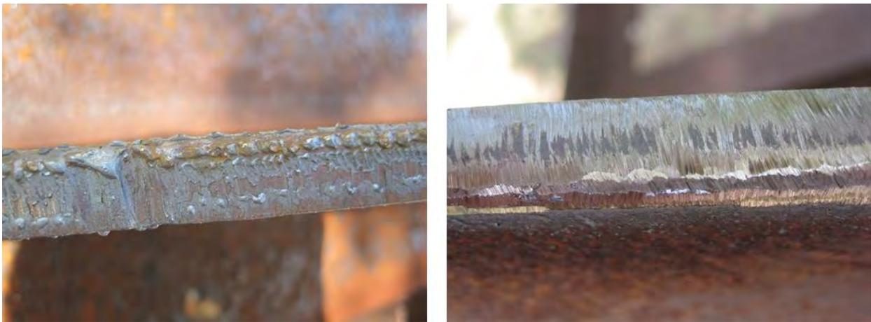
*Figure 7.13: Surface Condition (a) After Flame Cut and (b) After Subsequent Grinding*
