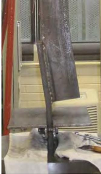
*Figure 7.2: Single Angle Strength Test Bending*
