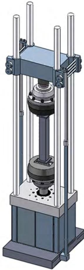
*Figure 4.1: 220 kip MTS Testing Machine with Specimen*
