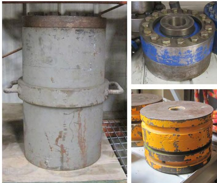
Figure 7.9: (a) Hydraulic Actuator, (b) Load Cell, and (c) Spherical Head
