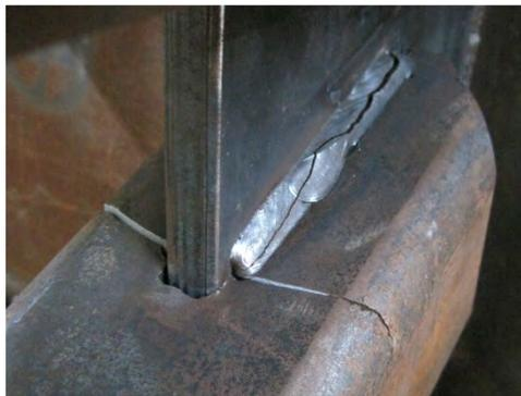
*Figure 7.59: Typical Z Frame HSS Fatigue Crack (ZF\_HSS\_3)*
