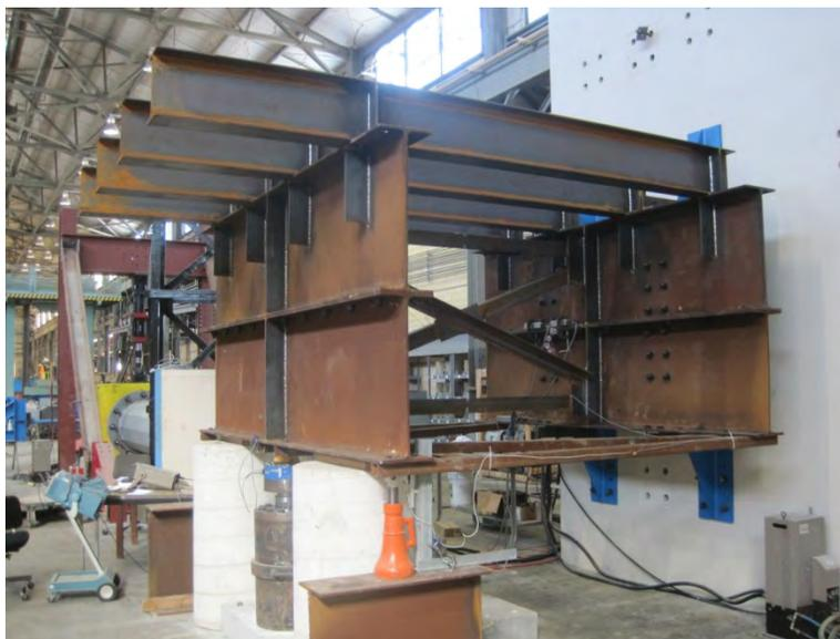
*Figure 7.4: Completed Cross Frame Fatigue Test Setup*
