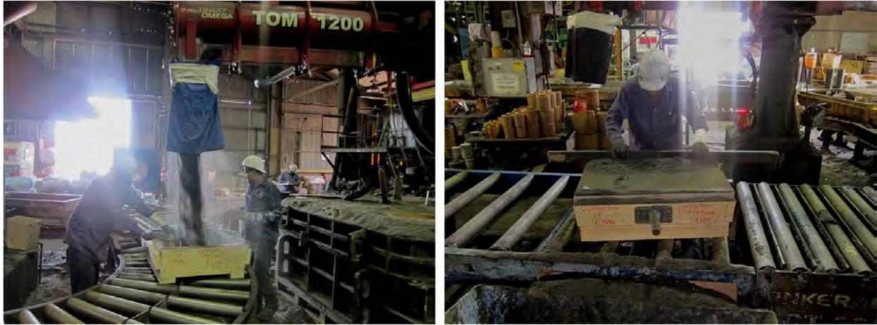
*Figure 3.8: (a) Pouring Sand Slurry into Pattern Box and (b) Compacting Sand Mold*
