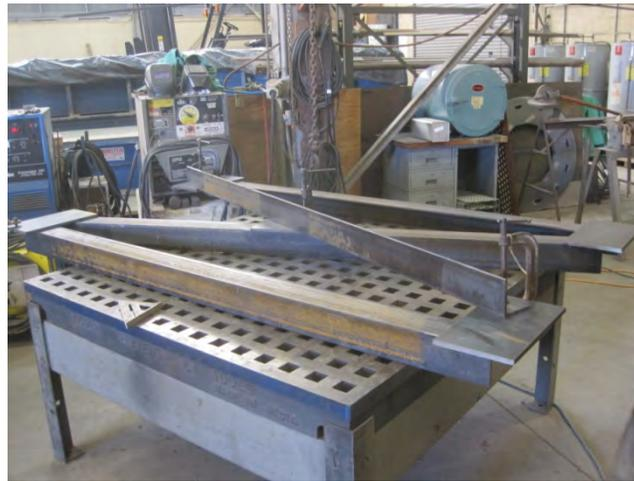
*Figure 7.14: Cross Frame Layout during Fabrication*
