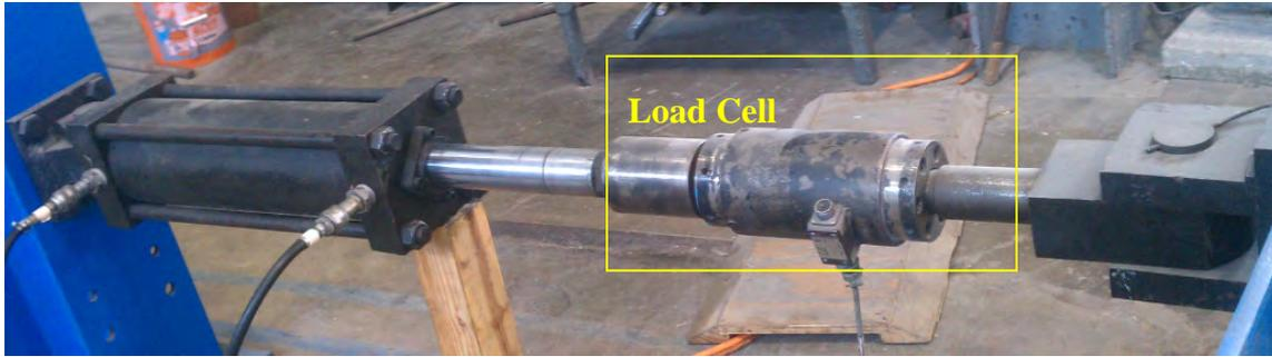
*Figure 5.4: Load Cell for Actuator*
