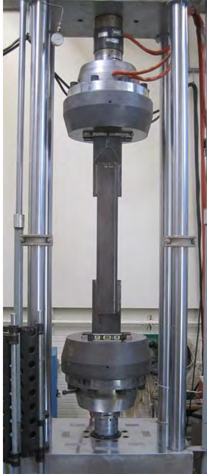
*Figure 4.7: Basic Fatigue Setup*
