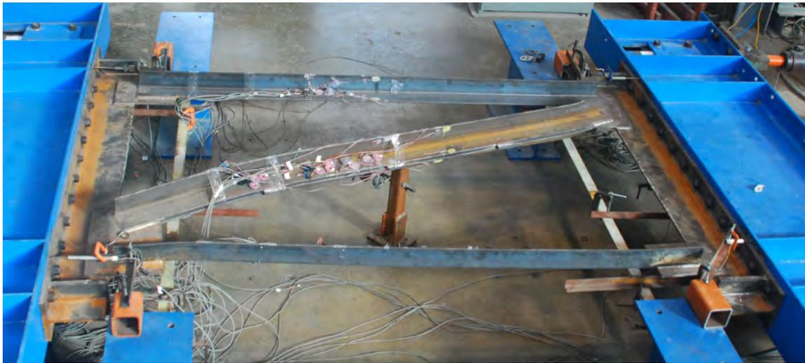
*Figure 5.42: Failure of Double Angle Z-frame*
