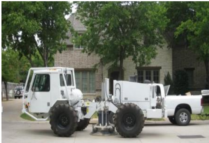
Figure 2.2: Vibe Buggy Operating in the Barnett Shale
