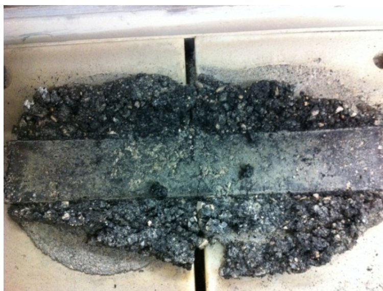
Figure 8.7 HWT of Marble Falls CAM with fine component replaced with SAC-A
