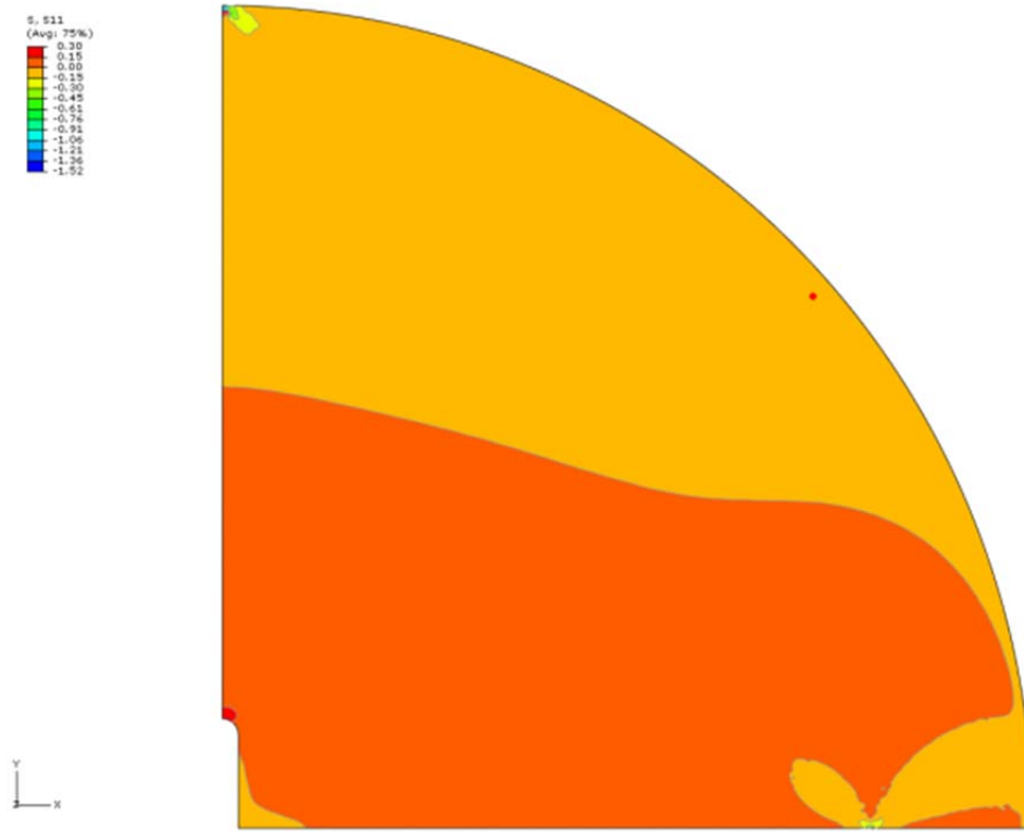
Figure 10.2 Tensile stress distribution in notched SCB specimen
