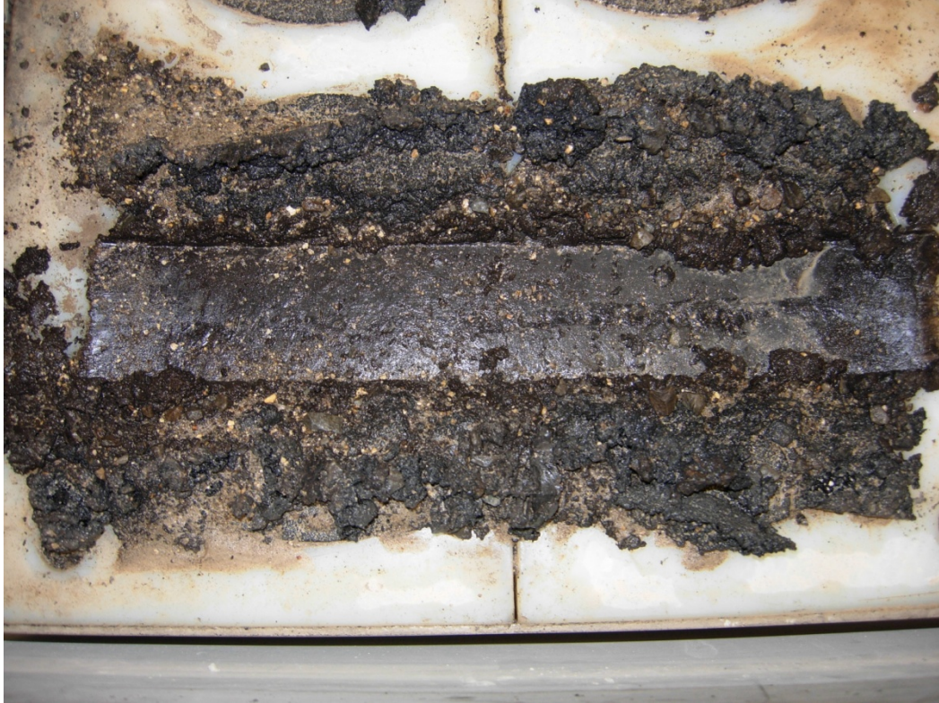
Figure 6.2 HWT testing of RTI mix
