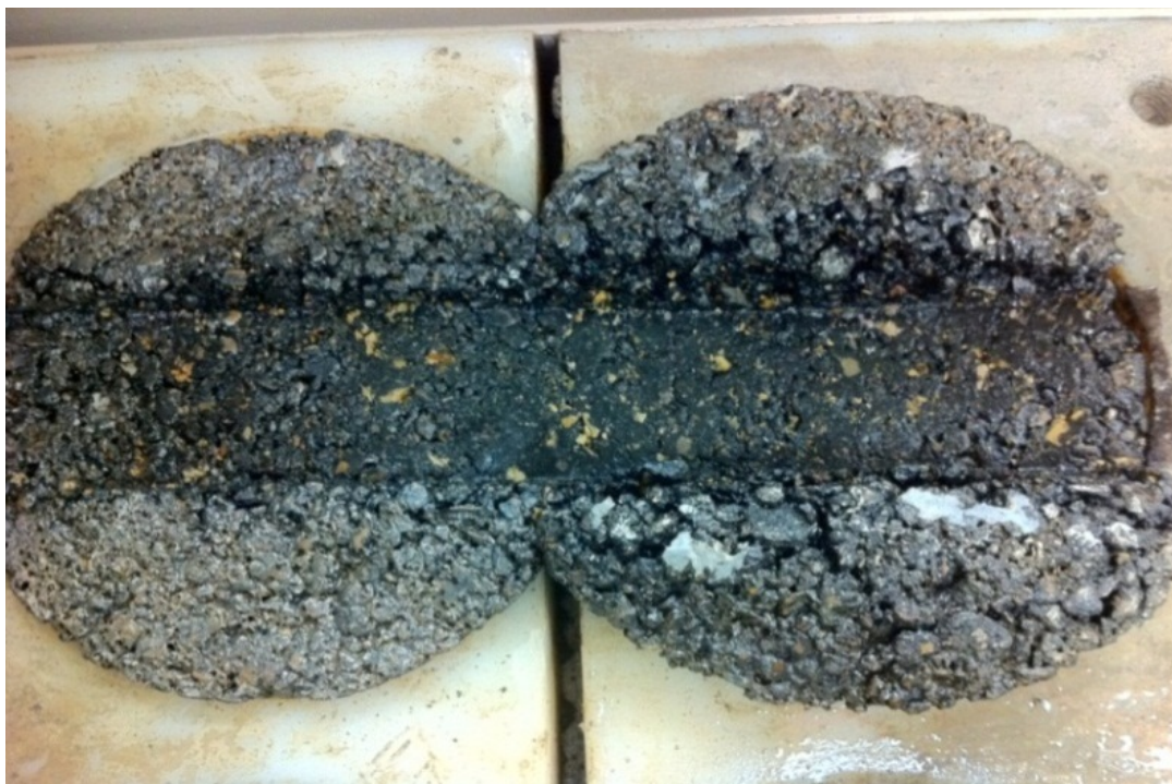
Figure 8.5 HWT specimen failure for CMHB Fordyce mix
