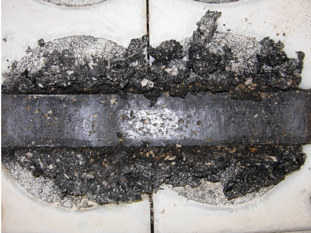
Figure 6.4 HWT testing of Spicewood mix
