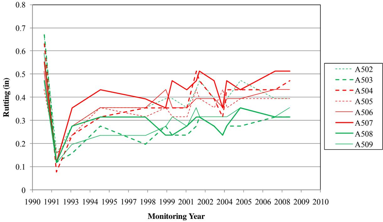
Figure 4.2: Rutting of Texas SPS-5 pavement structures
