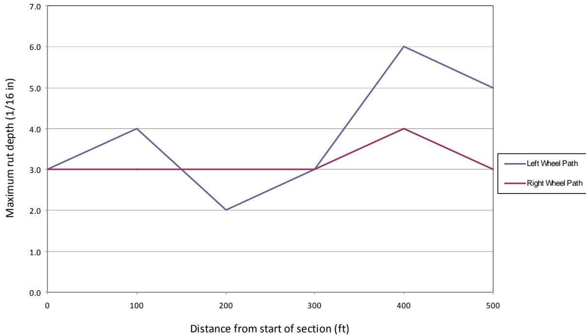
Figure 8.2: Rutting along CAM section on LP 20, Laredo (LACAMIW)
