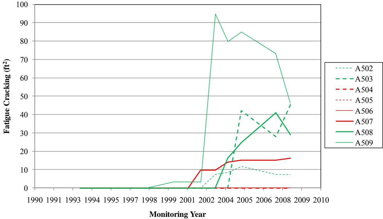
Figure 4.3: Fatigue cracking of Texas SPS-5 pavement structures
