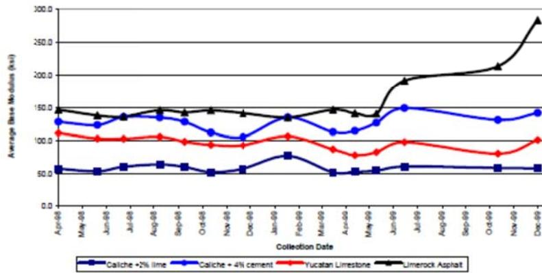
*Figure 2.3: Base layer moduli on US 77 from 1998 to 1999*
