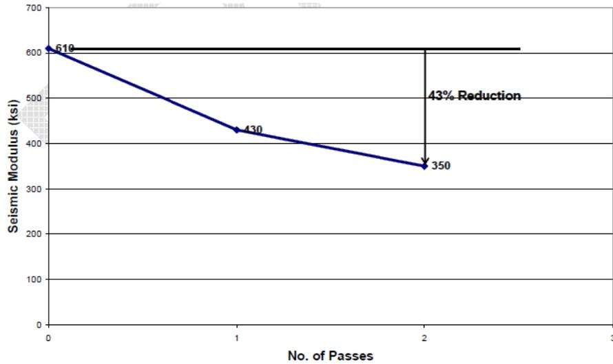
Figure 2.11: Reduction of base modulus with micro-cracking
