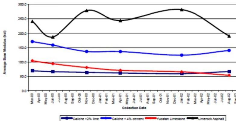
*Figure 2.4: Base layer moduli on US 77 from 2000 to 2002*
