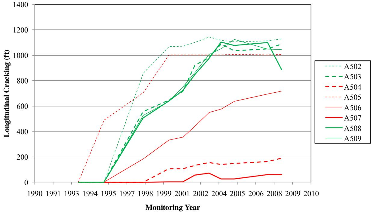
Figure 4.4: Longitudinal cracking of Texas SPS-5 pavement structures
