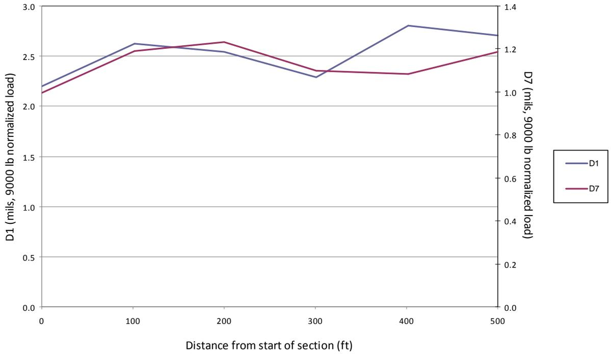
Figure 7.10: Deflections along perpetual pavement structure, R1, IH 35 (LAPERPIN)
