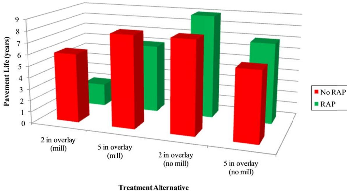
Figure 4.9: Estimated pavement life of analysis pavement sections
