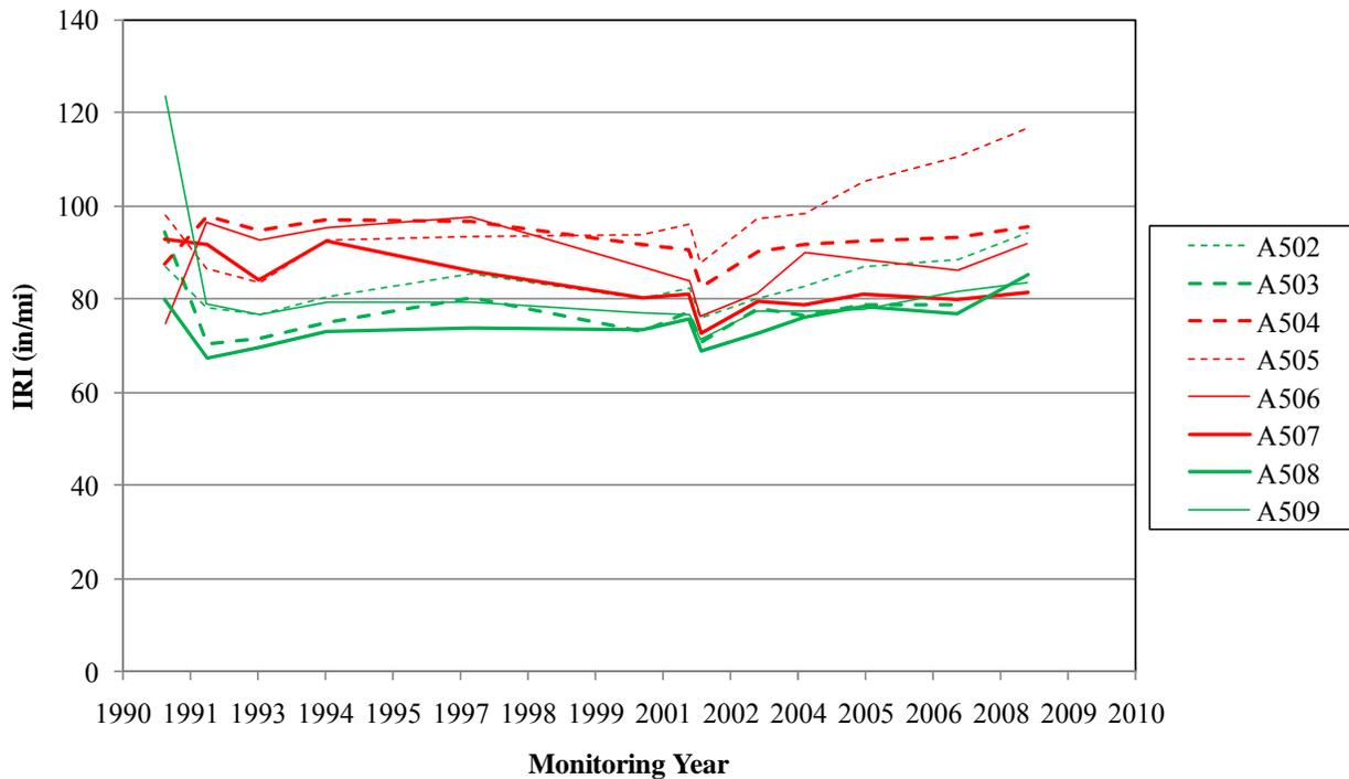
Figure 4.6: Roughness of Texas SPS-5 pavement structures
