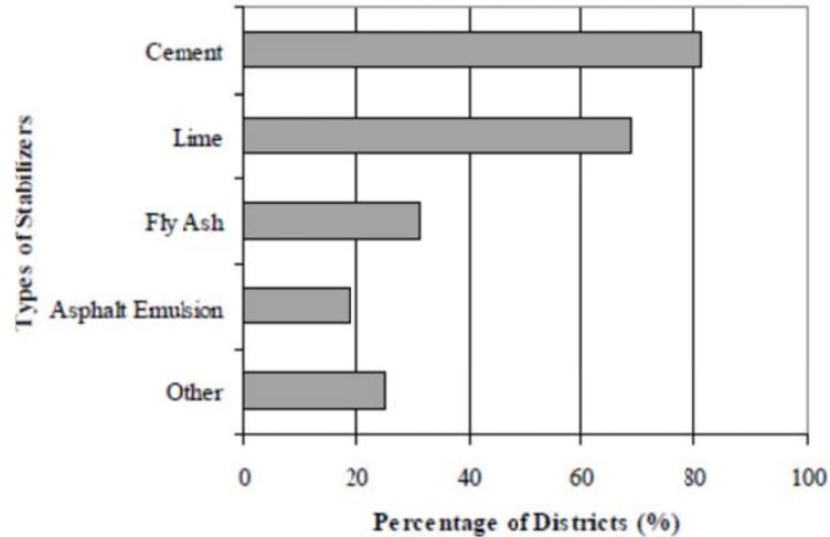
Figure 2.7: Stabilizers used by TxDOT
