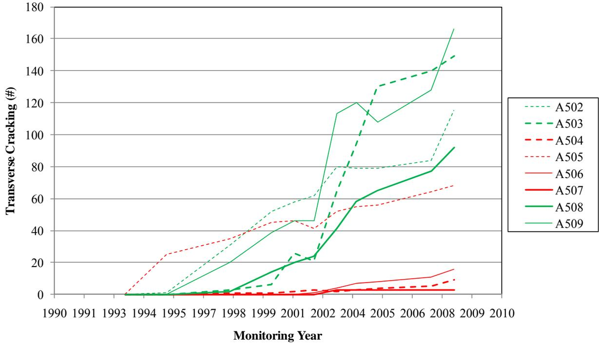
Figure 4.5: Transverse cracking of Texas SPS-5 pavement structures
