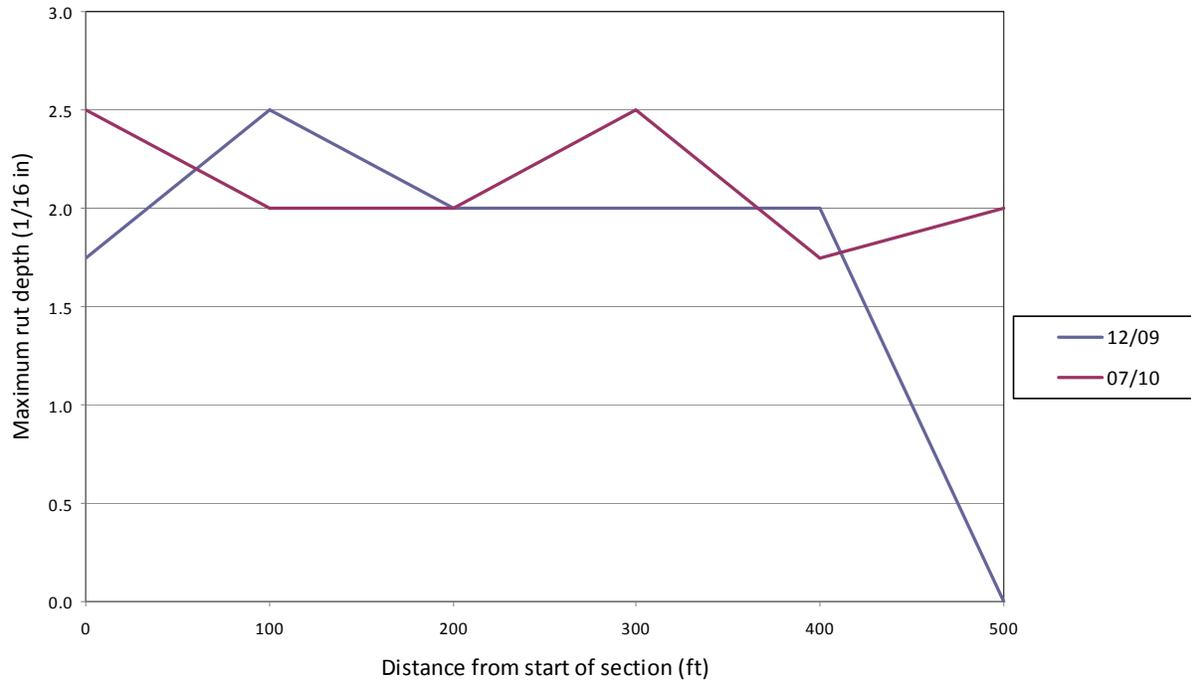
Figure 7.4: Rutting along perpetual pavement structure, RI, Fort Worth (FWPERPIE)
