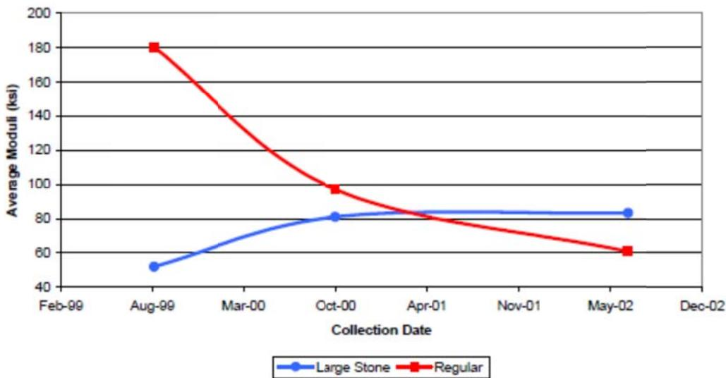
Figure 2.5: Base layer moduli on FM 1810 from 1999 to 2002.
