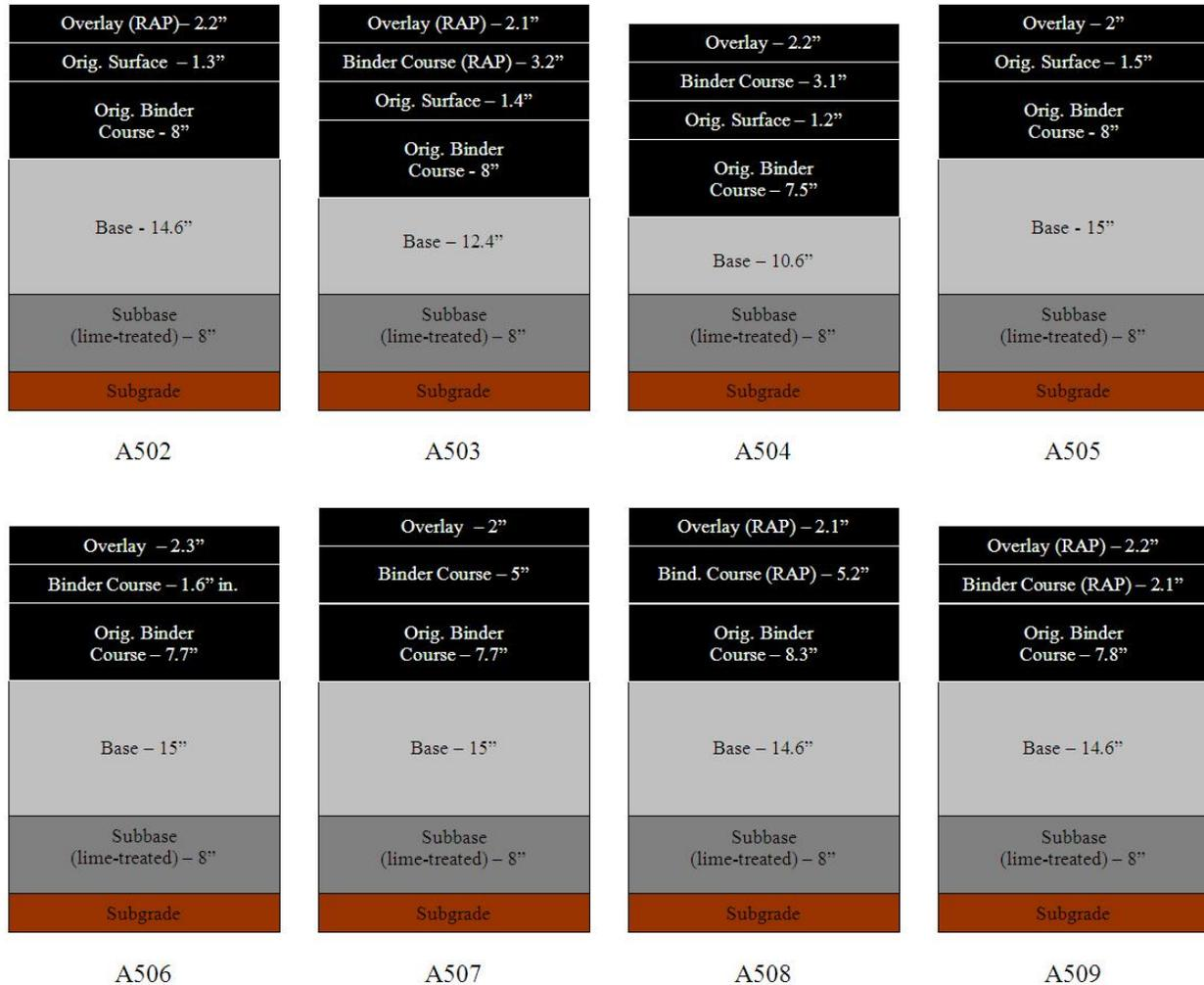
Figure 4.1: Texas SPS-5 pavement structures
