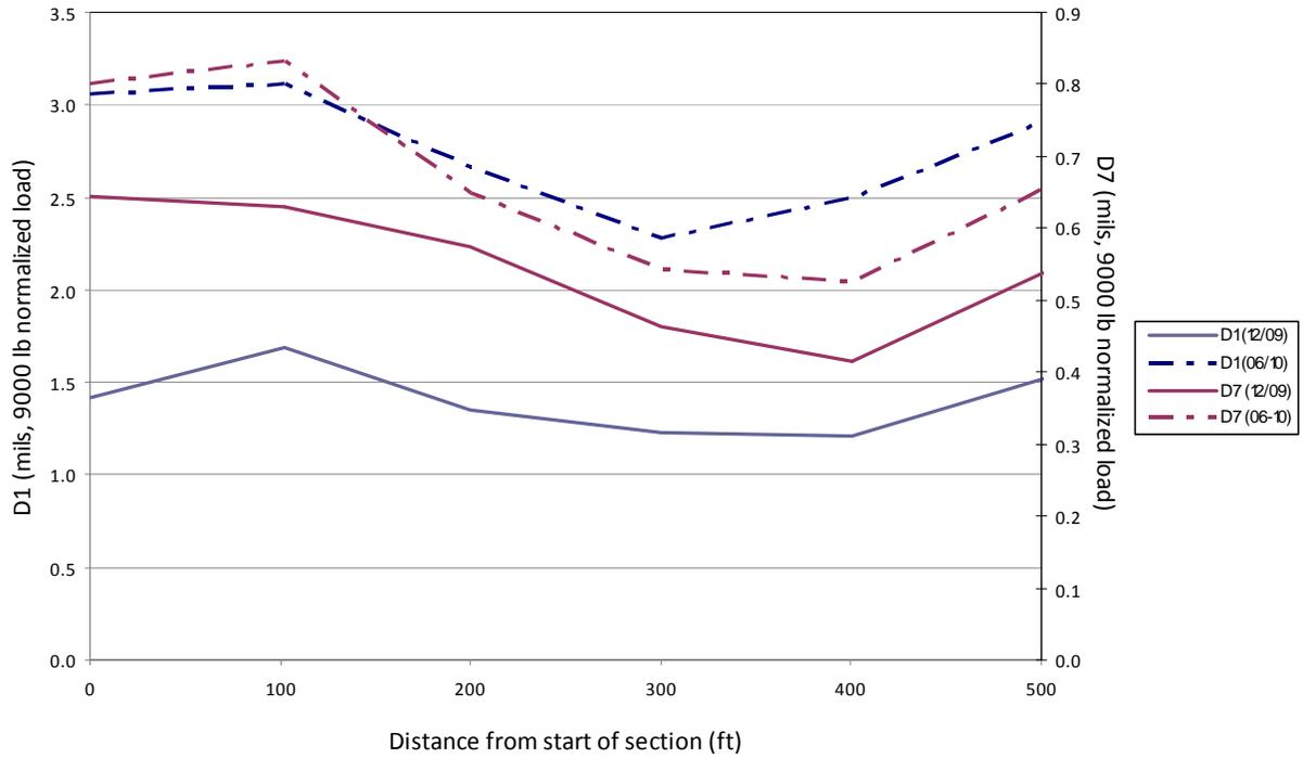
Figure 7.6: Deflections along perpetual pavement structure, R1, IH 35 (SAPERPIN)
