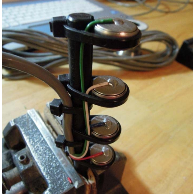
Figure 7.41: Sensor stick prior to epoxy coating.
