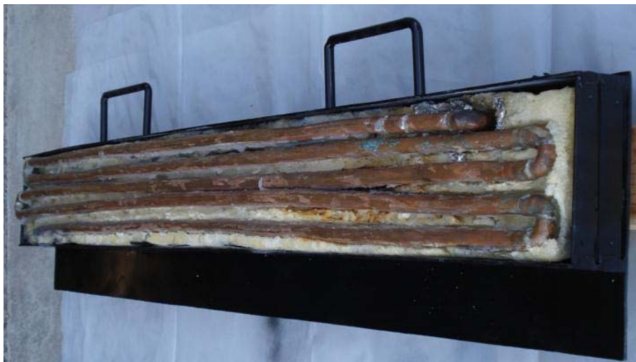
Figure C.9: Side walls prior to application of flashing.
