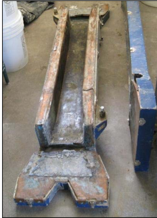
Figure 3.10: Old formwork for rigid cracking frame.
