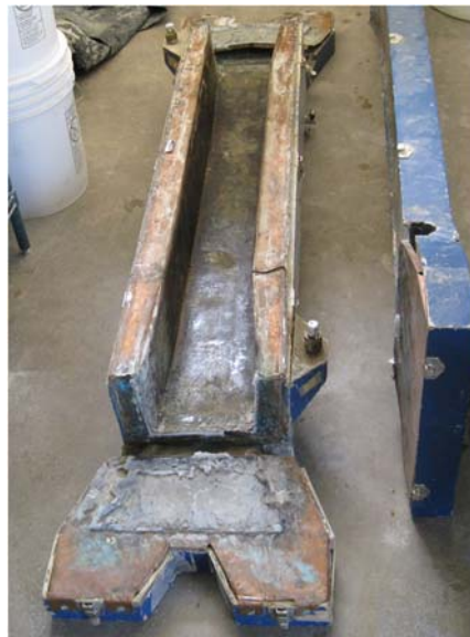
Figure C.3: Deterioration of existing formwork.
