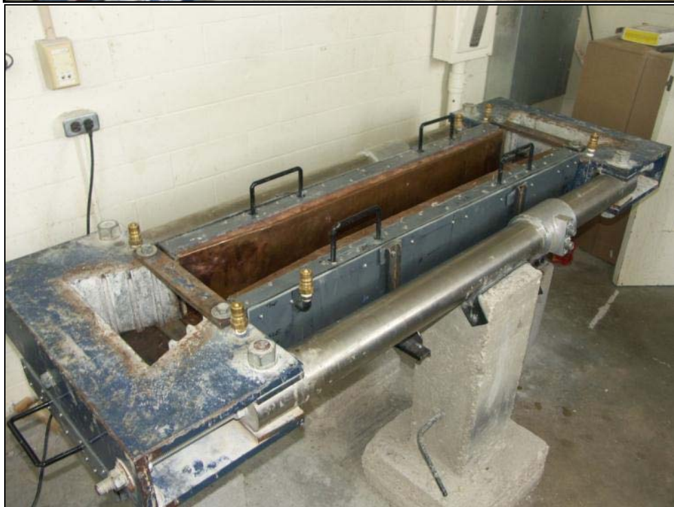
Figure 3.11: Rigid cracking frame with new formwork.
