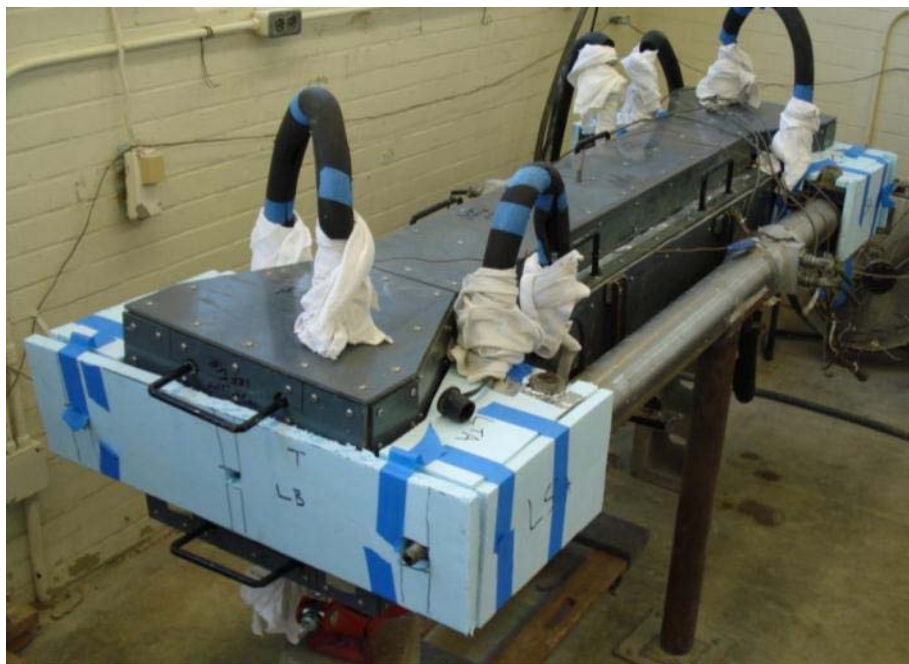
Figure 3.9: Rigid cracking frame with added insulation.
