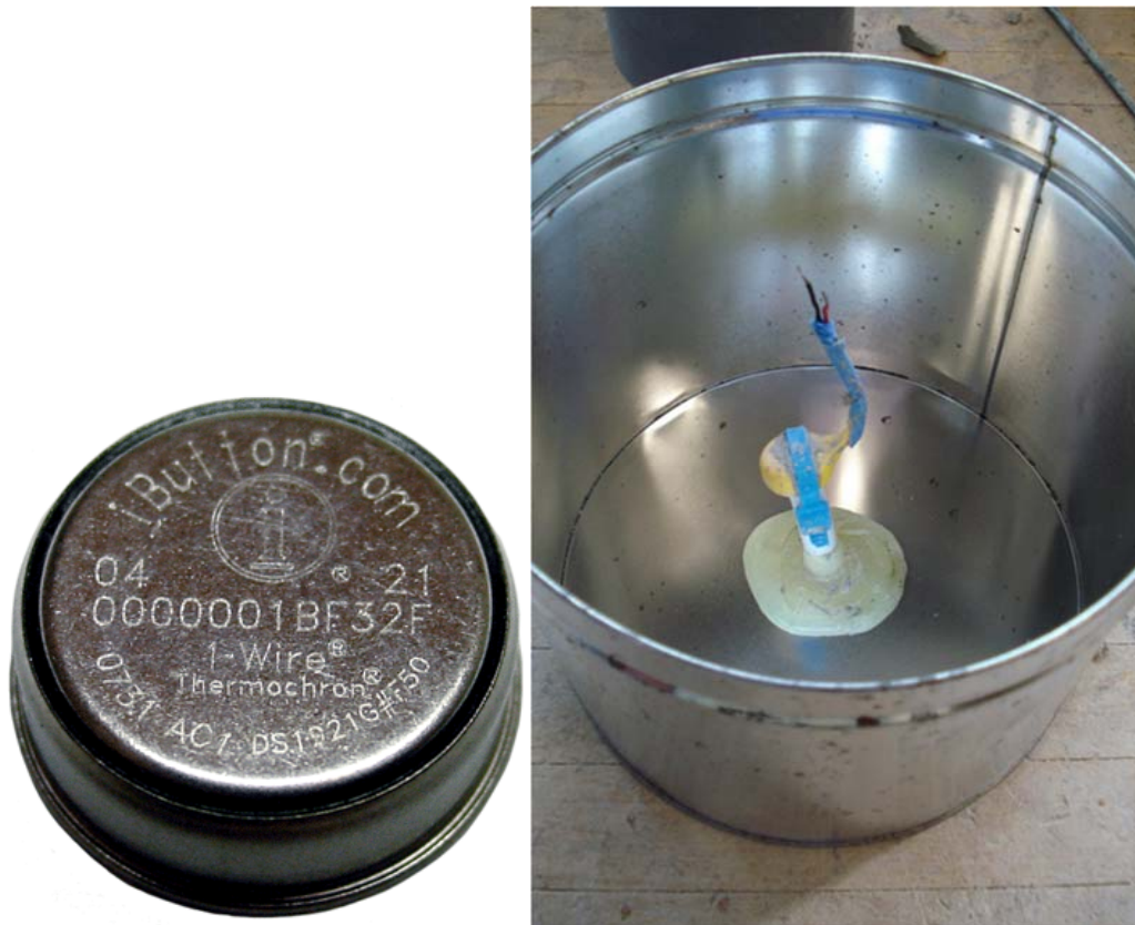
Figure 3.14: Temperature collection inside time-of-set can.
