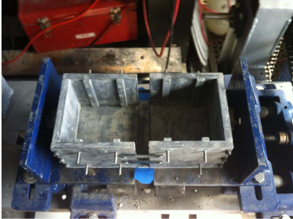
Figure 6.2: Direct tensile mold with PVC dowels.
