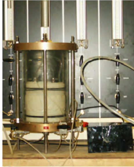
Figure 3.10: Flexible-wall hydraulic conductivity test
