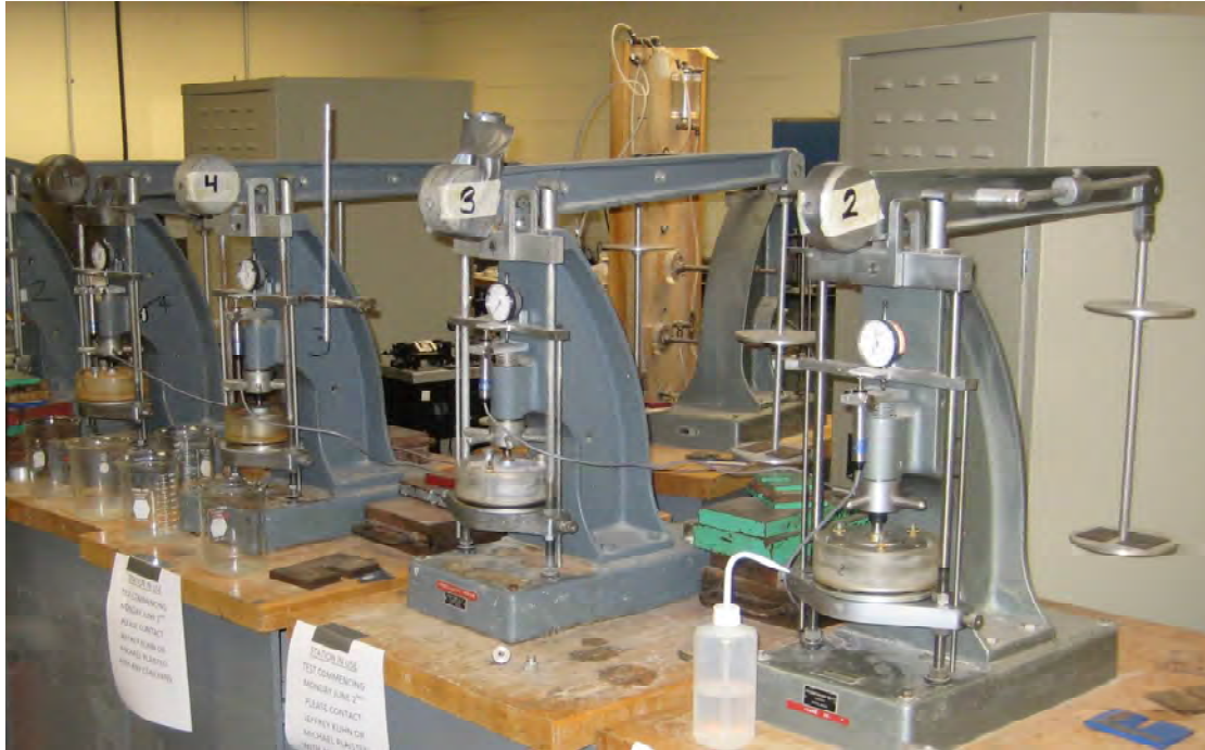
Figure 3.4: Free-swell testing setup
