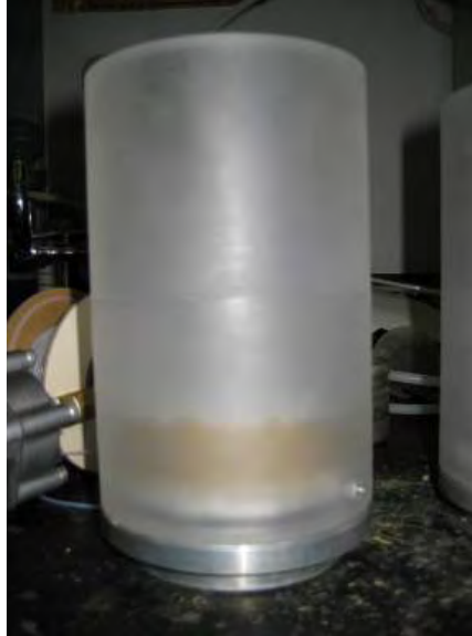
Figure 5.3: Acrylic permeameter cup for the large centrifuge
