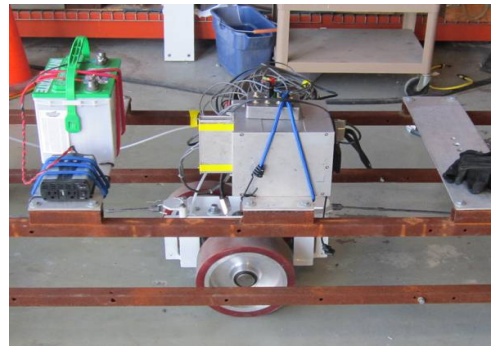
(b) SB: 9-in. Diameter Wheels; Two, 2-in. and One, 4-in. Wide Treads
