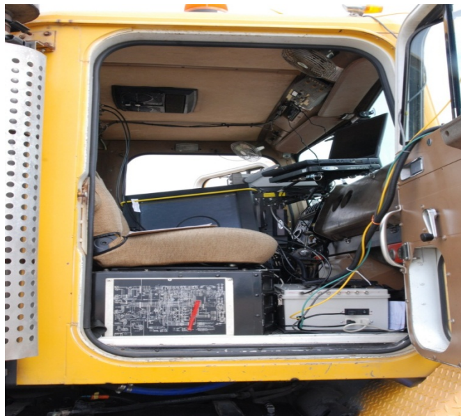
Figure 4.2: Mounted Data Acquisition computer and control box in the classic RDD
