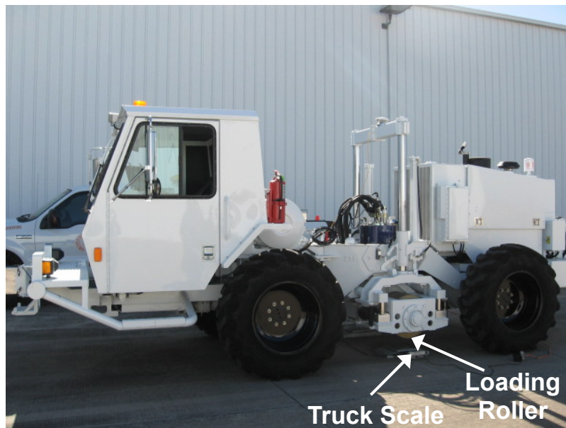
Figure 2.7: TPAD Loading Rollers Sitting on the Truck Scales during Static-Load Acceptance Testing at TxDOT FSF, ABI on December 09, 2010
