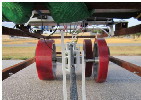
(d) SD: 12-in. Diameter Wheels; Two, 2-in. and One, 4-in. Wide Treads
