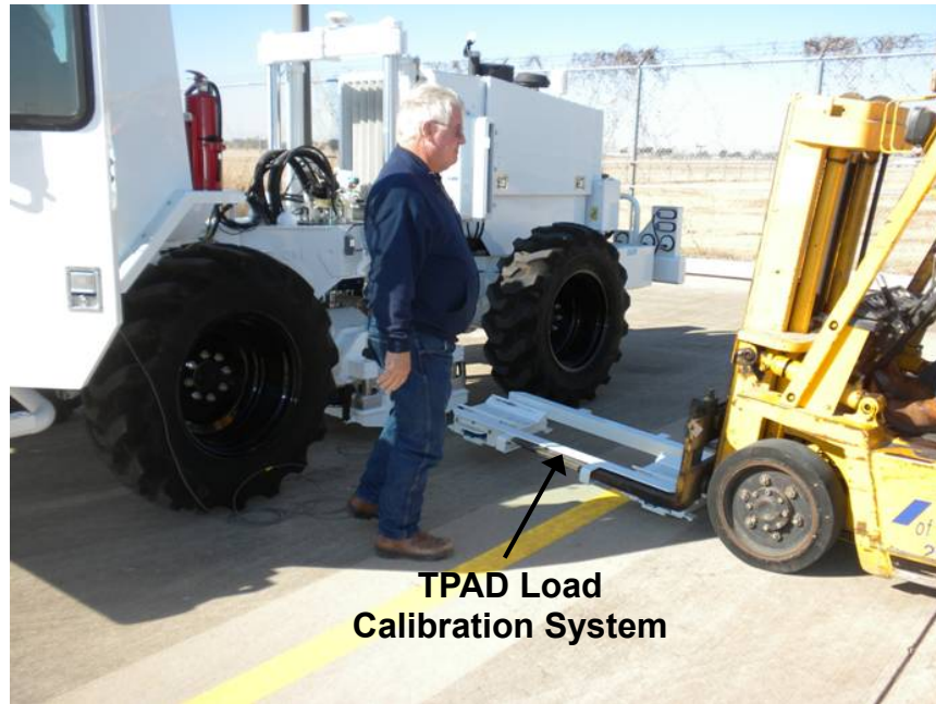
(a) Installation of Load Calibration System under the TPAD
