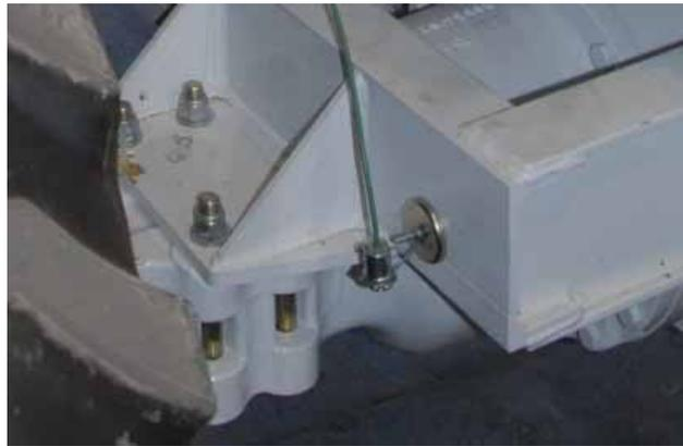
*Figure A.20: Infrared Sensor for Getting the Surface Temperature*
