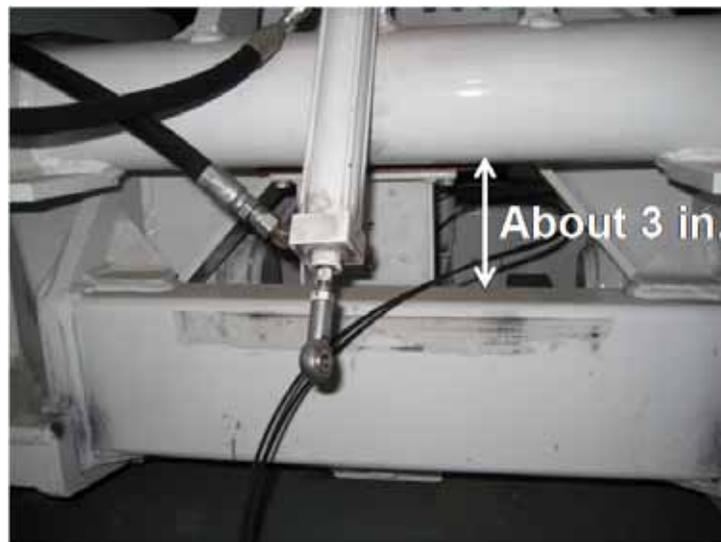
*Figure 2.7: Vertical Space Constraints under the TPAD for Towing Frame*
