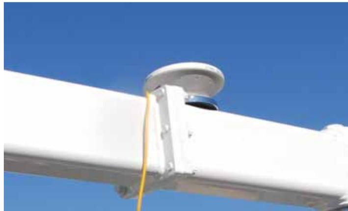
*Figure A.21: GPS Antenna Mounted at the Top of the Loading Frame*
