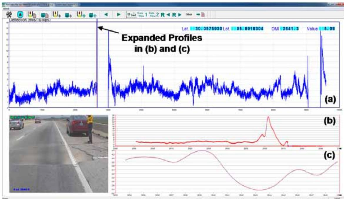
Figure 5.1: Typical TPAD Data from Full-Depth Asphalt Section of US 290
