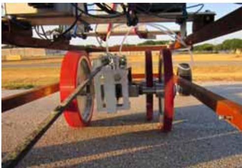
(c) SC: 12.5-in. Diameter Wheels: Two, 1-in. and One, 2-in. Wide Treads
