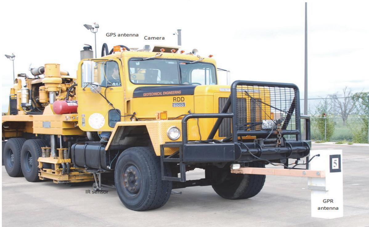
*Figure 5.8: Mounting the GPS, GPR and Digital Video System on the Original TPAD Unit*
