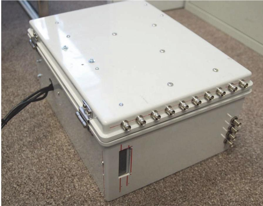
*Figure 5.6: TPAD Data Acquisition Instrument Box (When Closed)*
