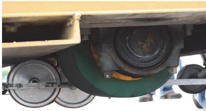
*Figure 5.9: Loading Roller and Rolling Sensors Arrangement Used in Testing*
