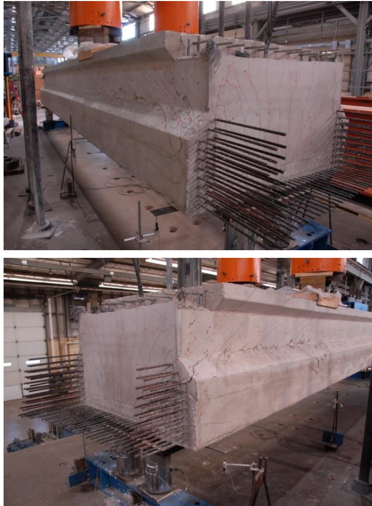
Figure 6-31: Symmetric failure of both webs in 5B40-4-Q
