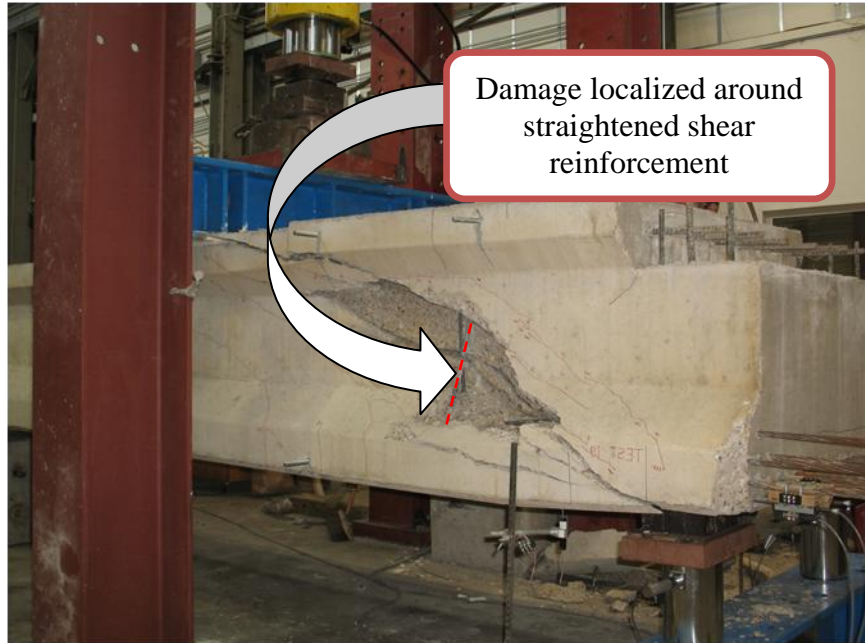
Figure 4-21: Failure of Square end of BB-09 (SCC).
