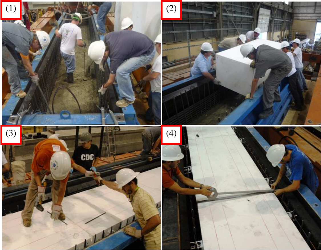
Figure 3-17: Step-by-step Box Beam fabrication process
