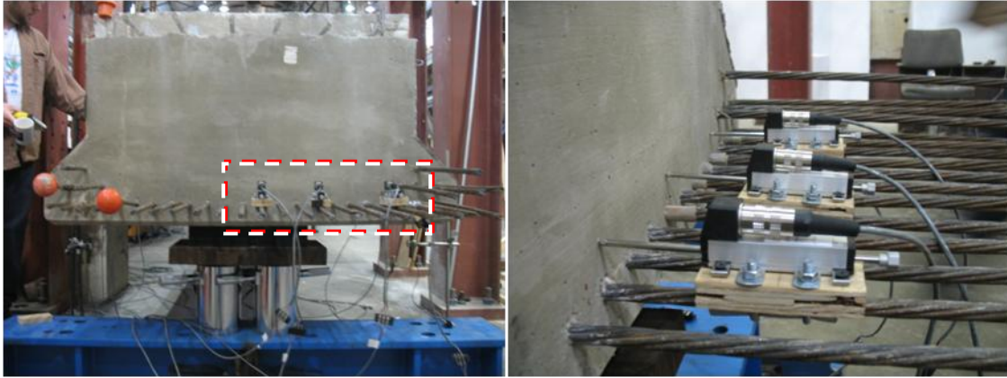
Figure 3-12: Strand slip instrumentation.
