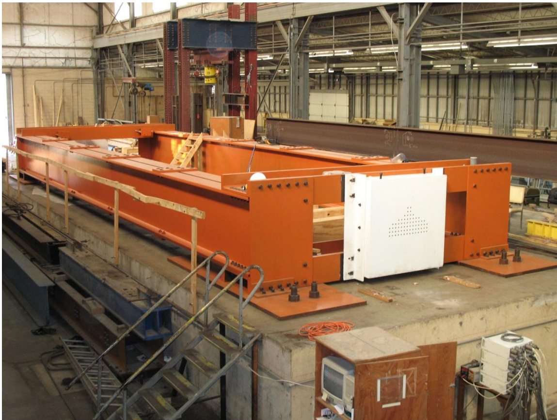
Figure 2-17: Prestressing Bed facility in FSEL
