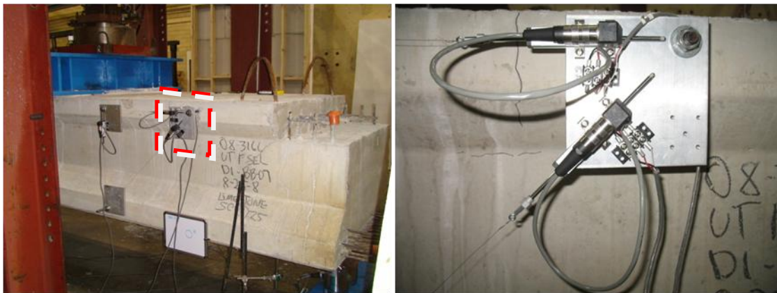
Figure 3-11: Shear deformation measurement instrumentation.
