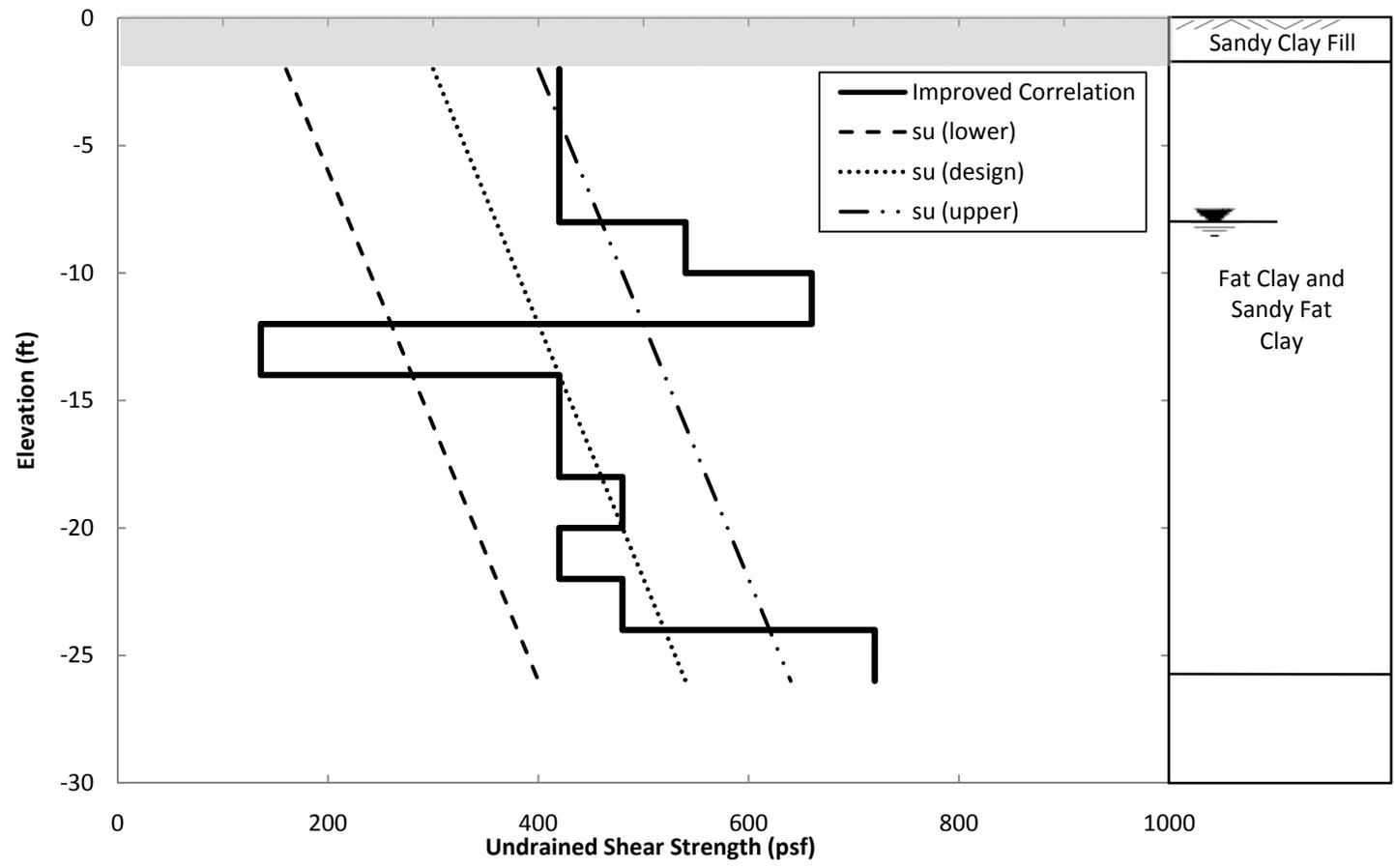
Figure 6.38: Undrained Shear Strength Profiles for Site No. 6
