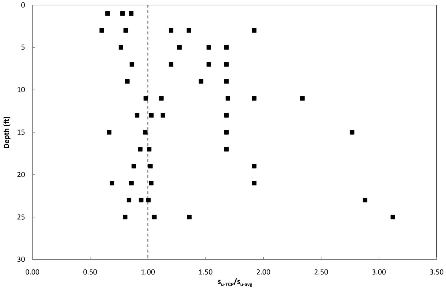
Figure 5.31: Ratio of the Undrained Shear Strength Computed from the Improved Correlation to the Undrained Shear Strength Determined Using the Average Undrained Strength Profile from Varathungarajan (2008)
