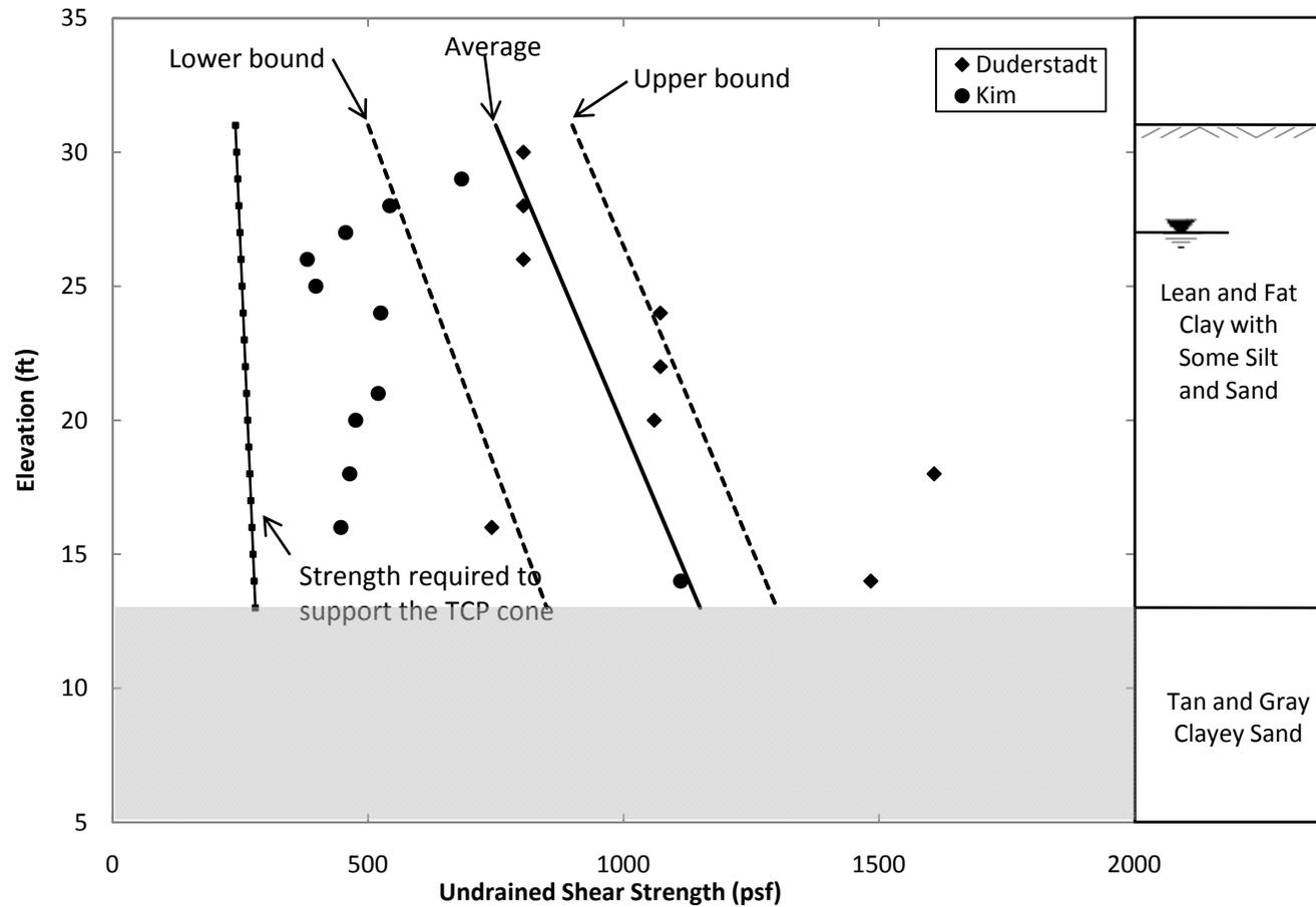
Figure 5.18: Undrained Shear Strengths for Site No. 3 using the Texas Cone Penetrometer Correlations from Duderstadt et al. (1977) and Kim et al. (2007)
