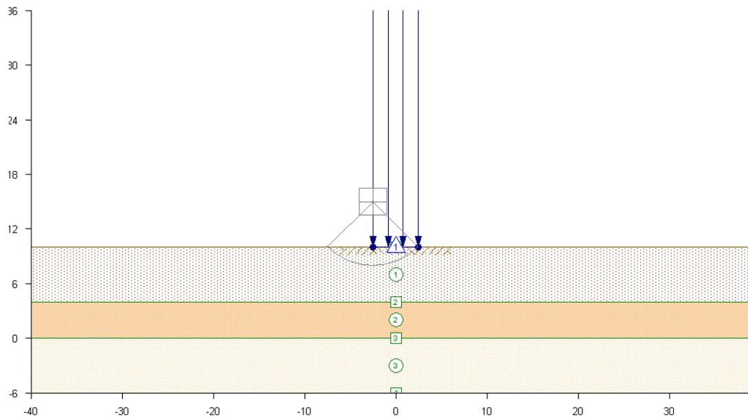
Figure 6.33: Simplified Graphic File for Site 1 using the Average Undrained Shear Strength Profile and a Load Width of 5 Feet
