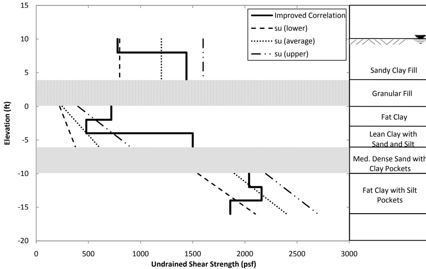
Figure 6.34: Undrained Shear Strength Profiles for Site No. 1
