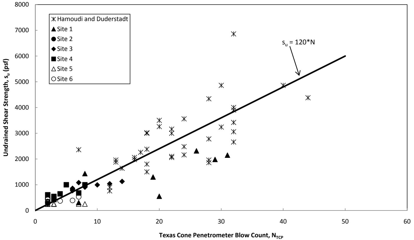
Figure 5.23: All Texas Cone Penetrometer Data from Hamoudi et al. (1974), Duderstadt et al. (1977) and the Additional Six Sites of this Study
