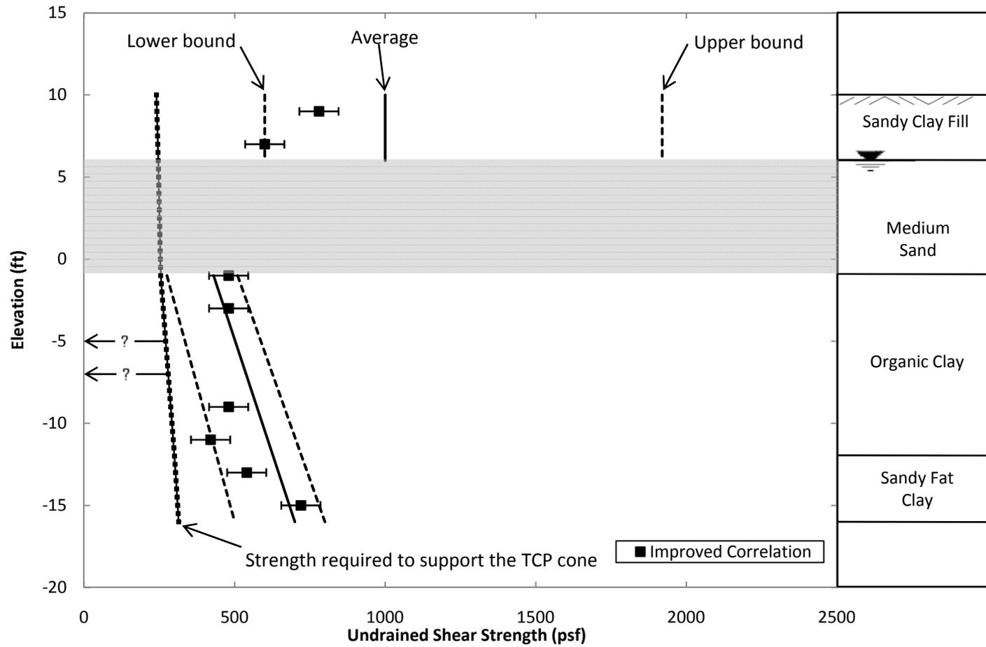
Figure 5.28: Undrained Shear Strengths for Site No. 4 using the Improved Correlation
