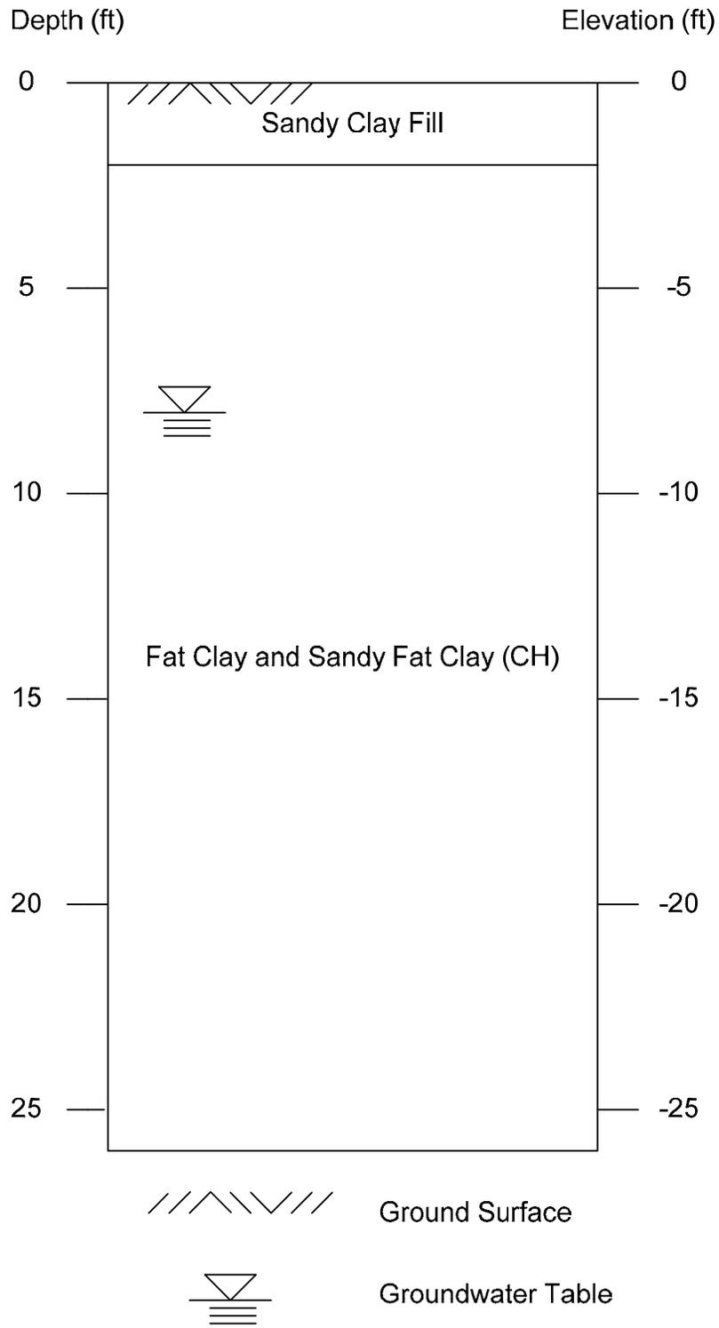
Figure 4.14: Stratigraphic Profile of Site No. 5
