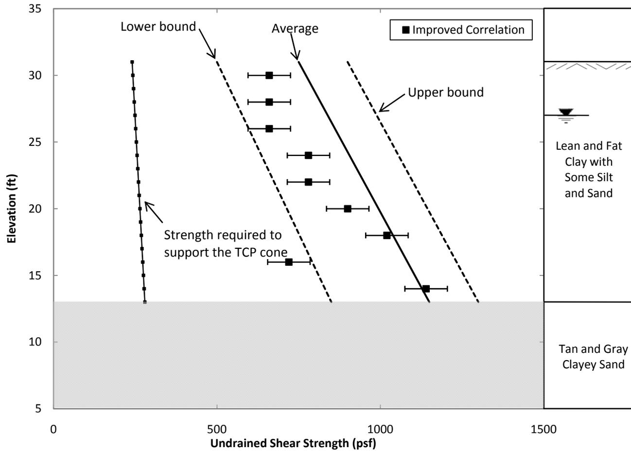
Figure 5.27: Undrained Shear Strengths for Site No. 3 using the Improved Correlation
