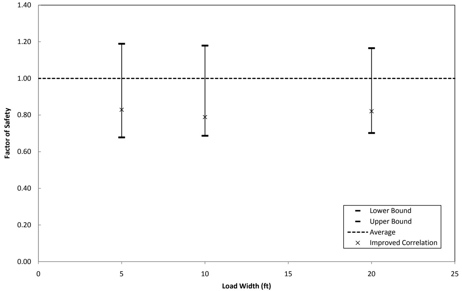
Figure 6.40: Factors of Safety Computed using UTEXAS4 for Site No. 3
