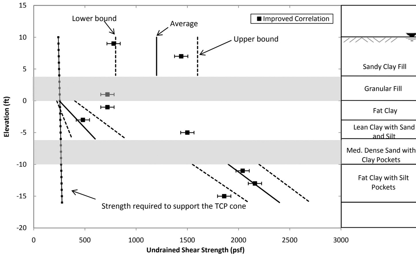
Figure 5.25: Undrained Shear Strengths for Site No. 1 using the Improved Correlation
