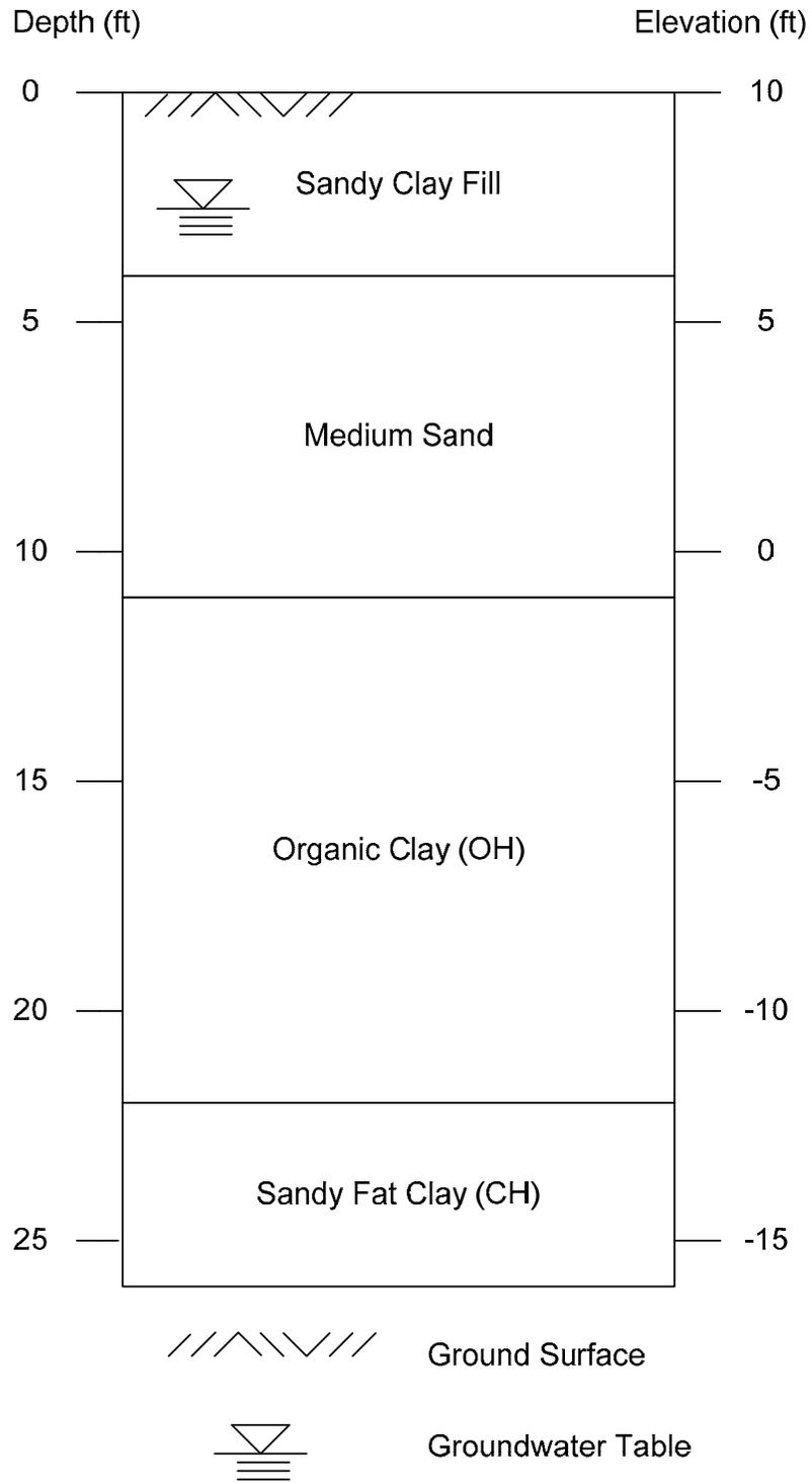
Figure 4.12: Stratigraphic Profile of Site No. 4
