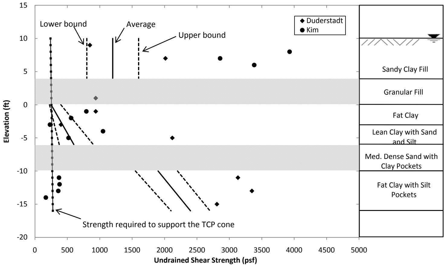
Figure 5.16: Undrained Shear Strengths for Site No. 1 using the Texas Cone Penetrometer Correlations from Duderstadt et al. (1977) and Kim et al. (2007)
