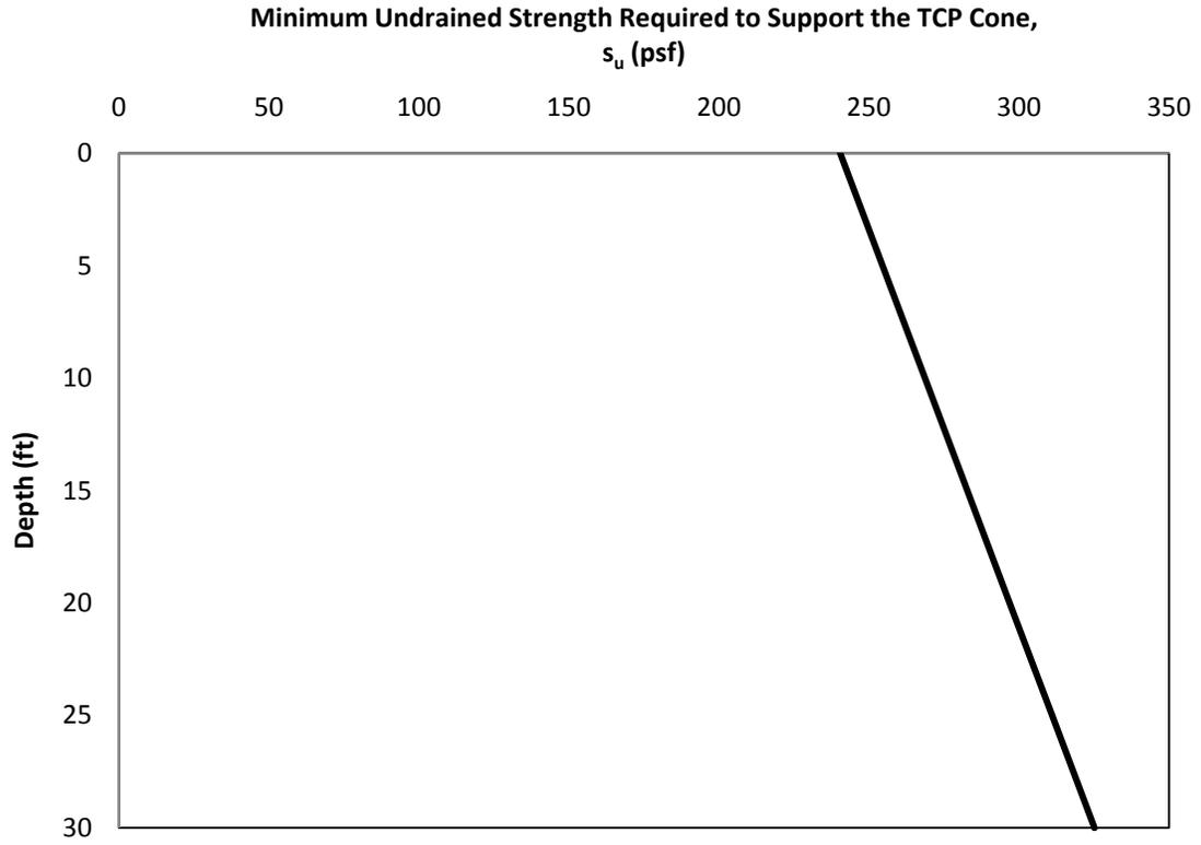
*Figure 2.2: Minimum Strength Required to Support the TCP Cone for Example*
