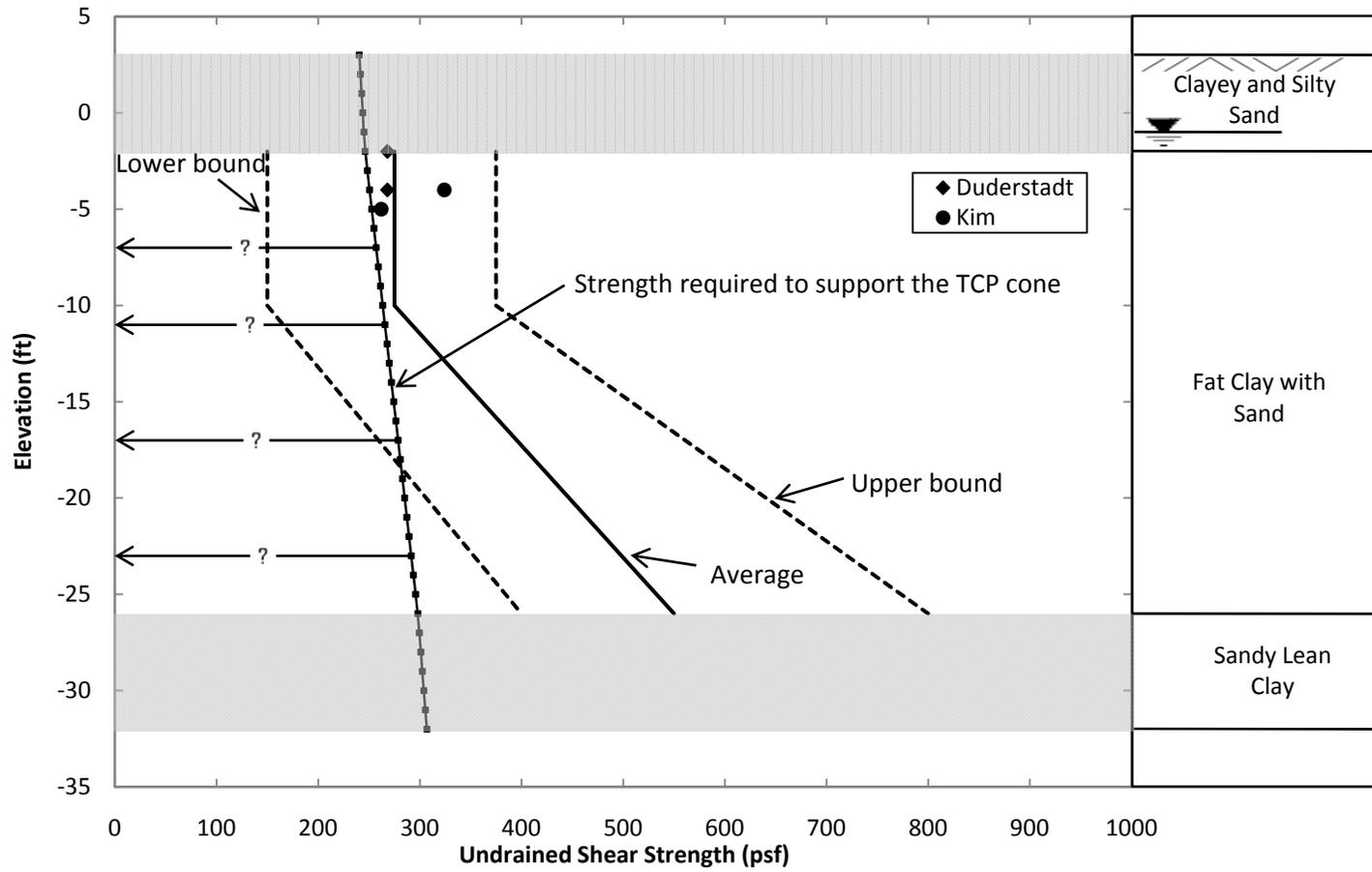
Figure 5.17: Undrained Shear Strengths for Site No. 2 using the Texas Cone Penetrometer Correlations from Duderstadt et al. (1977) and Kim et al. (2007)
