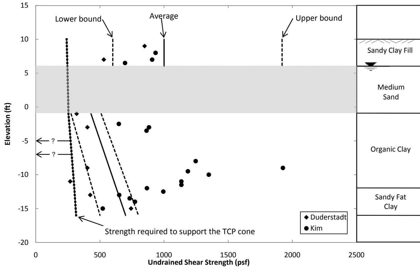
Figure 5.19: Undrained Shear Strengths for Site No. 4 using the Texas Cone Penetrometer Correlations from Duderstadt et al. (1977) and Kim et al. (2007)
