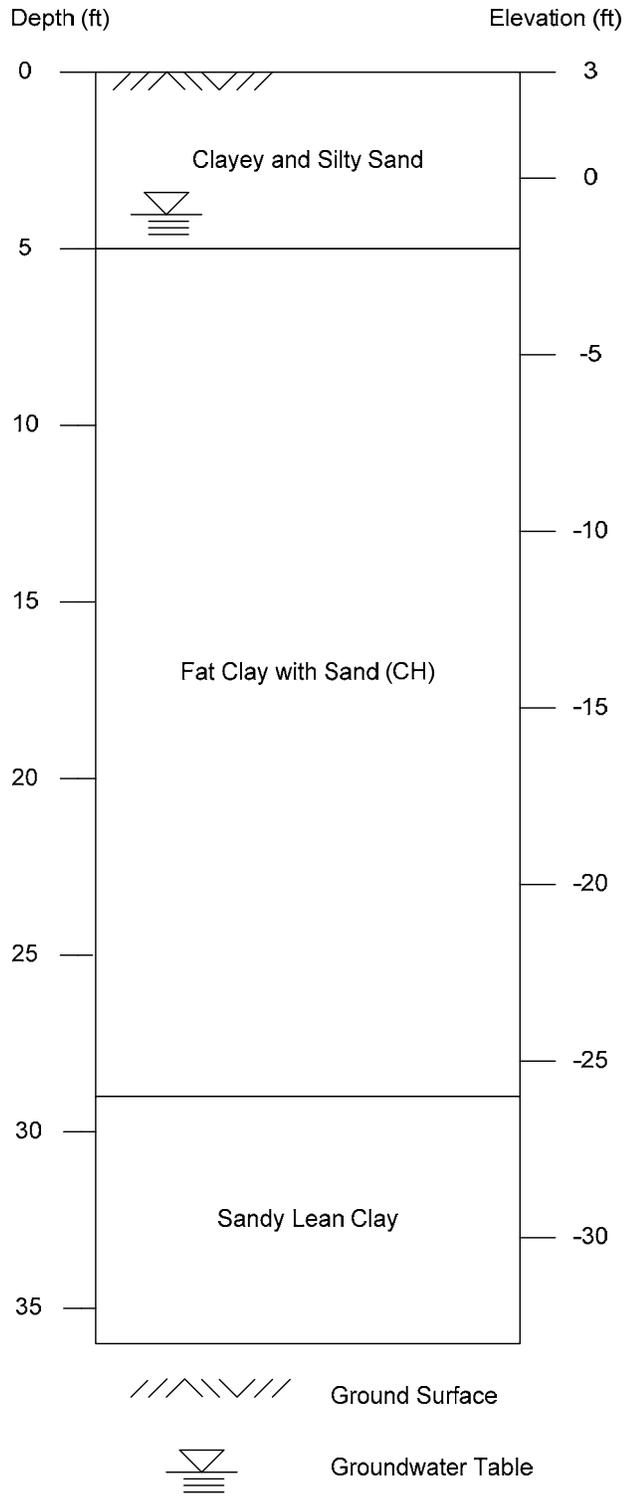
Figure 4.8: Stratigraphic Profile of Site No. 2
