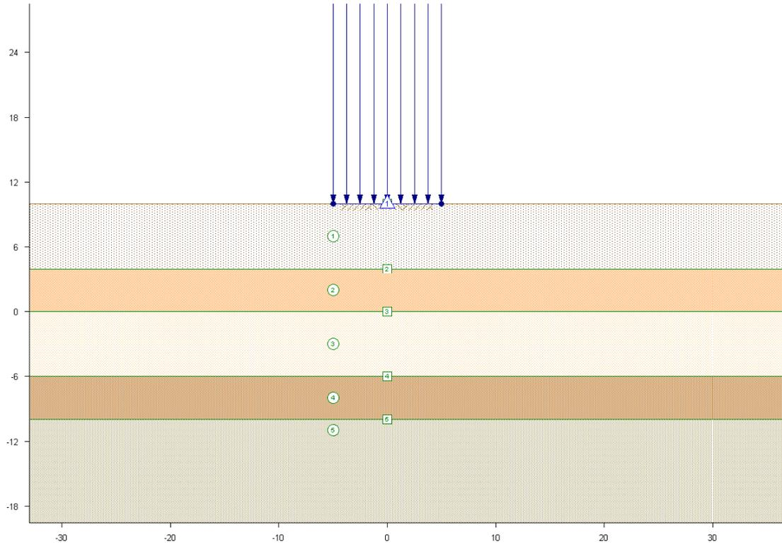
Figure 6.32: Graphic File for Site 1 using the Average Undrained Shear Strength Profile and a Load Width of 10 Feet
