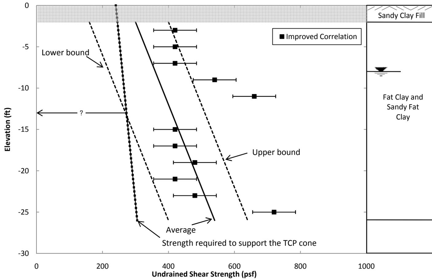
Figure 5.30: Undrained Shear Strengths for Site No. 6 using the Improved Correlation
