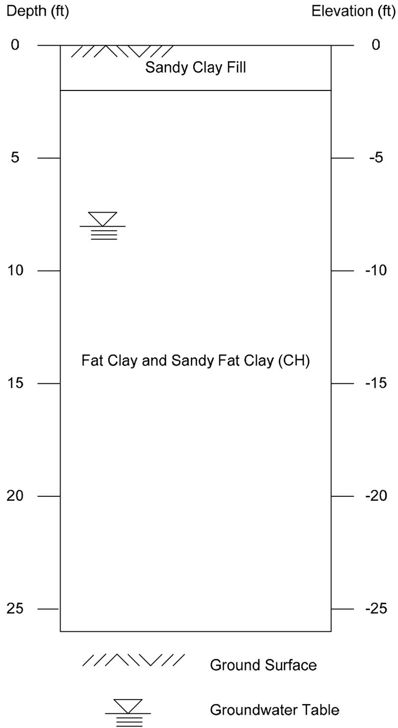
Figure 4.15: Stratigraphic Profile of Site No. 6
