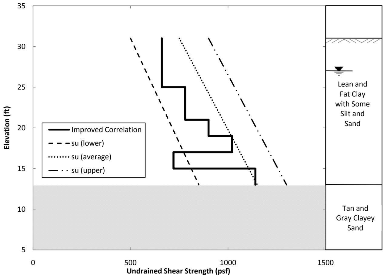
*Figure 6.35: Undrained Shear Strength Profiles for Site No. 3*
