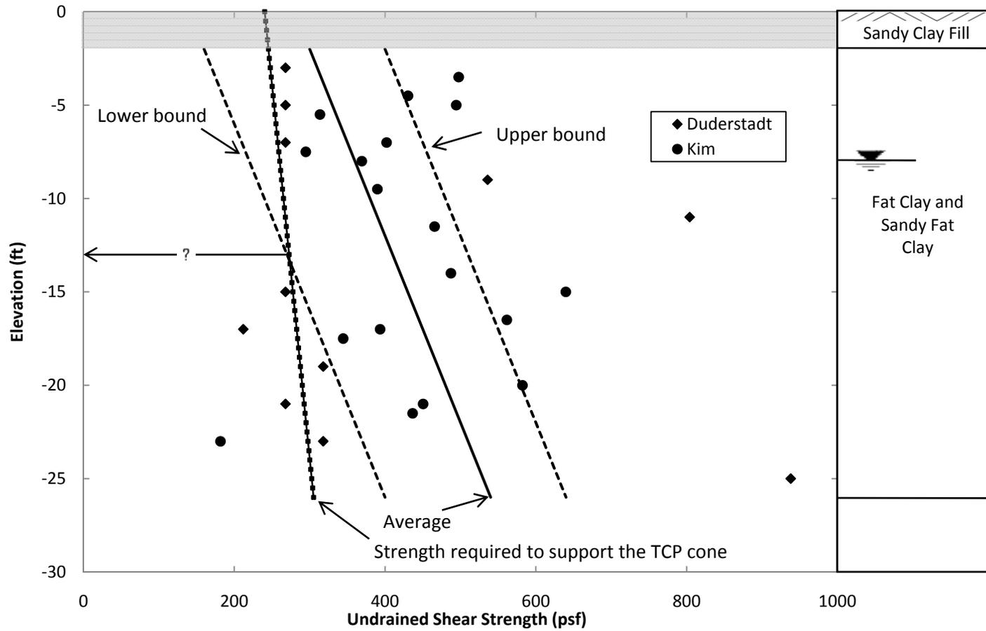
Figure 5.21: Undrained Shear Strengths for Site No. 6 using the Texas Cone Penetrometer Correlations from Duderstadt et al. (1977) and Kim et al. (2007)
