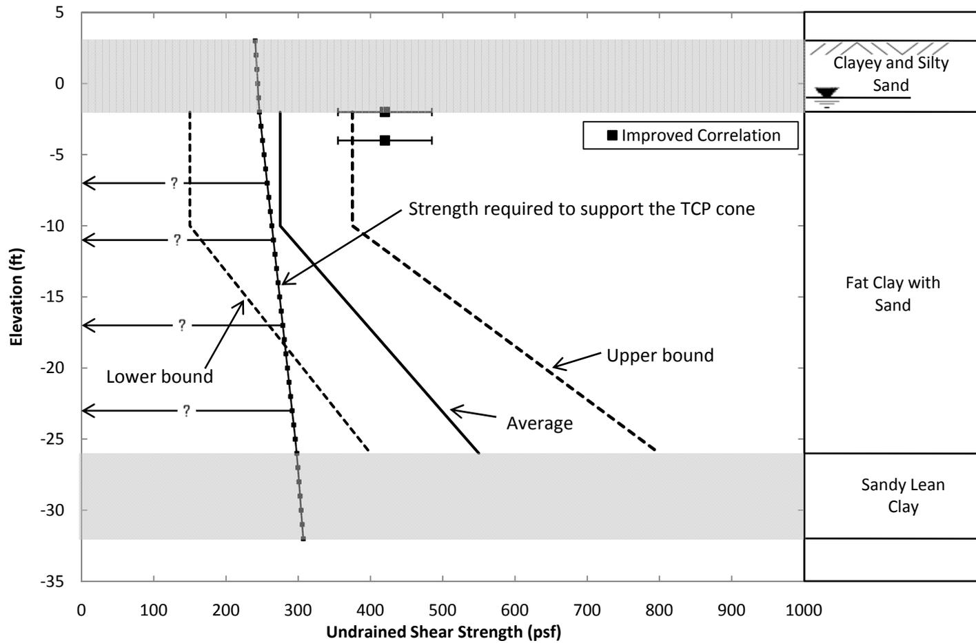
Figure 5.26: Undrained Shear Strengths for Site No. 2 using the Improved Correlation
