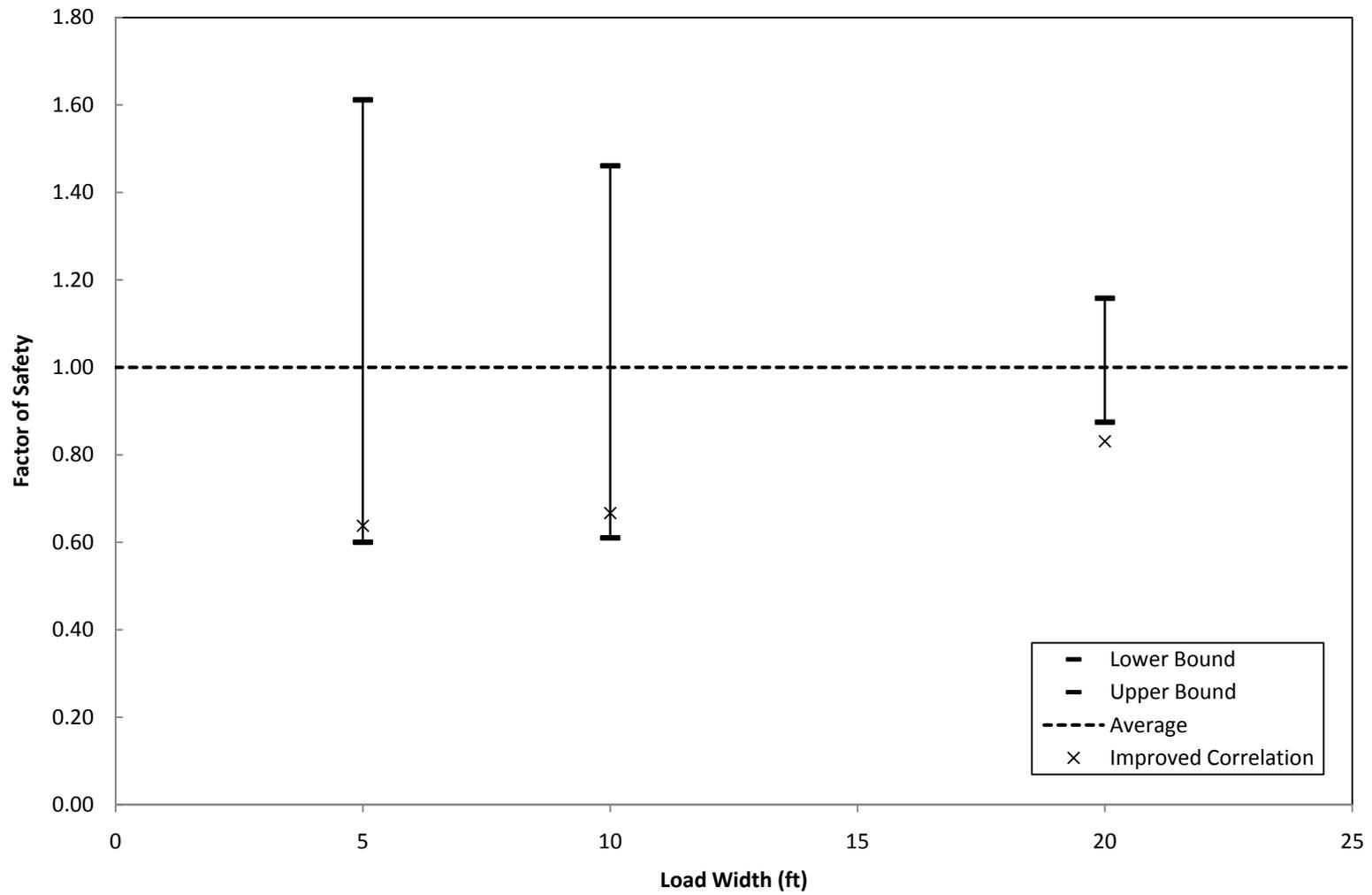
Figure 6.41: Factors of Safety Computed using UTEXAS4 for Site No. 4
