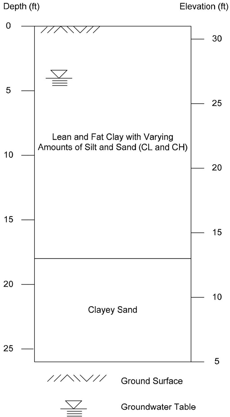
Figure 4.10: Stratigraphic Profile of Site No. 3
