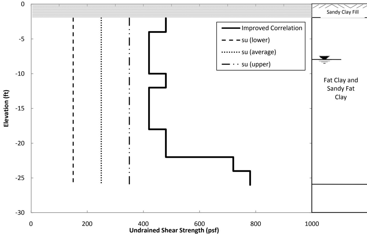
Figure 6.37: Undrained Shear Strength Profiles for Site No. 5
