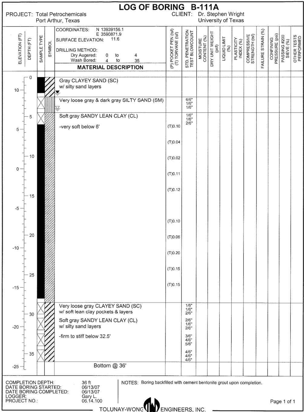
Figure B.3: Boring log with thin-walled tube samples for Site No. 2
