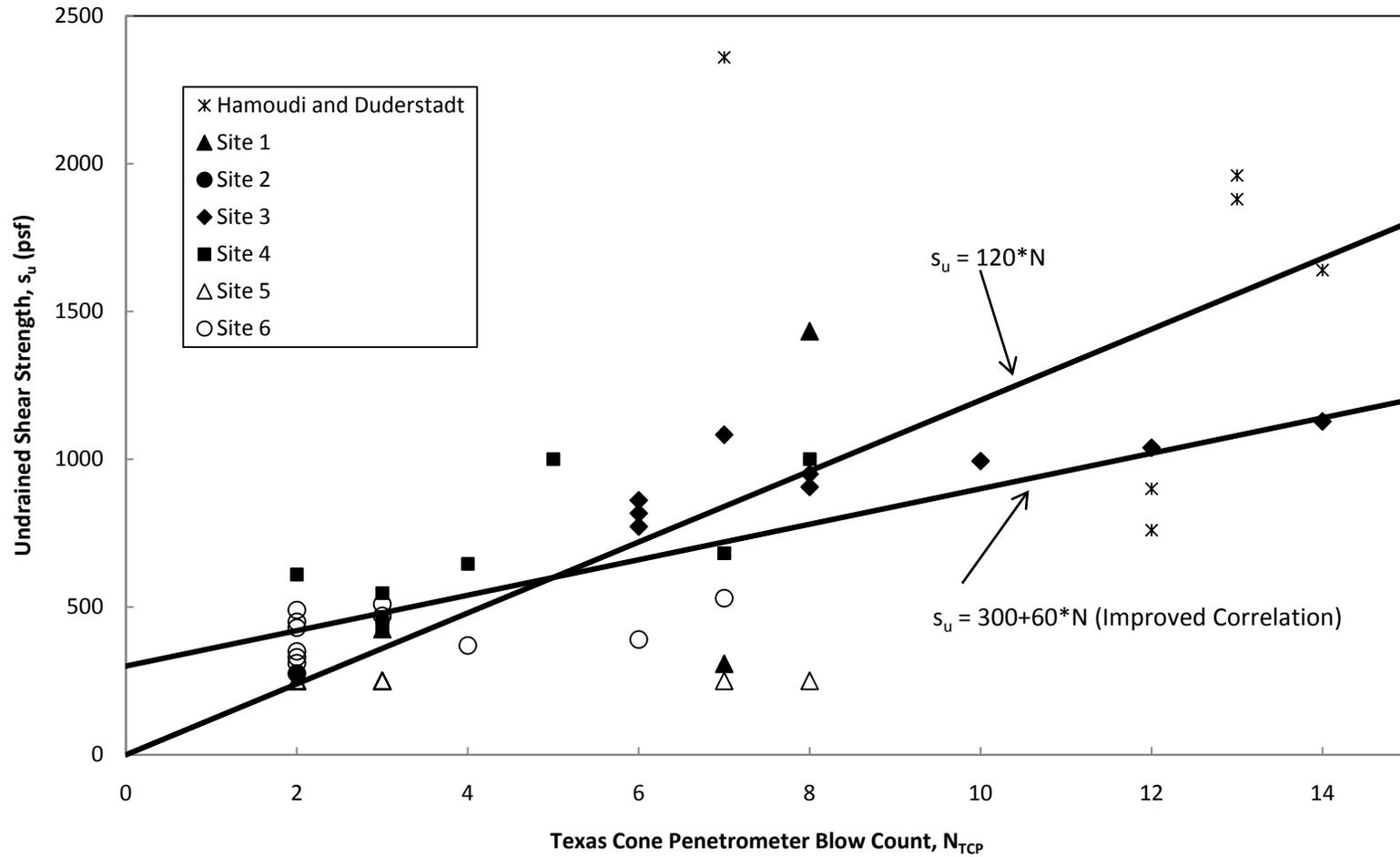
Figure 5.24: Texas Cone Penetrometer Data from Hamoudi et al. (1974), Duderstadt et al. (1977) and the Additional Six Sites of this Study for Blow Counts of 15 or less
