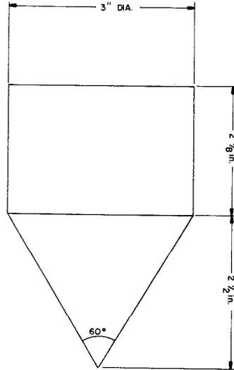
FIG-1 DETAILS OF THE CONE PENETROMETER
