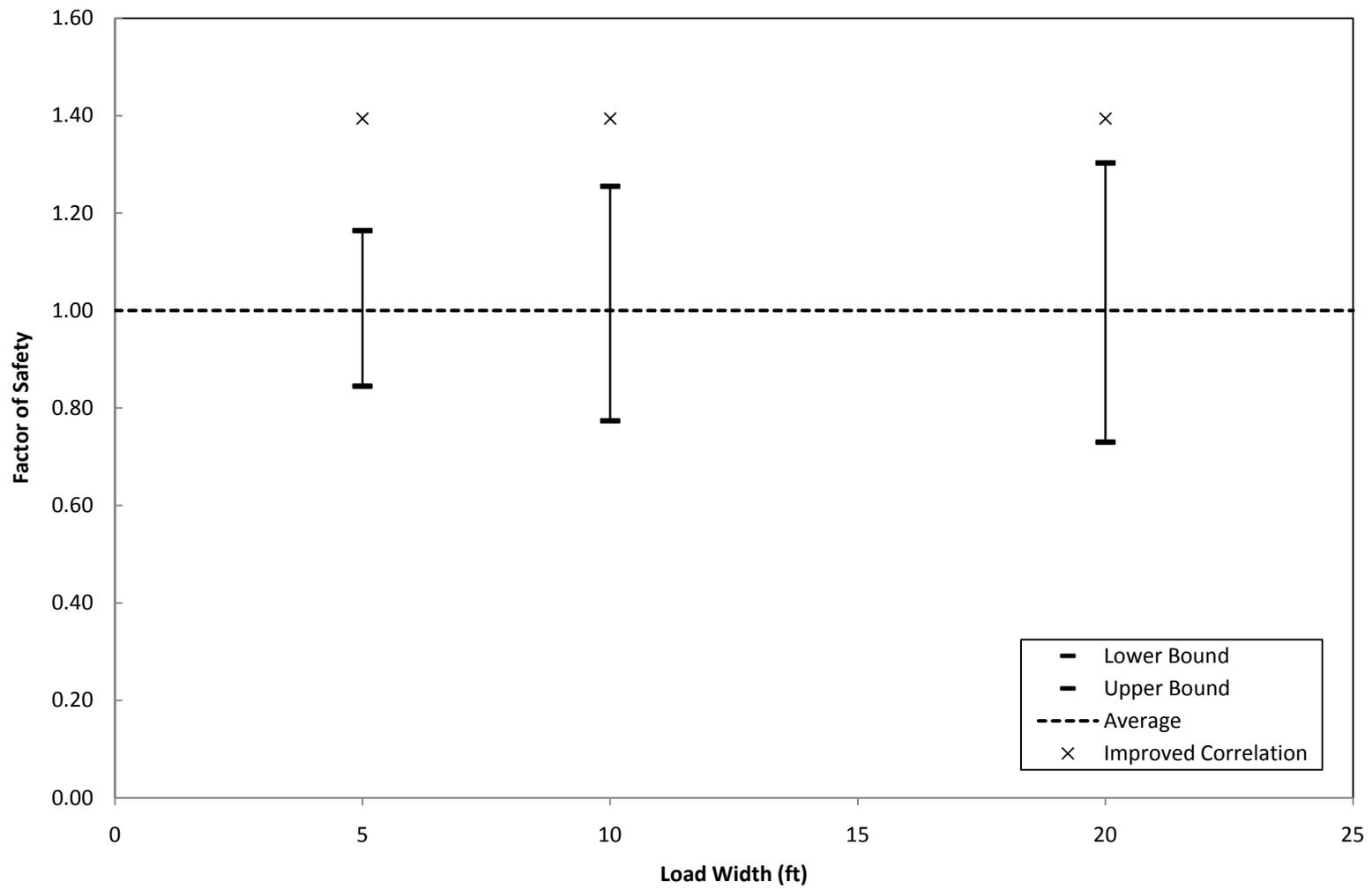
Figure 6.42: Factors of Safety Computed using UTEXAS4 for Site No. 5
