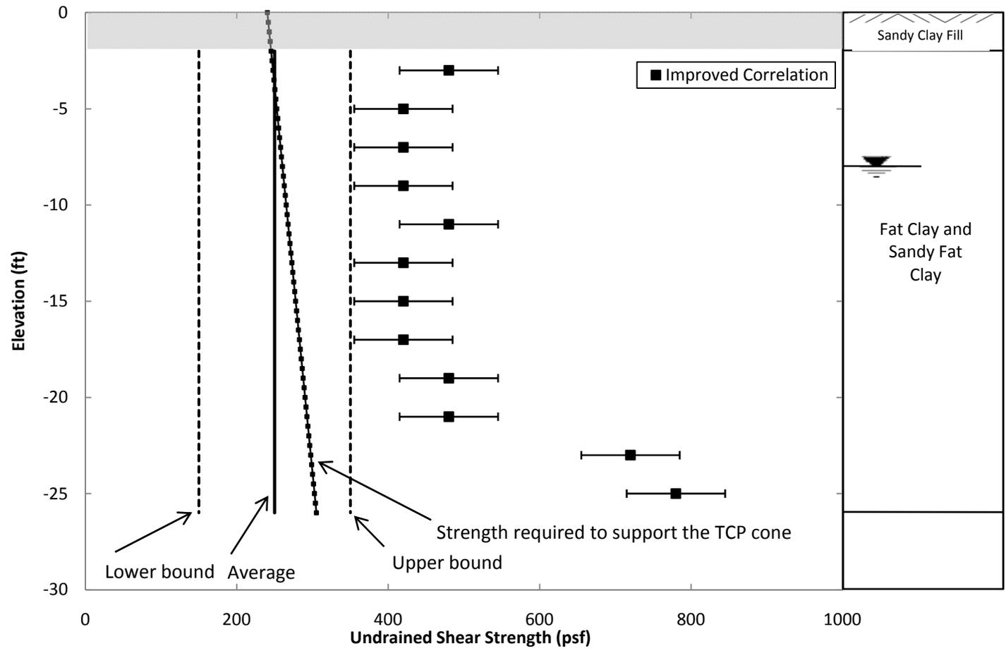
Figure 5.29: Undrained Shear Strengths for Site No. 5 using the Improved Correlation
