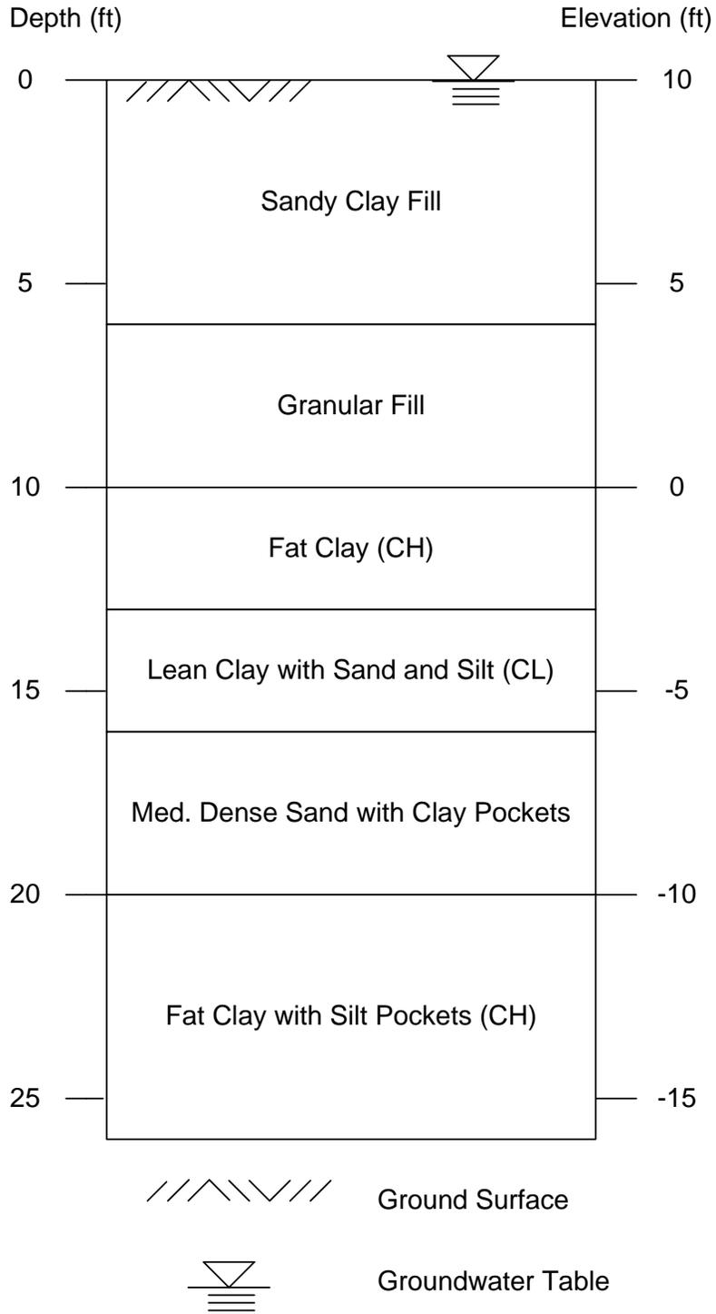
Figure 4.6: Stratigraphic Profile of Site No. 1
