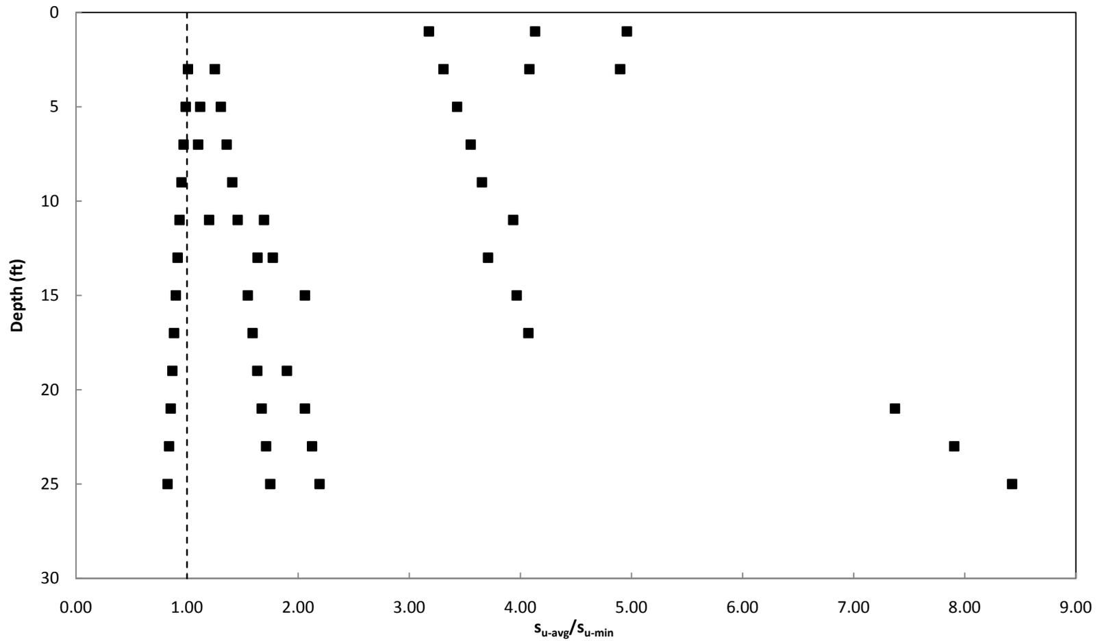
Figure 5.22: Ratio of the Undrained Shear Strength Determined Using the Average Undrained Strength Profile from Varathungarajan (2008) to the Minimum Undrained Shear Strength Required to Support the TCP Cone
