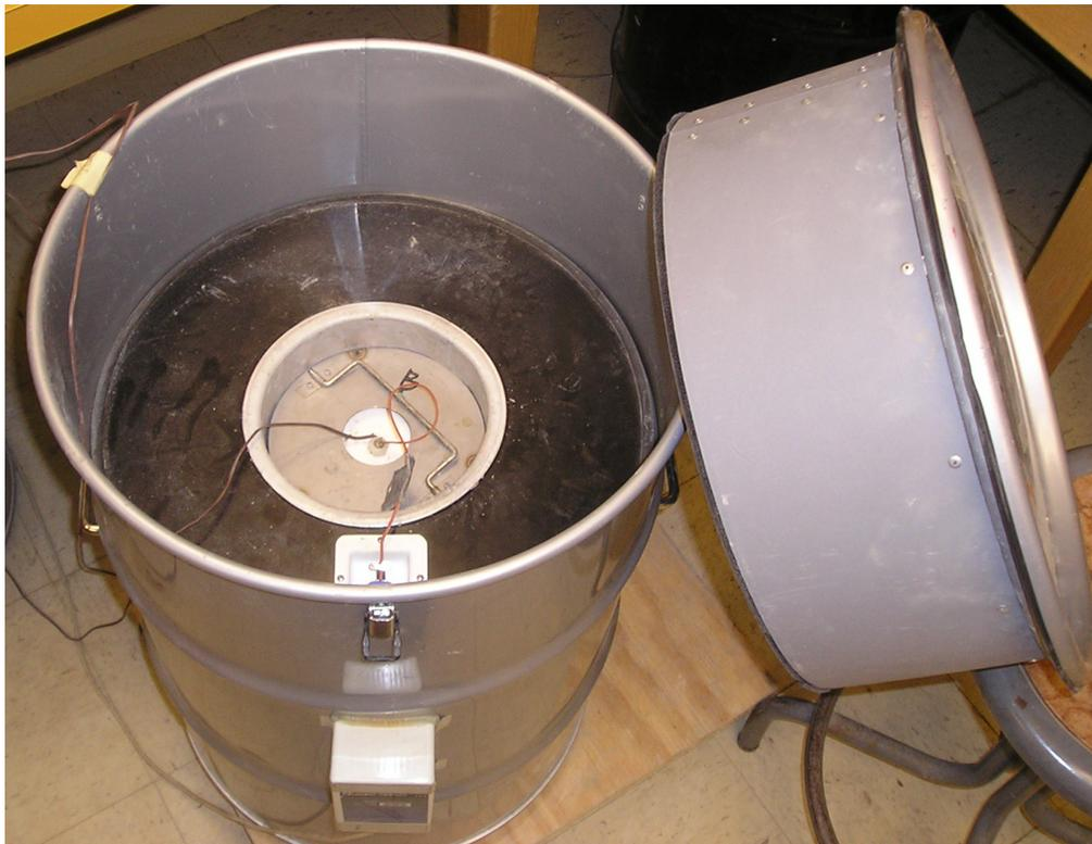
*Figure 3.1: Semi-adiabatic calorimeter*
