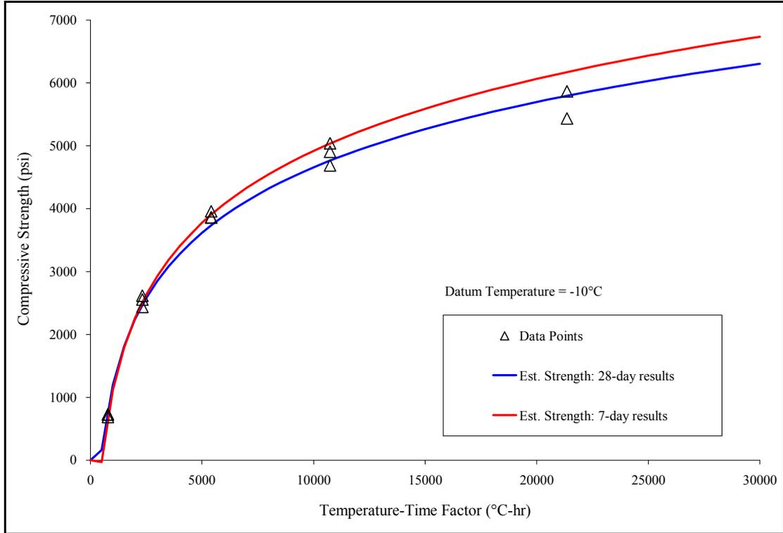
Figure C-9: Compressive strength vs. TTF: Mix 9 (35% Slag, 15% FAI, Optimum)
