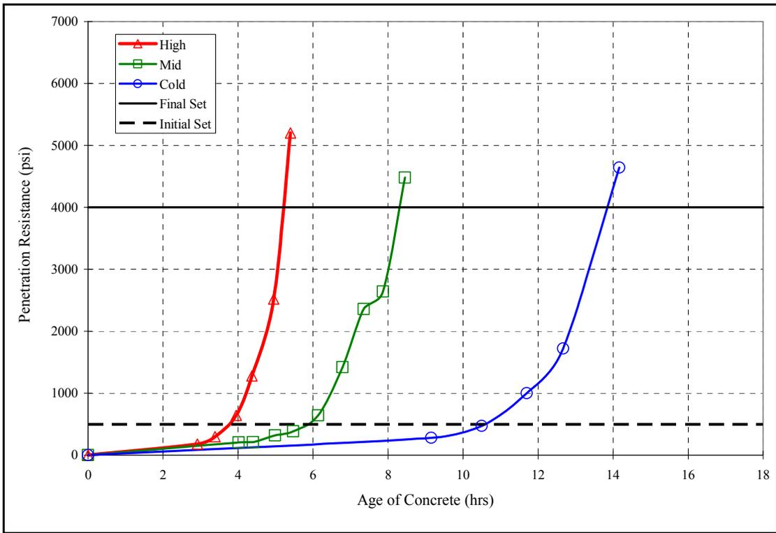
Figure D-6: Penetration resistance vs. time: Mix 6 (35% Slag)
