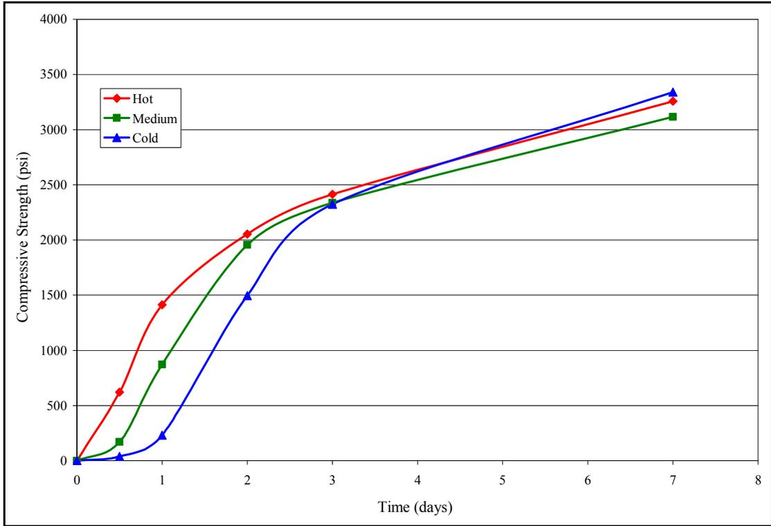
Figure 4.8: Compressive strength vs. time: mix 2 (20% FA1)
