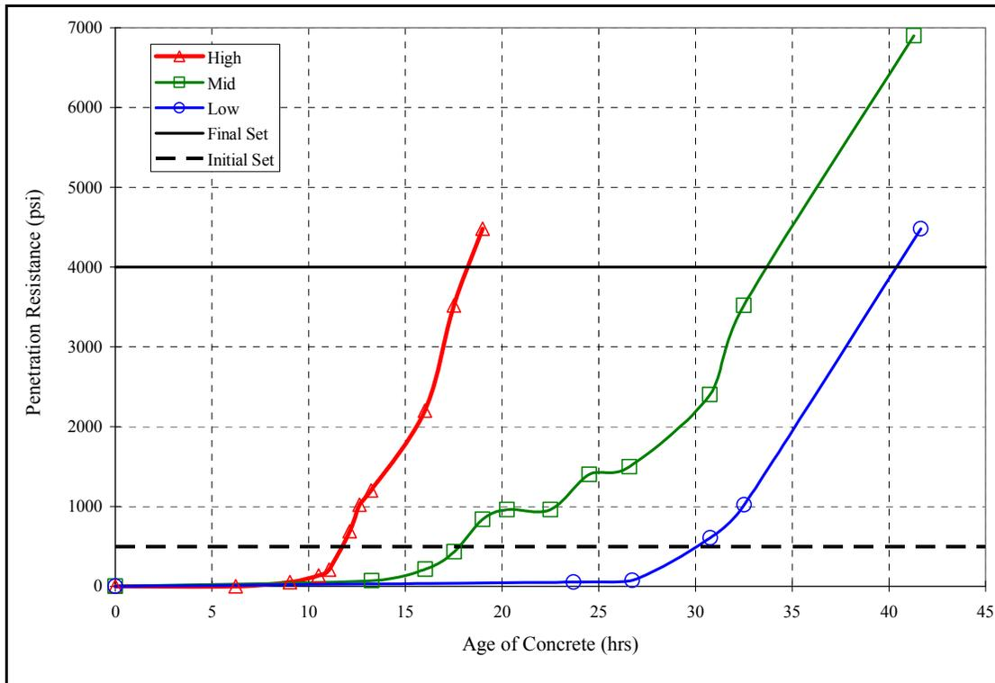
Figure D-11: Penetration resistance vs. time: El Paso mix (w/c = .55)
