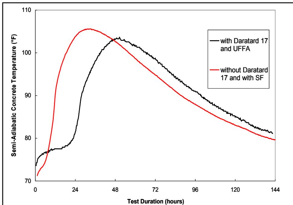
Figure 2.1: Semi-adiabatic calorimetry curves for concrete mixtures containing 30% Oklaunion fly ash. (J. Poole, unpublished data)
