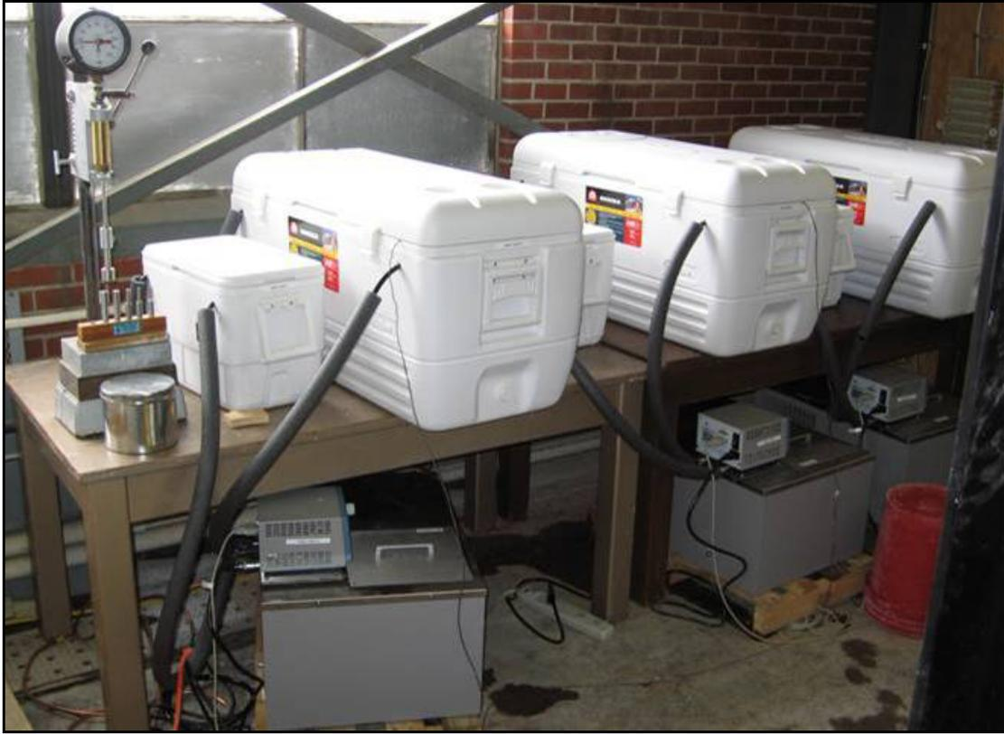
*Figure 3.4: Water baths and tanks used in TS testing*
