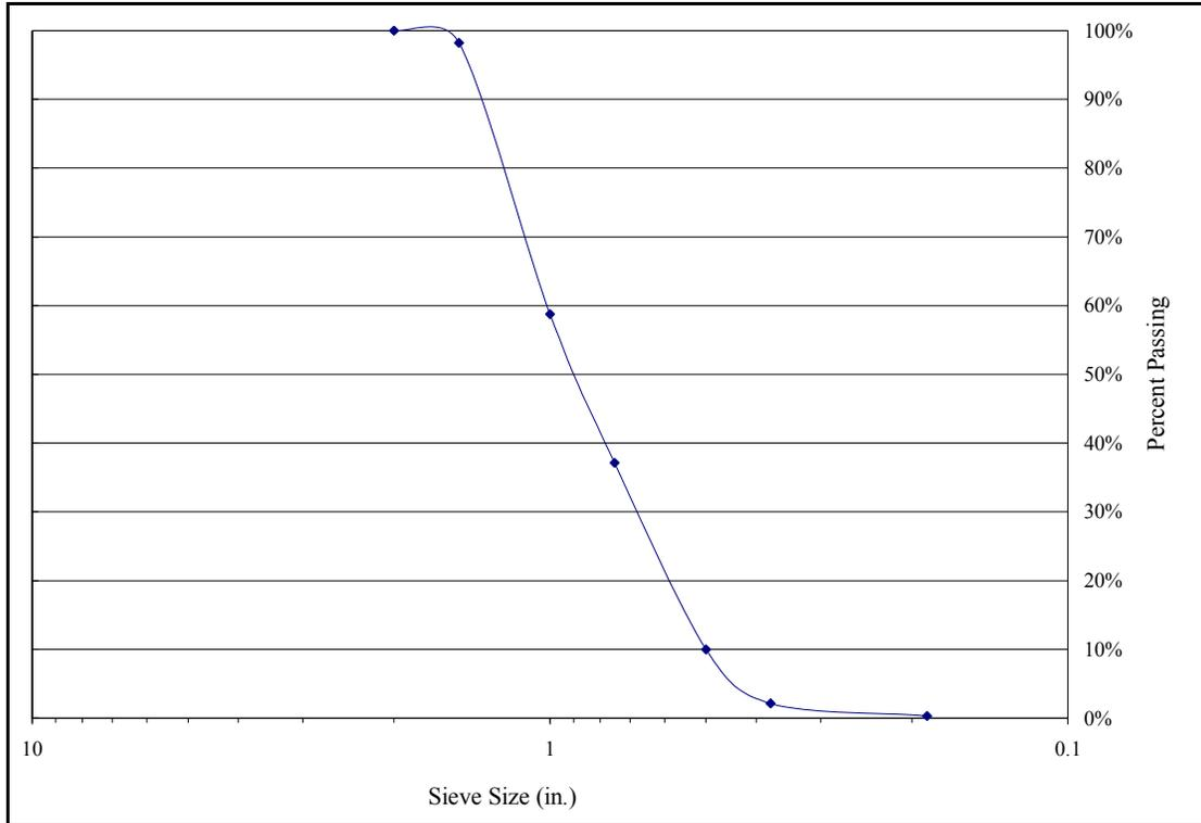
*Figure A-2: Average coarse aggregate gradation from 3 stockpile samples*
