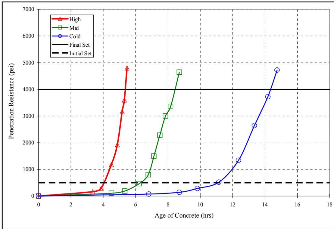
Figure D-8: Penetration resistance vs. time: Mix 8 (35% Slag, 15% FA1)
