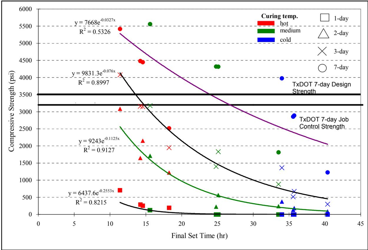
Figure 4.17: Compressive strength vs. final set time for El Paso mixes
