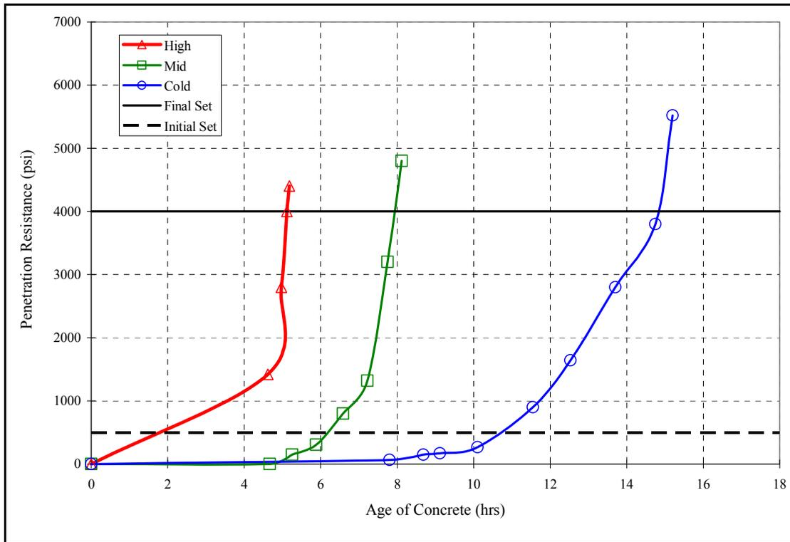
Figure D-4: Penetration resistance vs. time: Mix 4 (20% FA2)
