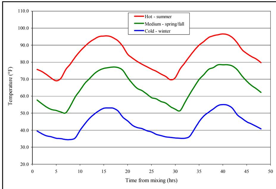
Figure 3.5: Ambient temperature profile used to predict concrete temperatures for a 48-hr period from mixing
