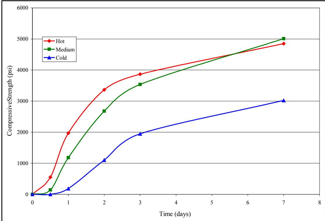
Figure 4.9: Compressive strength vs. time: mix 6 (35% Slag)
