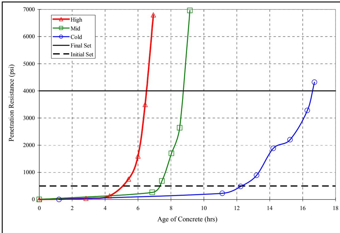
Figure D-2: Penetration resistance vs. time: Mix 2 (20% FA1)
