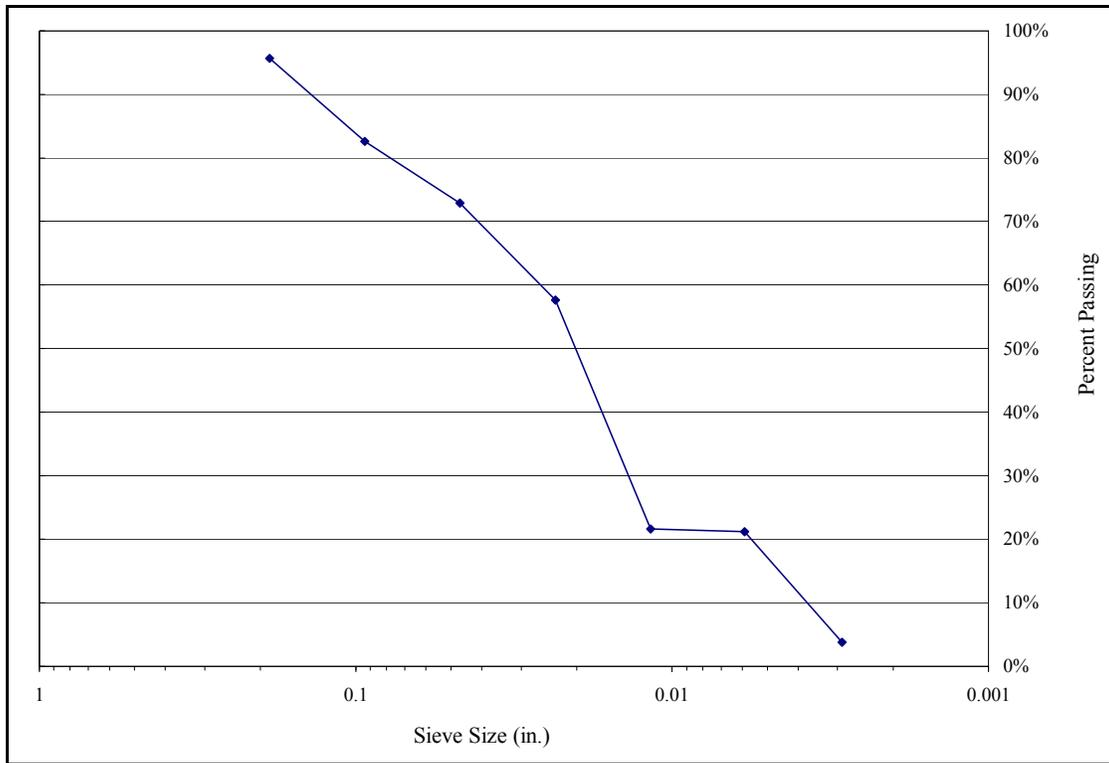
*Figure A-3: Fine aggregate gradation*
