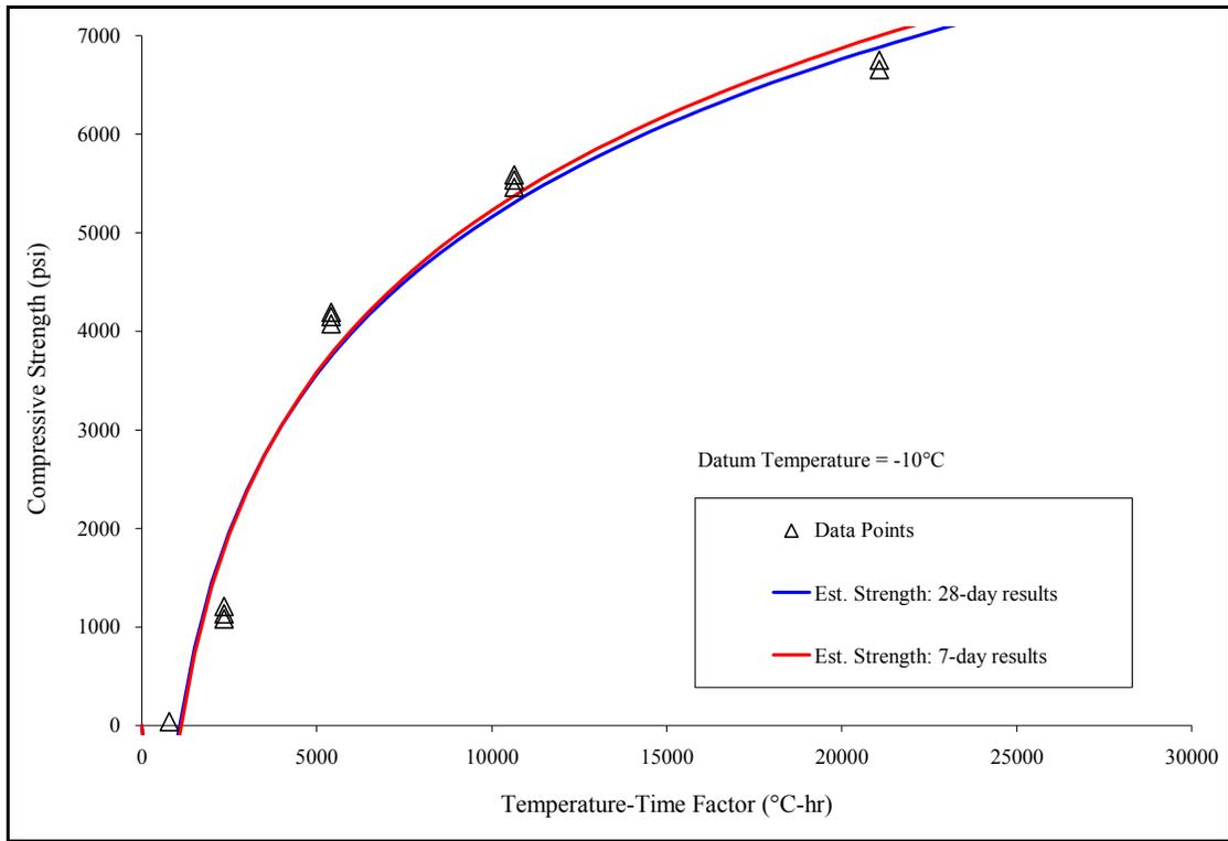
Figure C-10: Compressive strength vs. TTF: El Paso mix (w/c = .40)
