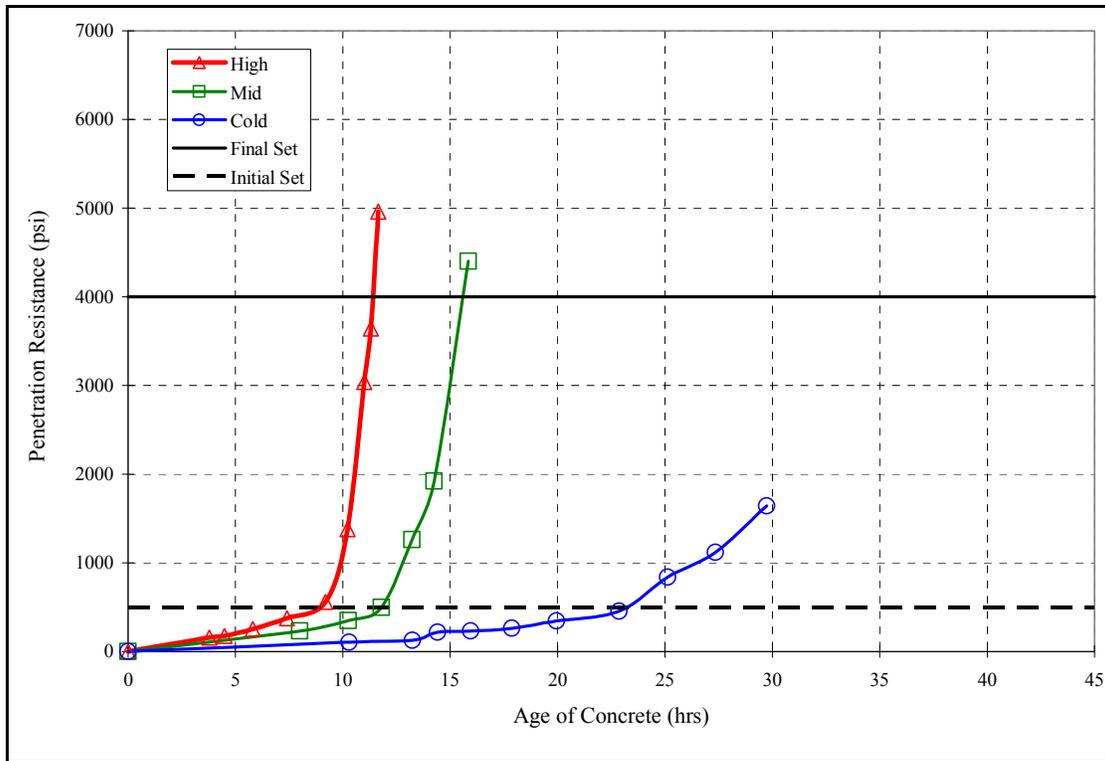
Figure D-9: Penetration resistance vs. time: El Paso mix (w/c = .40)
