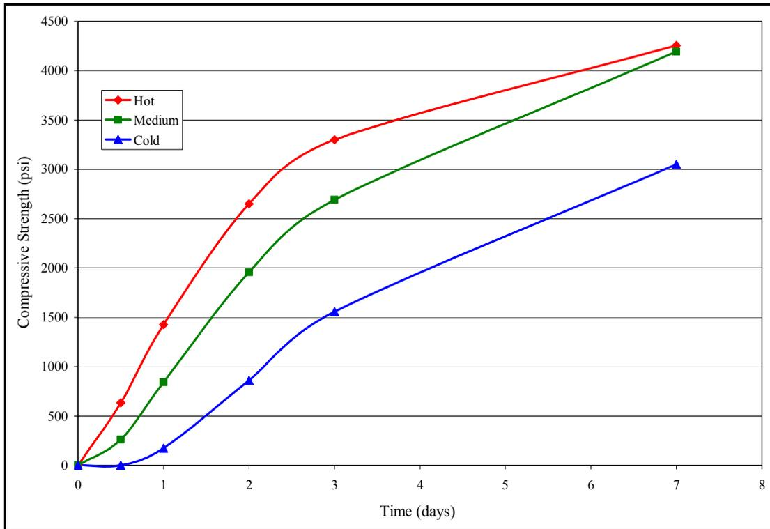
Figure 4.10: Compressive strength vs. time: mix 8 (35% Slag, 15% FAI)
