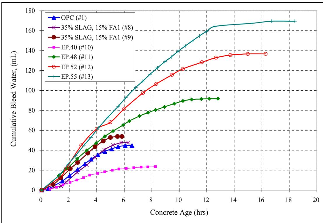
Figure 4.15: Cumulative bleed water vs. time from mixing for control and slag mixes
