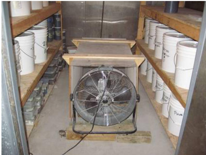
*Figure 3.7: Plastic shrinkage test no. 1. A fan was used to increase evaporation and thus maximize the potential for plastic shrinkage cracking.*
