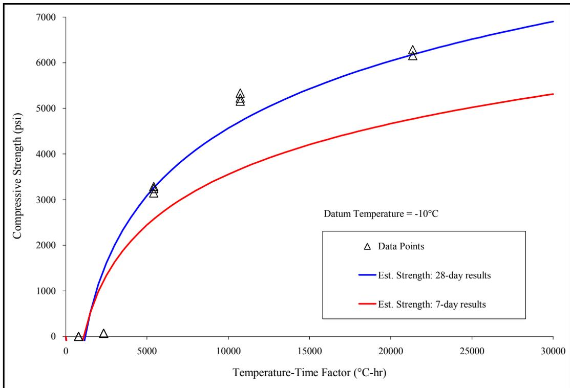
Figure C-11: Compressive strength vs. TTF: El Paso mix (w/c = .48)
