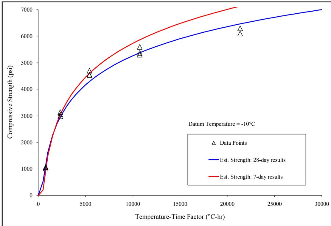
Figure C-6: Compressive strength vs. TTF: Mix 6 (35% Slag)
