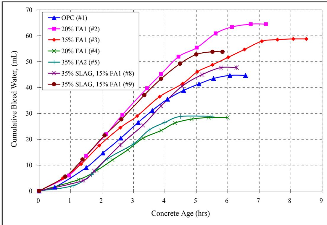
Figure 4.14: Cumulative bleed water vs. time from mixing for control and fly ash mixes
