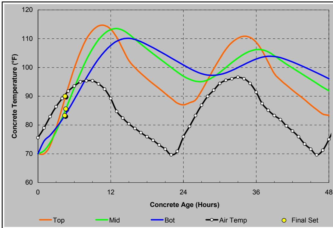
Figure 2.2: Temperature of an OPC concrete pavement as estimated by PavePro
