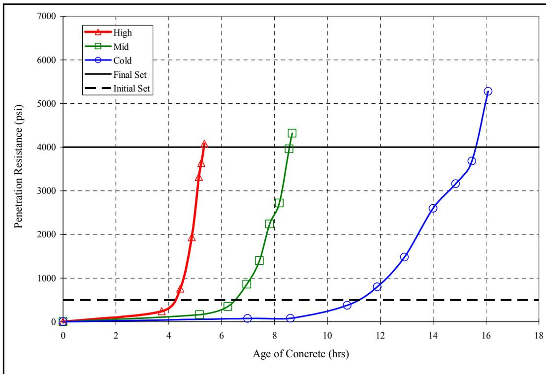
Figure D-8: Penetration resistance vs. time: Mix 9 (35% Slag, 15% FA1, Optimum)
