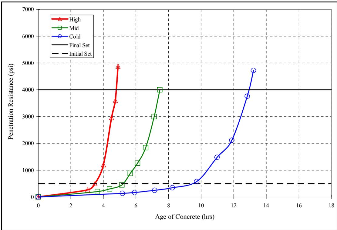
Figure D-7: Penetration resistance vs. time: Mix 7 (50% Slag)
