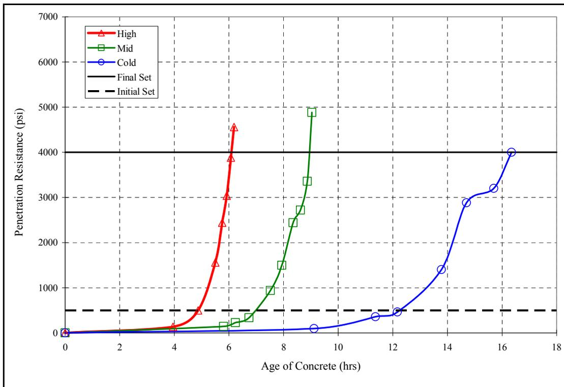
Figure D-5: Penetration resistance vs. time: Mix 5 (35% FA2)
