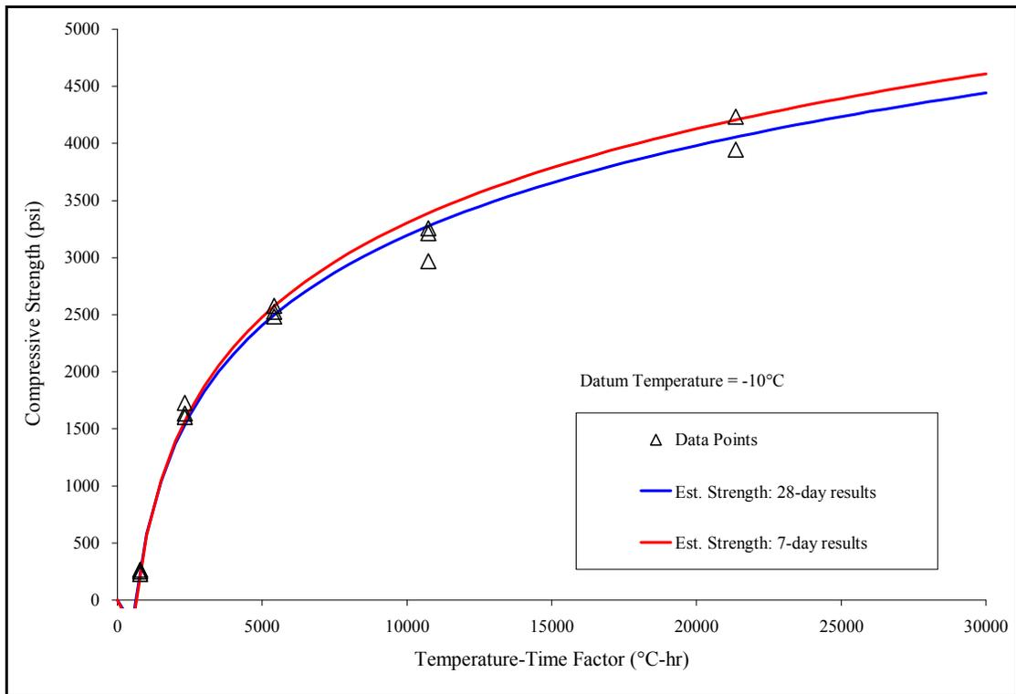
Figure C-3: Compressive strength vs. TTF: Mix 3 (35% FAI)
