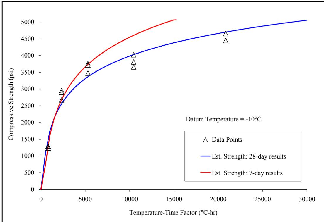
Figure 4.3: Maturity plot of compressive strength vs. TTF for the control mix
