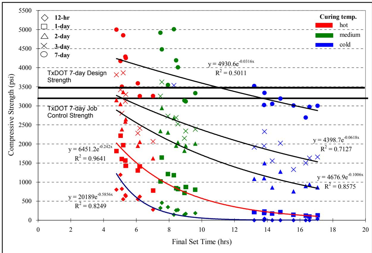
Figure 4.16: Compressive strength vs. final set time for mixes 1-9
