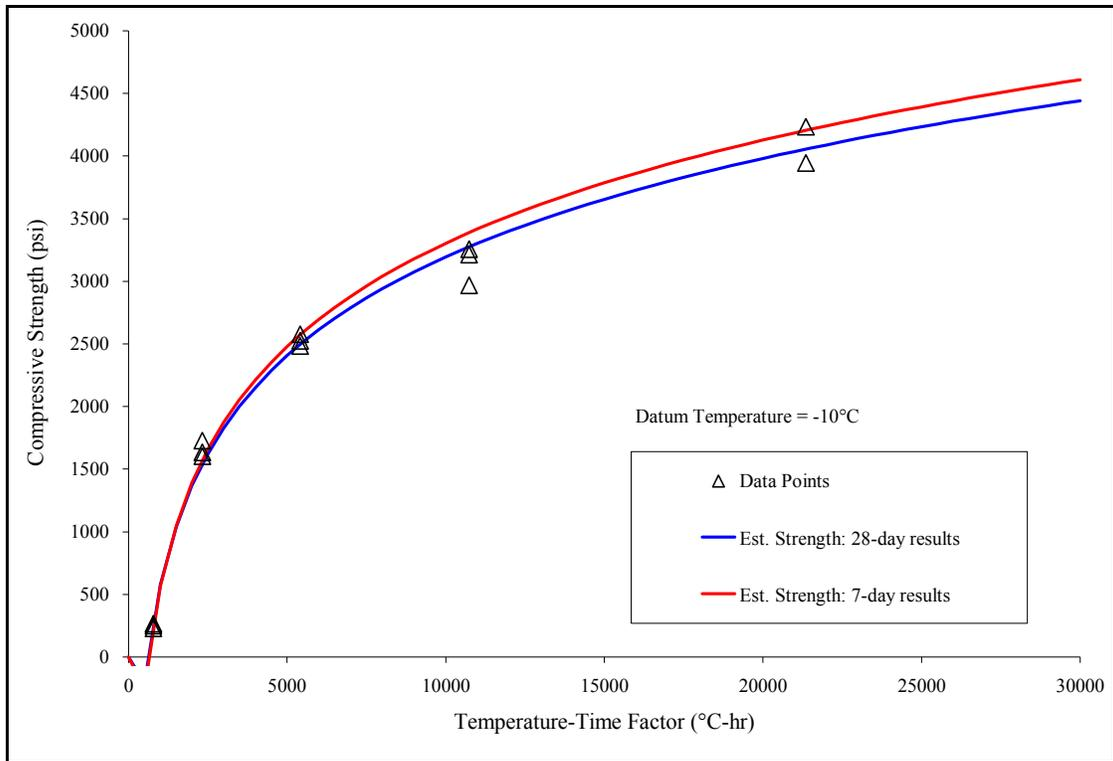
Figure C-4: Compressive strength vs. TTF: Mix 4 (20% FA2)
