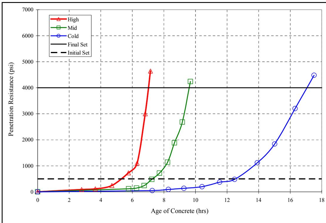
Figure D-3: Penetration resistance vs. time: Mix 3 (35% FA1)
