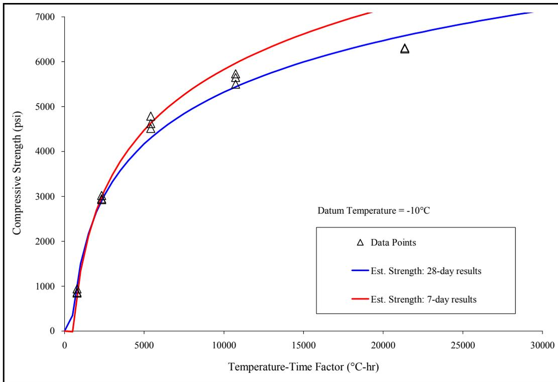
Figure C-7: Compressive strength vs. TTF: Mix 7 (50% Slag)
