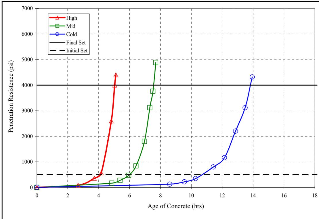
Figure D-1: Penetration resistance vs. time: Mix 1 (OPC)
