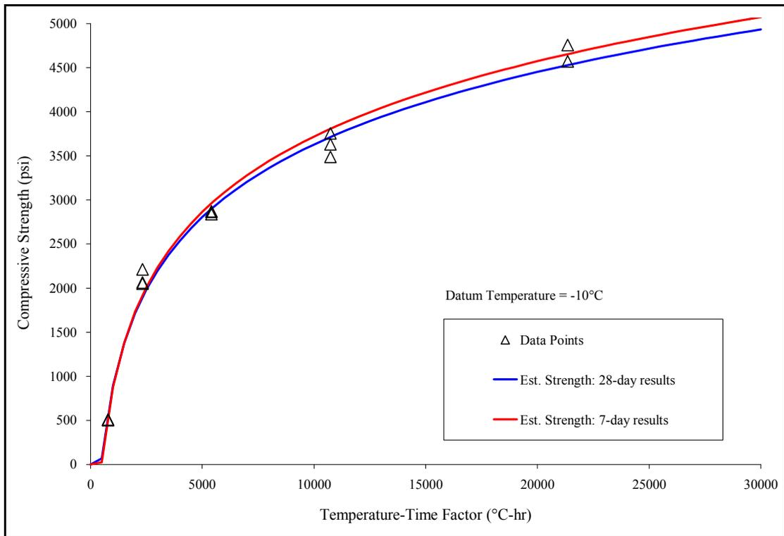
Figure C-5: Compressive strength vs. TTF: Mix 5 (35% FA2)
