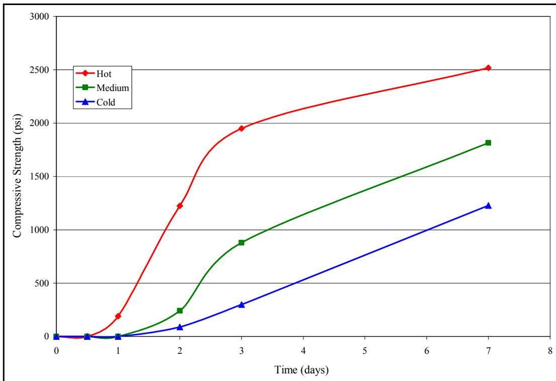
Figure 4.11: Compressive strength vs. time: El Paso mix (50% Slag, w/c = 0.55)
