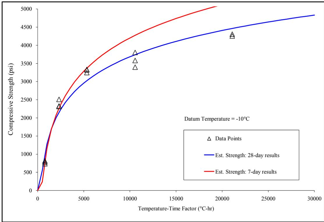
Figure C-2: Compressive strength vs. TTF: Mix 2 (20% FAI)
