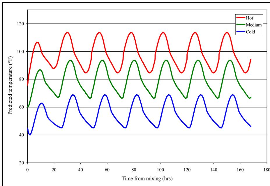
Figure 3.6: Predicted concrete temperature profiles for mix no. 8
