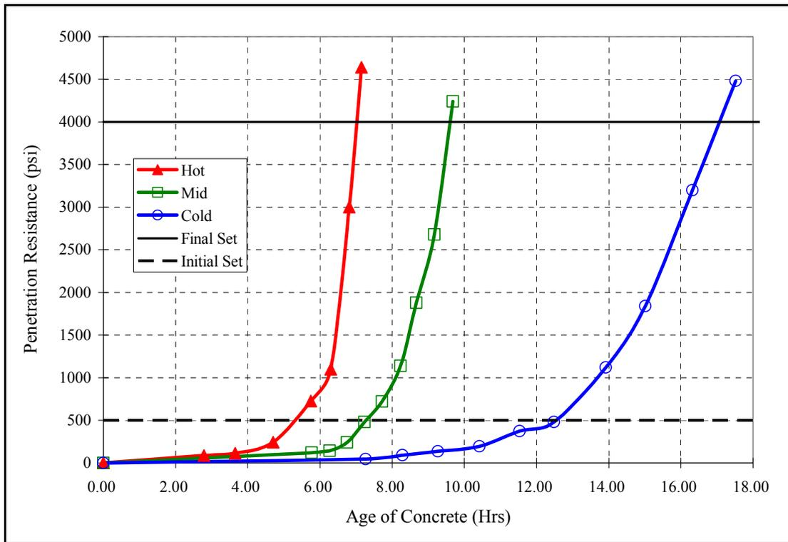
Figure 4.4: Example of penetration resistance as a function of time for mix no. 3
