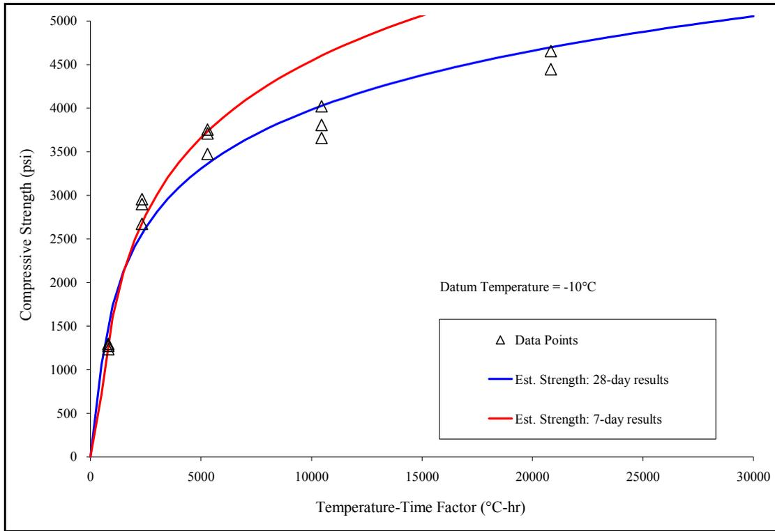
Figure C-1: Compressive strength vs. TTF: Mix 1 (OPC)
