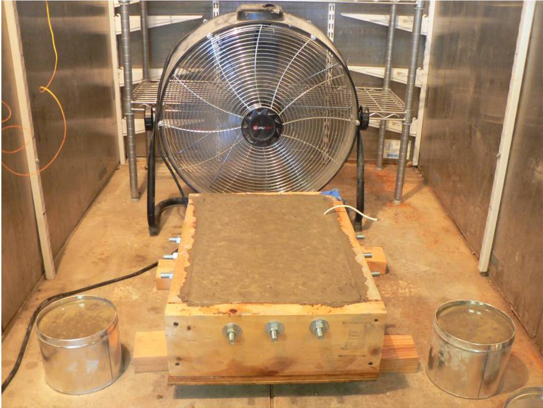
*Figure 3.8: Plastic shrinkage test no. 3. The bolts sticking out from the specimen were used to provide restraint.*
