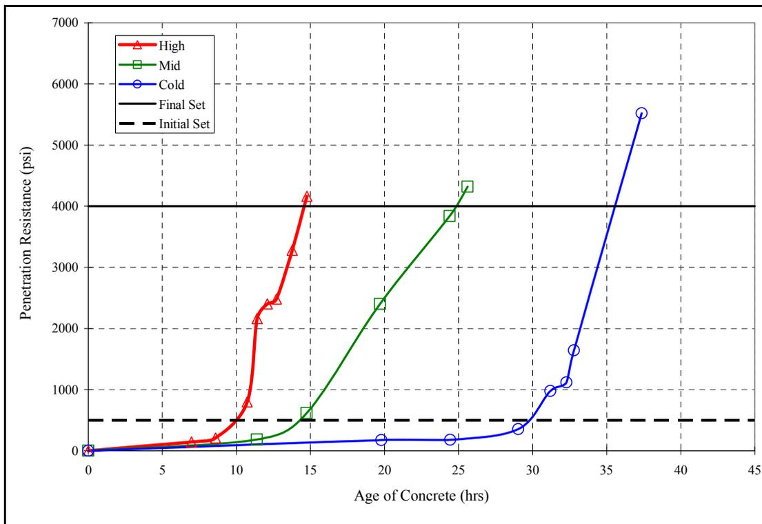
Figure D-10: Penetration resistance vs. time: El Paso mix (w/c = .48)
