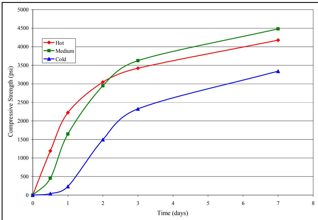
Figure 4.7: Compressive strength vs. time: mix 1 (control mix-OPC)
