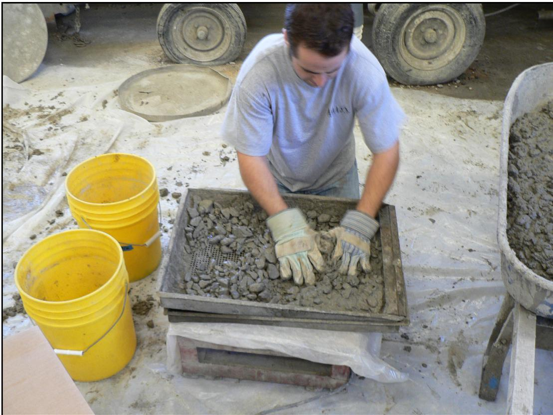
*Figure 3.2: Sieving concrete to produce mortar specimens for setting time determination*
