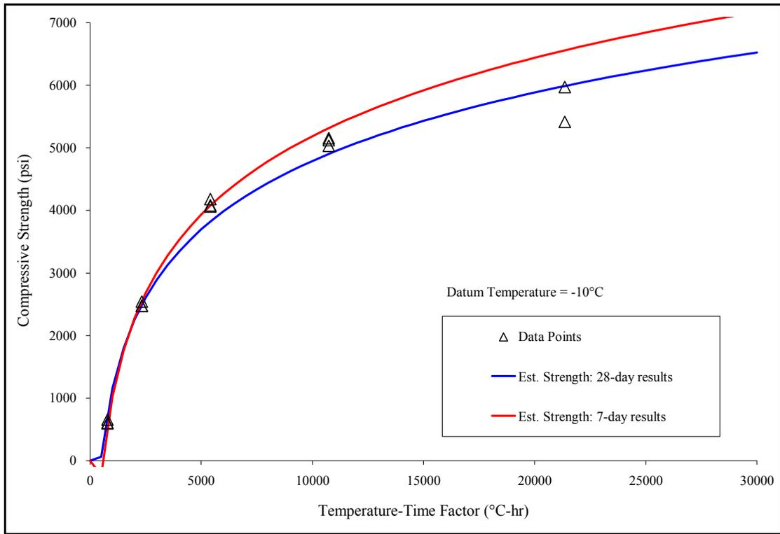
Figure C-8: Compressive strength vs. TTF: Mix 8 (35% Slag, 15% FAI)
